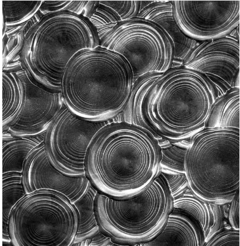
Fig. 16 A quasi-random Pixelmelt pattern of melt pools on the top surface of PBF-EB tungsten, imaged by scanning electron microscopy (Courtesy Freemelt)
