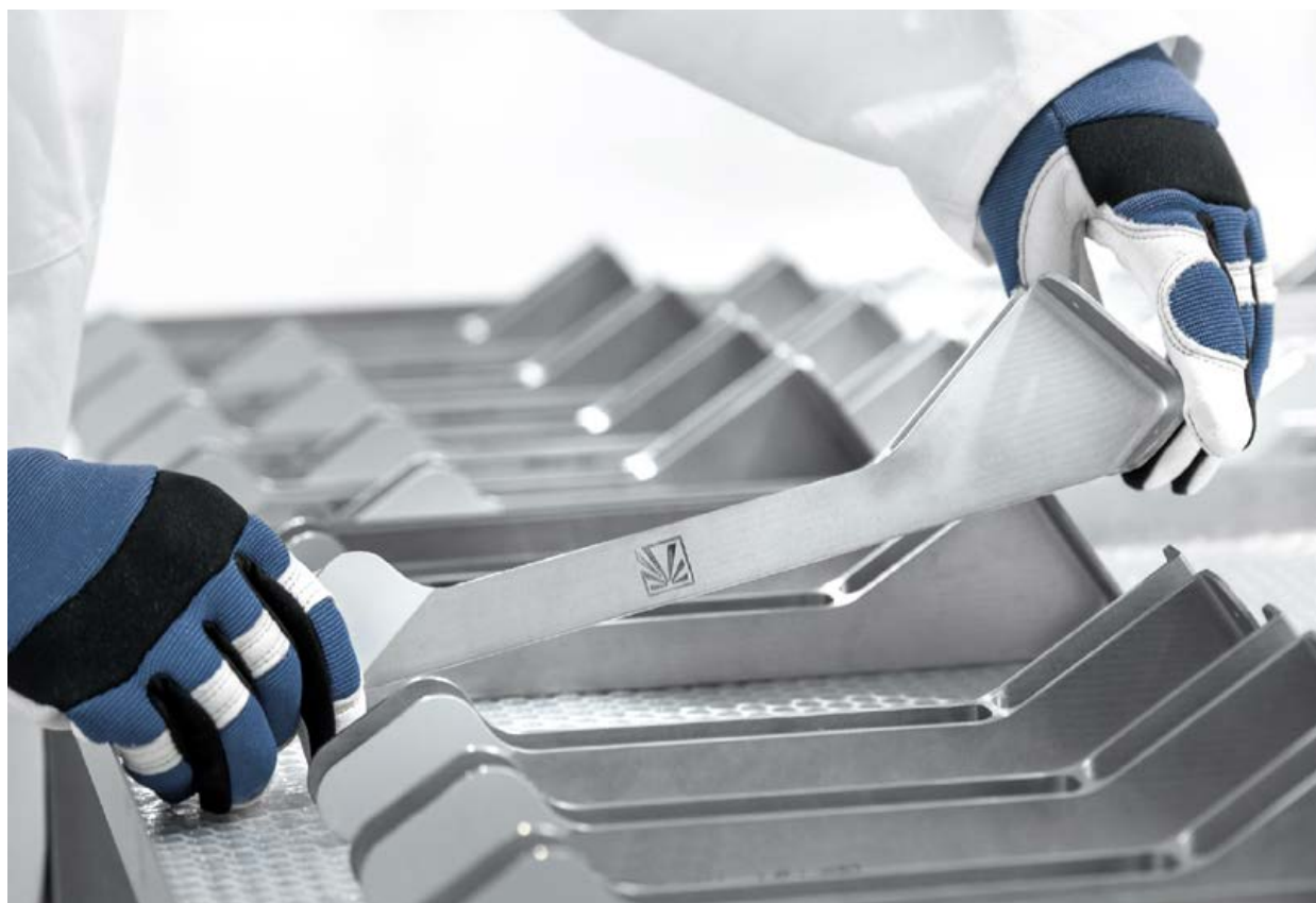
Fig. 13 An aft galley part for the Boeing 787 Dreamliner. Each of these aircraft has seven parts produced by Norsk Titanium (Courtesy Norsk Titanium)
