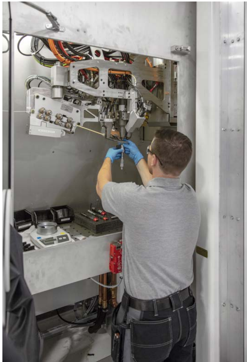
Fig. 5 Changing a consumable in a Merke IV machine. The three PBF-LB components used in the deposition system are clearly visible (Courtesy Norsk Titanium)
