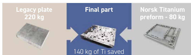
Fig. 18 Illustration of the potential savings when using AM for semiconductor applications (Courtesy Norsk Titanium)
