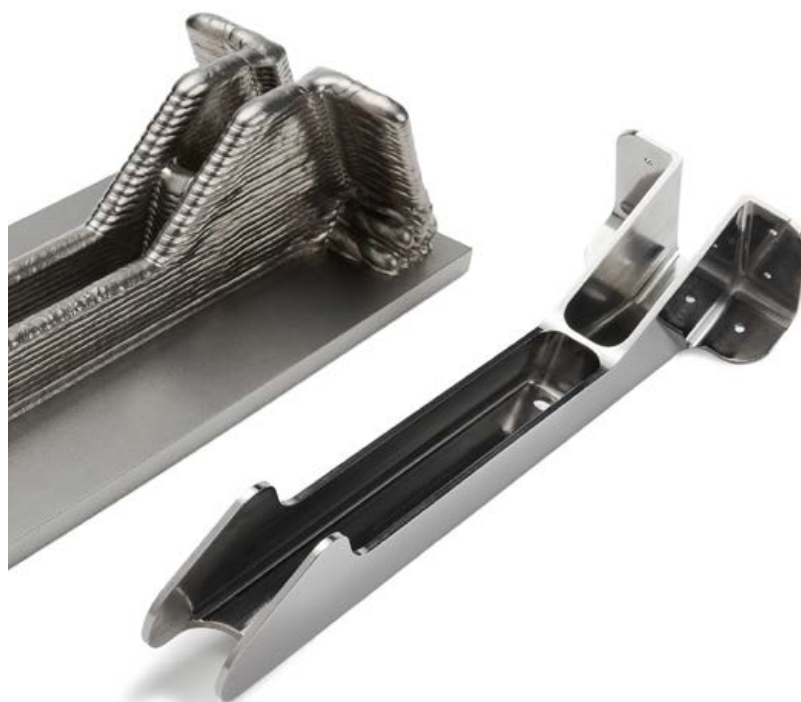
Fig. 14 Detail showing an as-built and machined galley part for the Boeing 787 Dreamliner (Courtesy Norsk Titanium)
