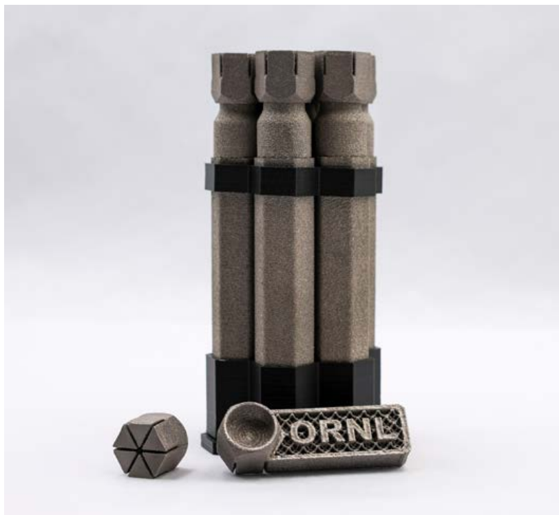
Fig. 8 PBF-EB built diverter geometry with tungsten plasma facing tiles (Courtesy ORNL)
