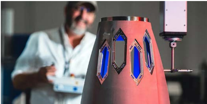
The Mako missile's guidance section was optimised via Additive Manufacturing (Courtesy Lockheed Martin)
