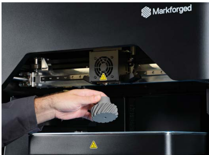
The new FX10 Metal Kit is reported to make the FX10 the world's first industrial AM machine that can process both metal filaments and composites with continuous fibre reinforcement (Courtesy Markforged)
