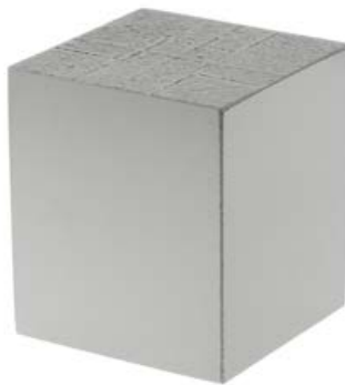
Fig. 11 Tungsten cube, 30 x 30 x 30 mm, built in Freemelt ONE®. The side surfaces have been polished afterwards and do not show any porosity or cracks. The density is estimated at >99.8% based on density measurements of similar cubes (Courtesy Freemelt)
