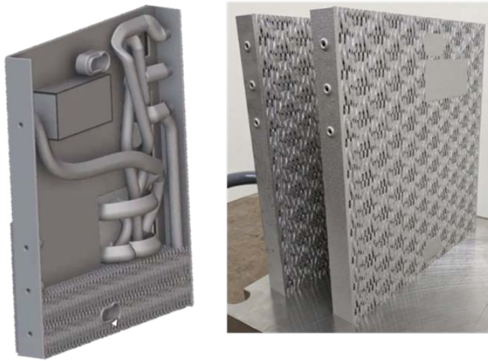
Fig. 4 Computational design (left) and a complex additively manufactured gas delivery manifold solution (right) for thin-film processing equipment (Courtesy Veeco Instruments)
