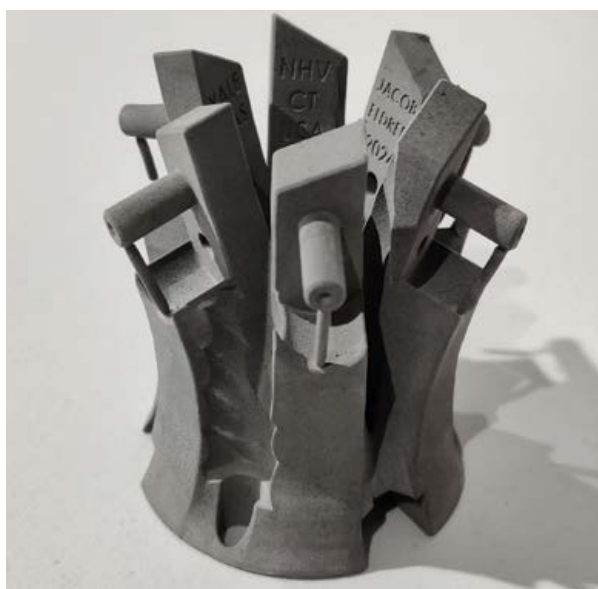
Incus has additively manufactured a stainless steel 316L part for a ceremonial mace for Yale University's School of Engineering (Courtesy Jacob Eldred and Kristin Wagner)
