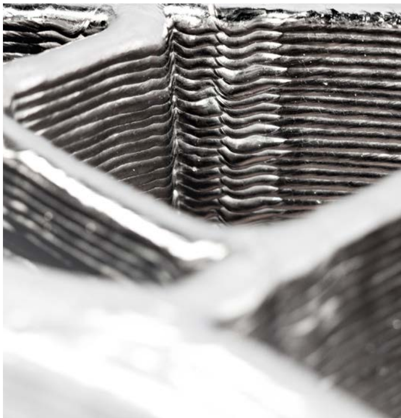
Fig. 4 Detail of an as-built component prior to finish machining (Courtesy Norsk Titanium)
