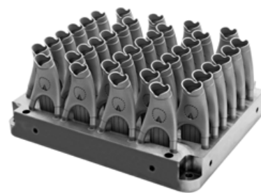
Hanglun aims to additively manufacture over 50,000 titanium bicycle components annually, for use in both high-volume production and custom models (Courtesy Farsoon/Hanglun)
