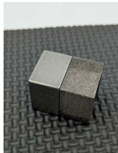
Example of PECM's finishing capabilities on Inconel 738 (Courtesy Voxel Innovations)
