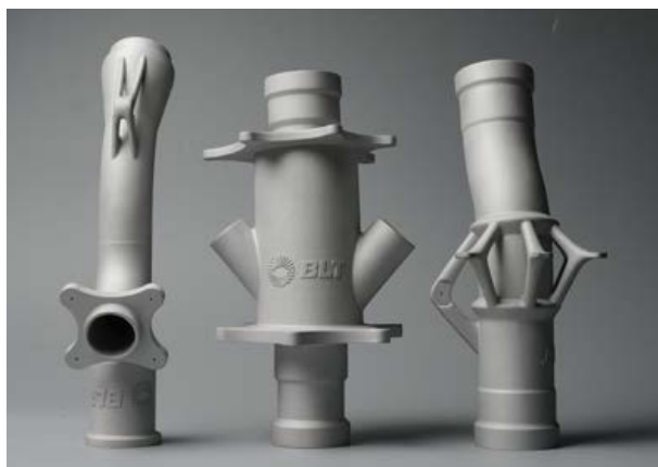
The bent tube, ventilation duct, and connecting pipe are additively manufactured from BLT-ALAM500 aluminium alloy powder (Courtesy BLT)
