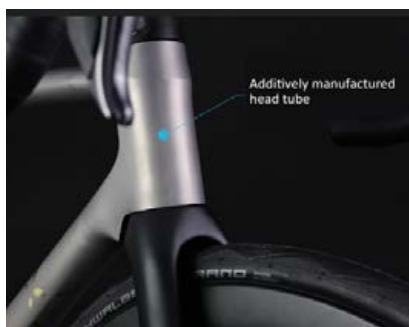
Additive Manufacturing allows for the seamless integration of complex structures into a single piece (Courtesy Farsoon/Hanglun)
