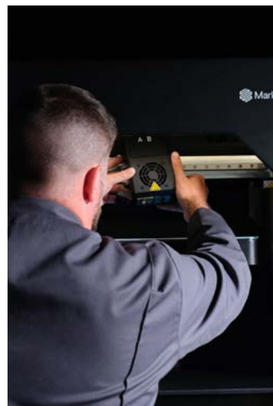
The FX10 can be swapped between metal or composite in around 15 minutes (Courtesy Markforged)
