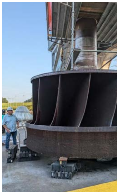
ORNL's Jay Tiley inspects a hydroelectric runner from TVA's Cherokee Dam. ORNL is partnering with TVA and others to develop a process to produce large metal components like this for clean energy applications (Courtesy Jim Tobin/ORNL, US Dept. of Energy)
