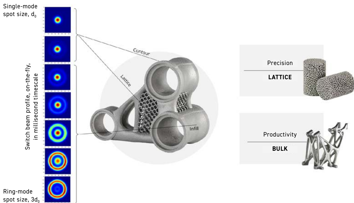
Fig. 3 Choosing the right beam shape for the geometry (objects shown are for illustrative purposes only) (Courtesy EOS GmbH)
