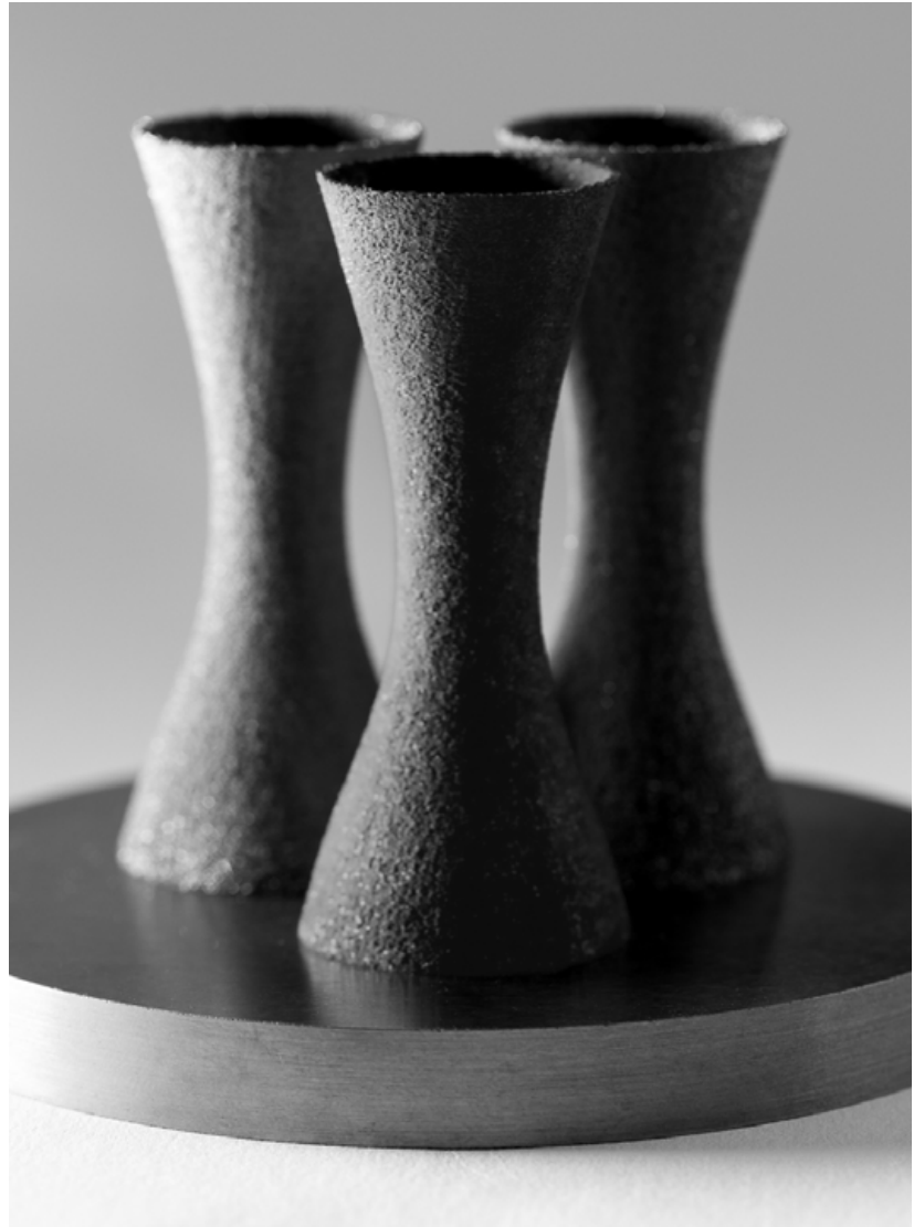
Fig. 13 Tungsten nozzles built in eMELT® (Courtesy Freemelt)
