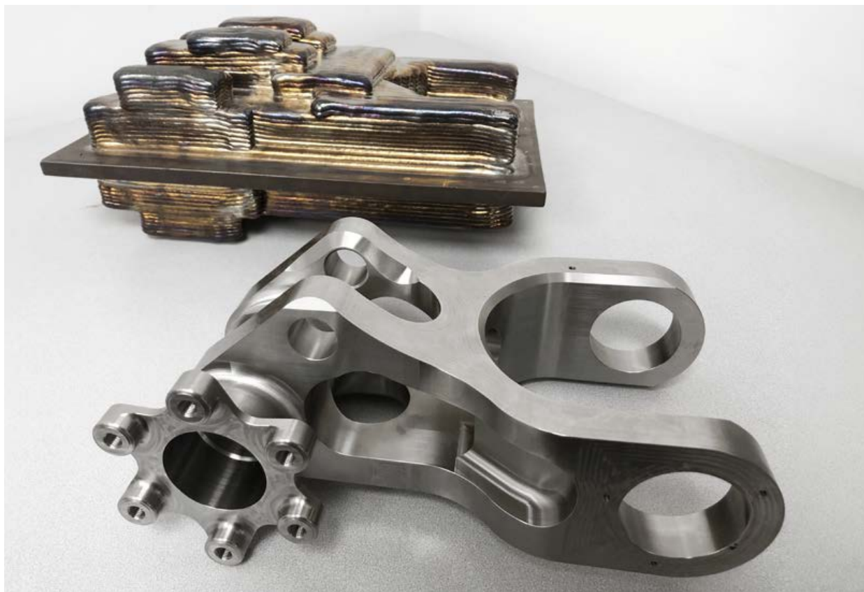
Fig. 15 DED Ti-6Al-4V landing gear structural component as an as-built preform and post-machined, delivering significant cost and lead-time savings compared to the legacy component. Note the double-sided use of the build plate for efficient fabrication (Courtesy General Atomics Aeronautical Systems Inc (GA-ASI))
