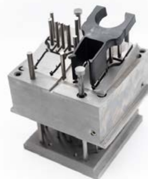
Heyco Products operating its Mantle machine (left). Heyco-printed tool for a deep-ribbed consumer product (right). (Courtesy Heyco Products)
