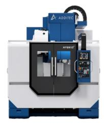
The new Hybrid 3 combines both Liquid Metal Jetting and laser-based Directed Energy Deposition with CNC machining (Courtesy ADDITEC)
