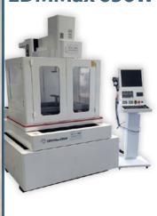
630x500x625 mm (x,y,z axis) - 4 axis Max. workpiece Wt: 1000kg . 2200 lbs
