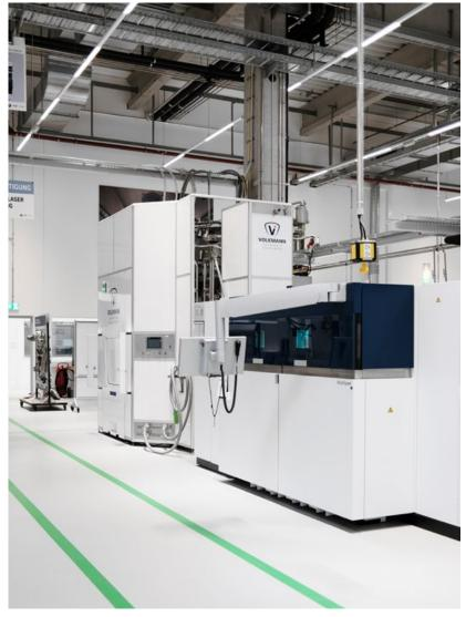
Fig. 6 A Volkmann centralised powder recovery and reconditioning unit to which all production PBF-LB machines are connected. Pipework to and from each AM machine passes overhead across the main thoroughfare
