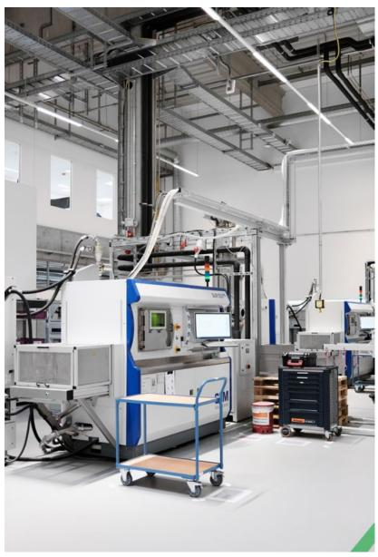
Fig. 5 Two SLM 500 HL PBF-LB Additive Manufacturing machines from Nikon SLM Solutions at BMW's AM campus
