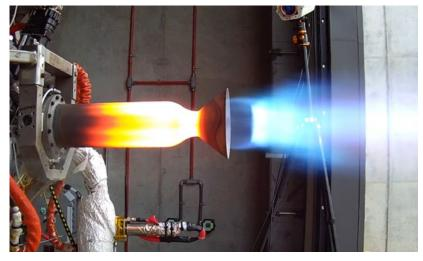
Intuitive Machines rigorously tested the nozzles under hot fire testing conditions, burning fuel up to the full throttle (Courtesy Intuitive Space/Sciaky)
