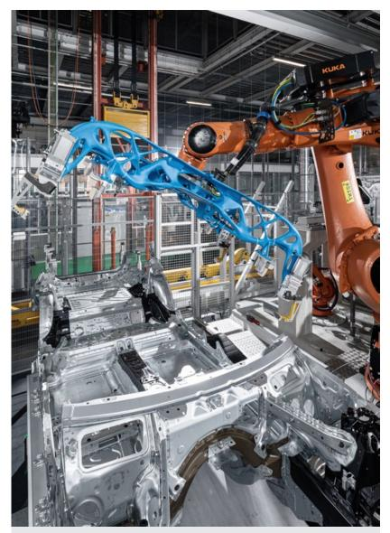
Fig. 15 This very large robotic gripper tool, cast in aluminium using additively manufactured sand cores for the castings, was reduced in weight by a factor of three to just 50 kg (Courtesy BMW)
