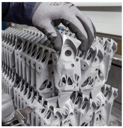
Fig. 4 Series production parts being separated in a tightly-packed PBF-LB build (Courtesy BMW)
