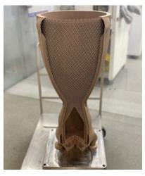
Sintavia has been awarded a US DoD contract to additively manufacture hypersonic propulsion components (Courtesy Sintavia)
