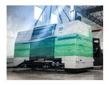
Hyliion has installed a GE Additive XLine Additive Manufacturing machine at its Austin headquarters (Courtesy Hyliion)
