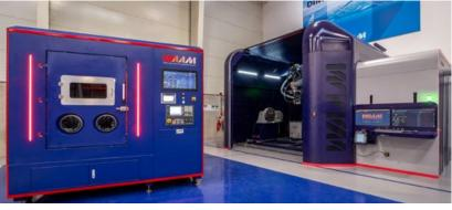
WAAM3D has added the MiniWAAM to its range of wire-based Additive Manufacturing machines (Courtesy WAAM3D)
