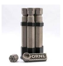
Researchers have used AM to produce defect-free complex tungsten parts for use in extreme environments (Courtesy Oak Ridge National Laboratory)
