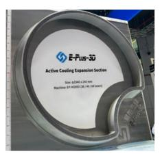
The EP-M2050 large format multi-laser metal Additive Manufacturing system has a 64-laser option. Seen right is a cooling component built on the new machine (Courtesy Eplus3D)
