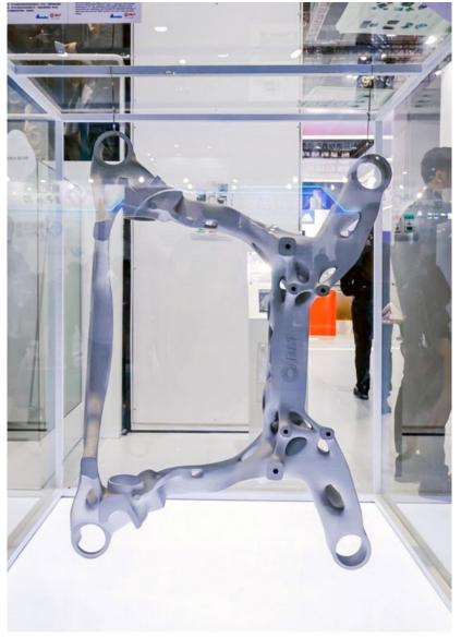
Fig. 4 This rear subframe of an electric vehicle uses what BLT calls a Bi-directional Evolutionary Structural Optimization (BESO) to create a topology with superior performance. The entire parametric design/optimisation process features a high degree of automation. The final part adopts a hollow lattice filling structure with a wall thickness of 2 mm and the part is 20% lighter than a die-cast aluminium alloy alternative. The part measures 1,230 mm x 845 mm x 337 mm (Courtesy BLT)
