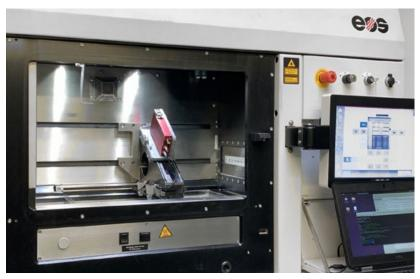
Fig. 1 An EOS M290 Laser Beam Powder Bed Fusion machine fitted with the AMiguam Eddy Current W1 device (Courtesy AMiguam)
