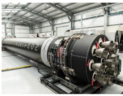
Rutherford engines are used as both first stage and second stage engines on the Electron launch vehicle, with nine engines on the first stage (above) and a single engine on the second stage (Courtesy Rocket Lab)
