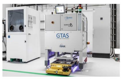
Fig. 7 A fully automated driverless transport systems (FTS), which began as a concept outlined in 2019, is being developed to carry mobile AM build chambers between modules in the IDAM production lines (Courtesy BMW)
