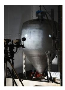
Dimecc has reported the successul testing of its DED-produced pressure vessel (Courtesy Dimecc Ltd)
