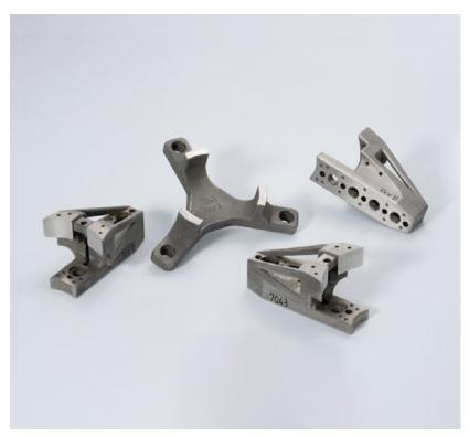
Fig. 7 APG-MIM, a division of Nichols Portland Inc, won an award for these 150 mm pneumatic chuck jaws for work-holding during precision turning. The parts are made by a sinter-based AM process, called Moldjet, developed by Tritone Technologies (Courtesy MPIF)
