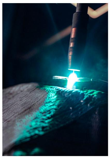
Fig. 10 The wire-based DED process offers significantly faster and cheaper builds than PBF-LB, making it well-suited to large structural elements (Courtesy BMW)
