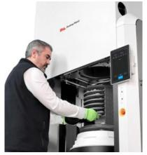
Loading the PureSinter furnace is straightforward (Courtesy Desktop Metal)
