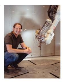
TitanSPEE3D is a large-format metal AM machine (CourtesySPEE3D)
