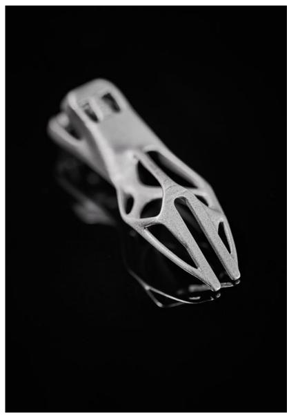
Fig. 13 This bracket, made for the convertible roof mechanism of the i8 Roadster, was manufactured as a left and right pair in AlSi10Mg. The metal part is lighter, and stiffer, than the proposed plastic part with which it competed (Courtesy BMW)
