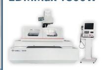
1000x800x1050 mm (x,y,z axis) - 4 axis Max. workpiece Wt: 2000kg . 4400 lbs
