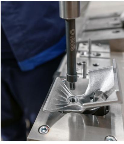
Fig. 18 Pre-assembly operations on a PBF-LB chassis component (Courtesy BMW)
