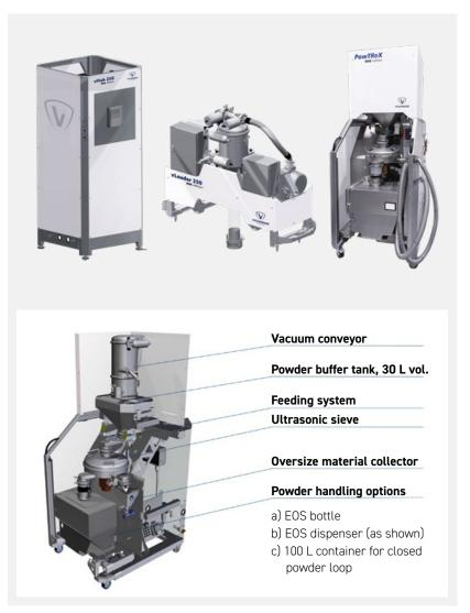
Fig. 3 Components of the Volkmann Automated Powder Handling Solution – EOS Edition, including interior details of the PowTReX – EOS Edition (Courtesy EOS/Volkmann)
