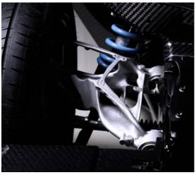
Additive Manufacturing unlocks more efficient geometries for chassis components (Courtesy Bugatti)
