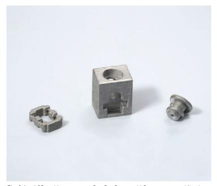
Fig. 8 Azoth3D and its customer, Sur-Set Connect LLC, won an award for these electromedical connector components comprising a set screw, set screw block, and a spring housing. These sinter-based AM parts are made using Xjet's Material Jetting (MJT) process (Courtesy MPIF)
