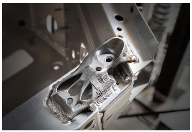
Fig. 14 A structural bracket used on the Rolls-Royce Phantom, demonstrating the weldability of PBF-LB AlSi10Mg (Courtesy BMW)
