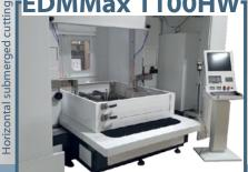
1100x1400x1250 mm (x,y,z axis) Max. workpiece Wt: 3000kg . 6600 lbs
