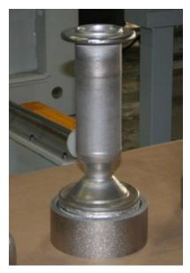
Sciaky additively manufactured the nozzle sections using its wire-based electron beam Directed Energy Deposition technology (Courtesy Intuitive Space/Sciaky)
