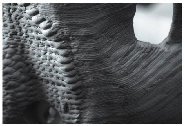
Fig. 11 A close-up view of the surface of the component shown in Fig. 9. BMW has demonstrated that DED components can be used for high loads, including cyclical loads, without any post-treatment of the surface (Courtesy BMW)
