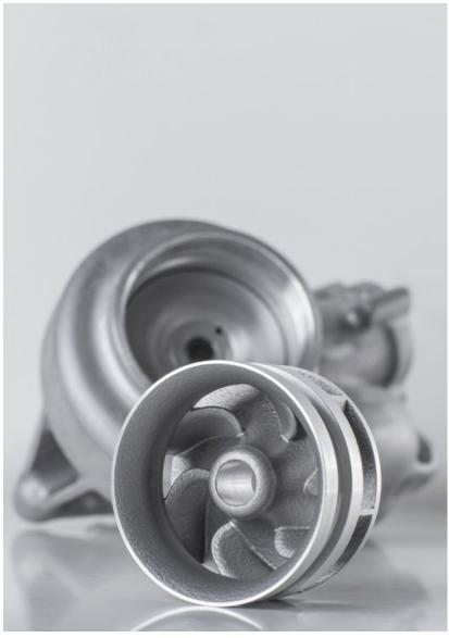
Fig. 3 Publicised back in 2015, this one-piece, lightweight aluminium water pump wheel, produced by Laser Beam Powder Bed Fusion (PBF-LB), was used in BMW German Touring Car Masters (DTM) vehicles as well as Z4 GT3 customer vehicles (Courtesy BMW)
