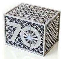
A team from LLNL developed a method for detecting and predicting strut defects in additively manufactured metal lattice structures during the build stage. Pictured is a sample lattice structure, celebrating the lab's seventieth anniversary, built by Gabe Guss (Courtesy Jean-Baptiste Forien/LLNL) ensure quality, scientists typically perform a post-build inspection, which takes time and is not always possible, especially with complex builds.
