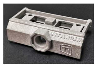
TriTech Titanium Parts LLC is producing titanium alloy Ti6Al4V parts, such as the one shown here, on its Production System AM machine (Courtesy Desktop Metal/Business Wire)
