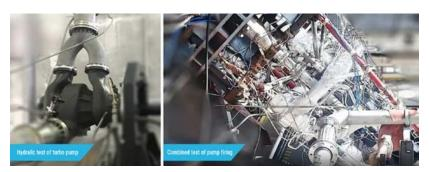
A series of functional tests were conducted on additively manufactured components at Galactic Energy (Courtesy Falcontech)
