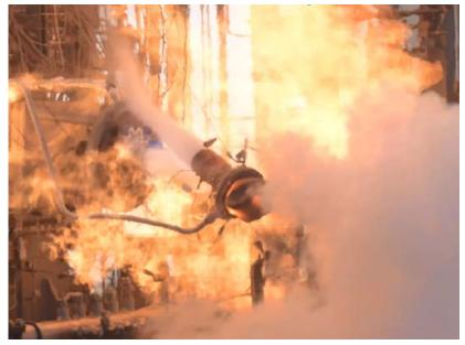
Fig. 4 Premature disassembly of the LLAMA GRCop-42 chamber during the ninth test (Courtesy NASA)
