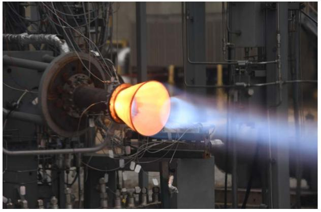
Fig. 3 Successful hot-fire test of a LLAMA GRCop-42 PBF-LB chamber and experimental C-C nozzle (Courtesy NASA)
