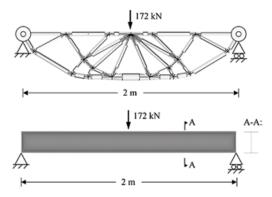
The topologically optimised DED beam (top) compared to the conventional hot-rolled I beam (Courtesy Journal of Cleaner Production)
