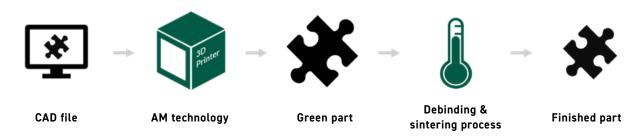
Fig. 2 Process chain of sinter-based Additive Manufacturing Technologies (Courtesy MetShape)
