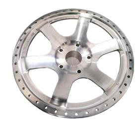
Fig. 4 A metal AM wheel produced by Cold Spray Additive Manufacturing (Courtesy SPEE3D)
