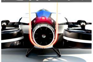
The Thunderstrike hydrogen turbogenerator incorporates an AM combustor (Courtesy Alauda Aeronautics)
