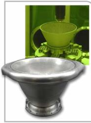
Laser/powder DED of integral channels for NASA HR-1 nozzle
