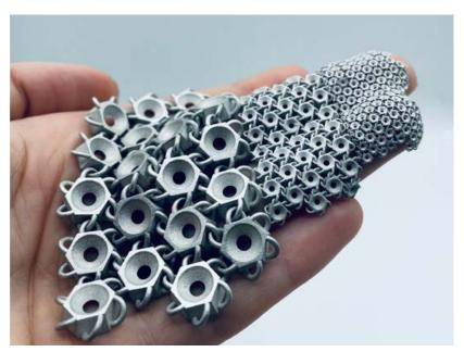
Fig. 1 Additively manufactured steel chain in three sizes, produced via LMM, in the as-sintered stated prior to surface polishing (Courtesy Incus)
