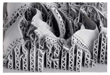
Fig. 5 Detail of a group of dental products on the build plate showing the support structures that are required (Courtesy 3D Systems)
