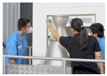
Fig. 2 Deep Blue Aerospace employees examine an as-built combustion chamber produced on Farsoon's FS621M PBF-LB machine (Courtesy Farsoon Technologies)
