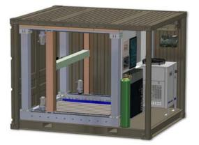
Snowbird's SAMMTech DED machine is incorporated in a shipping container, allowing use at point of need (Courtesy Snowbird Technologies)
