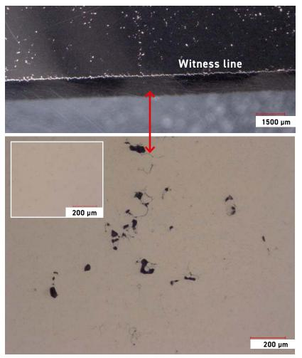
Fig. 9 Top, witness lines observed in chamber samples; bottom, optical microscopy of porosity, with an inset control sample from an ideal PBF-LB GRCop-42 build (Courtesy NASA)
