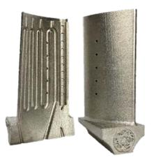
Uniformity Labs has introduced optimised parameters for PBF-LB manufacturing its IN718 nickel alloy (Courtesy Uniformity Labs)
