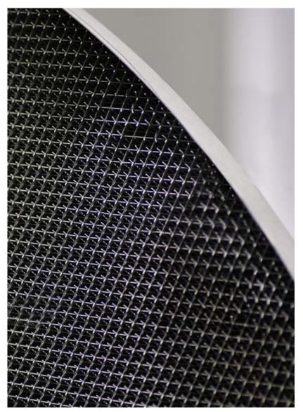
*Fig.* 4 Lattice structure of the hydrazine bottle adapter additively manufactured by BLT (Courtesy BLT)
