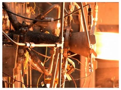
Fig. 1 NASA Marshall Space Flight Center (MSFC) is taking full advantage of AM for rocket propulsion systems to reduce time-to-test and iterations through the design-fail-fix cycle (Courtesy NASA)
