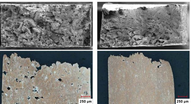
Fractured micro-tensile sample from suspect witness line
