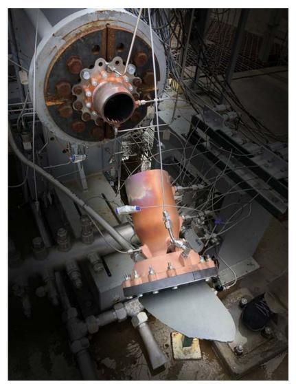
Fig. 5 Separated LLAMA chamber after the test shut down (Courtesy NASA)
