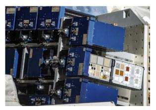
The Materials International Space Station Experiment (MISSE) Flight Facility on the exterior of the space station exposes L3Harris' materials to the harsh environment of space (Courtesy NASA)
