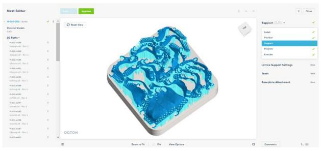
Fig. 4 Oqton's software automates part orientation, support generation, labelling and nesting, helping to prepare quality parts in record time to gain unprecedented control over the entire workflow, from design to manufacturing (Courtesy Oqton)
