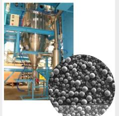
**HERMIGA - Vacuum Inert Gas** Atomiser (VIGA) supplied by PSI Ltd www.psiltd.co.uk
