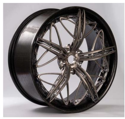
Fig. 12 Metal AM car wheel (Courtesy Ascension Design)
