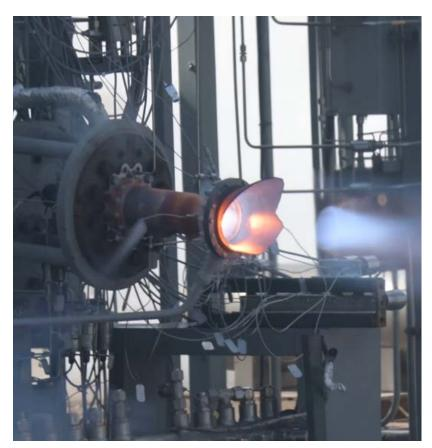
Fig. 6 Video capture showing the moment the chamber leaked in the barrel (Courtesy NASA)
