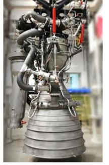
The Welkin reusable LOX/Kerosene Engine has undergone full system testing (Courtesy Galactic Energy)
