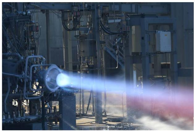
Fig. 12 Successful hot-fire test of an AM thrust chamber including PBF-LB Alloy 718 injector, PBF-LB GRCop-42 chamber, and DED-LB/powder NASA HR-1 regeneratively-cooled nozzle under LLAMA (Courtesy NASA)
