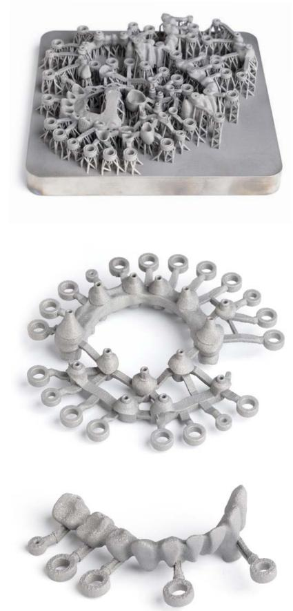
Fig. 3 Examples of titanium hybrid manufacturing for 'print & mill' supported by CIM Systems (Courtesy 3D Systems)
