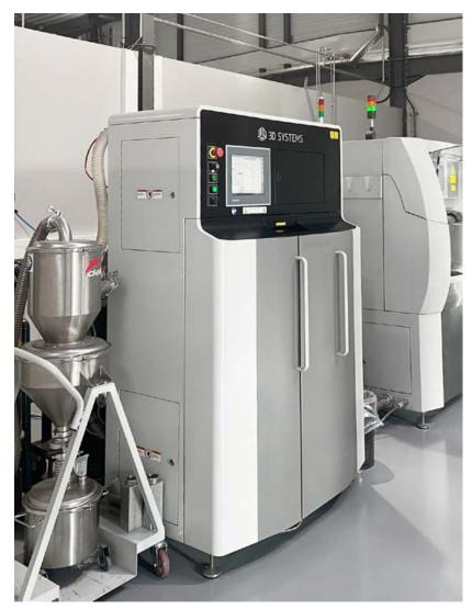
Fig. 6 A 3D Systems DMP Flex 200 metal AM machine, installed at Dent All Group's facility in Lyon, France, is enabling fast dental application cycles for the production of next day RPDs, crowns, bridges and implant bars (Courtesy Dent All Group)
