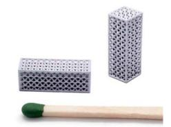
Stainless steel micro lattice structures developed by VCS for an experiment on capillary action in microgravity on the ISS (Courtesy Qualified3D)
