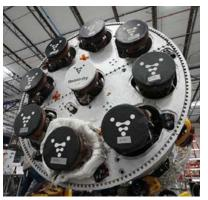
The Terran 1 has a total of nine Aeon engines in its first stage (Courtesy Relativity Space)
