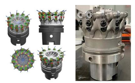
Finishing hybrid AM tool on Seco's HSK100 (Courtesy Seco Tools)
