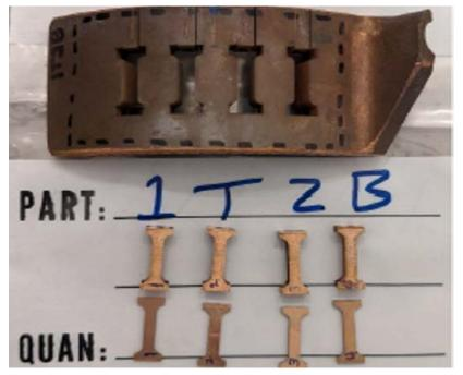
Fig. 8 Microtensile specimens excised from an untested chamber at location of the suspect witness line (Courtesy NASA)
