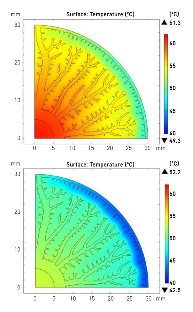
Fig. 5. The heat sink made of aluminium shown on the top has a significantly higher (average) temperature (59.3°C) compared to the multi-material heat sink shown on bottom (52.1°C) (Courtesy Fraunhofer IAPT)
