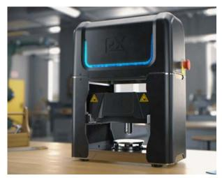
Plastometrex's equipment for profilometry-based Indentation Plastometry (PIP) will be used for the testing of parts made by metal Additive Manufacturing (Courtesy Plastometrex)
