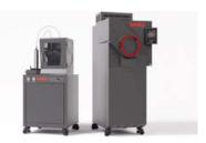
Rapidia's Conflux 1 system consists of a metal AM machine and vacuum sintering furnace (Courtesy Rapidia)
