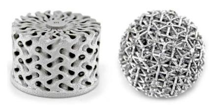
Fig. 1 Examples of 6000 series aluminium parts additively manufactured using Binder Jetting (Courtesy Ricoh)
