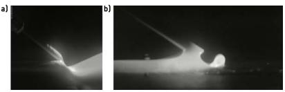
Image of the wire DED-EB processes from the XVC-1000 HDR camera. a) shows a view perpendicular to the build of a wall with leading wire and good parameters for a liquid bridge, while b) shows trailing wire and turbulent deposition (Courtesy pro-beam)
