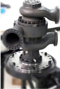
The additively manufactured turbo pump assembly for hydraulic testing (Courtesy Falcontech)
