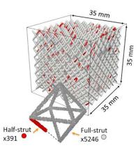
Schematic of the experimental setup and sample design lattice additively manufactured using an octet truss unit cell. The lattice structure contains intentional full and top-half struts randomly positioned. Horizontal struts as well as vertical walls were omitted in the rendering for clarity (Courtesy Jean-Baptiste Forien, et al, "Detecting missing struts in metallic micro-lattices using high speed melt pool thermal monitoring", Additive Manufacturing Letters)
