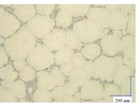
Fig 3 Microstructure of the 6000 series aluminium sample parts (Courtesy Ricoh)
