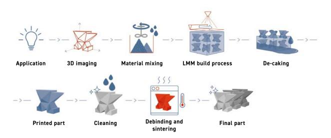
Fig. 3 Process chain in Lithography-based Metal Manufacturing or VPP (Courtesy Incus)
