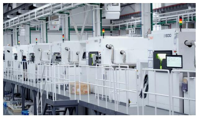
Fig. 5 BLT-S600 metal AM machines (Courtesy BLT)
