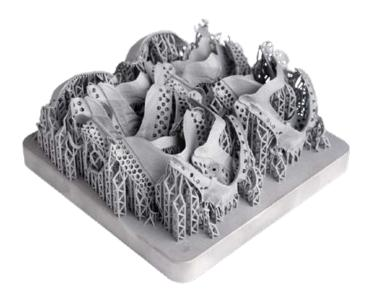
Fig. 1 Full platform with removable partial dentures in CoCr, manufactured on the DMP Flex 200 (Courtesy 3D Systems)
