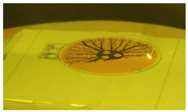
Fig. 4 Powder bed and scanning process of the multi-material heat sink (Courtesy Aerosint)
