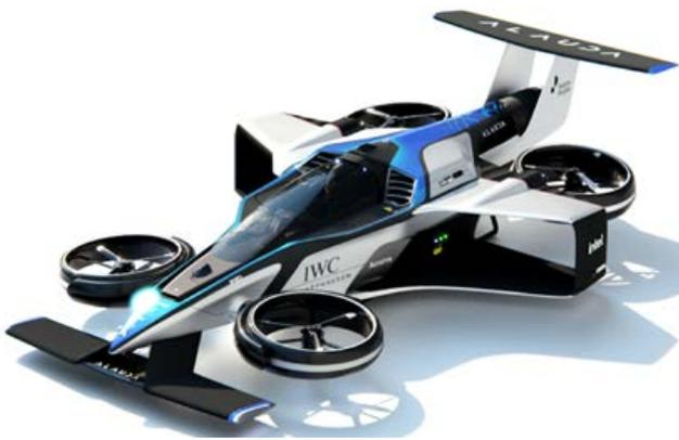
The Airspeeder Mk4 is the world’s first crewed electric flying race car (Courtesy Alauda Aeronautics)
