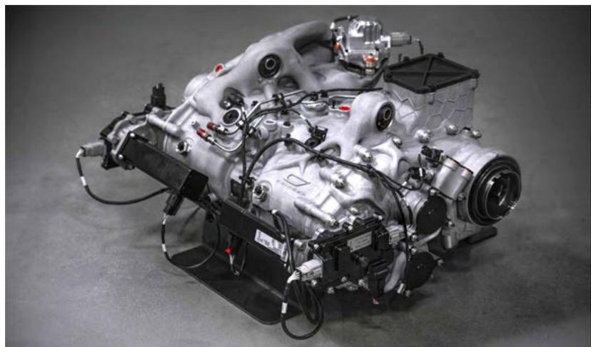
*The additively manufactured gearbox is currently undergoing validation in the Czinger 21C and Vmax hypercars (Courtesy Czinger Vehicles)*
