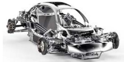
*The Czinger 21C incorporates over 350 metal additively manufactured components and structures throughout the car, from the vehicle's chassis to brake, suspension and exhaust components (Courtesy Czinger Vehicles)*
