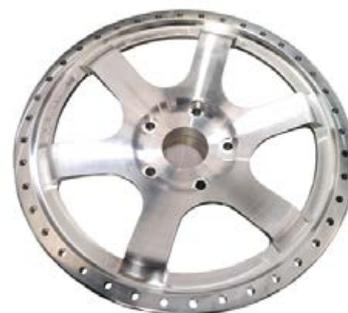
*This 9 kg wheel centre is manufactured in just under 6 hours on a WarpSPEE3D (Courtesy SPEE3D)*
