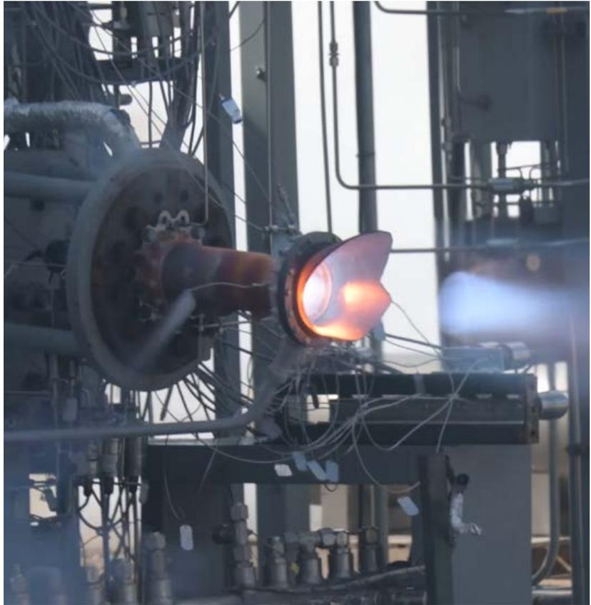
Fig. 6 Video capture showing the moment the chamber leaked in the barrel (Courtesy NASA)
