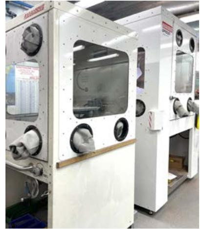
AviaTools has developed a line of depowdering machines for the AM industry (Courtesy AviaTools)
