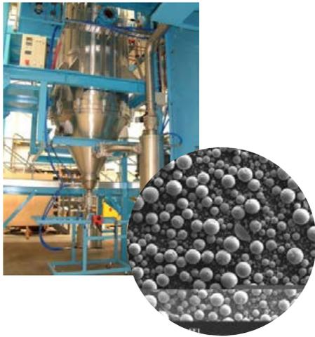
**HERMIGA - Vacuum Inert Gas Atomiser (VIGA) supplied by PSI Ltd**
