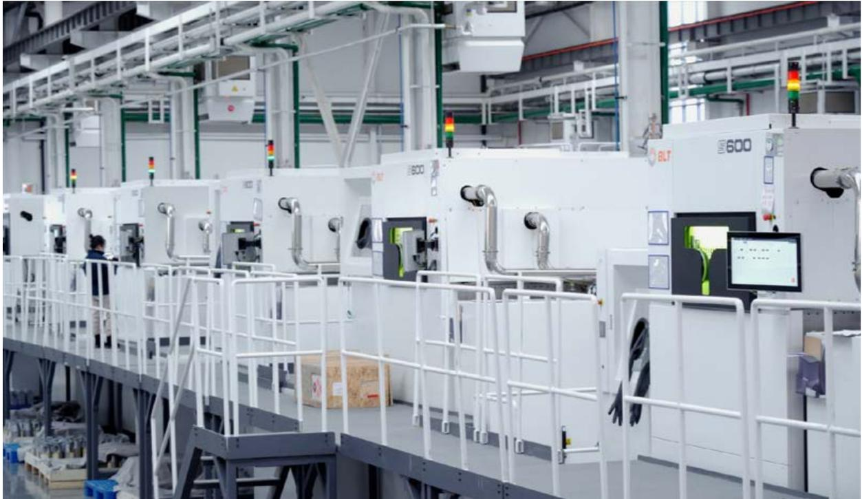
Fig. 5 BLT-S600 metal AM machines (Courtesy BLT)
