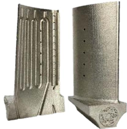
*Uniformity Labs has introduced optimised parameters for PBF-LB manufacturing its IN718 nickel alloy (Courtesy Uniformity Labs)*
