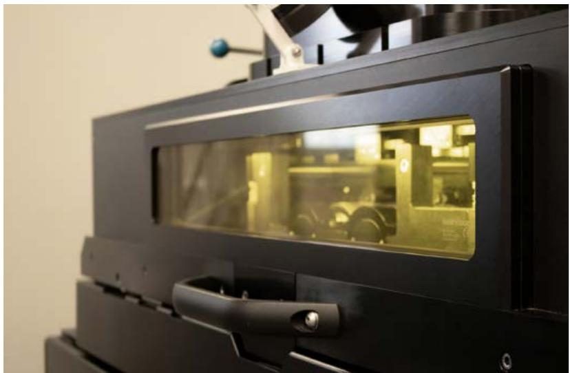
*Fig. 1 Aerosint's Selective Powder Deposition (SPD) system installed on a MIDI+ machine supplied by Aconity3D GmbH (Courtesy Aerosint)*
