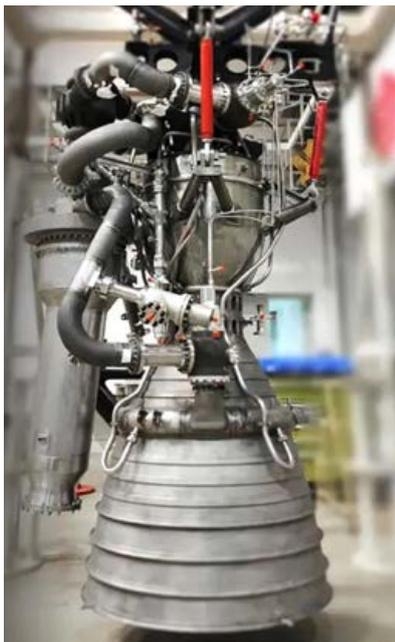
The Welkin reusable LOX/Kerosene Engine has undergone full system testing (Courtesy Galactic Energy)
