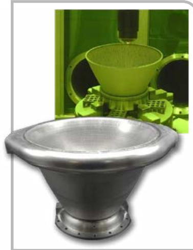
**Laser/powder DED of integral channels for NASA HR-1 nozzle**
