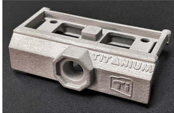
TriTech Titanium Parts LLC is producing titanium alloy Ti6Al4V parts, such as the one shown here, on its Production System AM machine (Courtesy Desktop Metal/Business Wire)
