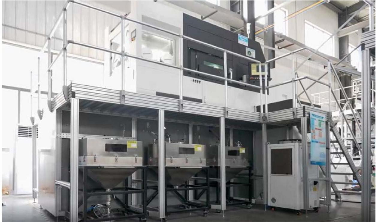
Fig. 8 Farsoon FS621M machine (Courtesy Farsoon Technologies)
