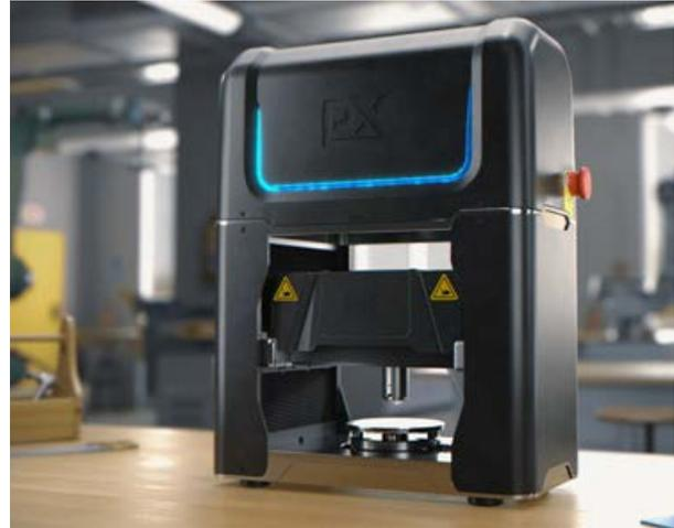
*Plastometrex's equipment for profilometry-based Indentation Plastometry (PIP) will be used for the testing of parts made by metal Additive Manufacturing (Courtesy Plastometrex)*
