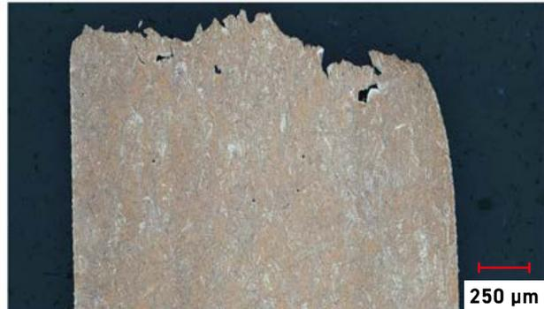
Fig. 11 Tensile results comparing emulated witness line samples and excised samples from chamber (Courtesy NASA)
