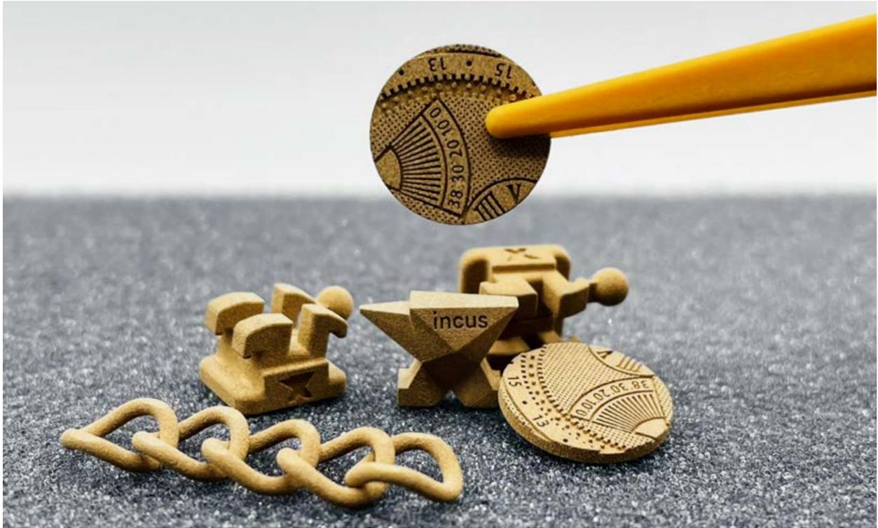
Fig. 12 Red gold "green parts" additively manufactured with LMM (Courtesy Incus)
