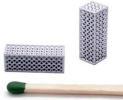
*Stainless steel micro lattice structures developed by VCS for an experiment on capillary action in microgravity on the ISS (Courtesy Qualified3D)*
