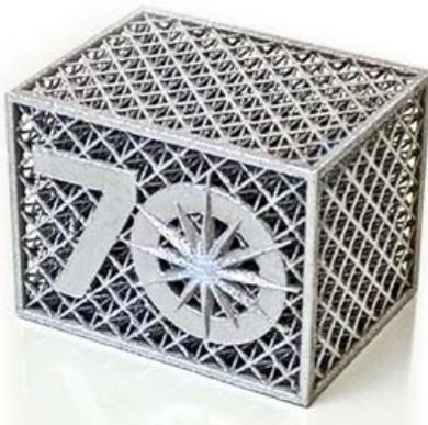
*A team from LLNL developed a method for detecting and predicting strut defects in additively manufactured metal lattice structures during the build stage. Pictured is a sample lattice structure, celebrating the lab's seventieth anniversary, built by Gabe Guss (Courtesy Jean-Baptiste Forien/LLNL)*
