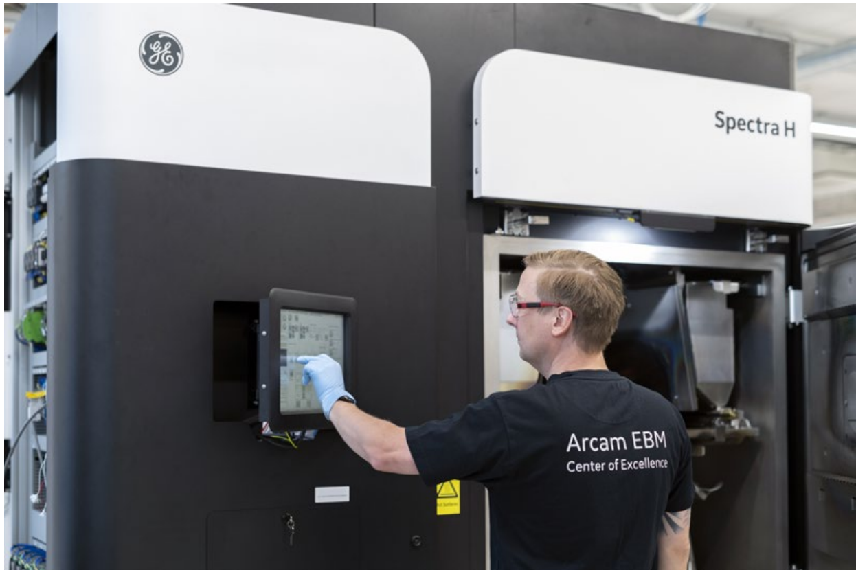
Fig. 10 A GE Additive Arcam PBF-EB machine in operation at the Arcam EBM Center of Excellence (Courtesy GE Additive)
