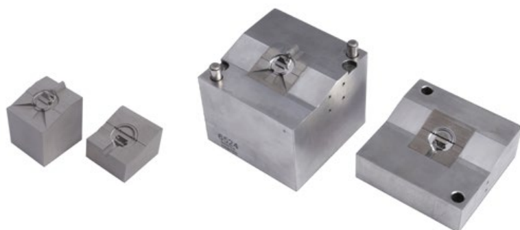
Left: Fathom's cavity and core inserts as additively manufactured with Mantle's TrueShape metal AM technology. Right: Cavity and core inserts after Fathom finished the additively manufactured inserts and assembled them in its modular mould system (Courtesy Mantle)
