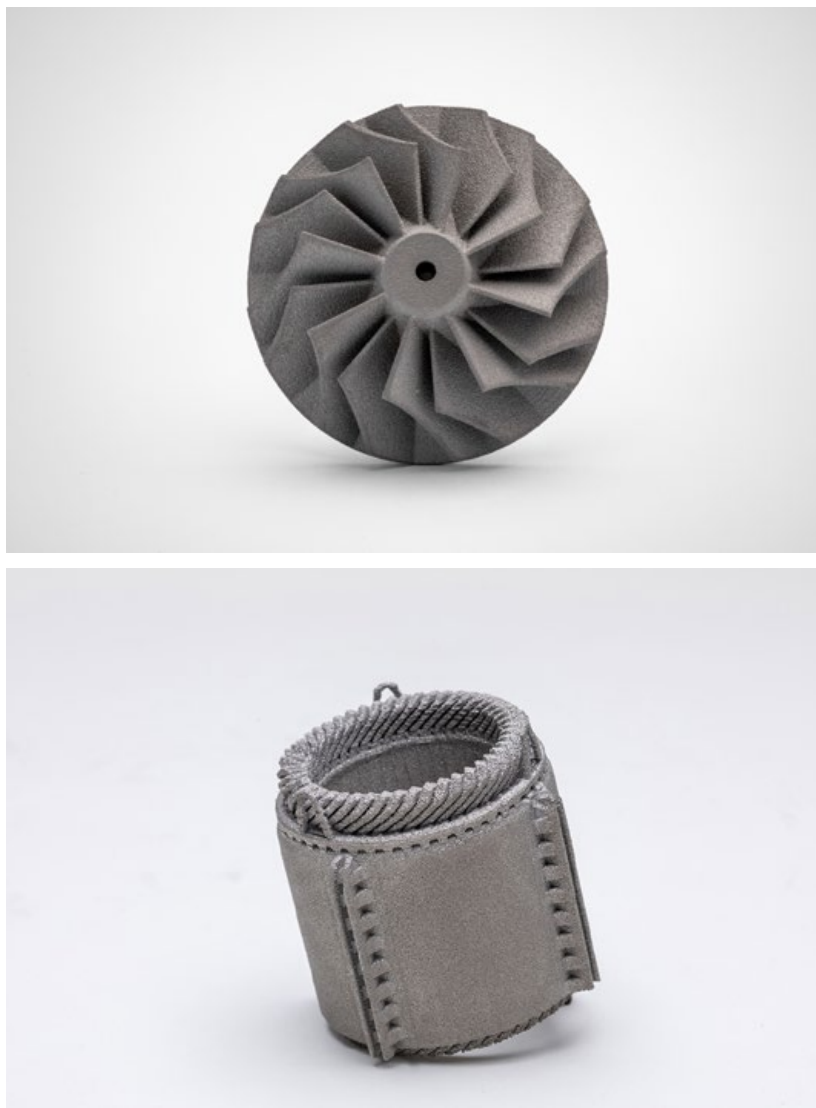
Fig. 6 Parts produced using pro-beam's PBF-EB technology. Top is a turbo-charger component, bottom is a component for an electric motor (Courtesy pro-beam)
