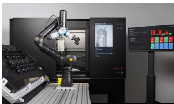
Lumafield's industrial CT scanner with robotic arm for high volume inspection (Courtesy Lumafield)
