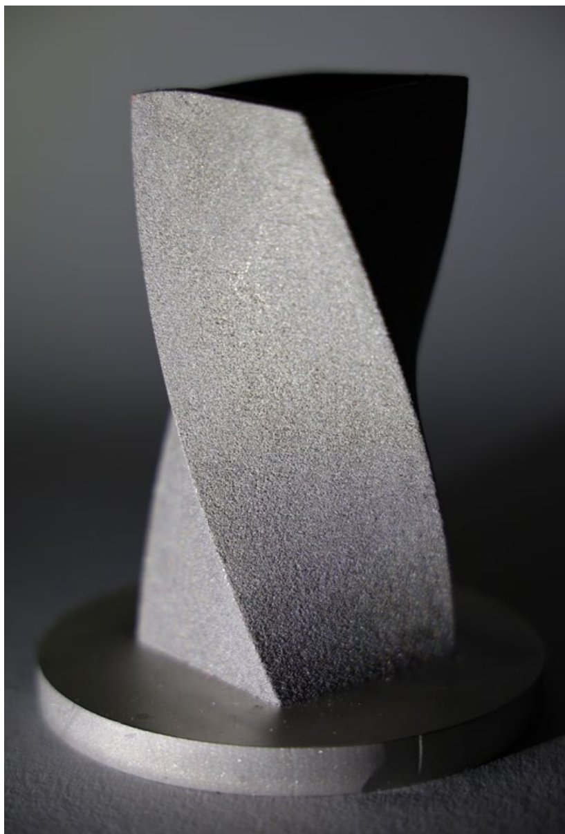
Fig. 13 A demonstrator part built in stainless steel on the Freemelt ONE PBF-EB machine (Courtesy Freemelt AB)
