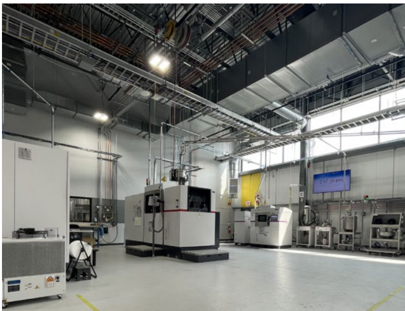
Fig. 5 Views of part of the metals area of the AIC showing EOS M400-4 and M290 metal Laser Beam Powder Bed Fusion (PBF-LB) machines
