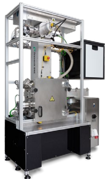
Fig. 8 The Freemelt ONE, Freemelt's first AM machine, was designed for material development and has mainly served academic, government and corporate research facilities (Courtesy Freemelt AB)
