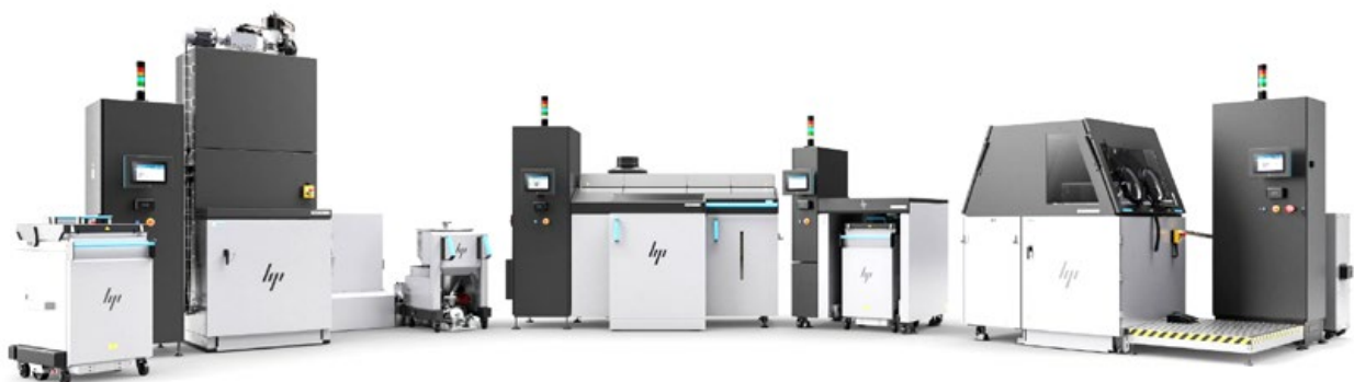
HP's new Metal Jet S100 Solution for metal Binder Jetting, which features multiple modules including depowdering and curing, is now commercially available (Courtesy HP)
