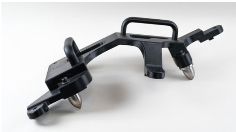
Fig. 4 An example of AM tooling used on automotive production lines, bringing increased safety and productivity benefits (Courtesy Steve Fecht / General Motors)
