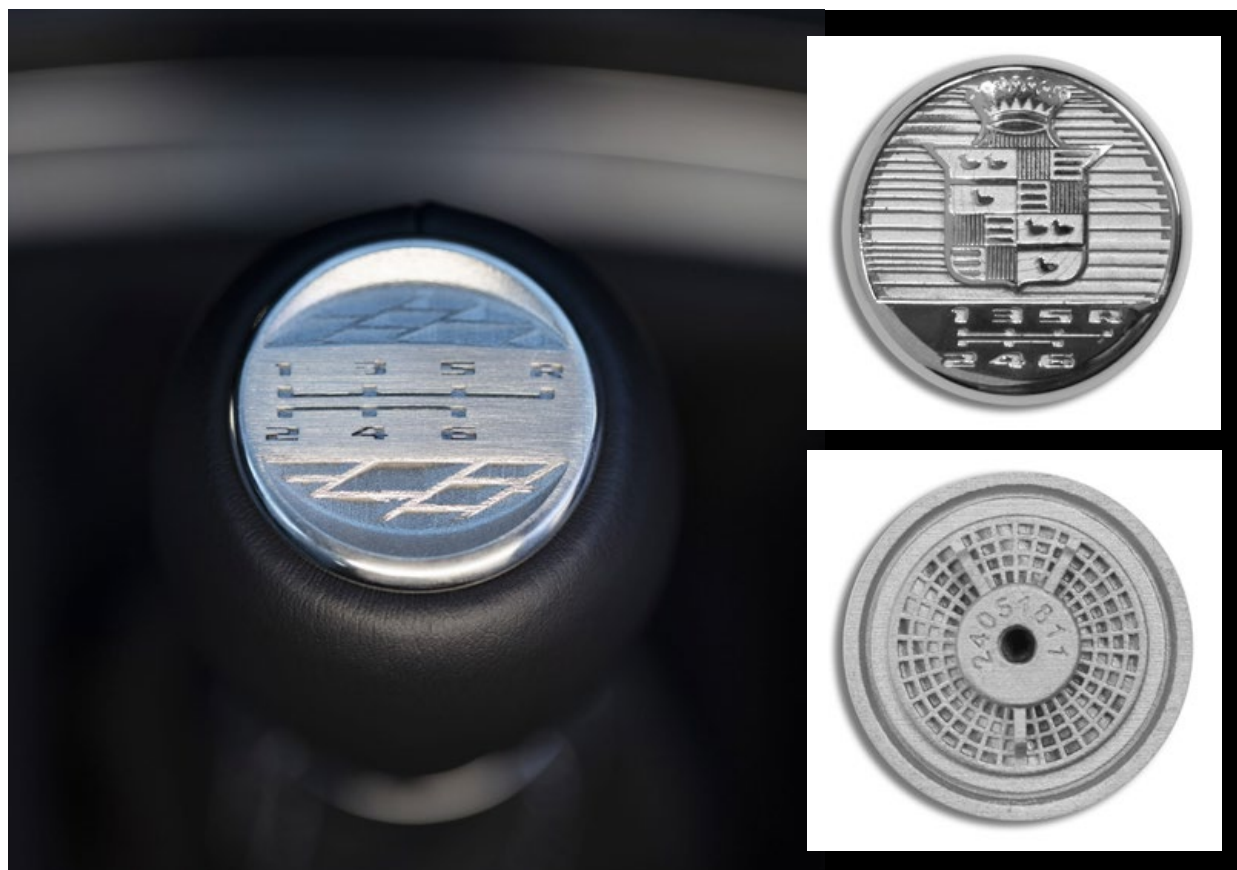
Fig. 7 A metal additively manufactured shifter emblem for the Cadillac Blackwing V-series, produced in stainless steel by Binder Jetting. Top right inset shows a design variant, easily achievable with AM, whilst lower right shows the heat dissipating design on the part's rear (Courtesy General Motors)
