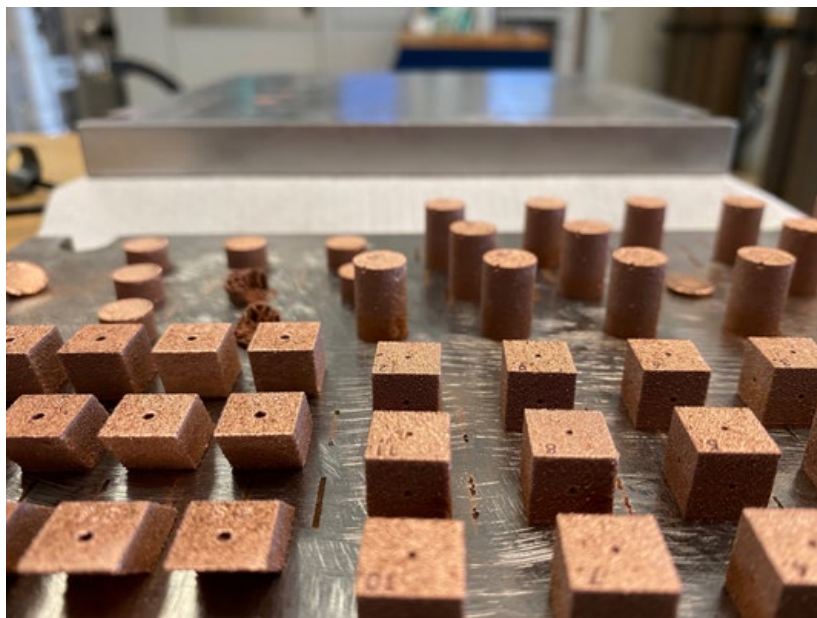
Fig. 7 Experimental build plate for testing process parameters (density, surface roughness) produced on an EOS M290-1 kW machine
