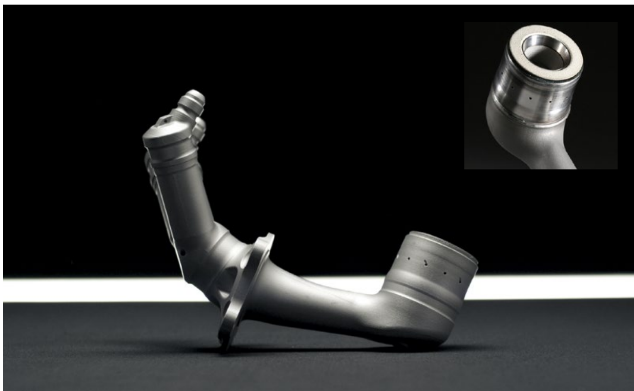
Fig. 2 Rather than twenty pieces welded together, the new tip (inside the punctured ring section, inset) was a single elegant piece that weighed 25% less than its predecessor, and was five times more durable and 30% more cost-efficient (Courtesy GE Aviation)
