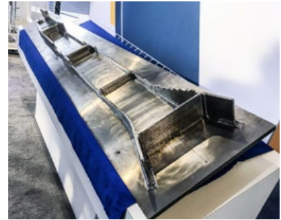
The titanium AM aerostructure component measures around 2.5 m in length (Courtesy GKN Aerospace)
