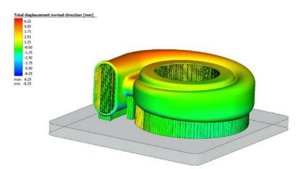
Fig. 1 Simufact Additive has been a class leading solution provider for metal Powder Bed Fusion (PBF) process simulation since its release in 2016. Here, predicted distortion of a turbo-pump housing built on a large format (400 mm) machine is shown
