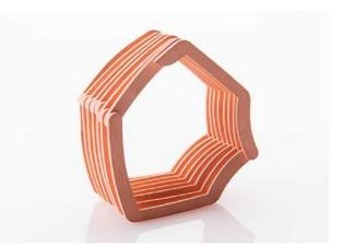
ExOne and Maxxwell have successfully proven a new concept for Binder Jetting a high-efficiency copper e-winding design that eliminates many of the challenges that come with traditional manufacturing of copper coils for electric motors (Courtesy The ExOne Company)
