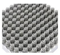
Additive Manufacturing sample on a build plate (Courtesy Zeiss Group)
