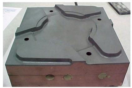
Fig. 2 A 3.18 mm H13 steel surface on a chromium copper block of 254 x 254 x 76 mm (Courtesy Additive Manufacturing Institute of Science and Technology, University of Louisville)
