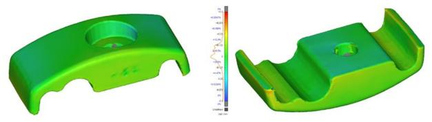
Fig. 9 Shape comparison between scan of compensated geometries post-sintering and nominal geometry for horizontal orientation
