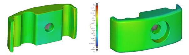
Fig. 10 Shape comparison between scan of compensated geometries post-sintering and nominal geometry for vertical orientation
