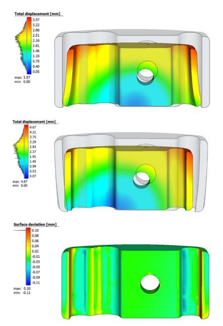
Fig. 2 Top: Distortion of nominal geometry, middle: Distortion of compensated geometry, bottom: Comparison between compensated and nominal
