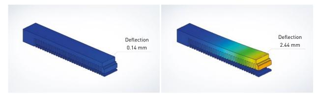
Fig. 3 Preheating the substrate plate to 500°C reduces deflection of the Ti64 cantilever by 95% (left) compared to 200°C (right)
