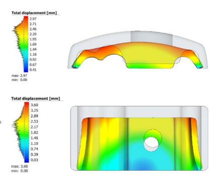
Fig. 5 Simulated deformation of nominal geometry in horizontal and vertical sintering orientations
