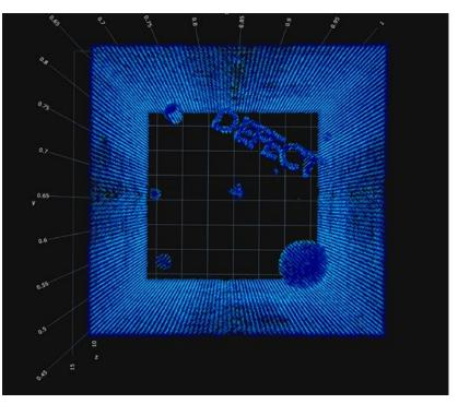
Fig. 3 3D visualisation of the lack of fusion defects, as captured by the melt pool monitor sensors and shown in 3D after MRL construction of the data
