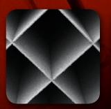
Finest tungston wall structure 100 µm thickness
