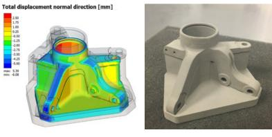
Fig. 6 Simulated deformation and actual sintered nominal steering knuckle geometry with live setter
