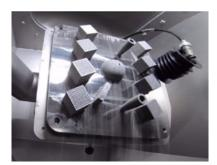
Ultrasonic excitation aims to completely depowder components with particularly narrow internal channels or porous structures (Courtesy Solukon)
