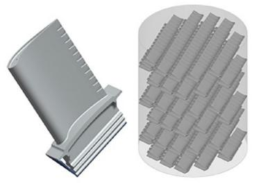
Fig. 2 A simulation of two builds showing when (top) supports are required and (bottom) how support free capability enables 'stacking' of parts. The productivity, specifically the output, of the machine on the right is much higher than the output of the machine on the left
