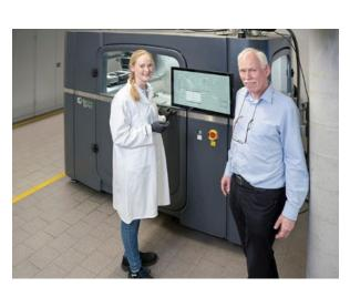
With the new X1 25Pro from ExOne, Prof Frank Petzoldt and his team aim to investigate pilot and pre-series production of components using metal Binder Jetting (Courtesy Fraunhofer IFAM)
