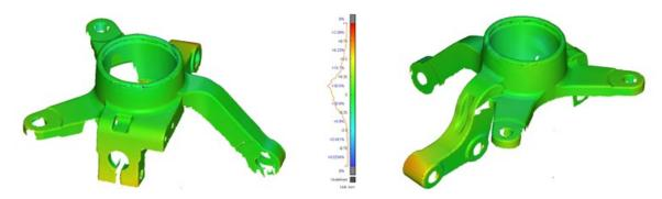
Fig. 11 Shape comparison between scan and simulation predicted final geometry
