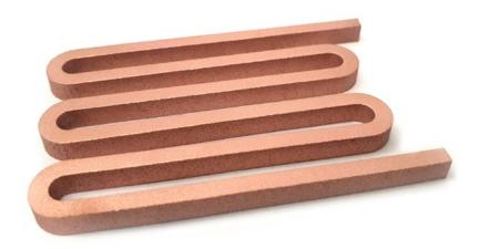
IEC electrical conductivity geometries for future studies investigating electrical conductivity and electromagnetic applications. Manufactured from high purity copper on an EOS M290 machine (Courtesy University of Wolverhampton)
