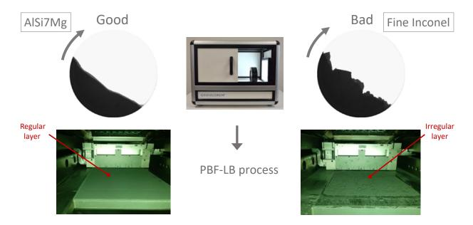
Fig. 4 General principle of how to relate GranuDrum measurements to powder performance inside a PBF-LB machine
