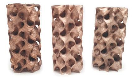
Copper-silver alloy gyroid TPMS structures for investigating EV thermal management and impact protection crashworthiness. Designed in nTopology and manufactured on an EOS M290. Left to right: Cu, CuAg10, CuAg20 (Courtesy University of Wolverhampton)
