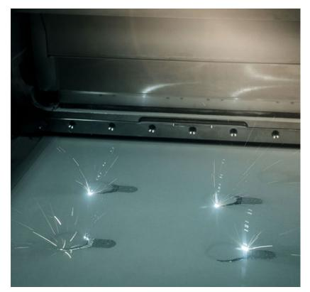
Fig. 3 A four-laser PBF machine in operation (Courtesy EOS)
