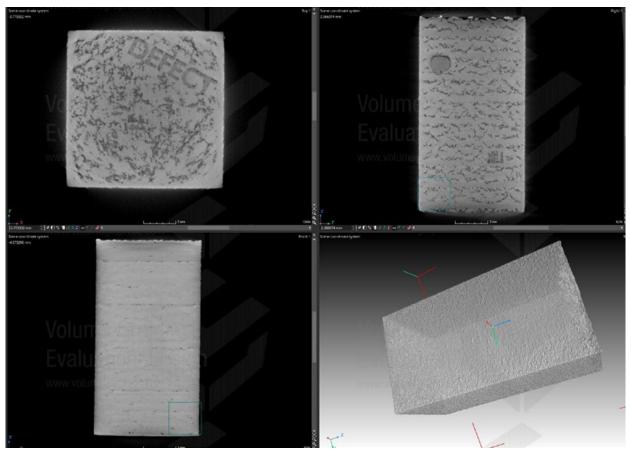
Fig. 2 Screenshot of the scanned data from optimised process parameters built to generate data on lack of fusion defects which is used to establish process maps in 17-4 PH steel
