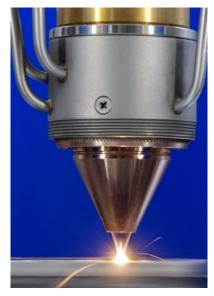
Metal powder melts before reaching the surface (Courtesy Ponticon)
