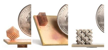
Fabric8Labs' patented process rapidly fabricates complex metal parts at the atomic level, enabling high feature resolution and enhanced material properties (Courtesy Fabric8Labs)
