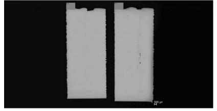
Fig. 5 Right: Cracking in H11 after 200°C preheating and PBF. Left: Crackfree H11 after preheating at 500°C and PBF-LB. In a downstream step, any remaining small defects can be corrected by annealing
