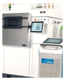
An EOS AM machine equipped with Linde's oxygen monitoring technology (Courtesy Linde)
