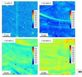
Electron beam microanalysis of the carbon content in the as-built state of the various alloys
