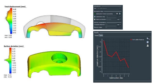
Fig. 7 Final compensated sintered geometry compared to compensated initial geometry, surface deviation, and compensation dialog box showing the max surface deviation of each iteration
