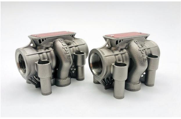
Fig. 7 Small AMES valves for hydraulic systems. AMES are CETOP directional control valves, here additively manufactured in 316L stainless steel and designed to work at 350 bar. These AM valves underwent high-pressure testing up to 1,400 bar (Courtesy Aidro)
