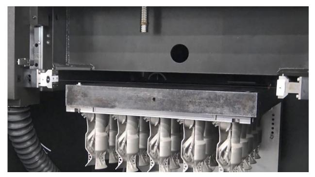
Fig. 2 The CUT AM 500 uses a horizontal rather than vertical cutting process
