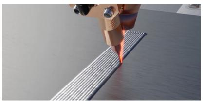
TWI intends its wire-feed head for Directed Energy Deposition to find uses in coatings, freeform AM and the remanufacture & repair of parts (Courtesy TWI)
