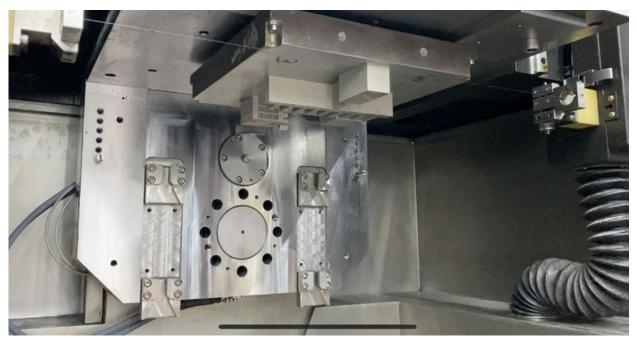
Fig. 5 A benchmark build plate inside the CUT AM 500
