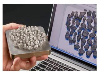
The new Dental Module of Materialise's Magics software offers an automatic manufacturing preparation for common AM dental applications such as crowns, bridges, and partial bases (Courtesy Materialise)
