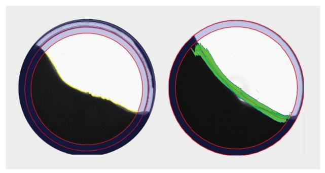
Fig. 3 The GranuDrum offers a customised image treatment algorithm to characterise cohesion
