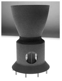
Quadrus Corporation used 6K's services to make spherical tungsten-rhenium used to produce a non-eroding throat insert for a solid rocket motor nozzle (Courtesy 6K Additive/Quadrus Corporation)
