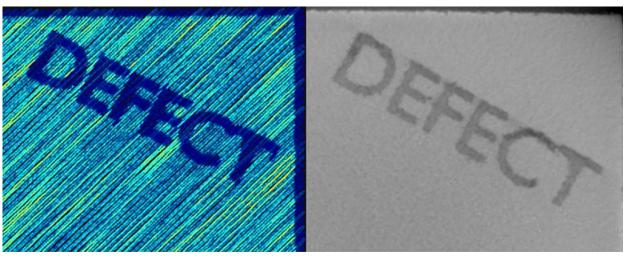
Fig. 4 Co-axial meltpool monitoring sensors stream the temperature of the melt pool. In the visualisation, blue indicates cold melt pools. An artefact of the word DEFECT is clearly visible in the sensor data (left) and is confirmed by the micro CT data (right)
