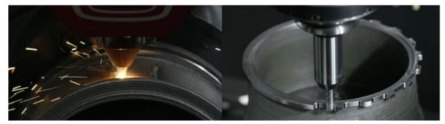
Fig. 1 Hybrid AM showing material deposition (left) and milling (right) (Courtesy DMG Mori)
