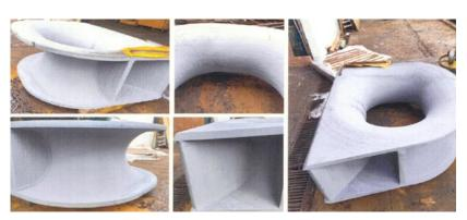
The Panama Chock underwent successful testing, being comprehensively function tested to 20% above its design load (Courtesy DNV)
