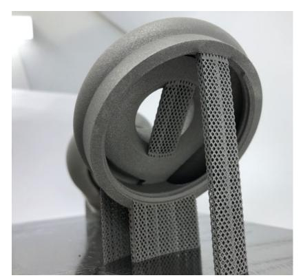
Fig. 6 The turbocharger with standard supports
