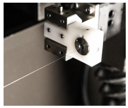
Fig. 3 Molybdenum wire used in the CUT AM 500
