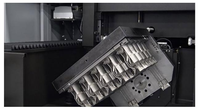
Fig. 4 Once loaded, the CUT AM 500 table inverts the build plate safely into the cutting position
