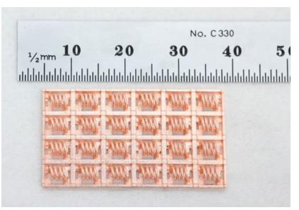
Micro inductor coils additively manufactured in a twenty-four piece array. Twenty such arrays can be additively manufactured simultaneously on one Holo PureForm AM machine (Courtesy Holo)
