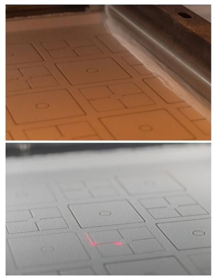
Fig. 5 Top; recoating of AlSi7Mg powder selected after GranuDrum measurements, bottom; PBF-LB in progress
