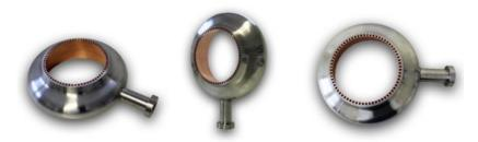
To demonstrate Cold Spray AM's efficacy for rocket engines, a demo sample with the inlet manifold was manufactured. The regeneratively cooled liner is a high-strength Cu alloy, and the outer jacket material is Inconel (Courtesy Impact Innovations)
