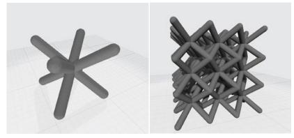
Fig. 1 The most commonly utilised lattice structure model is the body-centred cubic (BCC) structure (Courtesy S Obadimu, University of Limerick)
