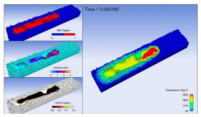
Fig. 4 Metal AM process monitoring and melt pool analysis (Courtesy Flow-3D)
