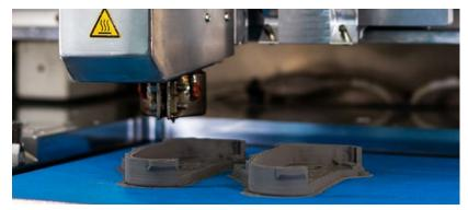
The CEM-E2 extruder allows manufacturing rates of up to 220 cm<sup>3</sup>/h with a 0.4 mm nozzle (Courtesy AIM3D)
