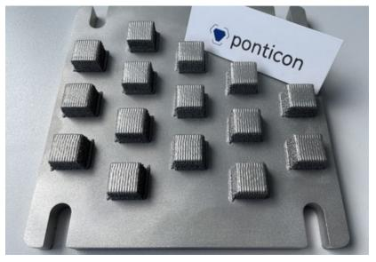
Samples used in the development of new alloys for specific AM applications (Courtesy Ponticon)
