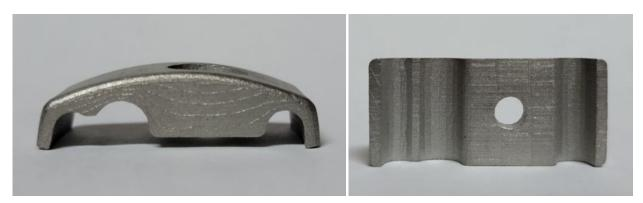
Fig. 8 Compensated, sintered cable fastener in horizontal and vertical orientations
