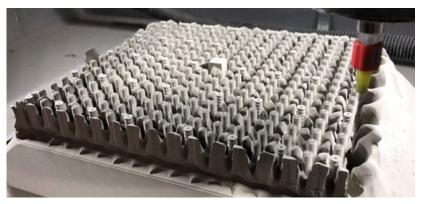
Metal binder jetted parts depowdered (Courtesy Digital Metal)
