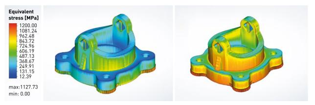
Fig. 4 If a gimbal bearing is additively manufactured with 500°C preheating, the residual stress in the Ti6Al4V component is significantly reduced (left). This opens up completely new possibilities in design, especially in the construction of large components. At 200°C, the internal stress is significantly higher (right); this leads to greater preparation, design reworking and part post-processing, as more simulations and support structures are needed
