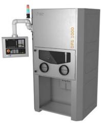
Digital Metal has added the DPS 1000 automated depowdering station for metal Binder Jetting to its AM solutions (Courtesy Digital Metal)
