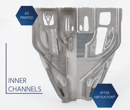
The water based process media can reach all cavities and inner surfaces of the part and can thus enable the full post-processing inside and outside.
