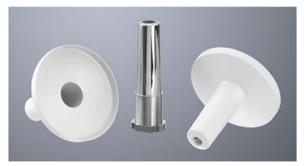
Fig. 6 Highly polished mould core made from H11 by Additive Manufacturing after preheating to 500°C, from Reinhard Bretthauer GmbH. The component is crack-free and has a density of more than 99.9%. The polishability is correspondingly high – no difference can be detected compared to conventional production. Due to the integrated cooling channels, the stable production of plastic injection moulded parts is possible and the cycle time reduced
