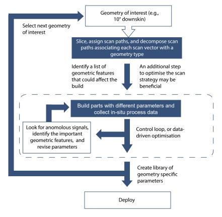
Fig. 3 Workflow for development of machine parameters from the perspective of the machine manufacturer
