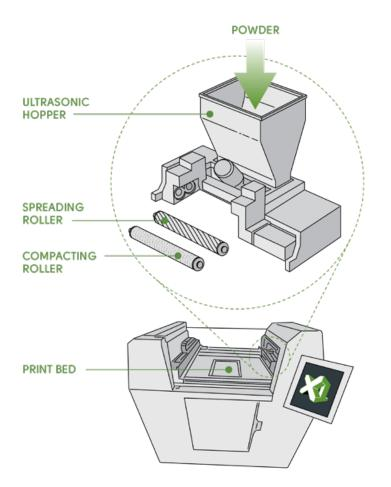
Fig. 4 ExOne's Triple Advanced Compaction Technology (ACT)
