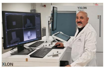
Fig. 1 Ayman Salem, PhD, founder of MRL, shown with the company's Yxlon FF35 CT high-resolution CT system, used for non-destructive testing of additively manufactured materials
