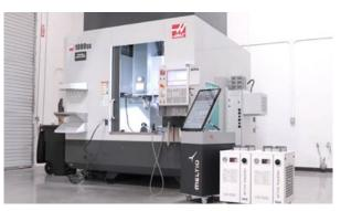
The Phillips Additive Hybrid system brings together CNC machine tooling from Haas with DED AM from Meltio (Courtesy Phillips Corporation)
