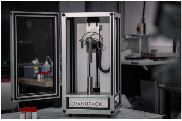
Fig. 7 The GranuPack is fully automated to measure the apparent, tapped density, the so-called Hausner ratio, Carr index and the complete packing curves at high resolution. It comes in two models: the Classic (for measurements at room temperature) and the High-Temperature (for measurements between room temperature and 200°C)
