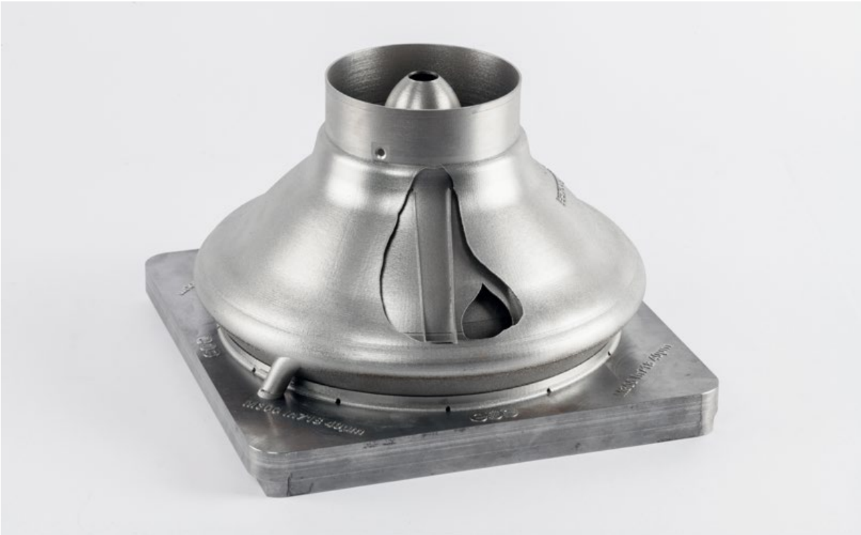
Fig. 4 An aerospace part produced by EOS using state-of-the-art NextGenAM processes (Courtesy EOS)
