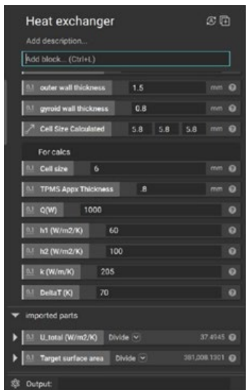
Fig. 4 Creation of gyroid with a cell size and wall thickness to meet specified heat transfer characteristics (left) with a cross section of the TPMS (right).
