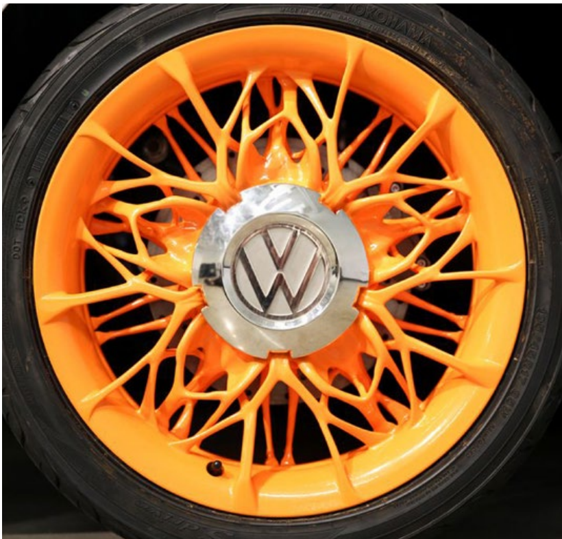
Fig. 6 Generatively designed alloy wheel from Volkswagen (Courtesy Volkswagen Group of America)
