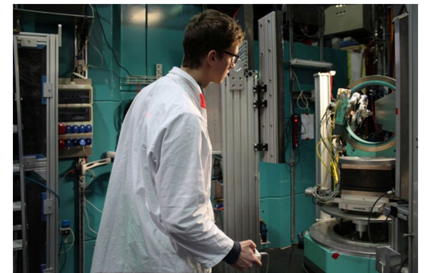
Using the remote control Dr Tobias Fritsch brings the lattice structure into the correct measuring position in the residual stress diffractometer STRESS-SPEC at the research neutron source (Courtesy Dr Michael Hofmann / TUM)
