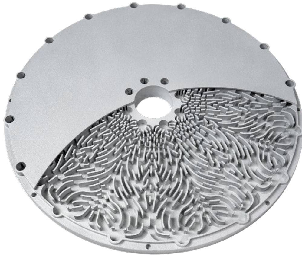
Fig. 4 A silicon wafer table with integrated advanced cooling structures (cut-away section) produced using 3D Systems' DMP Factory 500 (Courtesy 3D Systems)
