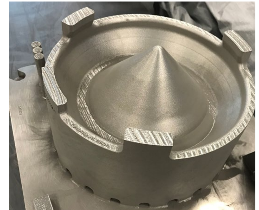
Additively manufactured, cobalt-chrome sump cover for F110 engine. Produced on a GE Additive Concept Laser M2 machine at the GE Additive Technology Center in Cincinnati, as part of collaboration with the US Air Force's Rapid Sustainment Office (Courtesy GE Additive)
