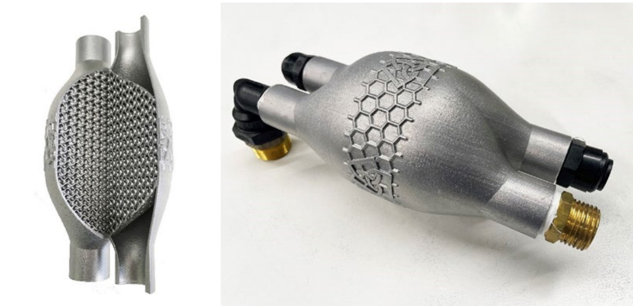
Fig. 7 Additively manufactured heat exchanger section (left) and assembly for testing (right)
