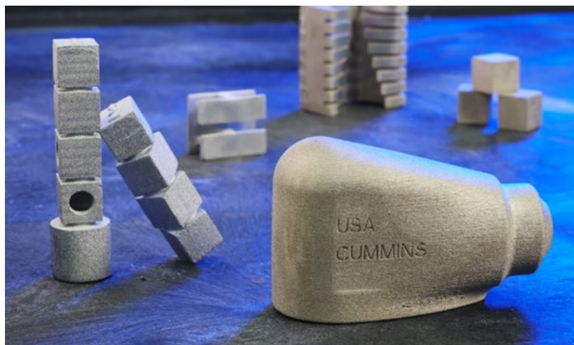
The Cummins Emission Solutions (CES) lance tip adapter is moving through the company's production part approval process (PPAP) for formal approval (Courtesy Cummins Inc)
