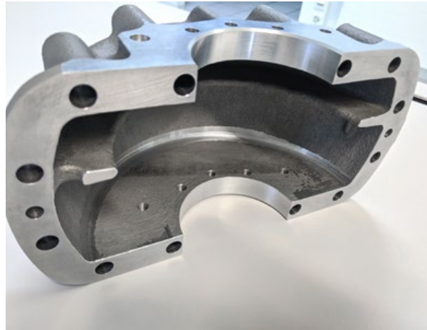
After the build, the gearbox casing was machined to required tolerances (Courtesy Sauber Engineering)
