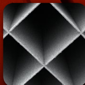
Finest tungsten wall structure 100 µm thickness
