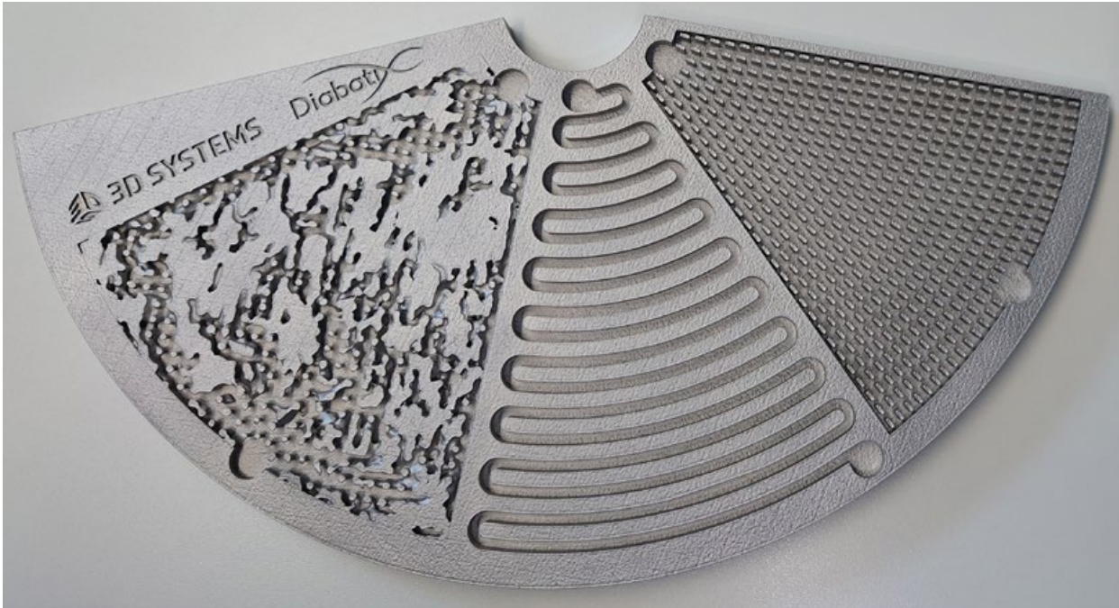
Fig. 15 The final metal additively manufactured cooling strategy demonstrator (Courtesy 3D Systems)
