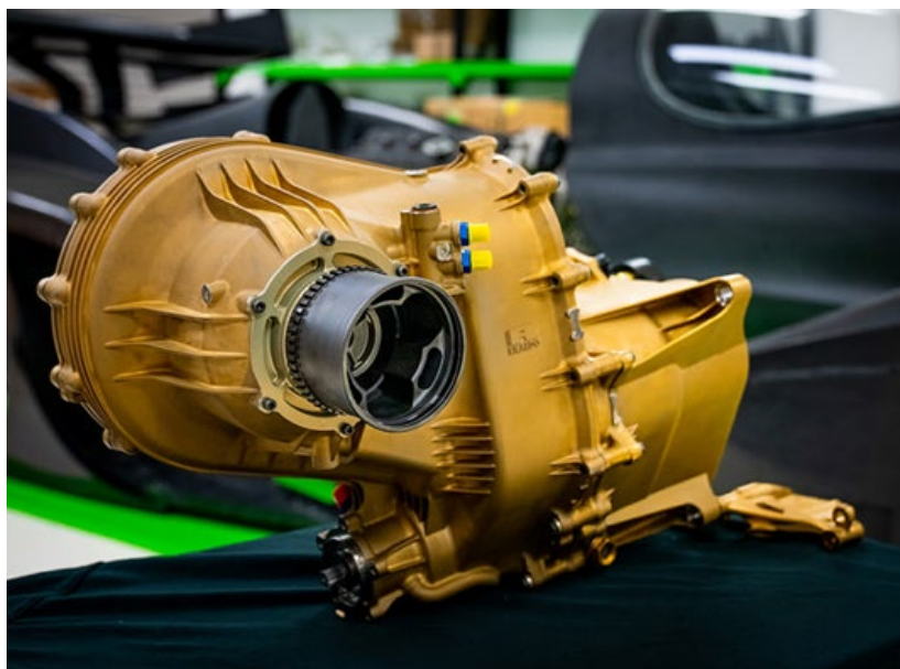
The 8 speed sequential gearbox weighs 68 kg and is additively manufactured from grade 23 titanium (Courtesy Rodin Cars)
