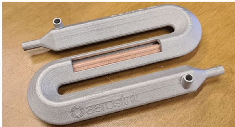
A multi-metal heat exchanger manufactured with Aerosint's multi-material deposition system (Courtesy Aerosint)
