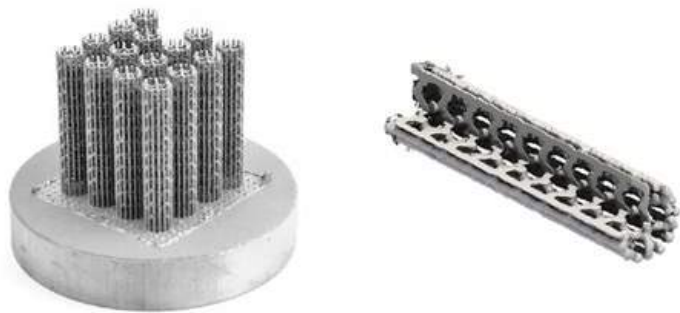
Fig. 7 Test bars built made from a Cu-70Al powder blend for catalyst structures by the University of Erlangen-Nuremberg, Germany, the first Freemelt ONE customer (Courtesy University of Erlangen-Nuremberg)
