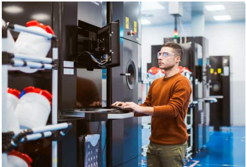
Fig. 1 GE Additive Arcam EBM is currently the dominant provider of PBF-EB technology, and accounts for the vast majority of all installed PBF-EB machines in the market (Courtesy GE Additive)
