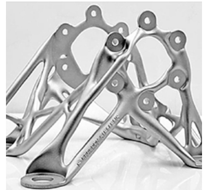
An aluminium gearbox mount from a Siemens sponsored Formula Racing car was the first collaboration. The part is designed by Siemens NX software and fabricated on a Farsoon FS301M (Courtesy Farsoon)
