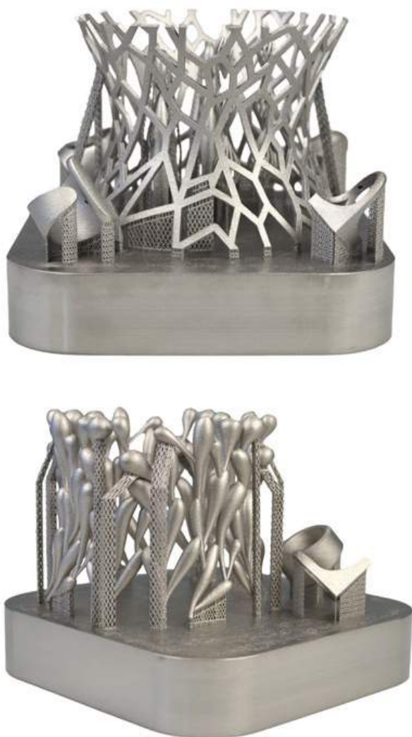
Fig. 3 PBF-LB build plates showing the support structures that are required during manufacture. Multiple items can be 'nested' on such build plates, but designers need to consider carefully the locations of removable support structures in order to minimise post-processing. Build by Progol3D® Internal Projects, Titanium (Courtesy Progold S.p.A.)
