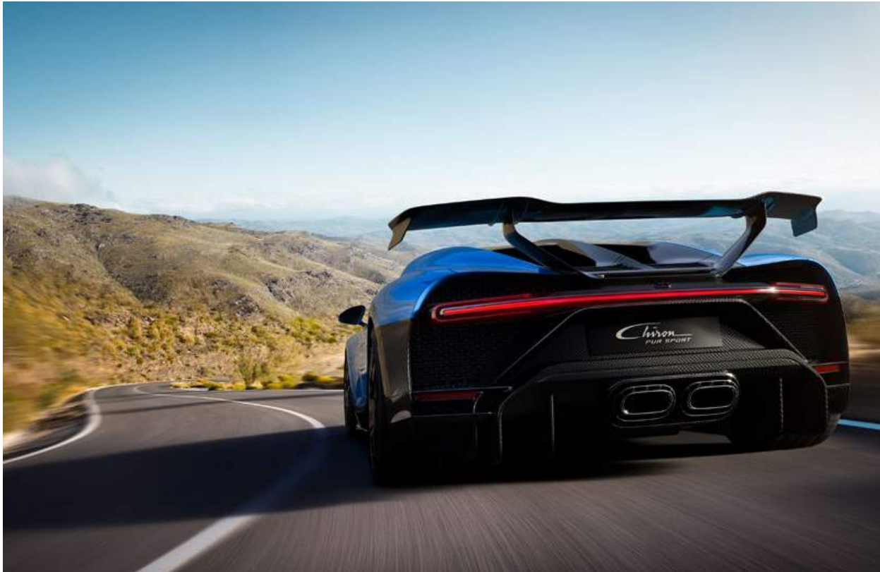
Fig. 5 Rear view of the Bugatti Chiron Pur Sport showing the additively manufactured titanium exhaust finisher (Courtesy Bugatti Automobiles S.A.S.)
