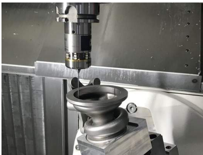
3T-am's part setup time was reduced from five hours to ten minutes (Courtesy MSP)
