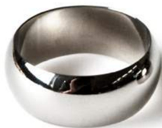
Fig. 15 An AM band produced using a gold and niobium powder blend. Weight is 12 g versus 16 g for regular palladium white gold. Premium white WGC colour, fineness 750%, manufactured by Progol3D® (Courtesy Progold S.p.A.)
