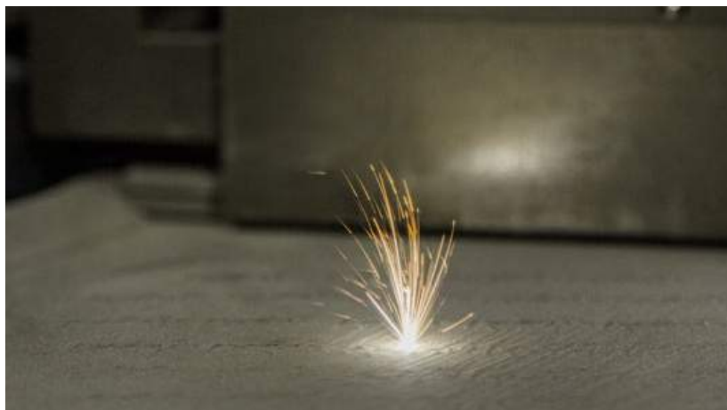
Fig. 2 Inside the build chamber of a Laser Beam Powder Bed Fusion (PBF-LB) machine at Progol3D® Internal Projects, Titanium (Courtesy Progold S.p.A.)
