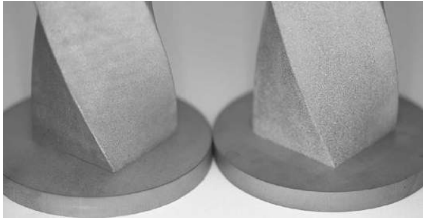
Fig. 6 Two geometries in 316L stainless steel, one built with 15–53 µm powder and 30 µm layers (left) and one built with 53–150 µm powder and 100 µm layers. Each build plate is 100 mm in diameter and the powder was supplied by Carpenter Additive. Both builds ran smoothly without smoke events or other issues. As can be expected, the fine powder and thinner layers give a notably better surface finish (Courtesy Freemelt AB)
