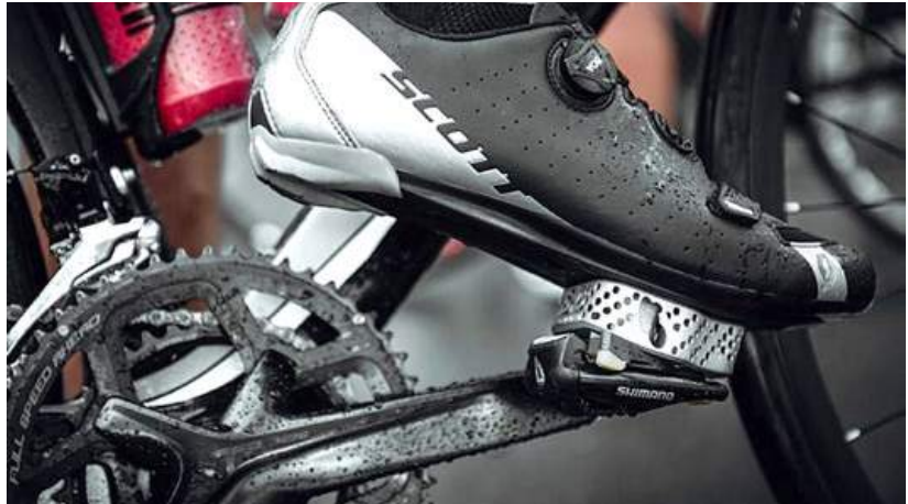
The titanium additively manufactured spacer and cleat in position on Creeggan's bike (Courtesy Zenith Tecnica)
