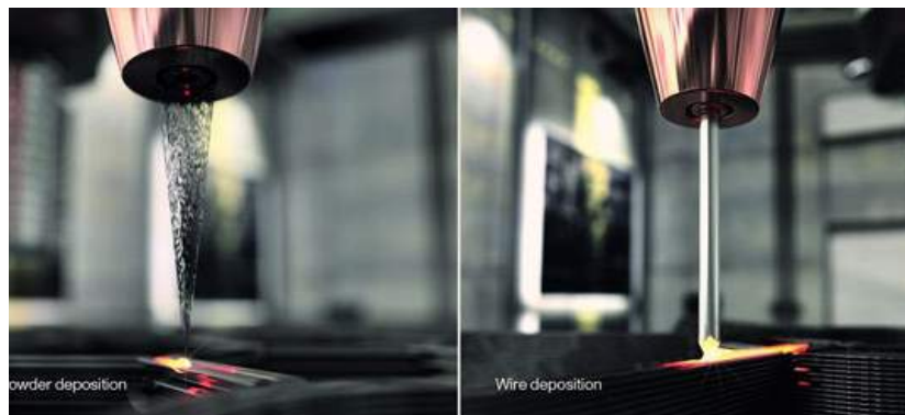
The Meltio M450 is capable of building fully-dense parts from powder (left) and wire (right) in the same machine, using a patented multi-laser deposition technology (Courtesy Meltio)
