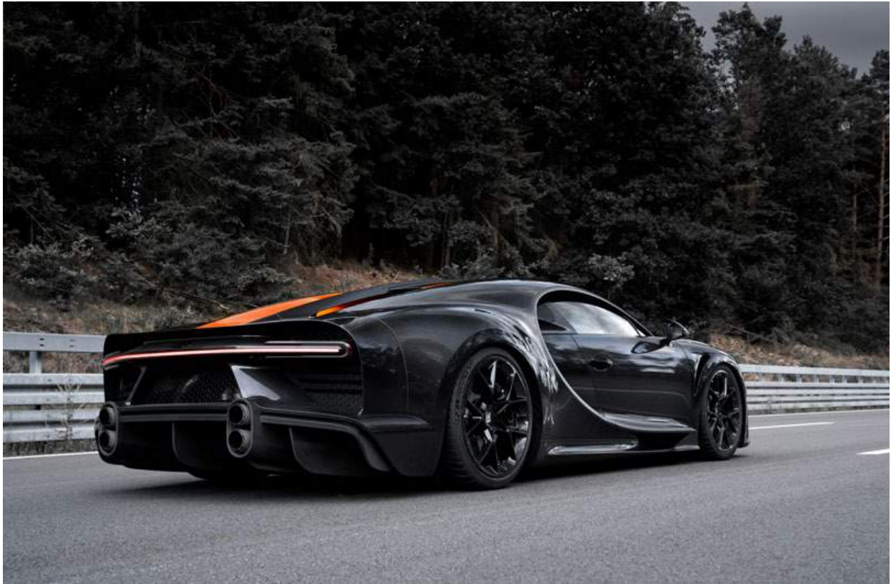
Fig. 8 This Bugatti Chiron Super Sport 300+ broke the 300 mph barrier with AM exhaust finishers produced by APWORKS (Courtesy Bugatti Automobiles S.A.S.)
