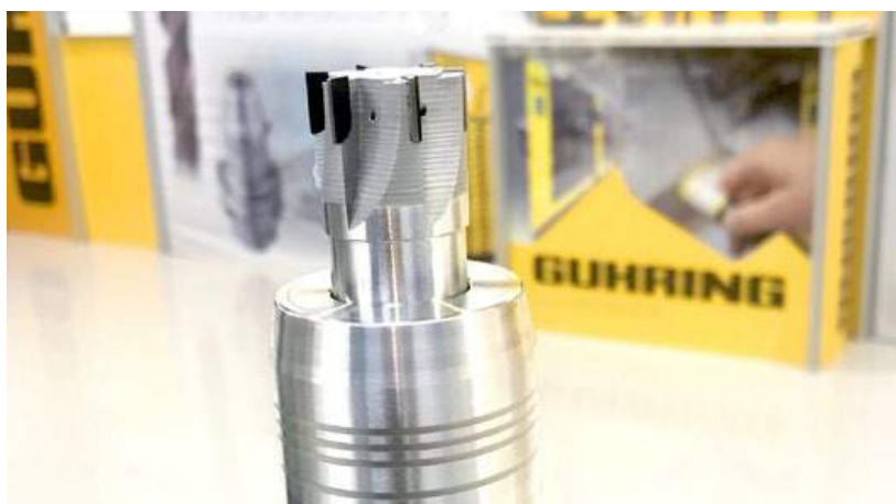
The additively manufactured H13 tool steel milling cutter was produced using a Markforged Metal X system (Courtesy Markforged)
