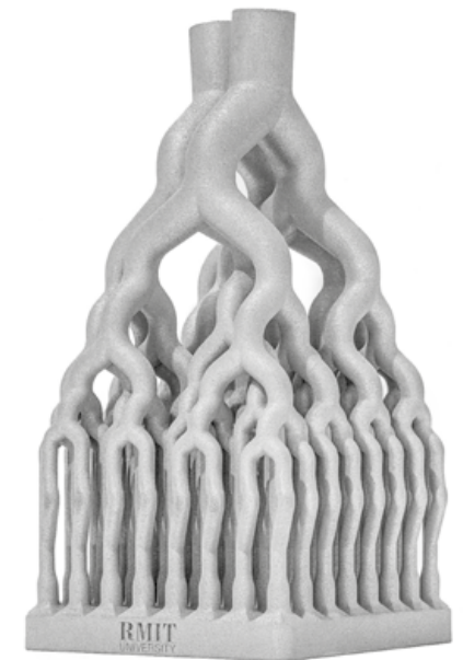
Additively manufactured Ti-6Al-4V dual fluid flow distributor and mixer comprising of 64 mixed outlets (Courtesy RMIT University)
