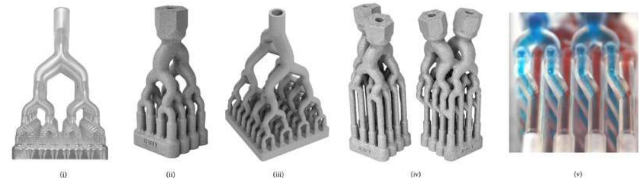
Flow distributor and mixer devices (i) Six-stage polymer flow distributor (64 outlets) (ii) Four-stage Inconel 625 flow distributor (16 outlets) (iii) Six-stage Inconel 625 flow distributor (64 outlets) (iv) Four-stage Inconel 625 dual fluid flow distributor and mixer (16 outlets) and (v) Four-stage dual fluid flow distributor and mixer in operation (Courtesy RMIT)
