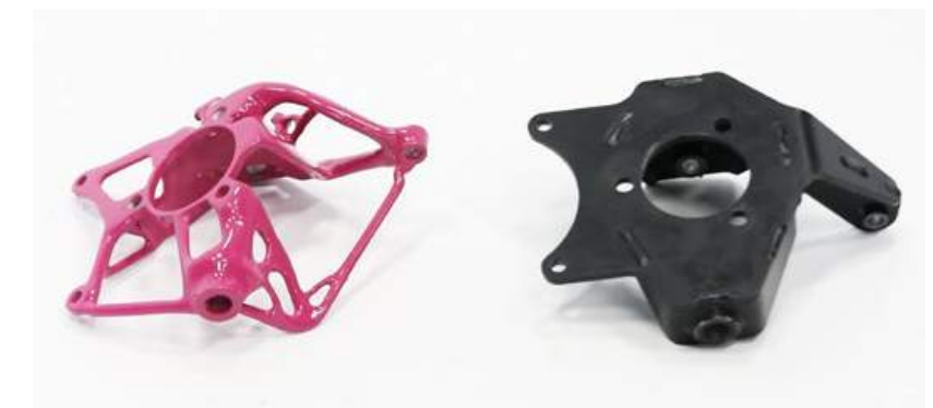
The metal additively manufactured steering knuckle (left) weighed 36% less than the conventionally produced part (right) (Courtesy XponentialWorks)
