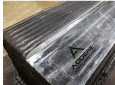
One of the 17-4 stainless steel blocks with machined section that ADDere produced using Laser Wire Additive Manufacturing (Courtesy ADDere)
