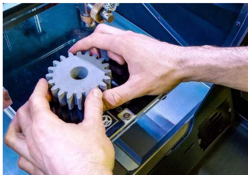
The Rapidia system builds parts using water-based metal paste technology (Courtesy Rapidia)
