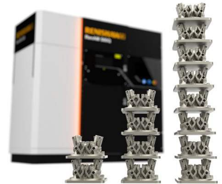
Fig. 3 There was a consensus that current build speeds are no longer a significant barrier to process adoption, with multi-laser machines offering dramatic increases in productivity. This image shows the difference in productivity within a fixed build time using 1, 2 and 4 lasers on a RenAM500Q machine (Courtesy Renishaw plc)
