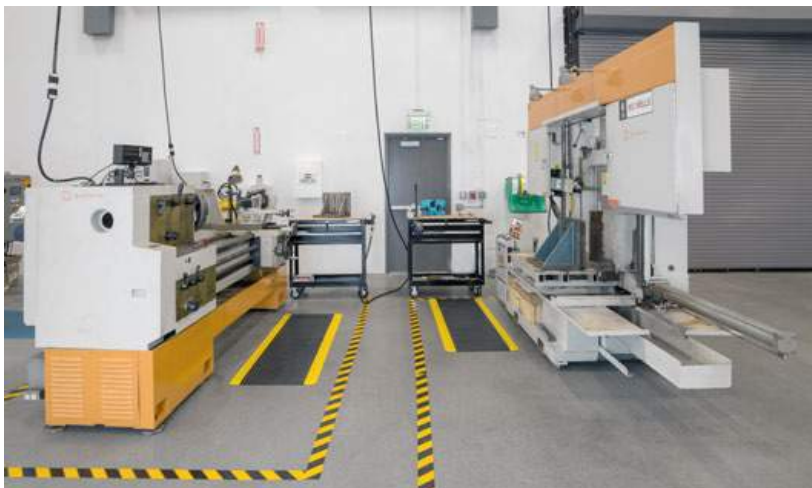
Fig. 6 A lathe and band saw for the post-processing of AM parts
