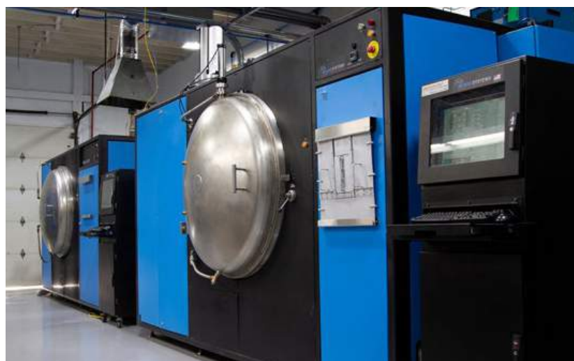
Fig. 1 Elnik Systems furnaces installed at DSH Technologies, the wholly owned subsidiary of Elnik Systems that offers process development, consulting and toll debinding and sintering services
