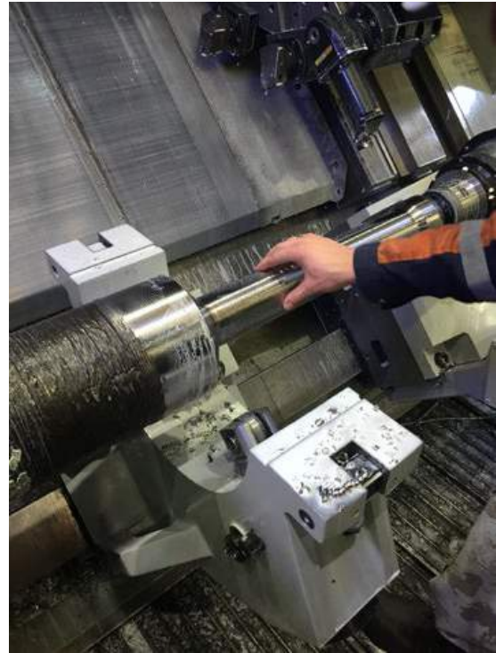
Fig. 6 Circulating head for Vallourec. Designed by Vallourec, shown as welded, during machining process using Böhler X90-IG
