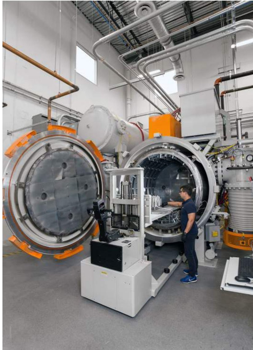
Fig. 9 An industrial scale GM vacuum furnace for the heat treatment of AM builds
