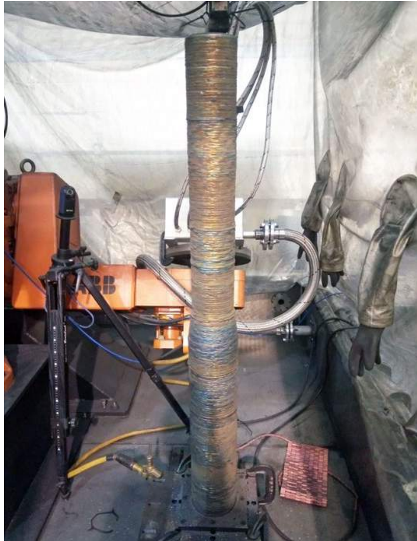
Fig. 7 A cross-over for BP in production at the AFRC Strathclyde University. Produced via WAAM in Inconel 718 in shielded environment based on a BP design
