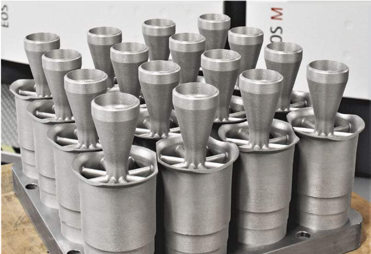
Fig. 4 Burners printed in an array of sixteen parts on a Laser Powder Bed Fusion machine (Courtesy of Siemens)
