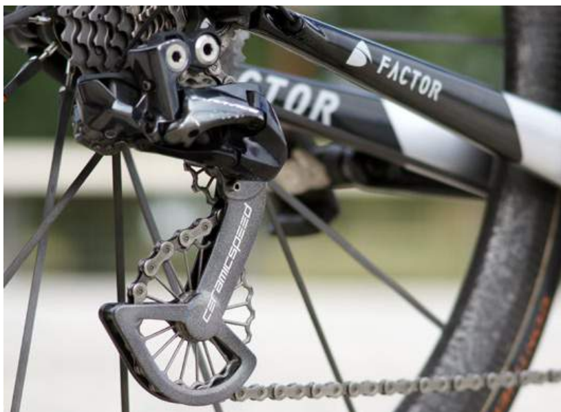
The additively manufactured titanium pulley wheel produced by CeramicSpeed and DTI (Courtesy SLM Solutions)
