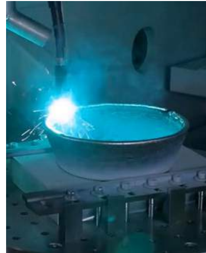
Gefertec's 3DMP process is a wire-based Additive Manufacturing system (Courtesy Gefertec)
