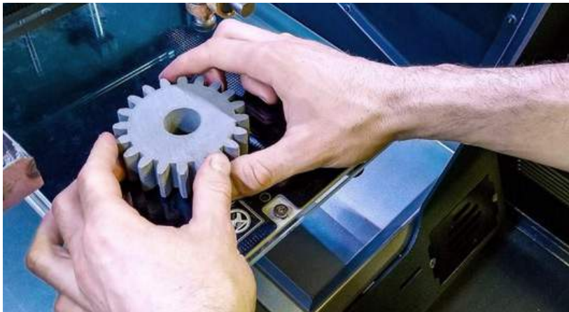
Rapidia uses water-based metal paste supplied in ready to use cartridges system (Courtesy Rapidia)
