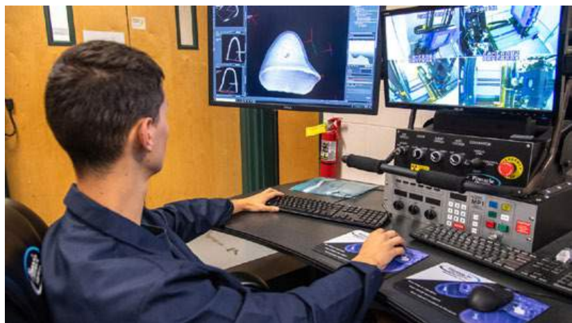
An Auburn University researcher examines a 3D rendering of scans produced by the new X-ray CT system (Courtesy Auburn University)
