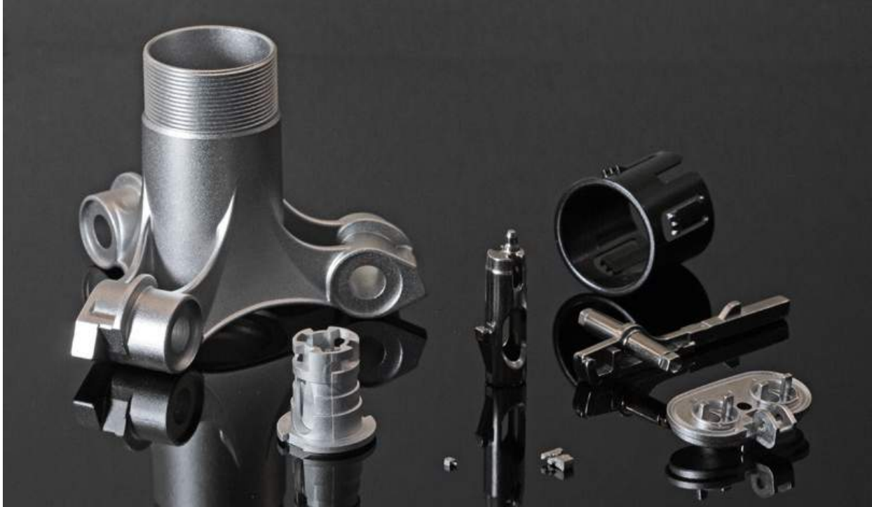
Fig. 6 A selection of MIM parts showing the range of shapes and sizes that can be manufactured by the technology, typically to net shape. The smallest part here is a 316L stainless steel locking device for a spectacle frame hinge, weighing 0.028 g and produced in volumes of more than 4 million parts a year. The largest part is a 316L tripod base which weighs 260 g and is 65 mm high
