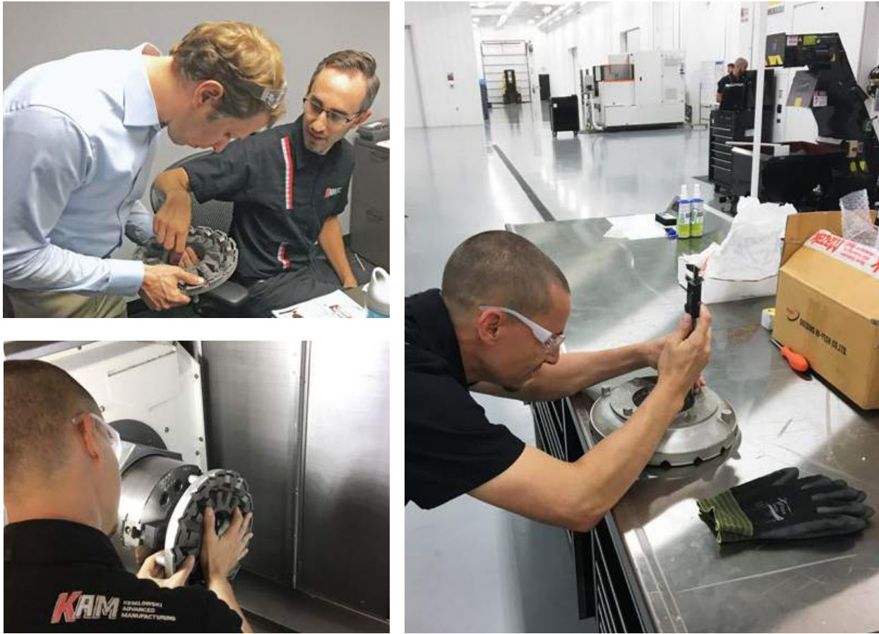
Fig. 8 Top left, Brad Keselowski, Founder & CEO of KAM, and Michael Mullen, KAM Engineering Manager, discuss the differences between two builds of the KW MicroPower diffuser before machining. Bottom left, qualifying the diffuser's datum surface on MAZAK i300 Integrex Mill/Turn machining centre. Right: CNC machinist Colby Burgin checks the diffuser dimensions for best fit of machining to built part, ensuring proper alignment of the part envelope with the machine work coordinate system
