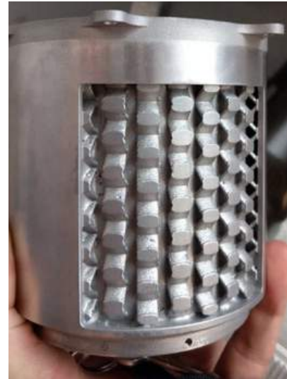
The inlet and outlet were separated from the main body for the build process in order to reduce the need for support structures (Courtesy JAMPT Corporation, TUfast)
