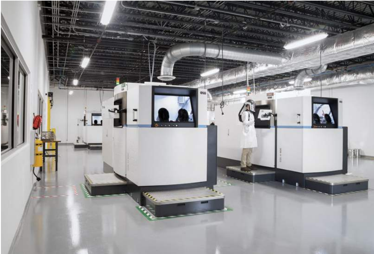
Fig. 3 EOS M400 systems installed at Sintavia for the production of components for the aerospace and defence sector
