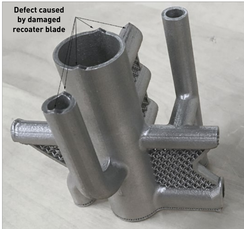
Fig. 2 A small chip in a recoater blade can cause multiple defects in the parts being produced
