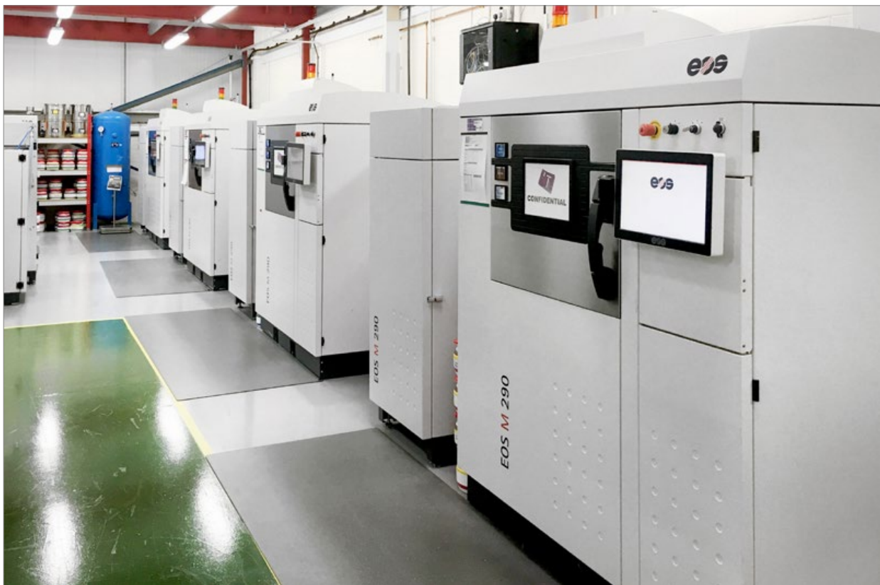
Fig. 2 Twelve EOS M290 machines form the bulk of 3T's metal Additive Manufacturing capacity
