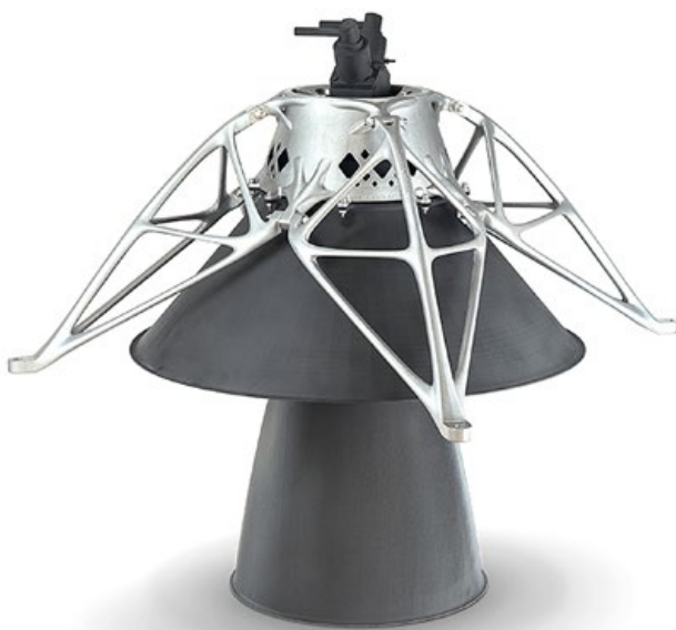
The additively manufactured aluminium bracket is used to hold the engine in the lunar lander (Courtesy RUAG Space)
