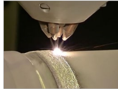
Optomec's LENS systems can be used for the building, repair and coating of parts (Courtesy Optomec)
