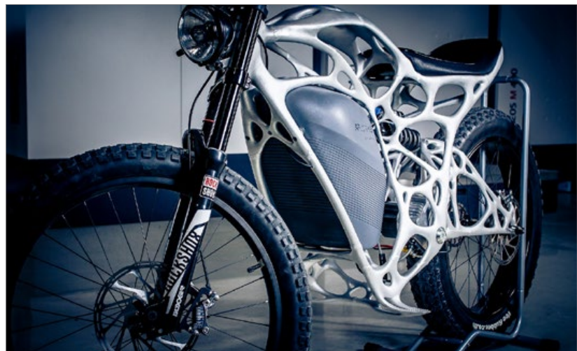
Fig. 1 This Light Rider electric motorcycle from APWORKS features an additively manufactured Scalmalloy frame
