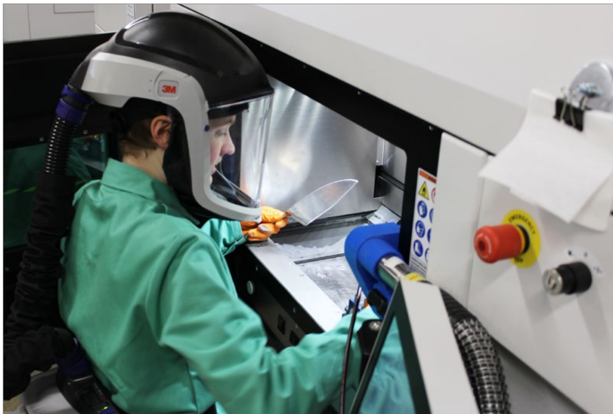
Fig. 3 Proper protection against exposure to metal powder dust is of fundamental importance during metal AM operation and maintenance
