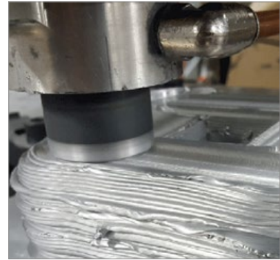
MELD uses a solid-state process which can use metal powders and rods as feedstock (Courtesy MELD Manufacturing)
