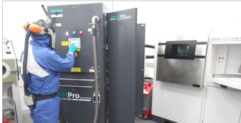
The AMPro Sieve Station incorporates a fully-automated one-button process (Courtesy Russell Finex)
