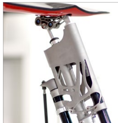
Additively manufactured spoiler bracket reduced weight by 5.4 kg (Courtesy VW Group)
