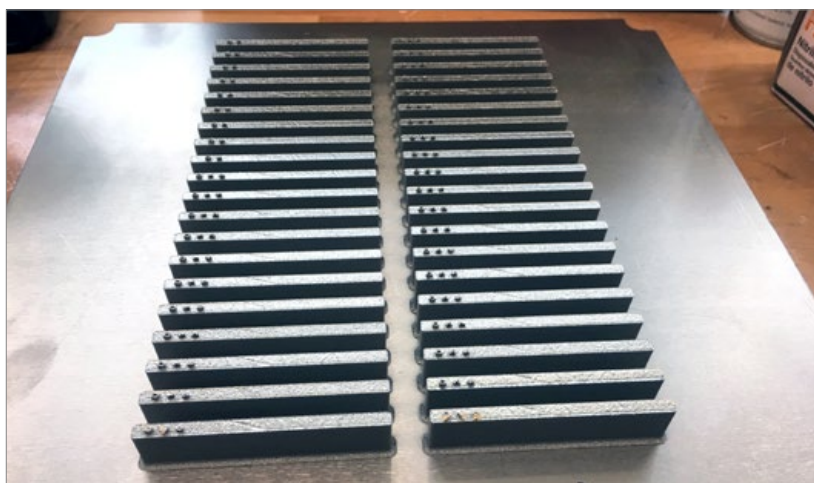
Fig. 1 Ti-6Al-4V (Ti64) specimens built on a Laser Powder Bed Fusion machine. The specimens were later tested and used as training data for Senvol's machine learning software
