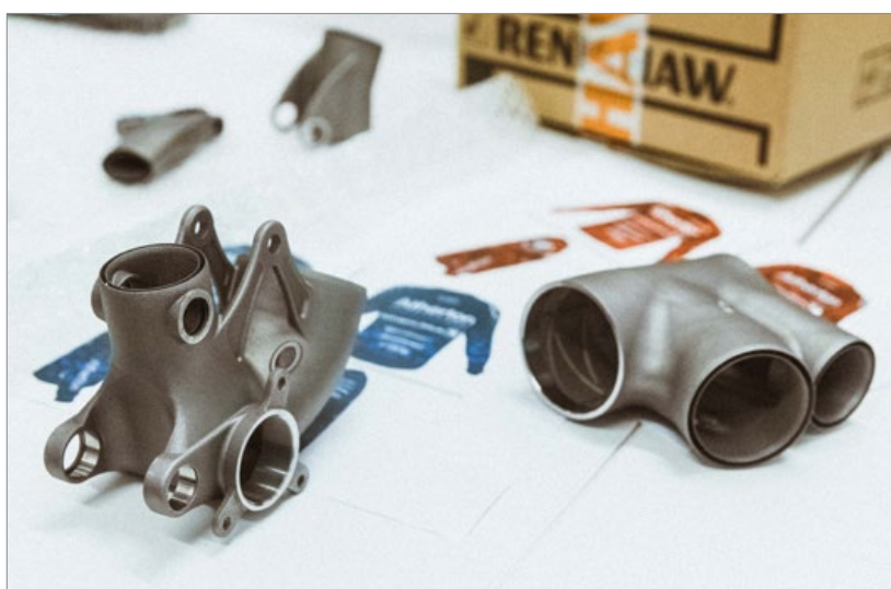
Titanium lugs, produced on a Renishaw 500Q, will join the carbon fibre tubing of the bike frame (Courtesy Renishaw)
