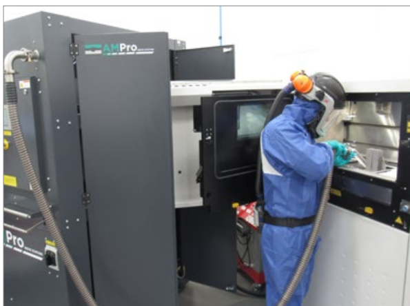
Progressive Technology use the AMPro to reclaim and requalify metal powder [Courtesy Russell Finex]
