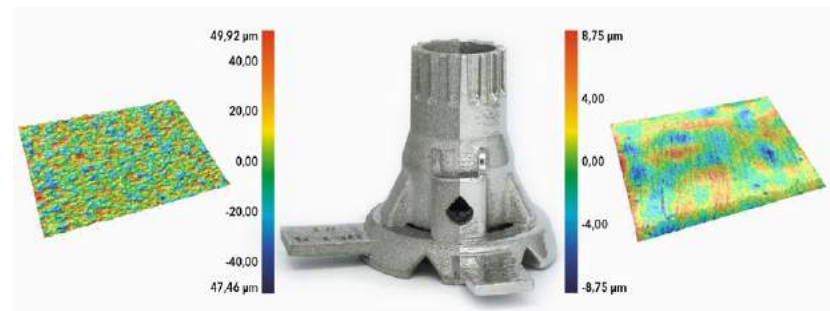
A comparison of roughness levels; original shown left and the polished sample on right (Courtesy Dlyte)
