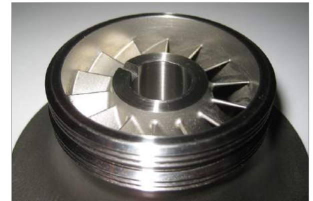
Following surface finishing using PostProcess's Hybrid DECI Duo solution, the impeller consistently passed aerodynamic tests (Courtesy PostProcess Technologies)
