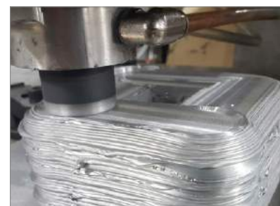
MELD is a solid-state process which can use a wide range of materials as feedstock, including metal powders and rods (Courtesy MELD Manufacturing)
