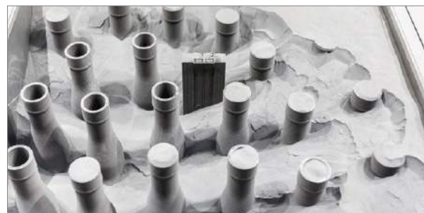
Metal additively manufactured latch shafts prior to depowdering at Airbus Helicopters (Courtesy Airbus)
