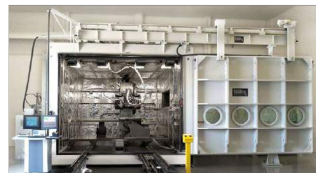
The custom EBAM system produced by Sciaky for FAMAero will be used to produce metal parts over 3.7 m in length (Courtesy Sciaky, Inc.)
