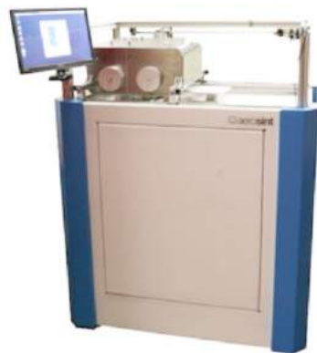
Aerosint's selective powder deposition system [Courtesy Aerosint]
