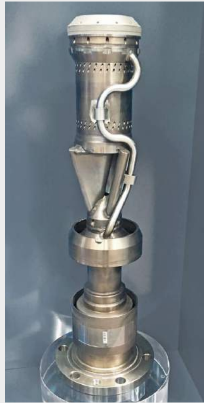
Fig. 7 A conventionally manufactured burner repaired using AM is shown on the left, with the repaired section visible at the top. Top right shows the original complete burner component, middle right shows the new AM design, and lower right shows a cutaway view highlighting the lattice structure
