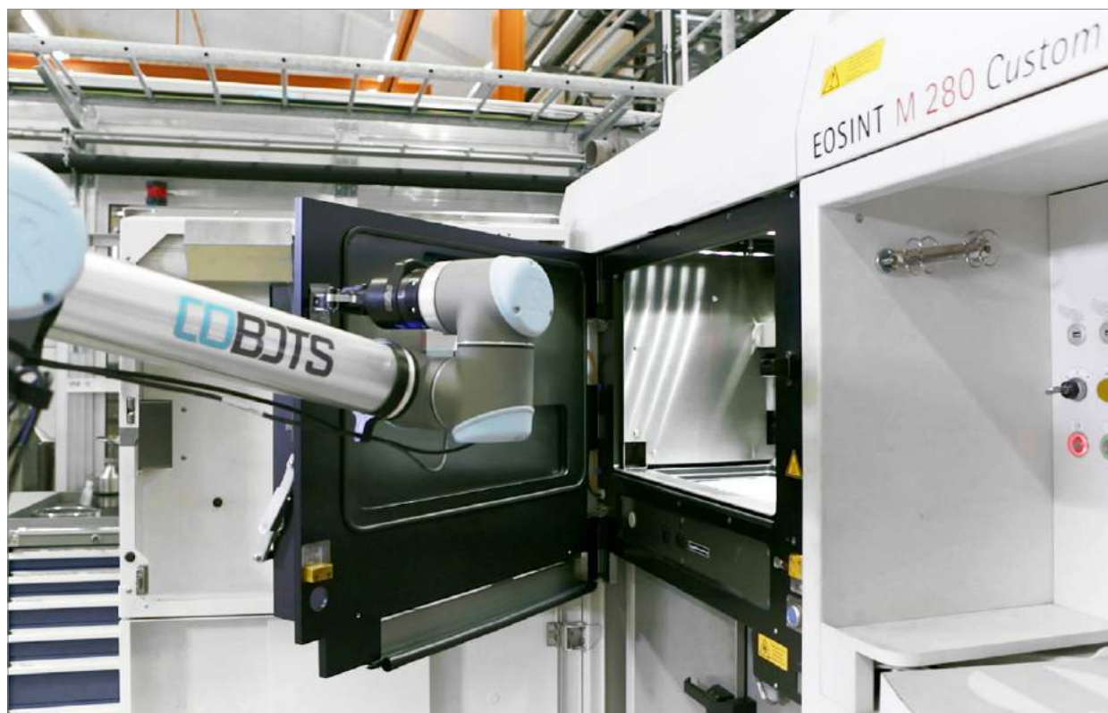
Fig. 12 Finspång has already built a robot arm capable of extracting powder from the current M280 machines where burner repairs are performed, relieving employees of this potentially dangerous task
