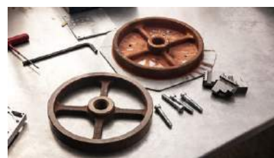
Components produced using SPEE3D's supersonic 3D deposition process (Courtesy SPEE3D)
