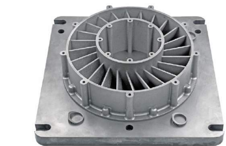
Fig. 6 Ti6Al4V fuel cell cartridge guide manufactured on a FS271M laser PBF system (Courtesy Farsoon)
