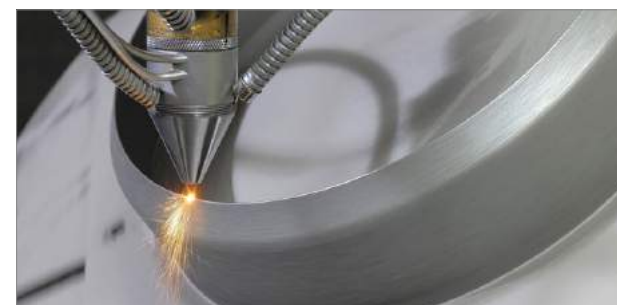
Directed Energy Deposition metal Additive Manufacturing in action (Courtesy TWI Ltd)
