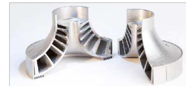
A shrouded impeller produced on the Sapphire system. The only support required on this part is the radial extrusion that supports the outer lip (Courtesy Velo3D)
