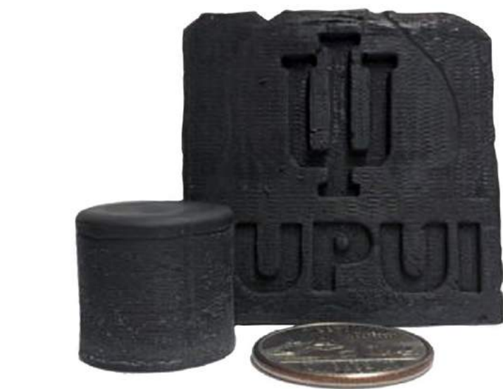
Fig. 9 Additively manufactured 17-4PH stainless steel samples [3]. The logo of IUPUI is shown on the plate sample
