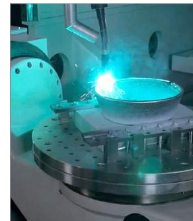
Gefertec's arc605 is a five axis wire based AM system (Courtesy Gefertec)
