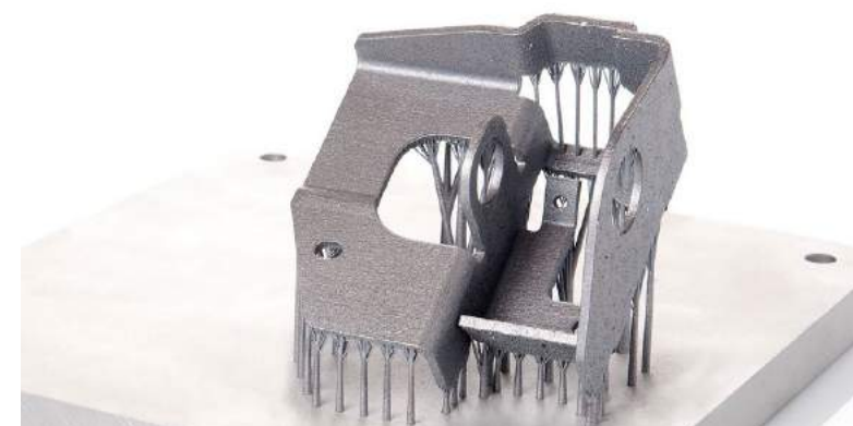
A part demonstrating support structures automatically generated by Materialise's Magics software (Courtesy Materialise)
