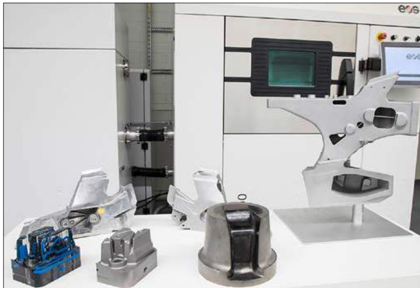
Fig. 7 Tooling and components produced by Audi using AM (Courtesy Audi AG)
