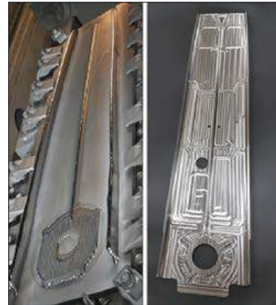
This photo highlights two different stages of an Airbus rear upper spar that was 3D printed in titanium with Sciaky's EBAM process. The image on the left shows the part in an early preform stage. The image on the right shows the finished part
