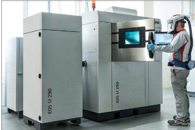
Fig. 6 Metal AM production at Audi using an EOS M 290 (Courtesy Audi AG)
