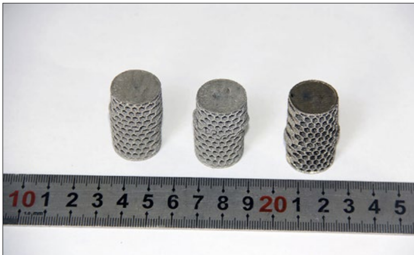
Fig. 3 Samples for compression testing
