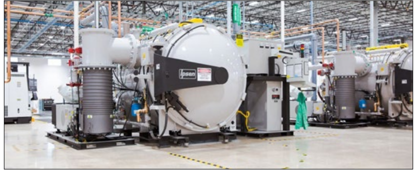
After printing the metal parts are placed inside curing ovens filled with argon or nitrogen (Image: GE Reports/Chris New)
