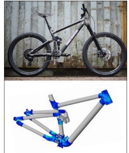
Altair performed design optimisation with solidThinking Inspire and design verification with OptiStruct
