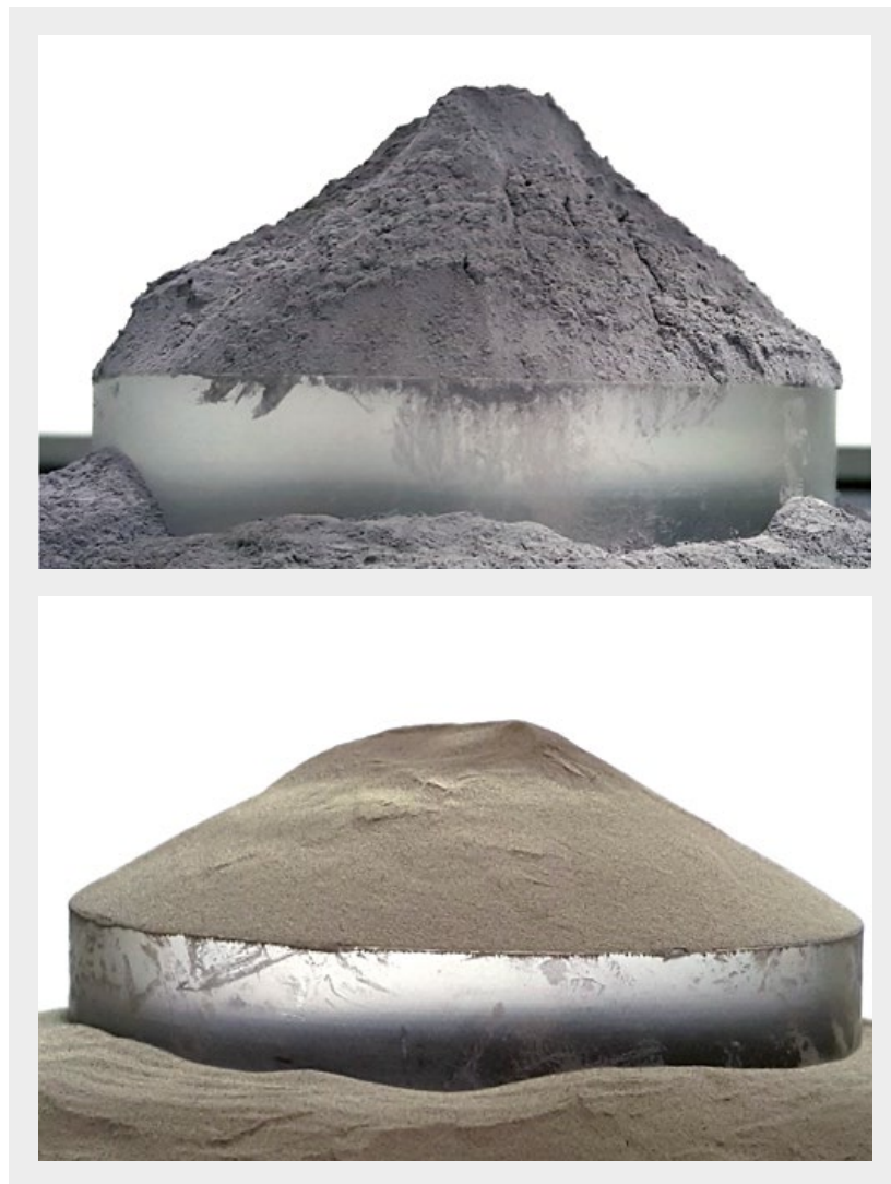
Fig. 3 Two powders showing a different flow behaviour
