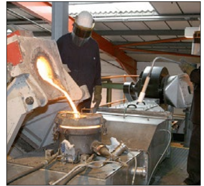
Gas atomising at Atomising Systems Limited
