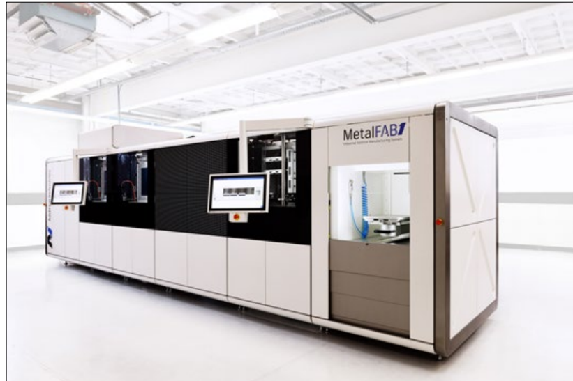
Fig. 4 Additive Industries' MetalFAB1 system is due to be installed at GKN Sinter Metals before the end of 2016 and promises to open the door to the serial production of AM components for GKN's core markets (Courtesy Additive Industries)
