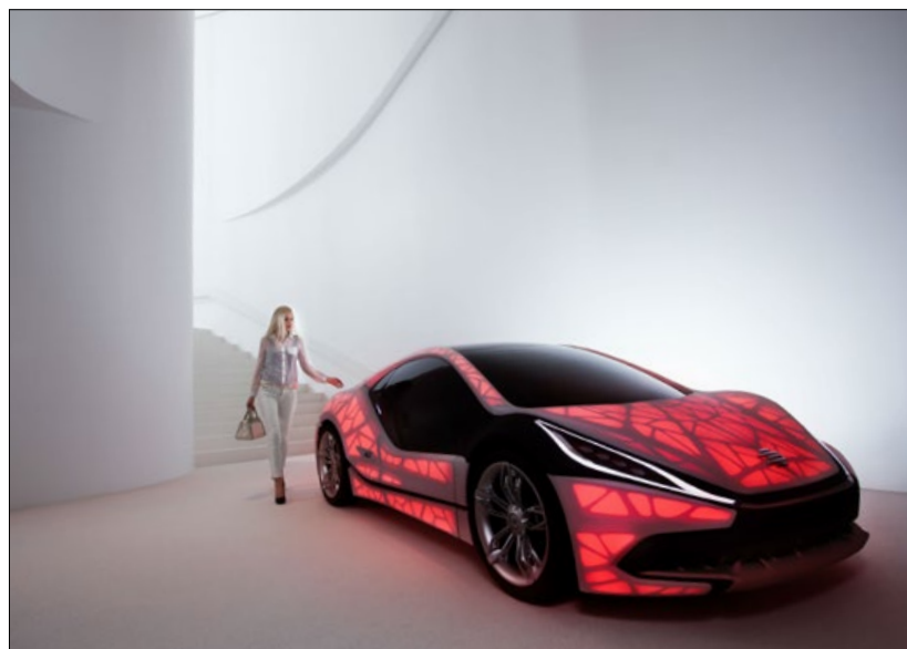
Fig. 1 The "EDAG Light Cocoon" concept car features a bionically optimised and additively manufactured vehicle structure
