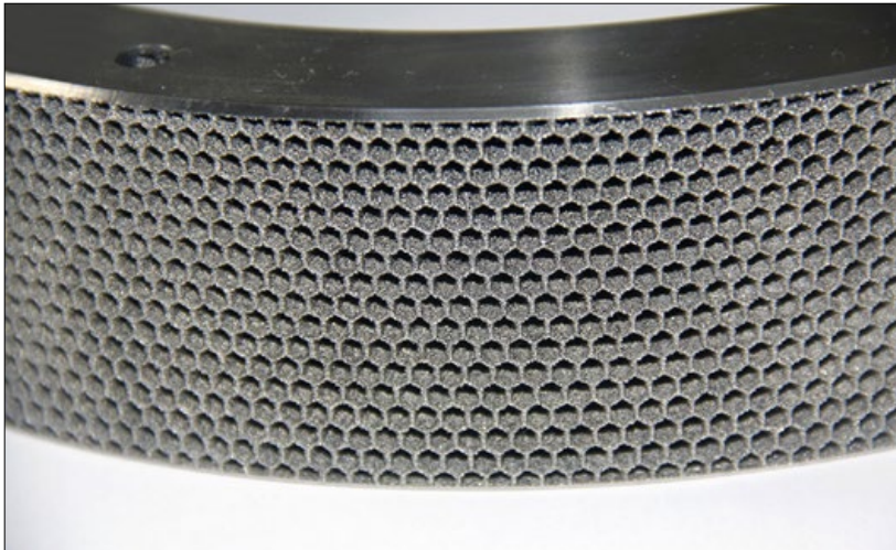
Fig. 2 Hexagonal structure on the outer cylindrical surface of the Ti-6Al-4V honeycomb oil-gas separation rotor
