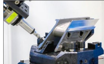
A robot automatically polishes a nozzle component (Courtesy GE Oil & Gas)
