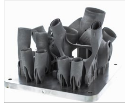
The R160 Build Plate with printed titanium lugs from the Renishaw AM 500M
