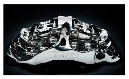
Bugatti and Laser Zentrum Nord report that they have been able to produce a complex structure which is significantly stiffer and stronger than would be possible with any conventional process (Courtesy Bugatti)
