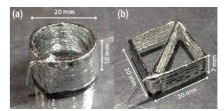
Demonstration structures produced using the modified gallium alloy (Courtesy OSU)
