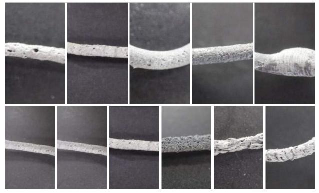
Fig. 16 Parameter testing with filament extruder setup for filament F1 and a nozzle of 0.8 mm. Top image:  $T = 250 \,^{\circ}$ C, Extrusion Speeds from left to right: 7 mm/s [0.88 mm³/s], 14 mm/s [1,76 mm³/s], 42 mm/s [5.3 mm³/s], 70 mm/s [8.8 mm³/s], 98 mm/s [12,37 mm³/s]. Bottom image: 14 mm/s extrusion speed, temperatures extruded at 14 mm/s from left to right: 225°C, 235°C, 250°C, 270°C, 280°C, 290°C [3]
