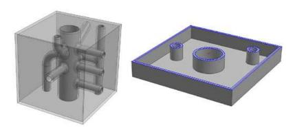
Fig. 2 If the bulk of the material is removed from the part by 'shelling' it to a specified wall thickness, the amount of scanning is greatly reduced, resulting in a faster print time
