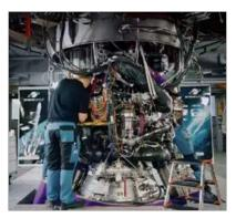
The Vulcain 2.1 engine incorporates a metal AM gas generator and is designed to power the main stage of the Ariane 6 launcher (Courtesy ArianeGroup)
