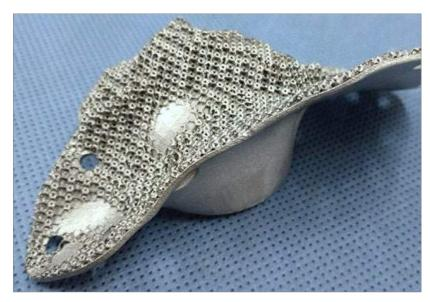
Imeco's first AM hip replacement was developed for a patient with a special medical condition (Courtesy Link3D)
