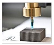
Fig. 8 3DFD (Robocasting) technology [2]
