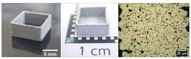
Fig. 17 Images of a printed box with a side length of 1 cm and a wall thickness of about 1.5 mm in green state (left), and thermally debound and sintered (middle, right). The cross section was taken perpendicular to the wall and feedstock F2 was used [3]
