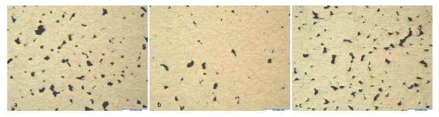
Fig. 12 Photomicrographs of Segment 11 (a) Part 2, 5.3% Porosity, (b) Part 5, 1.58% Porosity, and (c) Part 8, 4.77% Porosity.
