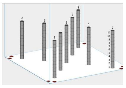
Fig. 1 CAD Image of the build configuration. The PCS cylinder is marked as specimen 2. Individual parametric build segments are numbered 1 to 11 starting directly against the build plate
