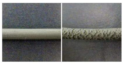
Fig. 15 Extruded filaments F4 (left) and F3 (right) with a diameter of 1.75 mm [3]
