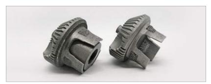
Fig. 5 The accuracy of a Digital Metal part (right) compared to an SLM part (left) (Courtesy CETIM)
