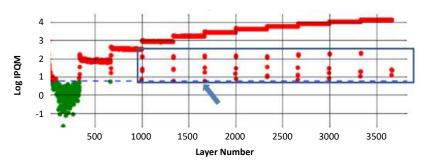
Fig. 6 Multivariate trend plot of IPQM parts graph from photodetector data collected from the entire build layer by layer
