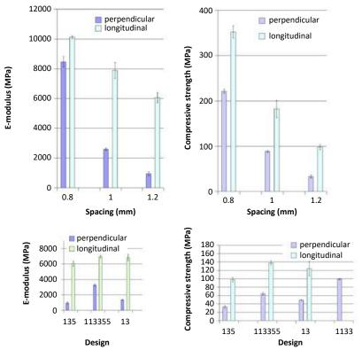
Fig. 13 Mechanical properties obtained by static compression testing of robocast samples with (top) 1-3-5 design and (bottom) 1.2 mm spacing between the fibres [2]
