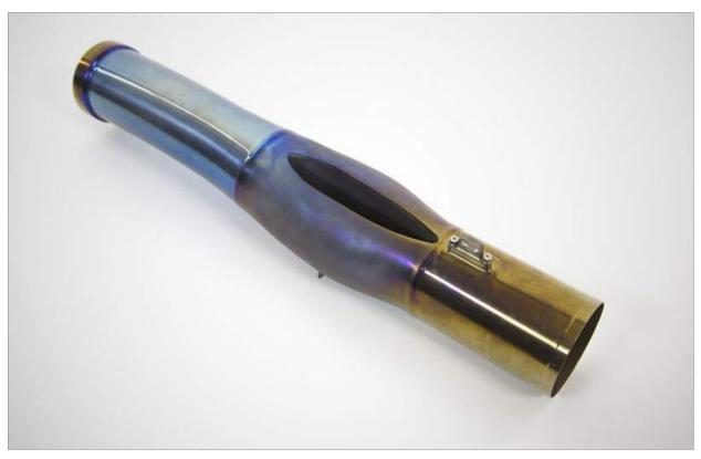
Fig. 10 Titanium race car tailpipe with the central section manufactured by metal Additive Manufacturing
