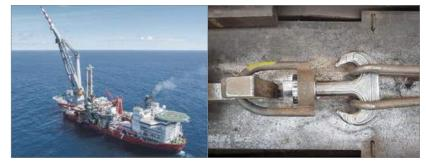
A typical offshore crane aboard a subsea vessel (left), additively manufactured crane hook under load test (right) (Courtesy Huisman Equipment)
