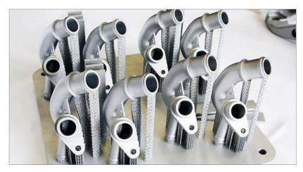
VW is already using on demand AM to make rarely needed water connectors for the Audi W12 engine (Courtesy VW Group)
