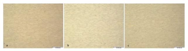
Fig. 10 Photomicrographs of segment 1 (a) part 2, 0.09% porosity, (b) part 5, 0.02% porosity, and (c) part 8, 0.07% porosity
