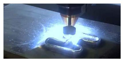
3D-Hybrid's Wire-Arc tool offers build speeds of more than 35 in<sup>3</sup>/min and can be used with a number of materials including aluminium alloys, stainless steel alloys and nickel-based super alloys (Courtesy 3D-Hybrid)
