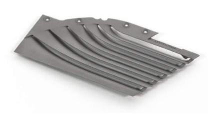
Fig. 7 Rear wing endplate louvre manufactured at 60% for the F1 wind tunnel model, material AlSi10Mg
