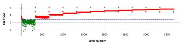
Fig. 7 Multivariate trend plot of the PCS specimen, part 2 generated using in-process photodetector data collected from a build and rolled up
