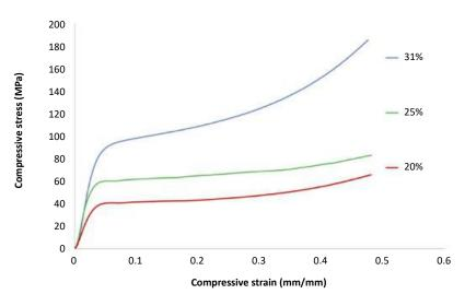
Fig. 12 Compression curves of gel cast Ti6Al4V foams. The relative densities of the foams are indicated [2]
