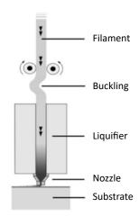
Fig. 14 Schematic printing process with soft filament that causes buckling between liquifier and driving wheels [3]
