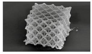
The final metal AM nanostructure was reported to be smaller than a speck of dust (Courtesy Caltech)
