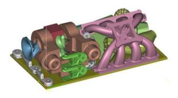
Fig. 3 Volume-based placement of multiple parts resulting in 18% occupancy
