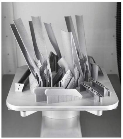
Fig. 6 A build plate with parts for the 60% F1 wind tunnel model and for the 1:1 F1 race car made from AlSi10Mg
