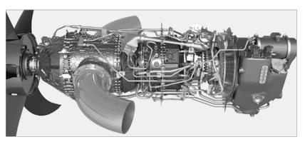
According to GE, more than a third of the ATP is metal additively manufactured from advanced alloys (Courtesy GE Reports)
