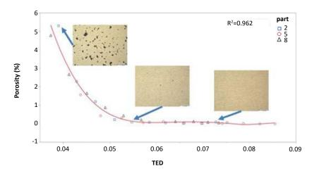
Fig. 13 Graph of porosity as a function of TED for all build segments tested for parts 2, 5 and 8
