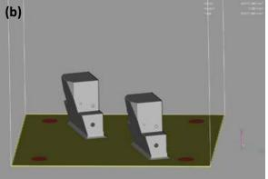
Fig. 7 (a) shows the finished printed parts with the island scan strategy shown as a checkered pattern. Part orientation in Magics build scene on the M2 platform is shown in (b). The red circles on the platform indicate build plate screw hole locations
