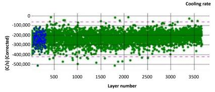
Fig. 2 Melt pool level trend plots for dependent in-process data mined from the pyrometer. The pyrometer was focused on the process control specimen
