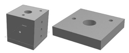
Fig. 1 A hydraulic manifold, left, with an example layer, right
