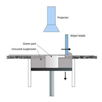
Fig. 2 Sketch of the prototype machine setup [1]
