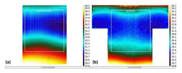
Fig. 8 Side-by-side comparison of the wedge thermal images acquired with the FLIR SC7650. (a) shows the conventional design, while (b) shows the AM design. The white outline on both wedges displays the region of interest. Thermal imaging data indicates that the AM wedge has lower average temperatures compared with the conventional wedge
