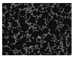
Fig. 10 Gel cast porous titanium alloy structures [2]
