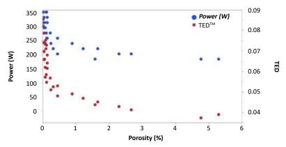
Fig. 14 Graph of porosity as a function of laser power (W) and the TED in-process quality metric
