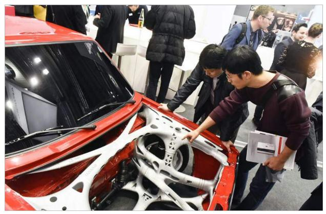
Fig. 7 The front-end structure of a VW Caddy redesigned using AM was shown on the APWorks booth. This was a project that also included Altair, csi entwicklungstechnik, EOS, GERG and Heraeus (Courtesy Mesago/Thomas Klerx)
