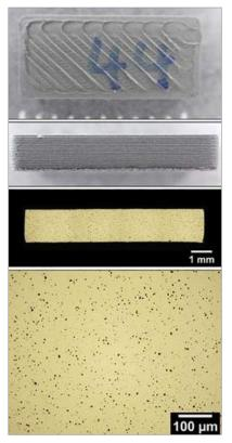
Fig. 18 Cross section of a cuboid part showing no layering effect [3]
