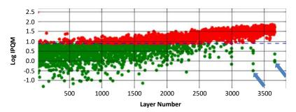
Fig. 4 Multivariate trend plot of melt pool level IPQM pyrometer data collected from the process control specimen
