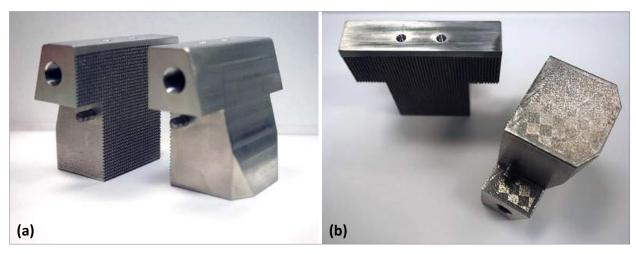
Fig. 9 (a) shows the AM wedges paired together, while in (b) the checkered pattern caused by the island scan strategy is visible on the far right wedge
