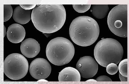
Our spherical Ti-6Al-4V titanium alloy powder's properties make it the material of choice for Additive Manufacturing
