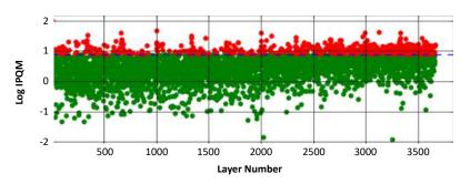
Fig. 5 Multivariate trend plot of layer level IPQM pyrometer data collected from the process control specimen.
