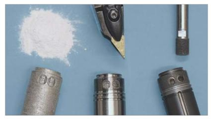
A component before, during and after machining (Courtesy GB Precision)
