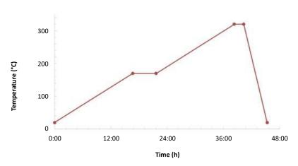
Fig. 4 Temperature program for thermal debinding and corresponding thermomechanical analysis (TMA) measurement [1]
