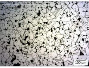
Fig. 6 Polished and etched micrograph of a sample sintered at 1355°C for 2 h [1]
