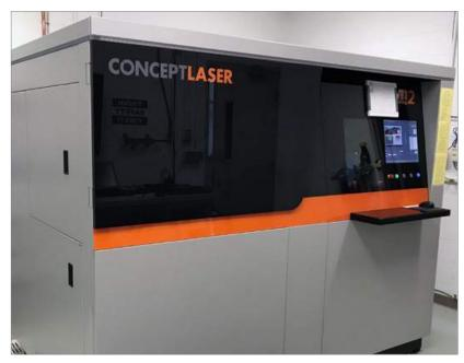
Fig. 6 AFIT's M2 Cusing metal Additive Manufacturing system
