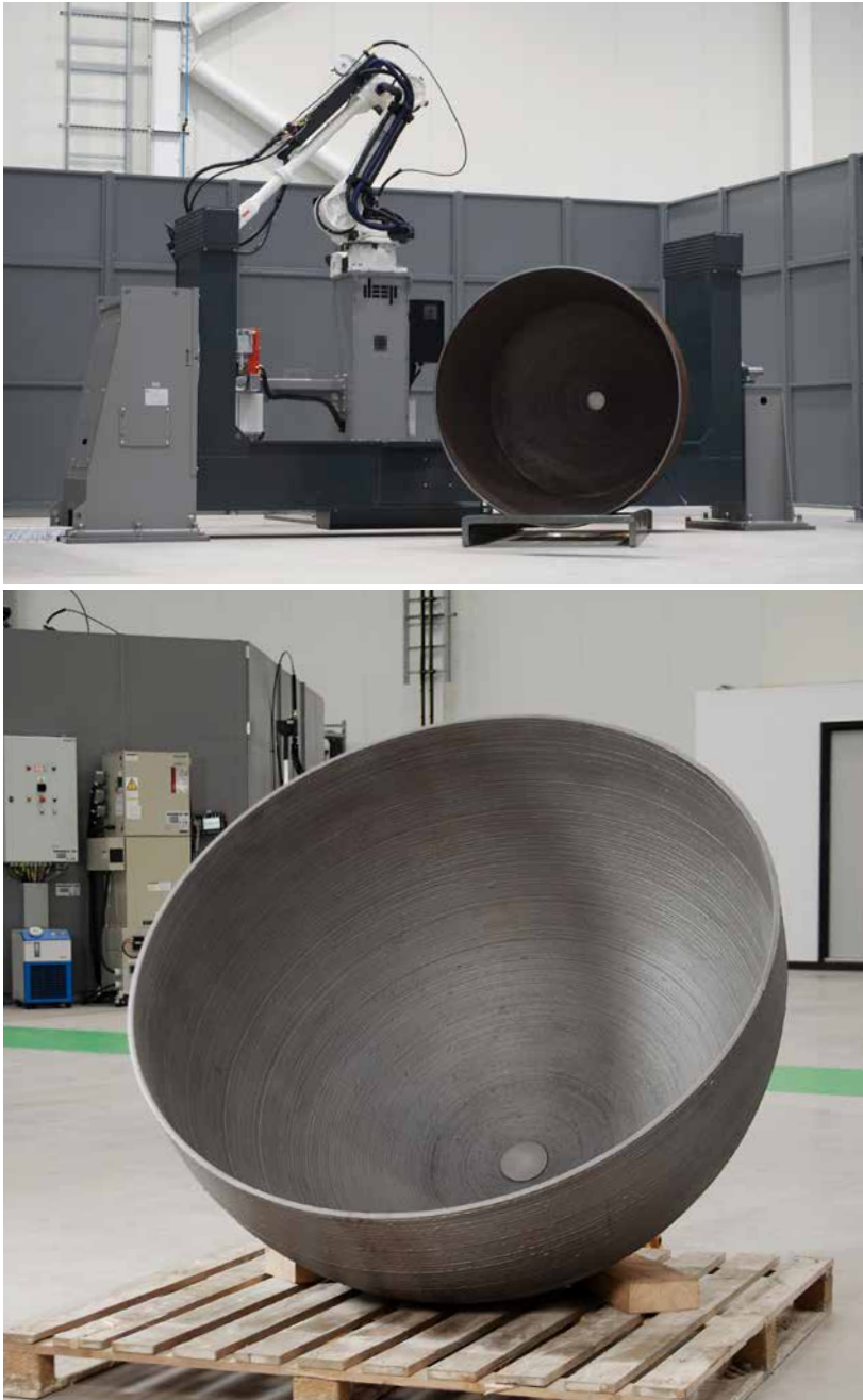
Fig. 10 A tilting and rotating two-axis manipulator (top) used for the manufacture of pressure-vessel end sections (above) and other complex geometries, allowing the workpiece to be positioned precisely during large-format wire-arc DED deposition (Courtesy DEEP Manufacturing)
