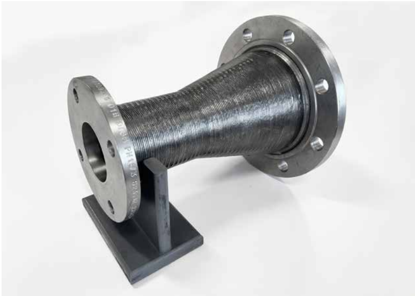
Fig. 12 A wire-arc DED valve component manufactured by DEEP Manufacturing, demonstrating the company's capability in safety-critical applications (Courtesy DEEP Manufacturing)
