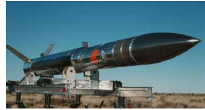
The ARMD sits staged for flight in late January. The missile was positioned on a specialised air log cart, used to transport and load the vehicle onto the Transportable Target Launcher (Courtesy Ryan Harty/US Army)
