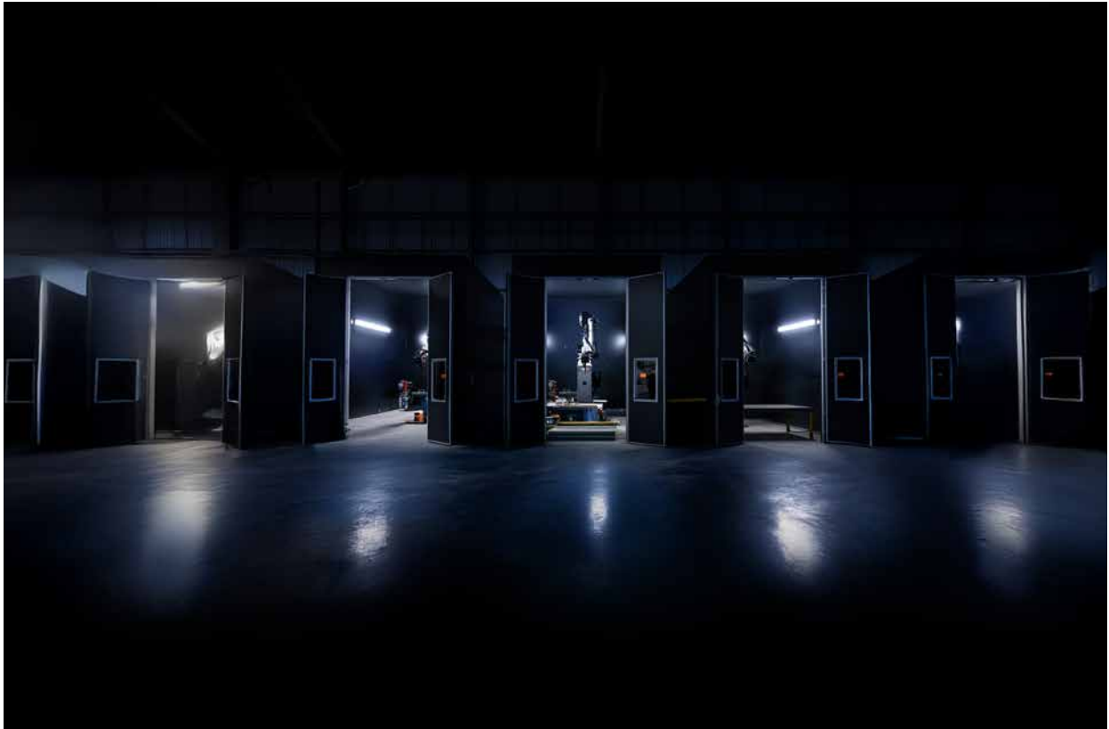
Fig. 5 Individual enclosed production cells at DEEP Manufacturing's Avonmouth facility, configured for controlled wire-arc DED operations on large-format metal components (Courtesy DEEP Manufacturing)
