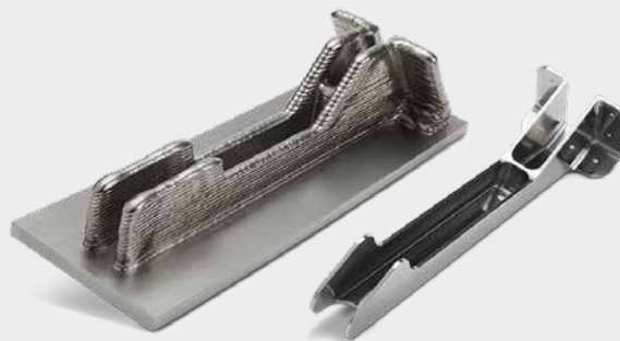
Fig. 3 Norsk Titanium's wire-fed, plasma arc Directed Energy Deposition Ti-6Al-4V, manufactured to SAE AMS7004 and AMS7005, is set to become the first AM alloy included in MMPDS Volume II. The milestone highlights the power of consensus standards to turn AM process maturity into recognised aerospace material allowables, supporting greater confidence in the use of metal AM for aircraft structures (Courtesy Norsk Titanium)
