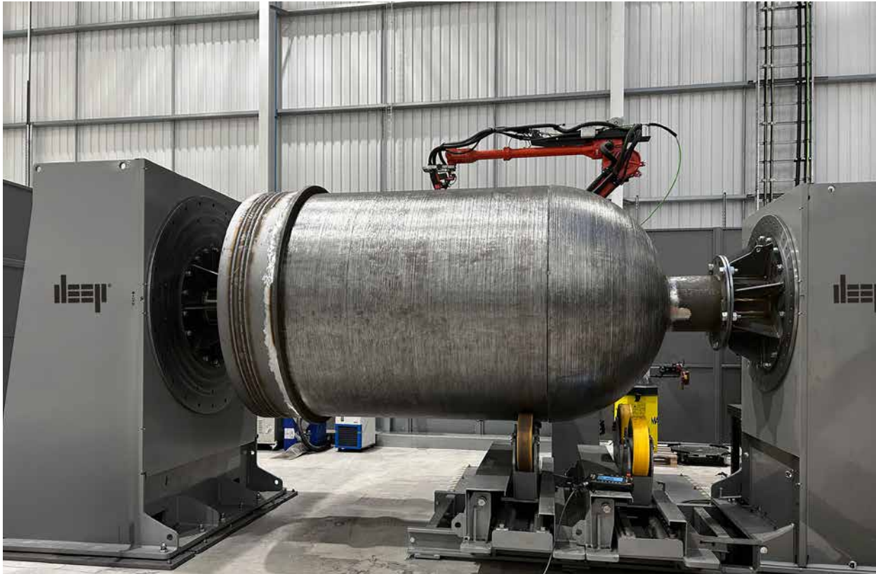
Fig. 11 Roller welding system used for fabrication, joining large pressure-vessel sections to support the assembly of full-scale structures manufactured using wire-arc DED (Courtesy DEEP Manufacturing)
