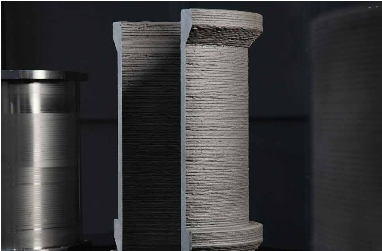
Fig. 14 Comparison of as-built and CNC-machined wire-arc DED test sections, illustrating the surface transformation achieved during post-processing and the role of machining (Courtesy DEEP Manufacturing)
