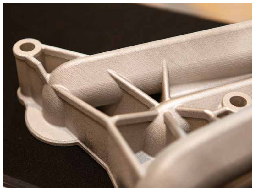
Fig. 8 Additively manufactured 316L stainless steel standpipe produced for Kawasaki Heavy Industries, reducing lead time from up to 135 days to fifteen days (Courtesy Pelagus)
