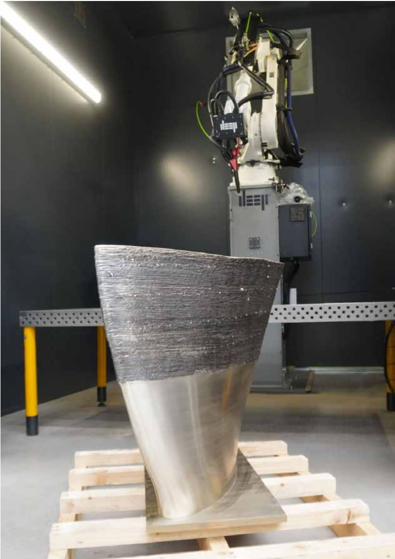
Fig. 8 A nickel aluminium bronze propeller blade produced using wire-arc DED, demonstrating DEEP Manufacturing's work with corrosion-resistant alloys for marine and subsea applications (Courtesy DEEP Manufacturing)
