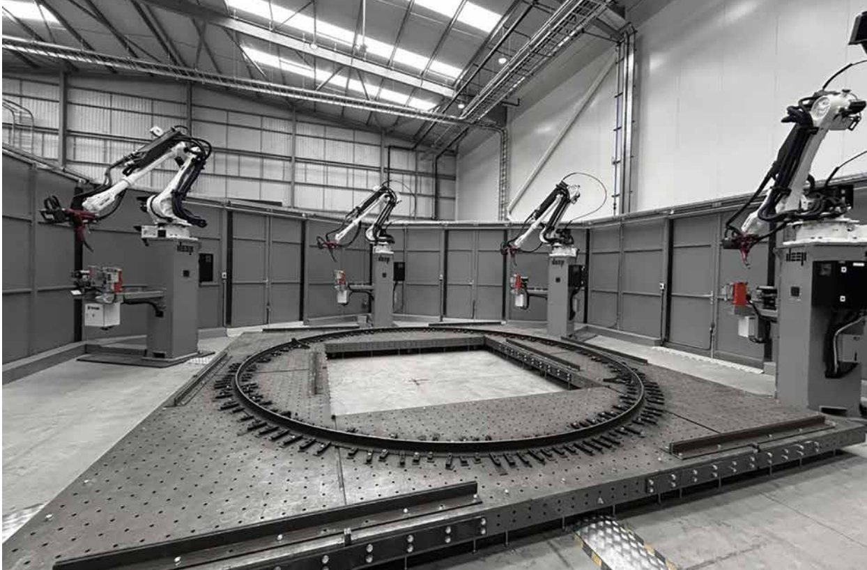
Fig. 6 DEEP Manufacturing's multi-robot system, currently configured with six coordinated robotic arms designed to increase build rate and working volume for large-scale wire-arc DED structures (Courtesy DEEP Manufacturing)
