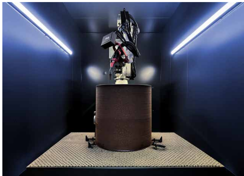
Fig. 1 A robotic wire-arc DED system at DEEP Manufacturing's Avonmouth facility, where the company is scaling large-format metal Additive Manufacturing for subsea and industrial applications (Courtesy DEEP Manufacturing)
