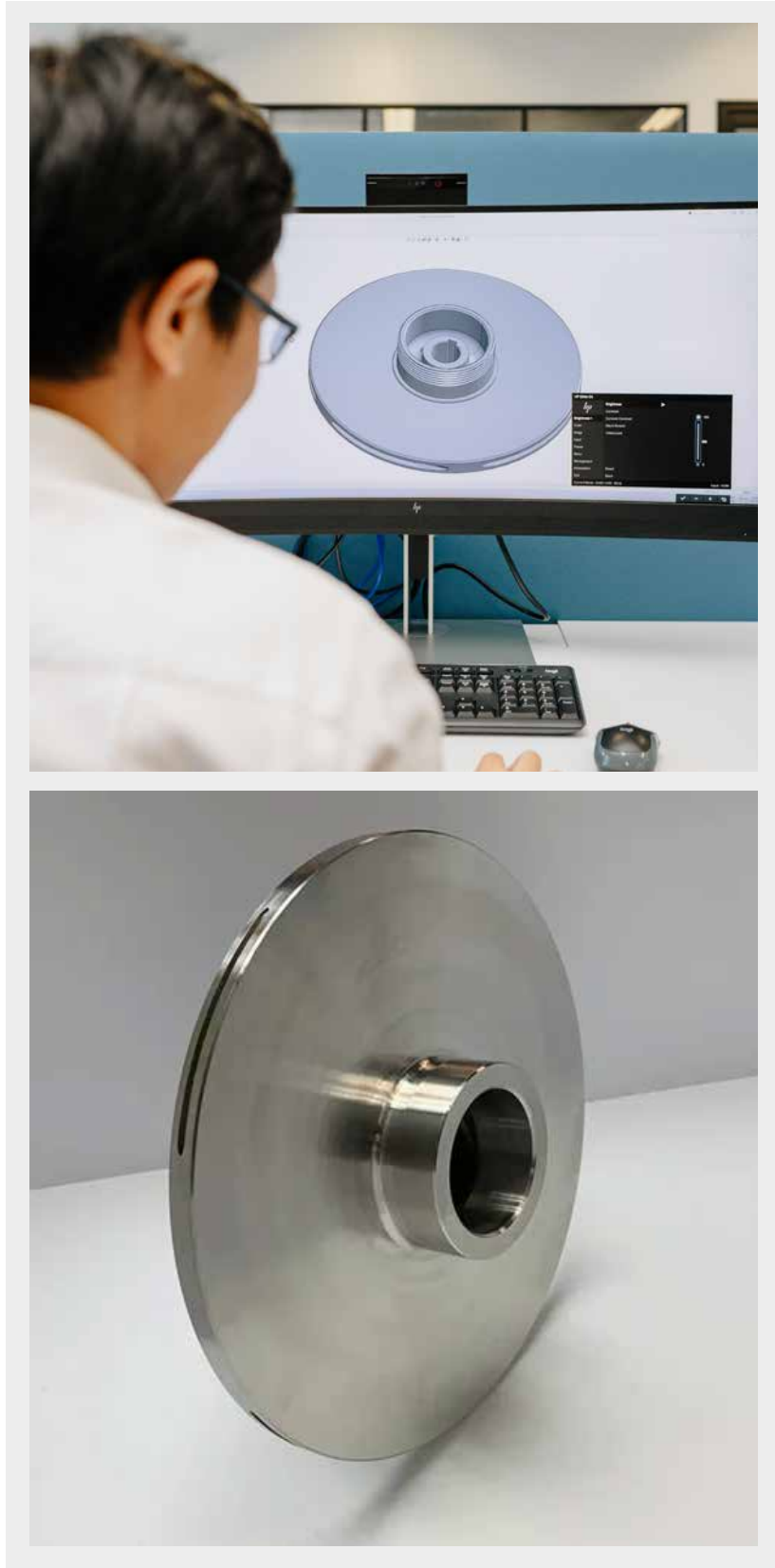
Fig. 5 An obsolete deck seal pump impeller for a Hafnia-operated vessel was reproduced on demand using Laser Beam Powder Bed Fusion in Stainless Steel 316L. The 2.6 kg replacement (153 x 153 x 45 mm) was delivered in four weeks, restoring pump functionality and avoiding lengthy spare-part lead times (Courtesy Pelagus)
