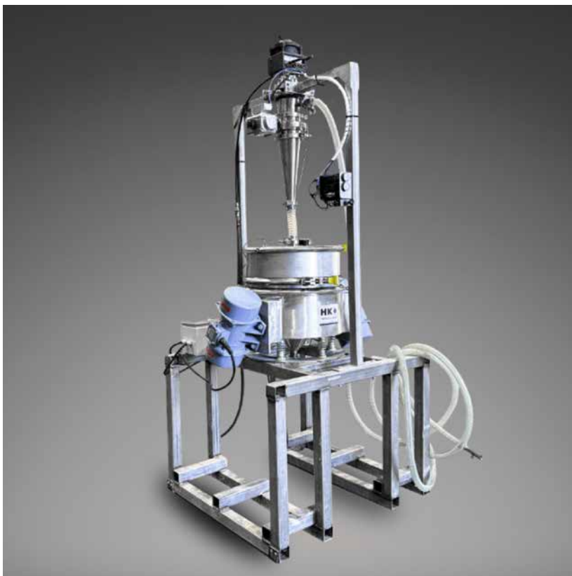
Fig. 4 The HK VacuSift Powder Conveying and Sifting System combines vacuum conveying and vibratory screening to recover and process powder from AM machines, drums, IBCs and other containers. It enables simultaneous conveying and screening as part of an integrated workflow (Courtesy HK Technologies)
