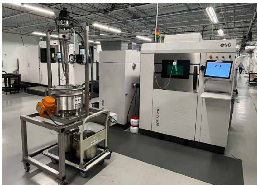
Fig. 1 HK Technologies' VacuSift Powder Conveying and Sifting System at Incodema3D's metal Additive Manufacturing facility, supporting powder recovery, screening and transfer (Courtesy HK Technologies/Incodema3D)
