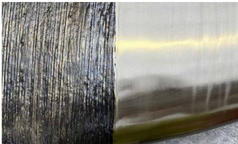
Fig. 9 Comparison of as-built and hand-polished wire-arc DED surfaces, showing the surface finish before and after manual finishing (Courtesy DEEP Manufacturing)
