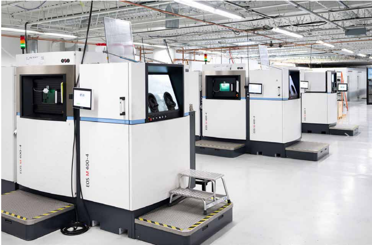
Fig. 3 EOS M 400-4 PBF-LB machines at Incodema3D's production facility. As the machine fleet expanded, efficient powder recovery and screening became increasingly important (Courtesy Incodema3D/EOS)
