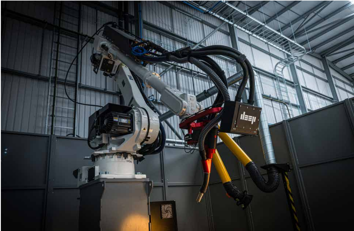
Fig. 16 Detail of a robotic welding arm used in DEEP Manufacturing's wire-arc DED production cells, where standard welding hardware is integrated with robotic motion control and process monitoring (Courtesy DEEP Manufacturing)
