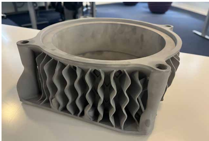
Fig. 11 PBF-LB motor flange with integrated cooling geometry, developed to improve heat dissipation during high-demand operation (Courtesy Pelagus)
