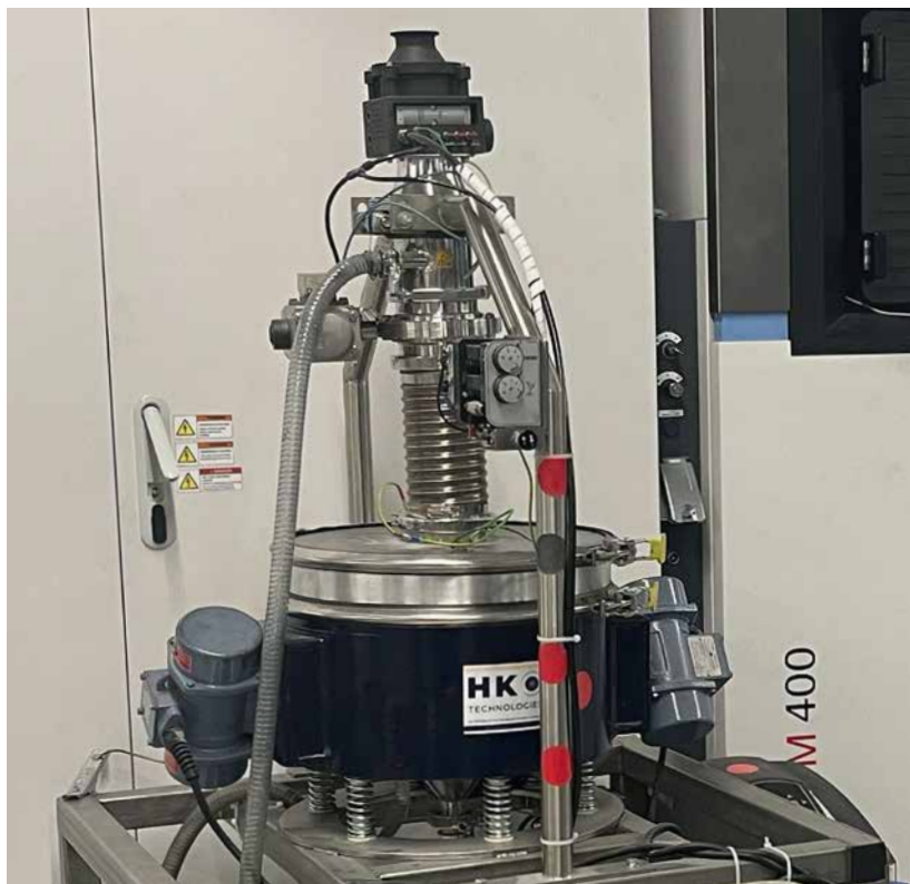
Fig. 8 The VacuSift system integrates vacuum conveying with vibratory screening, allowing operators to recover and screen powder in a continuous process. Unlike systems requiring separate conveying and screening steps, it supports simultaneous vacuuming and sieving (Courtesy HK Technologies)
