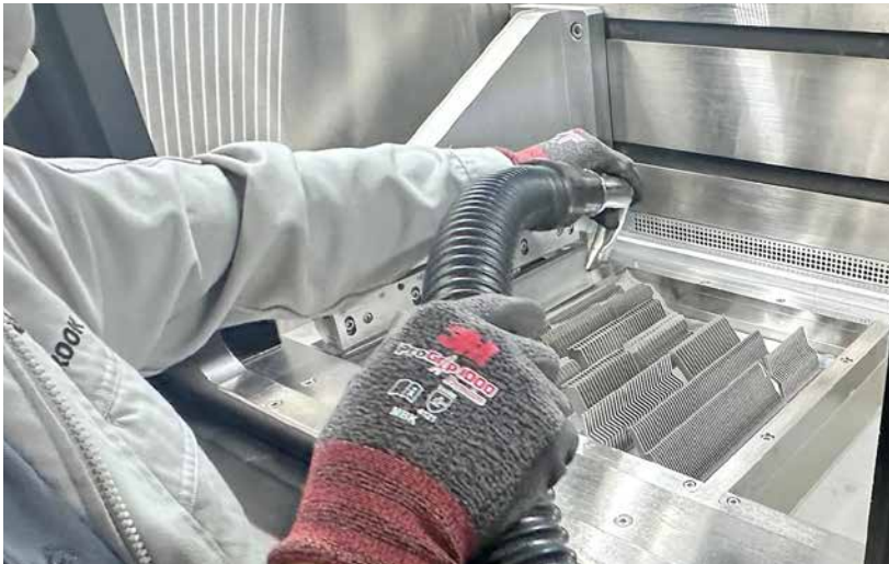
Post-processing the additively manufactured sipe mould components at Hankook (Courtesy Eplus3D)
