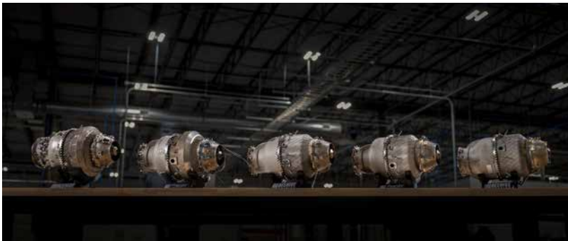
Frenzy 8 evolution (left to right) over a year, from First Engine to Test, to the flight-ready production unit (Courtesy Beehive Industries)
