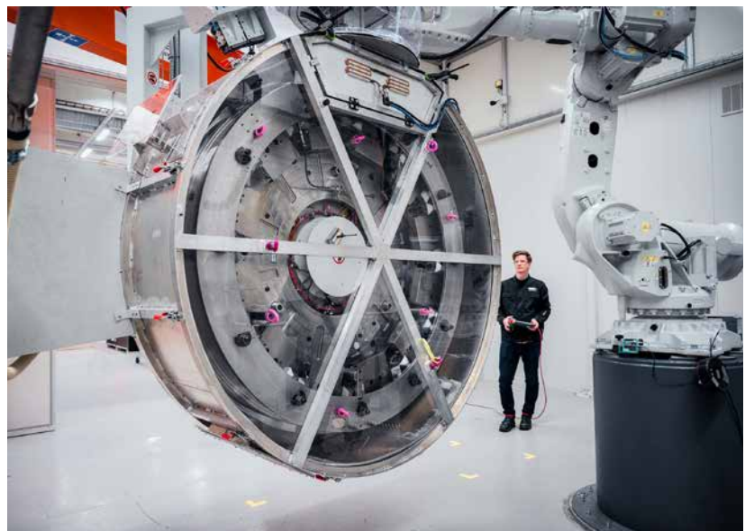
Fig. 1 GKN Aerospace's facility in Trollhättan, Sweden, hosted the SAE AMS AM Metals Sub-Committee spring meeting. The company is a leader in the adoption of AM for aerospace, with this fan case mount ring being a notable example (Courtesy GKN Aerospace)
