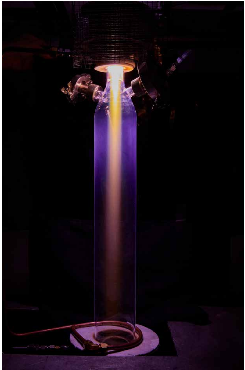
Fig. 6 Inside the UniMelt reactor, powder particles pass through a high-temperature microwave plasma plume, where they melt and form spherical particles through surface-tension effects (Courtesy 6K Additive)
