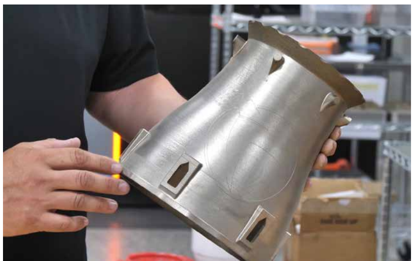
The additively manufactured afterburner casing for the hypersonic propulsion system combines several components into one part (Courtesy Renishaw)
