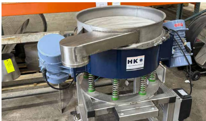
Fig. 7 Vibratory screener with an optional oversize discharge outlet for removing oversized particles, agglomerates and other unwanted material from the powder stream during screening (Courtesy HK Technologies)
