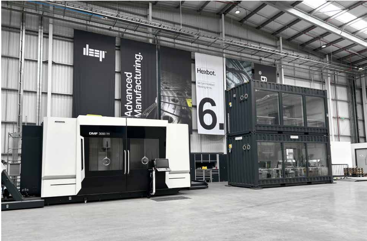
Fig. 13 DEEP Manufacturing's Avonmouth facility now includes large-scale five-axis CNC machining capability through the installation of a DMG DMF 300/11, enabling complex mill-turn components to be finished in-house with improved accuracy, reduced setup time and shorter lead times (Courtesy DEEP Manufacturing)
