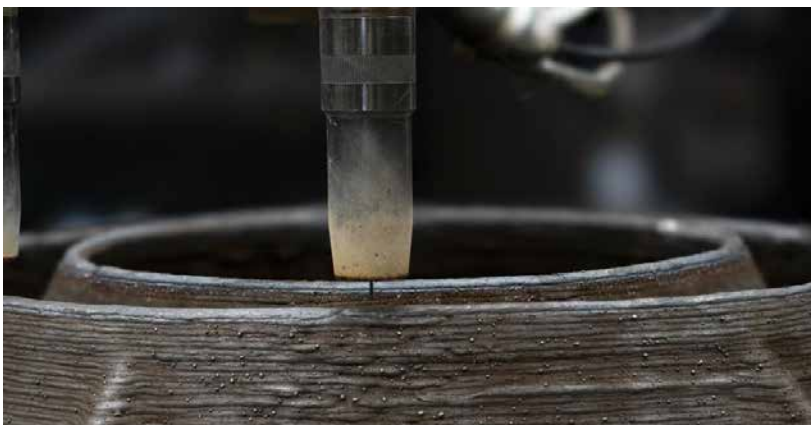
The Additive Manufacturing of the 410NiMo PM-HIP canister (Courtesy Carlos Jones/ORNL)
