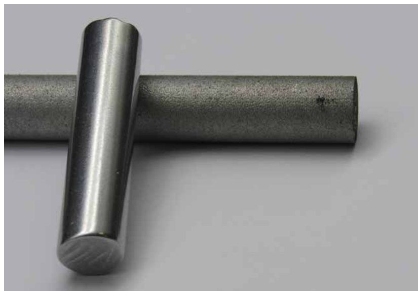
Fig. 9 PBF-LB/A6061-RAM2 specimens shown in as-built condition and after processing with REM's Extreme ISF Process (Courtesy REM Surface Engineering)
