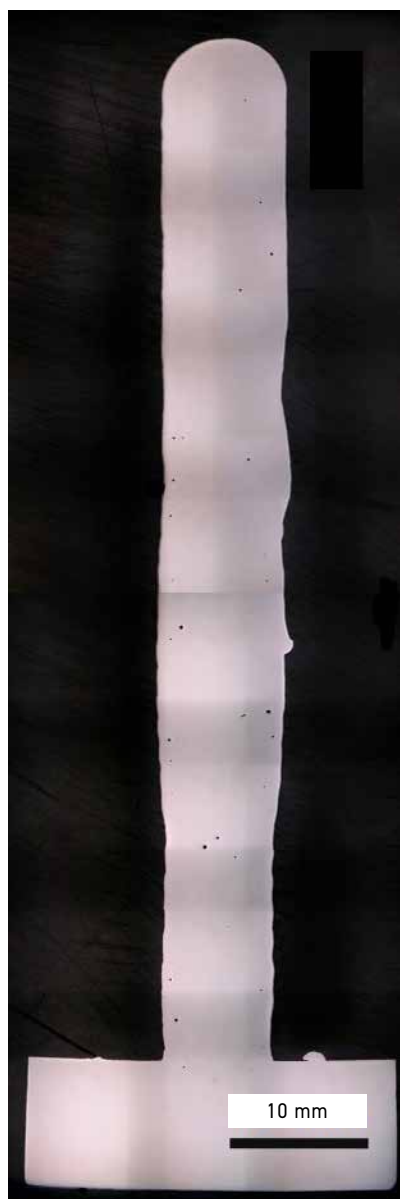
Fig. 9 Polished cross section of DED-EB/W wall, built using recycled wire (same component as C in Fig. 6) (Courtesy Pro-beam Additive GmbH)
