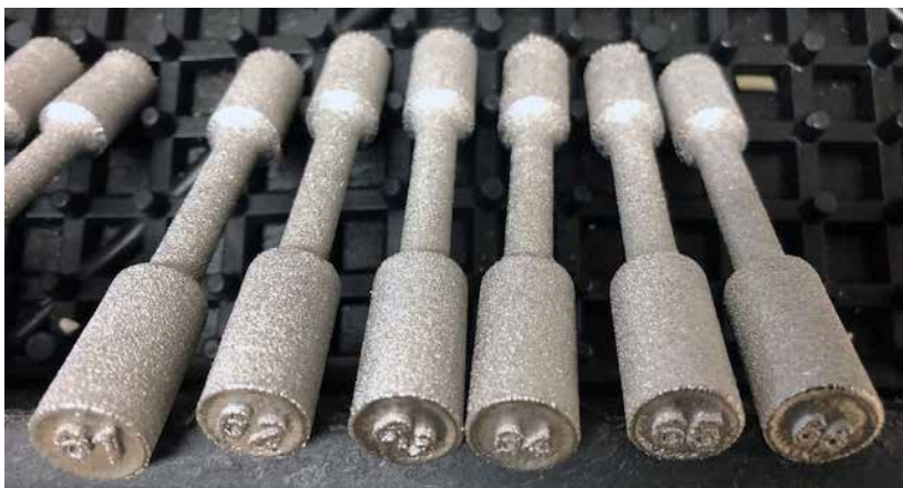
Fig. 4 Example of PBF-EB/Ti-6Al-4V components in their as-built condition (Courtesy REM Surface Engineering)
