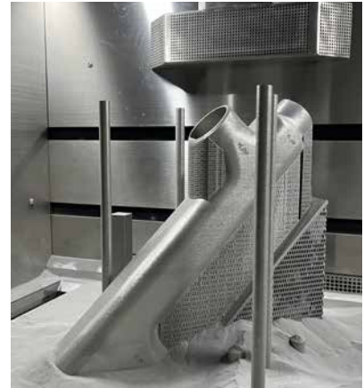
The heat exchanger was additively manufactured by TEMISTh using an Eplus3D EP-M300 (Courtesy Eplus3D)
