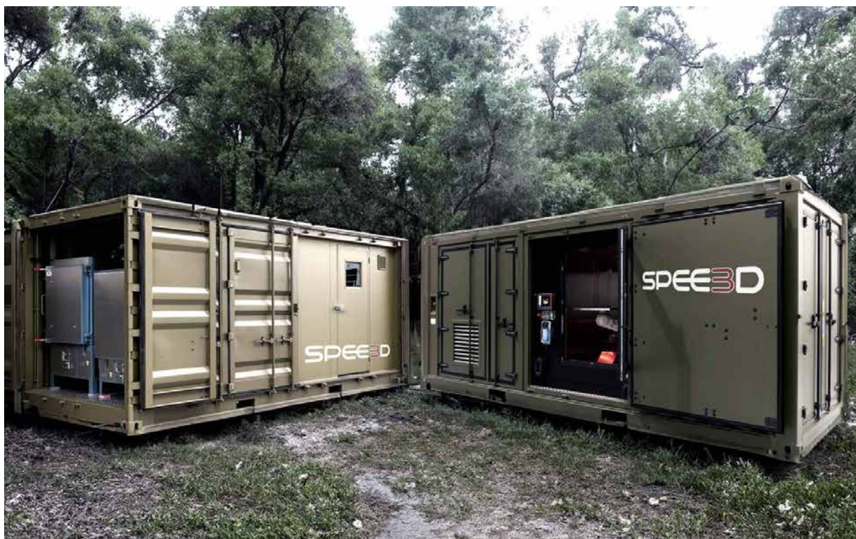
Fig. 4 SPEE3D's Expeditionary Manufacturing Unit (EMU) enables the rapid build, post-processing and validation of high-quality metal components exactly where they're needed (Courtesy SPEE3D)
