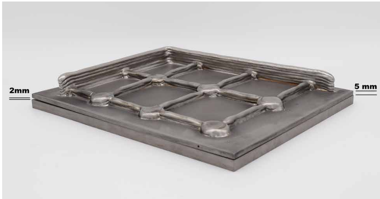
Fig. 7 DED-EB/W structural component (Ti6Al4V) for an application in the aerospace sector built on a 300 x 250 x 5 mm base plate, with a distortion of less than 2 mm. For comparison and highlighting the distortion, a 10 mm base plate is placed beneath (Courtesy Pro-beam Additive GmbH)
