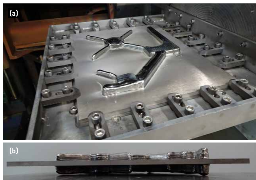
Fig. 8 DED-EB/W structural component (Ti6Al4V) for an application in the aerospace sector built on a 500 x 400 x 10 mm base plate. a: Top view of the component fixed on a flip frame. b: side view demonstrating minimised thermal distortion (Courtesy Pro-beam Additive GmbH)
