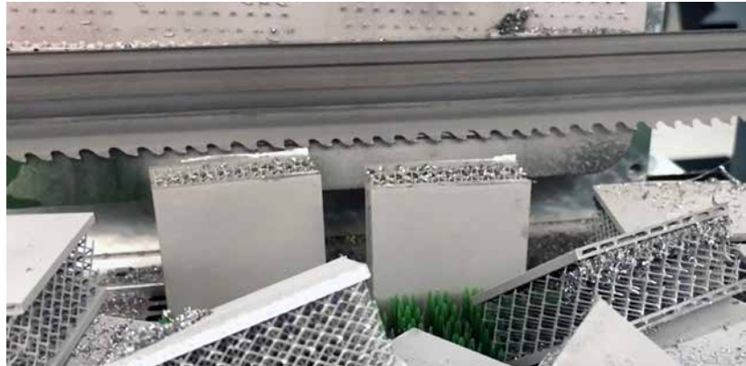
Klaeger's Bitron 3D and VBS 3D saws are designed for metal AM applications (Courtesy Klaeger)
