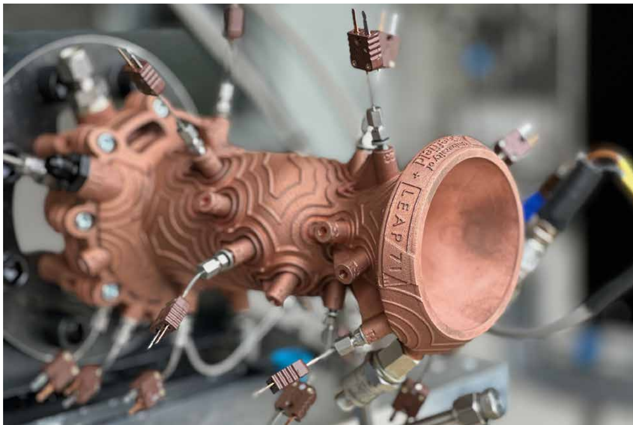
Fig. 4 Noyron TKL-5 thruster, producing 5,000 N of thrust and powered by kerosene and cryogenic liquid oxygen. Additively manufactured from CuCrZr by AMCM (Courtesy LEAP 71)
