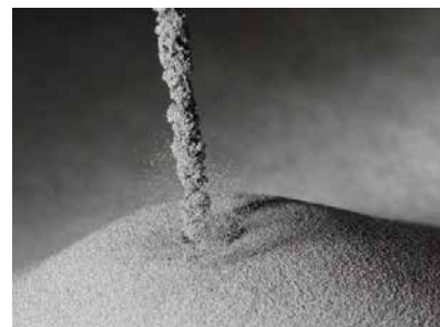
PyroGenesis titanium metal powder as produced by its NexGen plasma atomisation system (Courtesy PyroGenesis)
