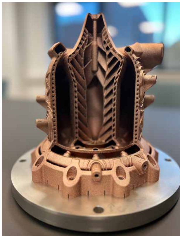
Fig. 9 A 5,000 newton annular aerospike rocket engine. The inner spike is regeneratively cooled using cryogenic liquid oxygen, while the outer jacket is regeneratively cooled with kerosene. Both hot propellants are then injected into the toroidal combustion chamber. Aerospikes offer greater efficiency than conventional bell-nozzle engines but are notoriously challenging to cool. The LEAP 71 engine was entirely designed using Noyron, additively manufactured by Aconity3D as a monolithic copper piece, and successfully hot-fired in December 2024. (Courtesy LEAP 71)
