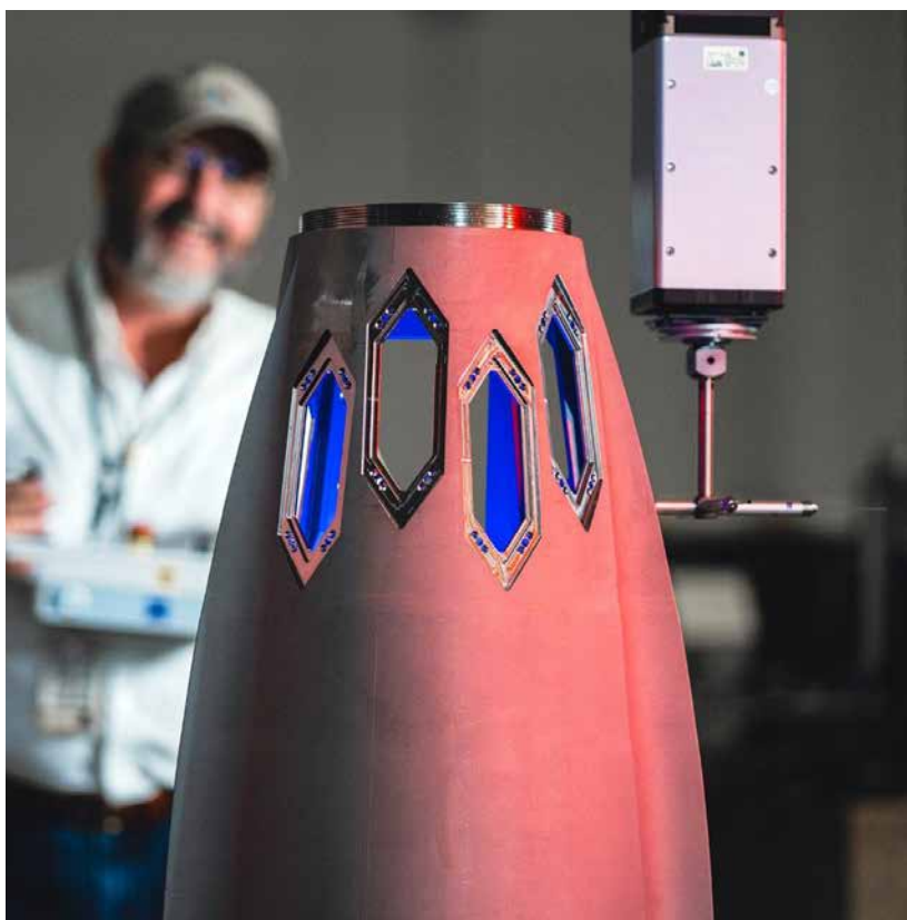
Fig. 2 In the US, Lockheed Martin has expanded its metal AM operations to meet the demand for advanced capabilities, such as this guidance housing for the Mako hypersonic missile (Courtesy Lockheed Martin)
