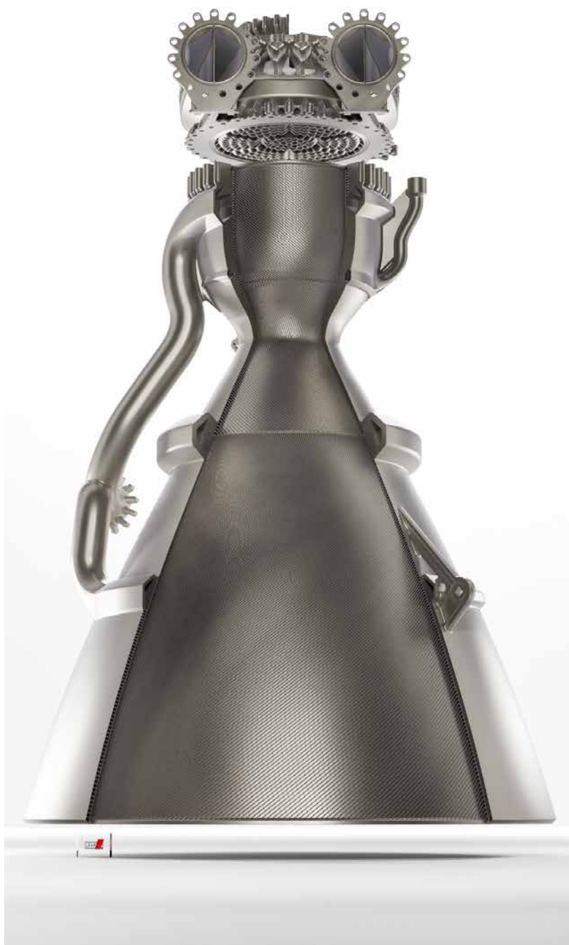
Fig. 7 Cut-through render of the XRB-2E6 rocket engine, generated using the latest version of Noyron. This 2,000,000 N (2 Meganewton) engine features a full-flow staged combustion cycle and stands at approximately 2 m tall. It represents the most advanced current rocket technology, comparable to the engines powering SpaceX's Starship. At the top, the injector directs hot gaseous methane through dual side inlets and hot gaseous oxygen through the centre, injecting the mixture into the combustion chamber below. The chamber wall and nozzle are cooled by an intricate network of channels through which methane propellant flows before being fed into the turbopump. The engine is now moving into manufacturing validation, with hot-fire testing targeted for late 2028 (Render courtesy LEAP 71)
