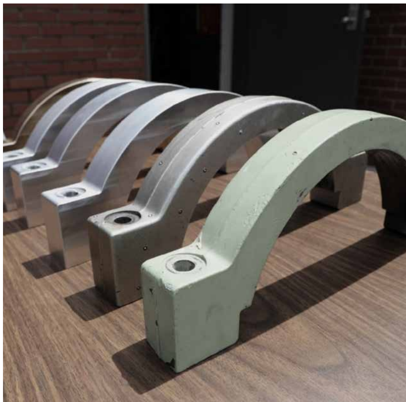
Fig. 5 A Bradley Fighting Vehicle's transmission mount (before and after) manufactured using SPEE3D technology by US soldier with no prior Additive Manufacturing experience during U.S. Army Combat Capabilities Development Command (DEVCOM) Army Research Laboratory (ARL) advanced manufacturing demonstration at the University of Tennessee Knoxville (Courtesy SPEE3D)
