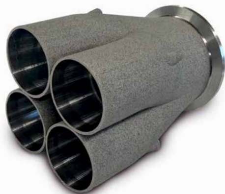
Wayland Additive has partnered with USC Racing – Formula SAE Team to produce and supply a titanium exhaust collector for its 2025 car (Courtesy Wayland Additive)
