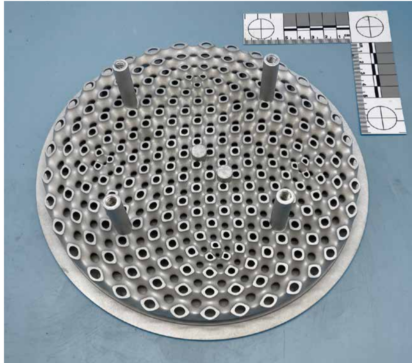
Fig. 15 PBF-LB/A6061-RAM2 reflector after Chemical Polishing [10]
