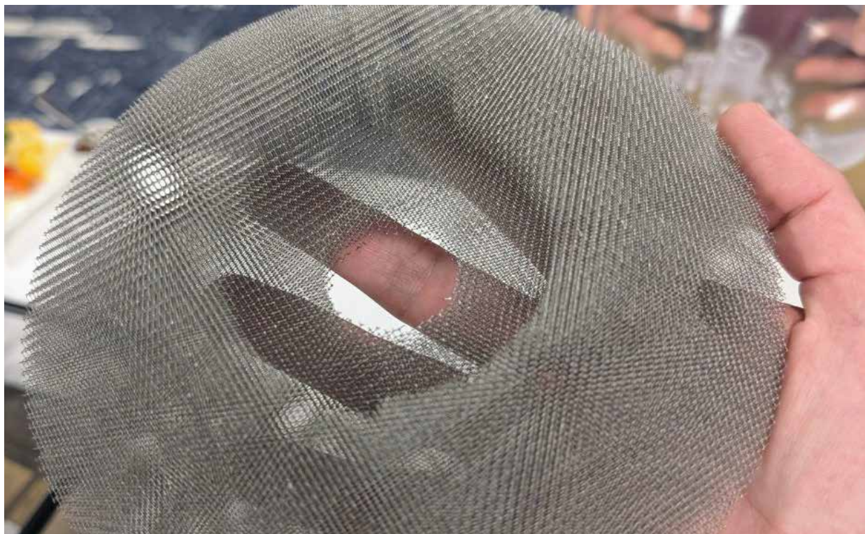
Fig. 20 Large MSR crush lattice component displayed at AMUG 2025 [14]
