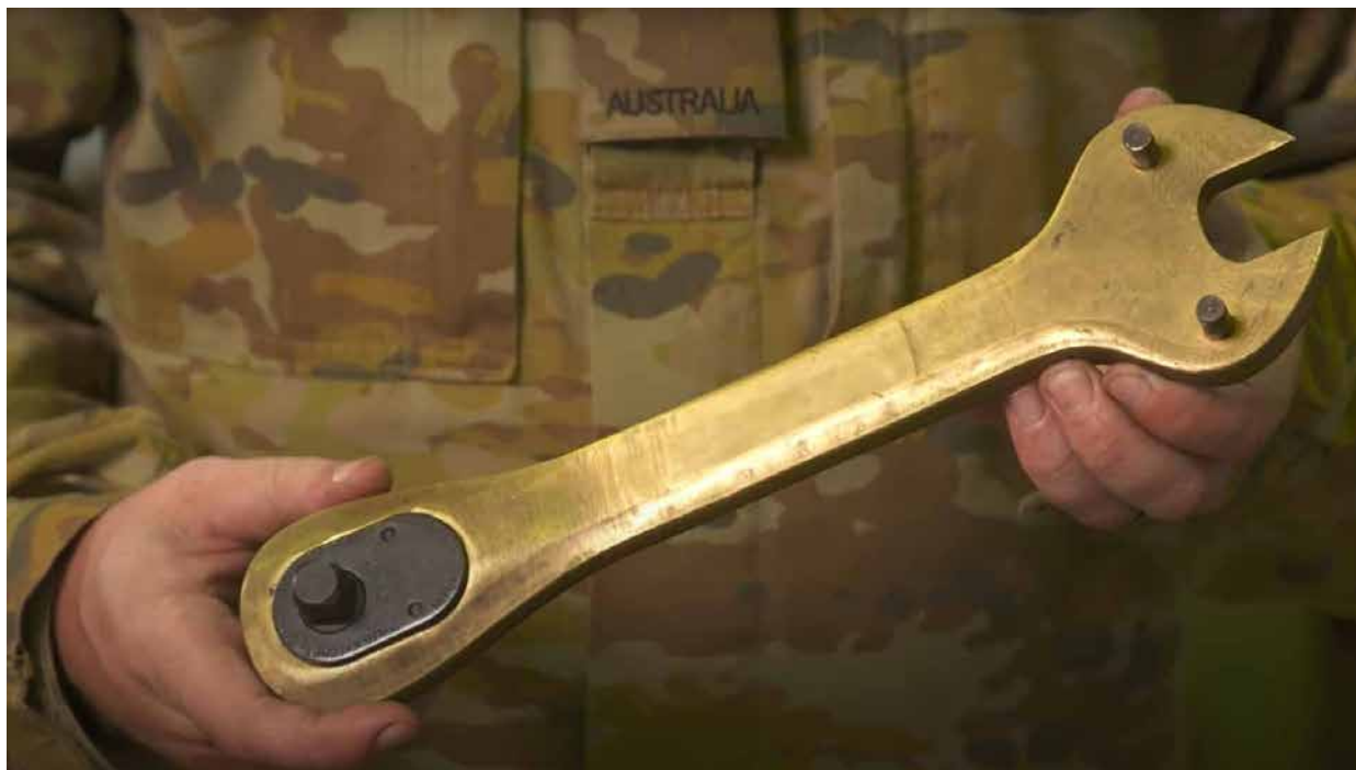
Fig. 11 A gunner's ratchet for the M242 Light Armoured Vehicle, additively manufactured in aluminium bronze using SPEE3D's Cold Spray technology (Courtesy SPEE3D)
