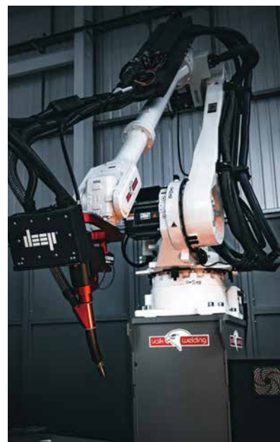
Each robotic arm can independently produce parts up to 3 m in diameter (Courtesy DEEP Manufacturing)
