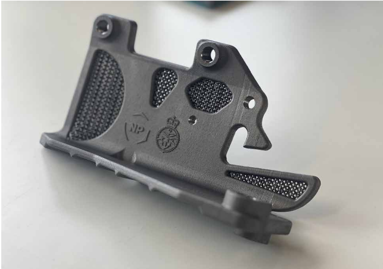
Fig. 6 The UK's Digital Manufacturing Centre (DMC) is working in partnership with NP Aerospace to deliver state-of-the-art metal engineering solutions as part of the UK Ministry of Defence's Project TAMPA. This Mastiff/Ridgeback patrol vehicle door latch was manufactured using Laser Beam Powder Bed Fusion (PBF-LB) Additive Manufacturing technology at the DMC (Courtesy DMC)
