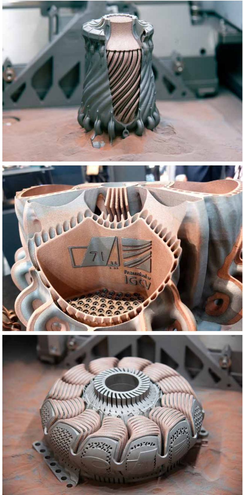
Fig. 12 Top: Multi-material heat exchanger. Middle: Multi-material (~300+ mm diameter) aerospike rocket engine; Above: Electric motor concept (~300 mm) diameter. All are produced using Fraunhofer IGCV's dual metal process on a Laser Beam Powder Bed Fusion (PBF-LB) machine from Nikon SLM Solutions (Courtesy Fraunhofer IGCV)
