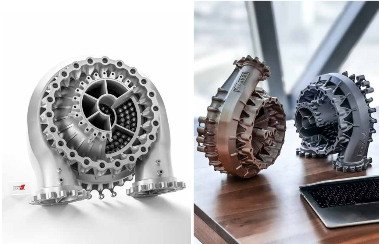
Fig. 8 Left: Render of the injector head for a 2,000,000 N (2 Meganewton) rocket engine featuring a full-flow staged combustion cycle. This advanced engine technology is comparable to the engines powering SpaceX's Starship. The injector directs hot gaseous methane through dual side inlets and hot gaseous oxygen through the centre before injecting the mixture into the combustion chamber. Right: Sub scale variants of the 2 MN engine injector head. Both support engines of 60,000 N. The left one is a gas-generator cycle engine, which takes in cryogenic liquid oxygen on the side before it mixes it with the methane coming from the regenerative cooling channels. The right injector supports full-flow staged combustion and takes in hot gaseous methane through twin inlets on the side and hot gaseous oxygen through a central inlet (Courtesy LEAP 71)
