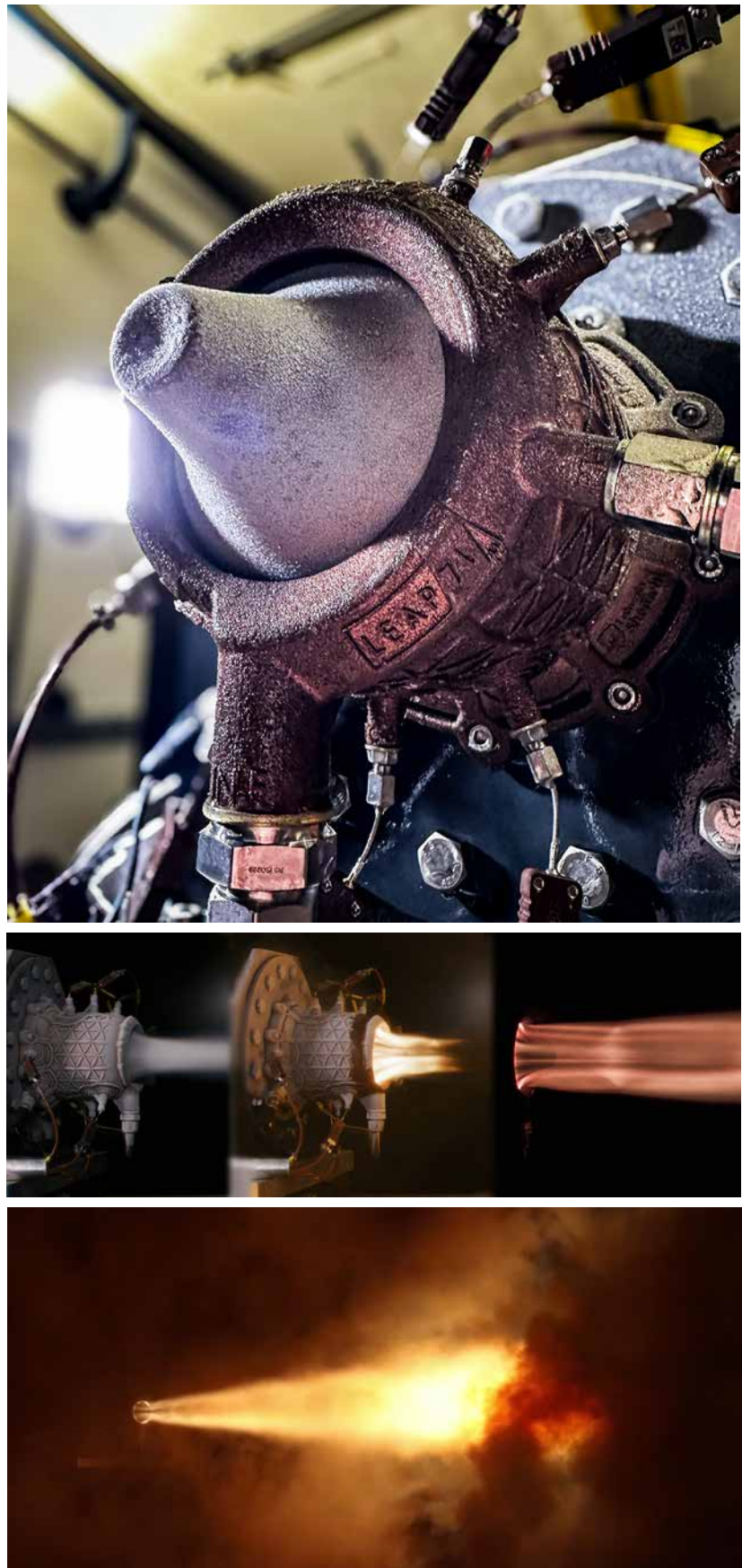
Fig. 10 Top: Aerospike rocket engine shortly before successful hot firing in December 2024. Middle: Aerospike rocket engine hot-fire sequence. Above: Aerospike rocket engine hot-fire (Courtesy LEAP 71)
