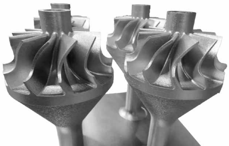
Additively manufactured rotating turbojet turbine wheels for the TJ150 engine (Courtesy Pratt & Whitney)
