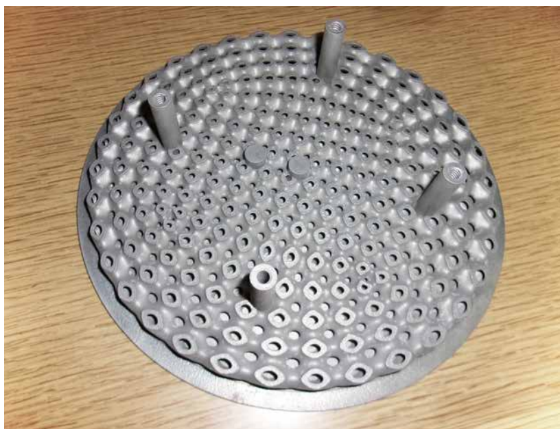
Fig. 14 As-built PBF-LB/A6061-RAM2 reflector [10]
