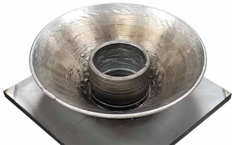
An example of an additively manufactured part produced using Sciaky's EBAM technology (Courtesy Sciaky)
