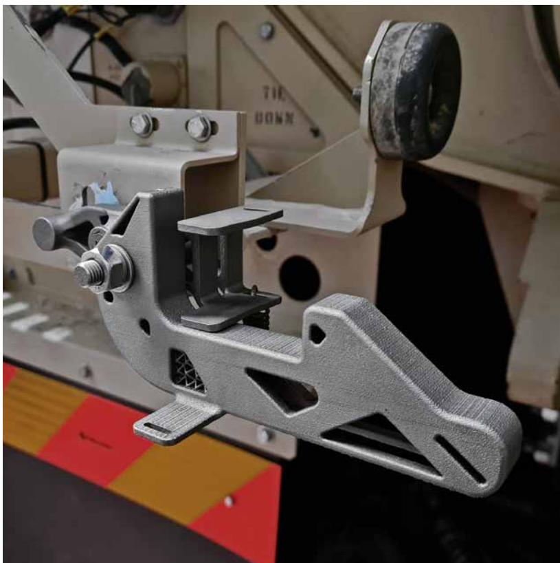
Fig. 7 Also manufactured by the Digital Manufacturing Centre (DMC), this Mastiff/Ridgeback patrol vehicle step assembly was manufactured using Laser Beam Powder Bed Fusion (PBF-LB) Additive Manufacturing technology (Courtesy DMC)
