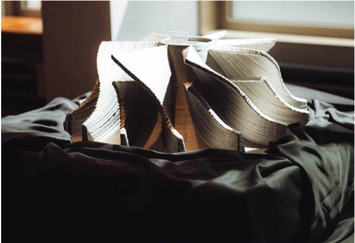
Fig. 11 Howden presented an impeller additively manufactured by GEFERTEC, This component has already gone from prototype to real application (Courtesy Studio vom Berg)
