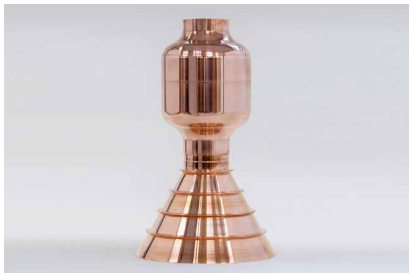
Fig. 1 A demonstrator rocket engine component post-machining. This was produced from copper using the DED-EB/W process and is 485 mm tall and 305 mm in diameter (Courtesy Pro-beam Additive GmbH)
