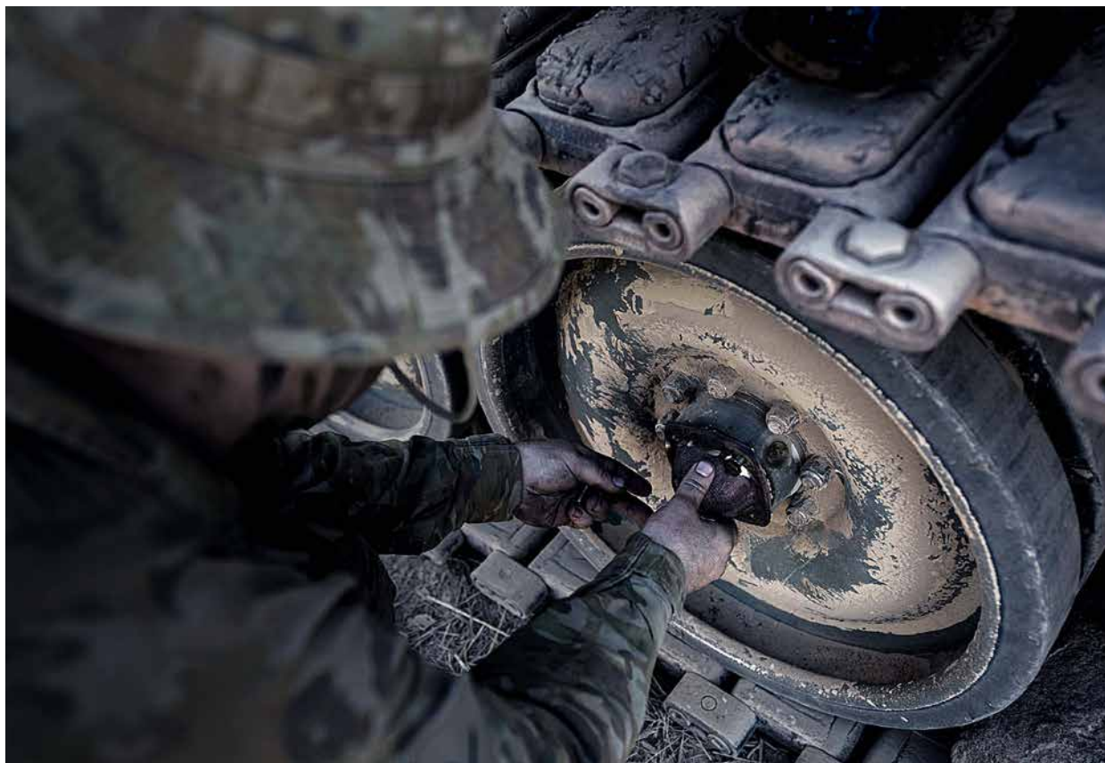
Fig. 9 A wheel bearing cover produced in the field using SPEE3D's Cold Spray Additive Manufacturing technology being fitted to an M113 fully tracked armoured personnel carrier (APC) (Courtesy SPEE3D)
