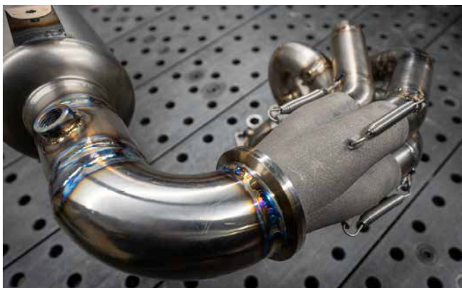
Wayland Additive has partnered with USC Racing – Formula SAE Team to produce and supply a titanium exhaust collector for its 2025 car (Courtesy Wayland Additive)
