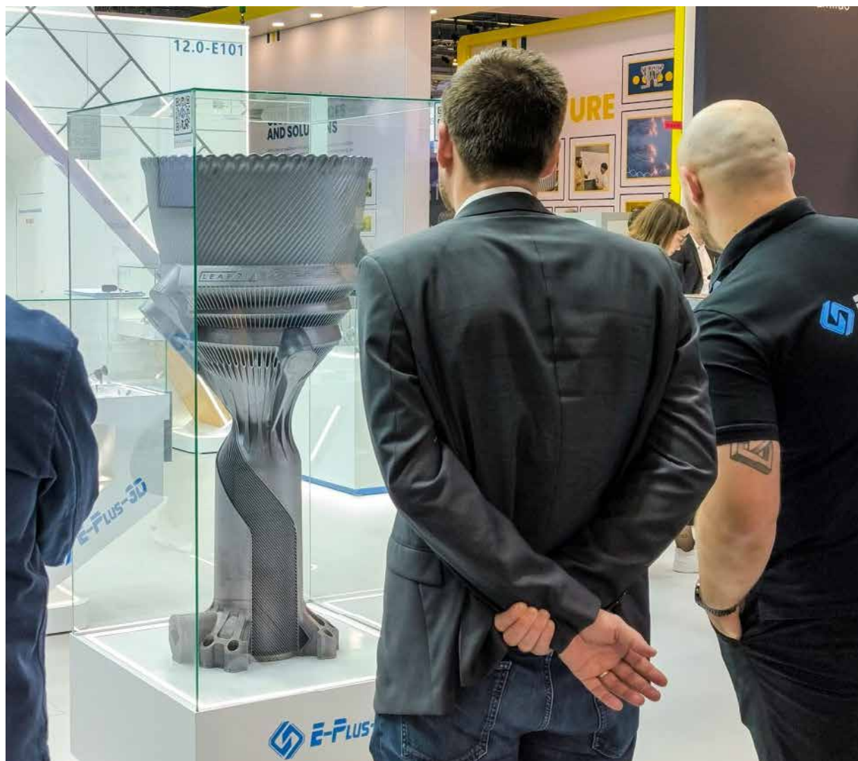
Fig. 13 Eplus3D and LEAP 71 produced the world's largest additively manufactured rocket thruster, exhibited at Formnext 2024. Built in a single 354 hour run on the EP-M650H, the 650 x 650 x 1600 mm thruster features a fully integrated design enabled by LEAP 71's Noyron software (Courtesy LEAP 71)
