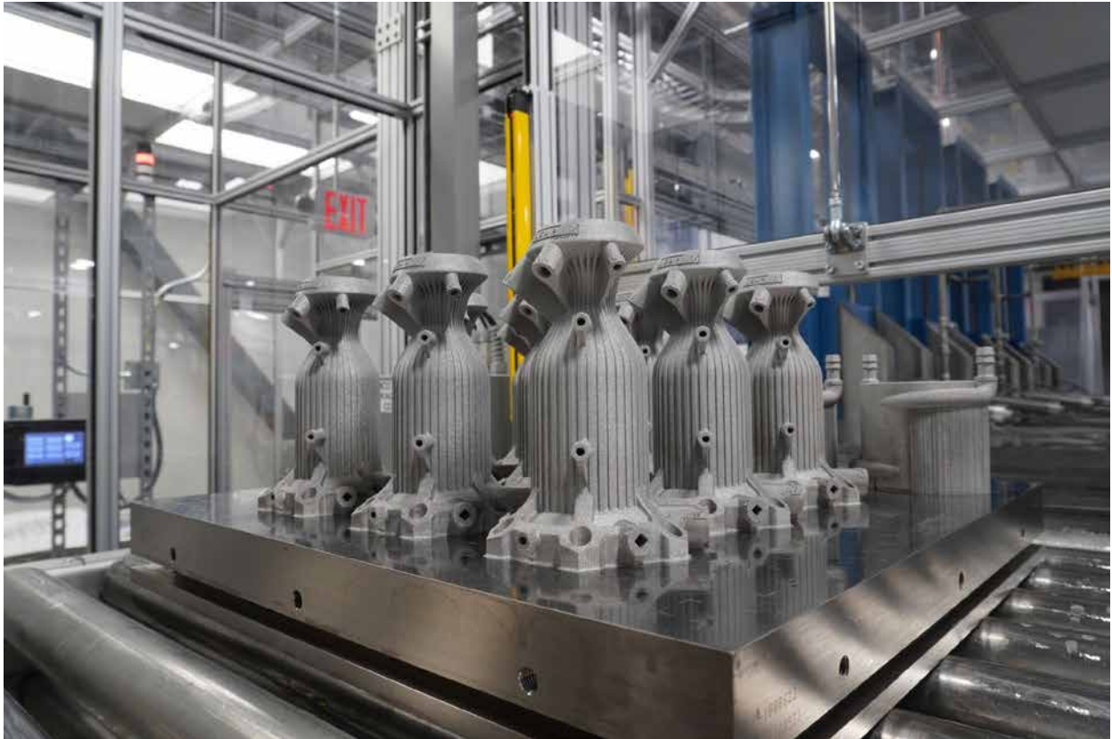
Fig. 6 Production batch of 2,000 N rocket thrusters, manufactured by VulcanForms (Courtesy VulcanForms)
