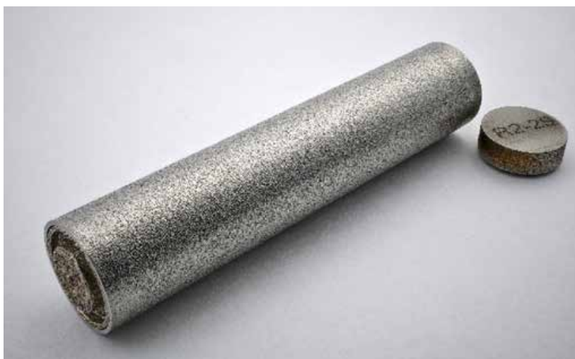
A research team from the Department of Energy's Oak Ridge National Laboratory (ORNL) has designed, manufactured, and successfully tested a specimen capsule for use in its High Flux Isotope Reactor (HFIR) (Courtesy Oak Ridge National Laboratory)
