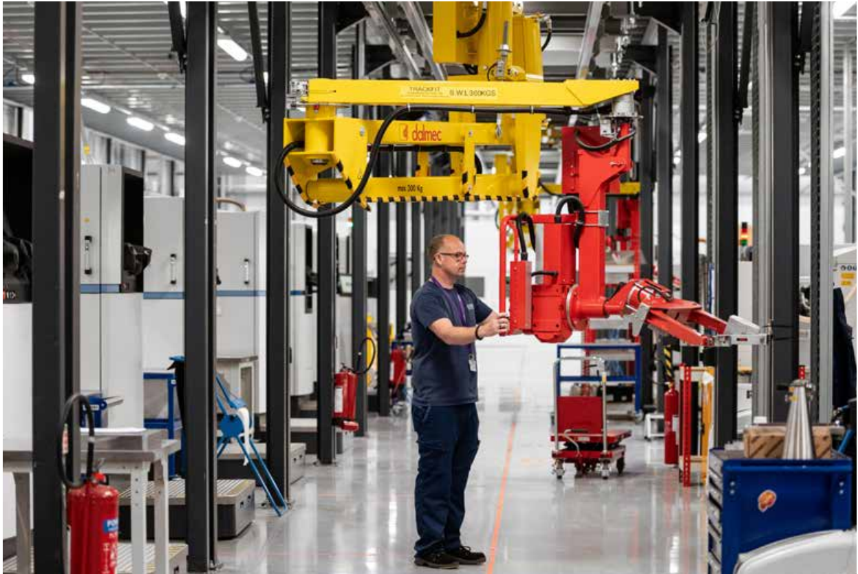
Fig. 5 This 'mech-lifter' is designed to speed up build turnarounds, supporting the drive for increased productivity measured by 'laser-on' time (Courtesy Materials Solutions Ltd)
