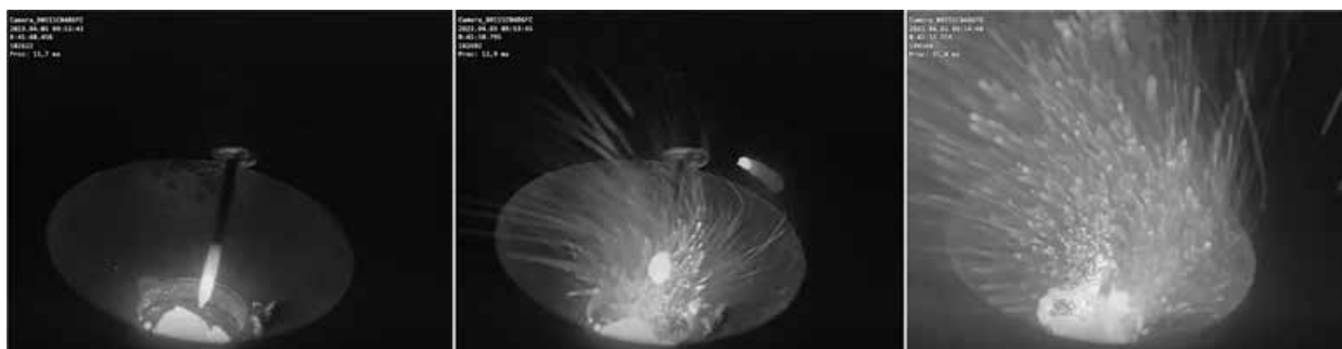
Laser-based ultrasonic atomisation process patented by Amazemet (Courtesy Amazemet)
