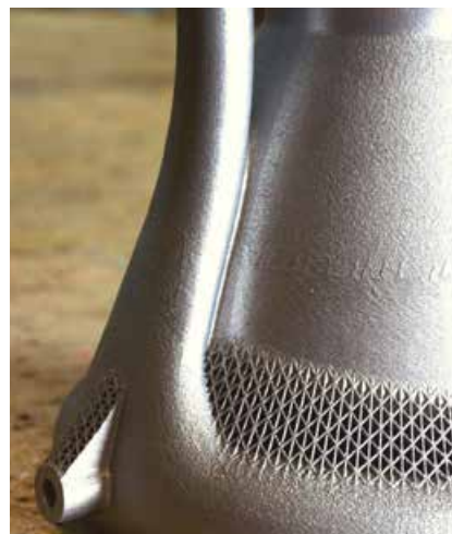
The DLX-150C built on the improvements seen in the DLX-150B. DARE removed the film cooling ring and redesigned a significant part of the engine as a single unit (Courtesy Delft Aerospace Rocket Engineering via LinkedIn)
