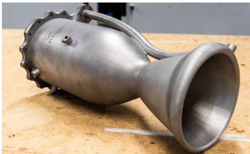
The DLX-150C built on the improvements seen in the DLX-150B. DARE removed the film cooling ring and redesigned a significant part of the engine as a single unit (Courtesy Delft Aerospace Rocket Engineering via LinkedIn)
