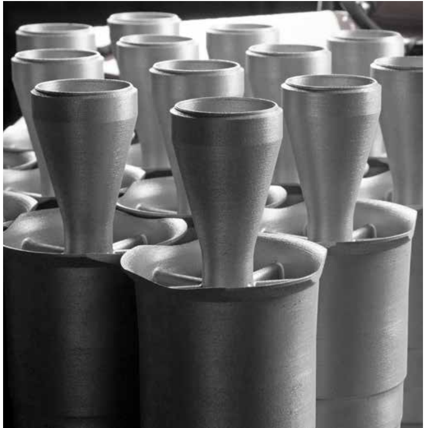
Fig. 3 High temperature PBF-LB gas turbine components produced by Materials Solutions for Siemens Energy (Courtesy Materials Solutions Ltd)
