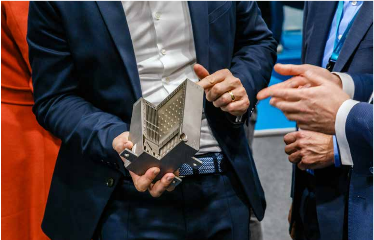
Fig. 8 A cutaway version of the AM chemical reactor revealing the internal geometry (Courtesy Siemens)
