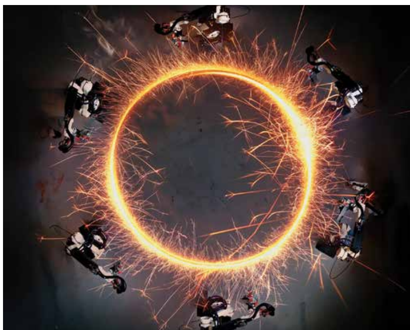
This six-arm synchronised configuration supports the production of parts up to 6.1 m in diameter and 3.2 m in height (Courtesy DEEP Manufacturing Ltd)
