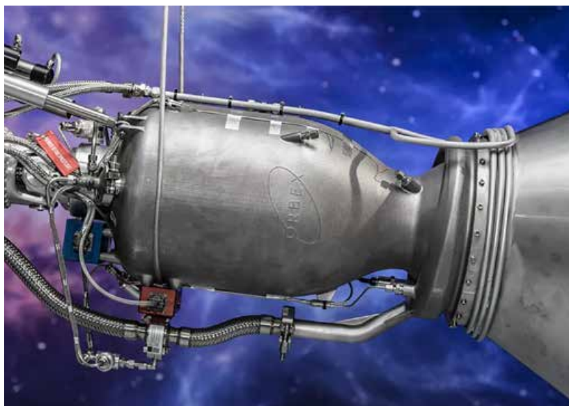
The Prime rocket is powered by a renewable bio-fuel (Courtesy Orbex)
