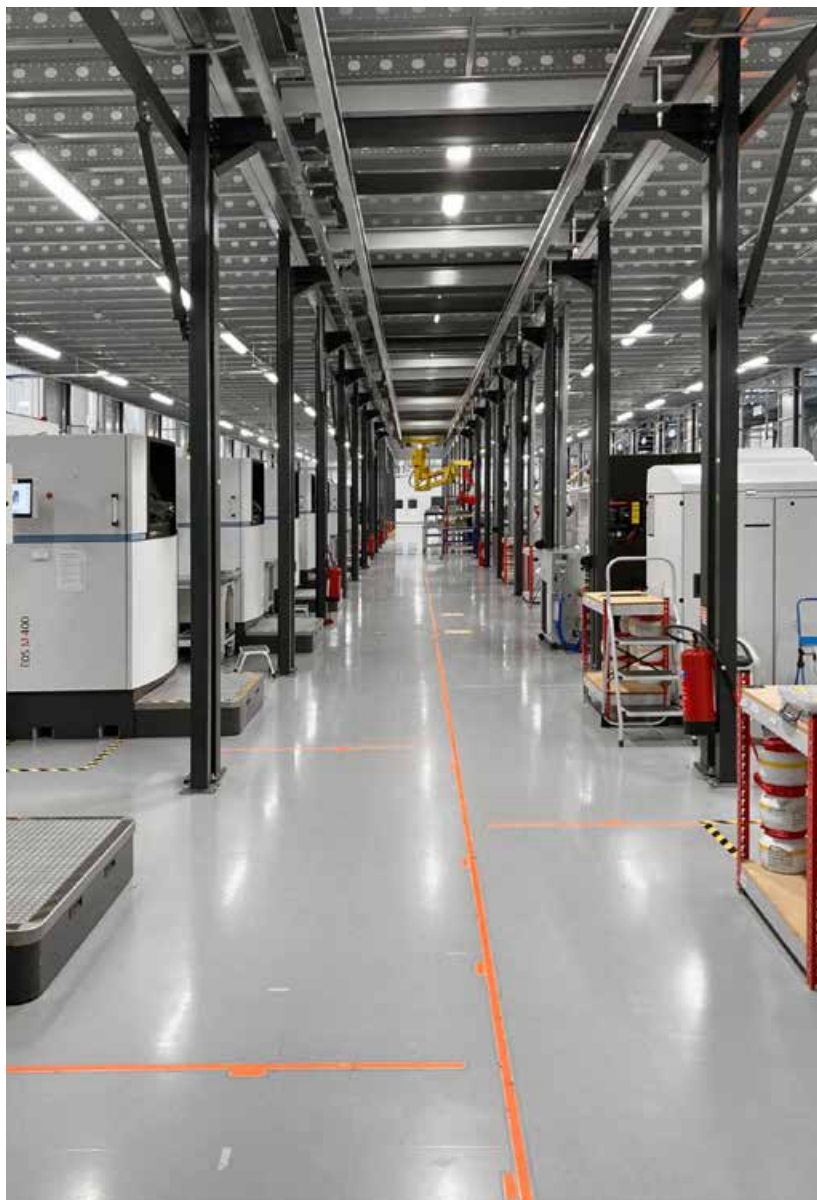
Fig. 4 A fleet of EOS M400-4 PBF-LB machines at Materials Solutions. Powder is supplied from the floor above (Courtesy Materials Solutions Ltd)
