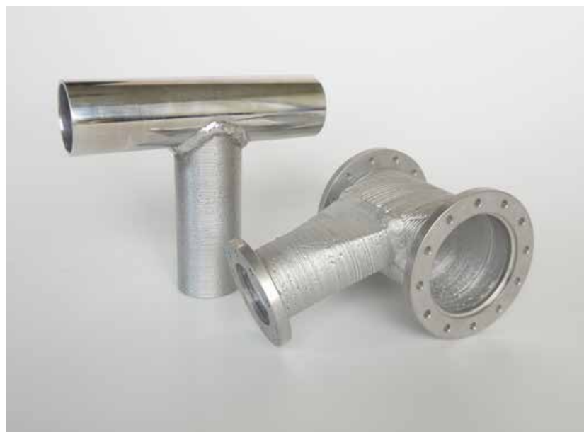
Fig. 1 Flanges welded onto housings manufactured using ValCUN's MMD technology (Courtesy ValCUN)
