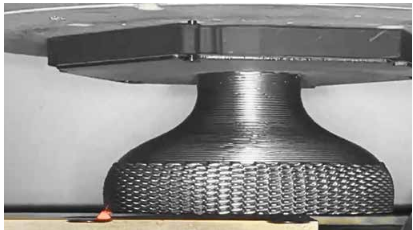
Fig. 6 Demonstration setup for upside-down printing (Courtesy ValCUN, supported by ESA)
