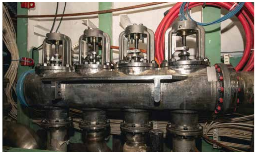
The additively manufactured manifold on US aircraft carrier Enterprise CVN 80 (Courtesy Ashley Cowan/HII)
