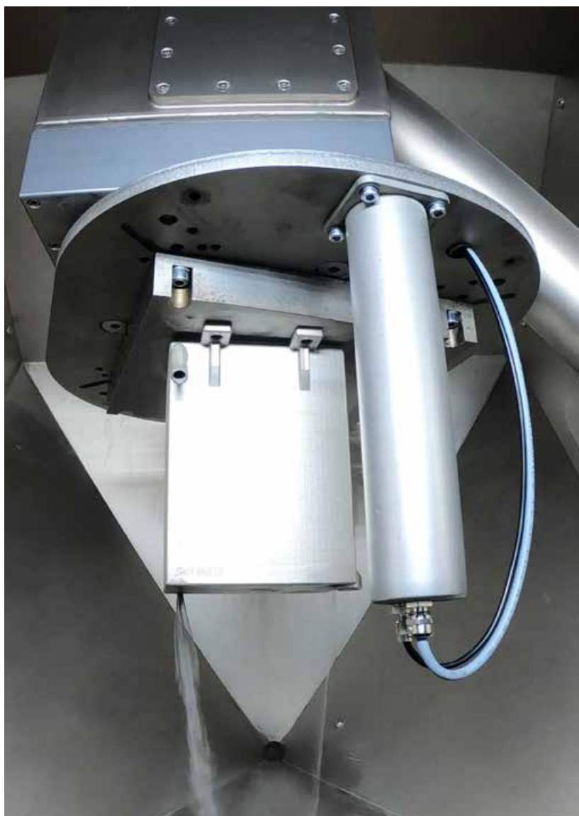
Fig. 10 The chemical reactor being depowdered inside a Solukon machine after simulation and planning using Pathfinder software (Courtesy Solukon)
