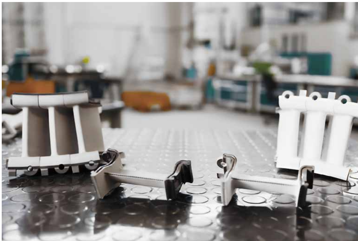
Fig. 6 High performance vanes for Siemens Energy gas turbines. Depowdering the fine cooling channels requires the utmost care and every part is inspected (Courtesy Materials Solutions Ltd)
