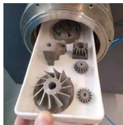
The Zetasinter 4L is four times bigger than the previous Zetasinter tubular furnace, allowing sintering of small production batches (Courtesy Nanoe)
