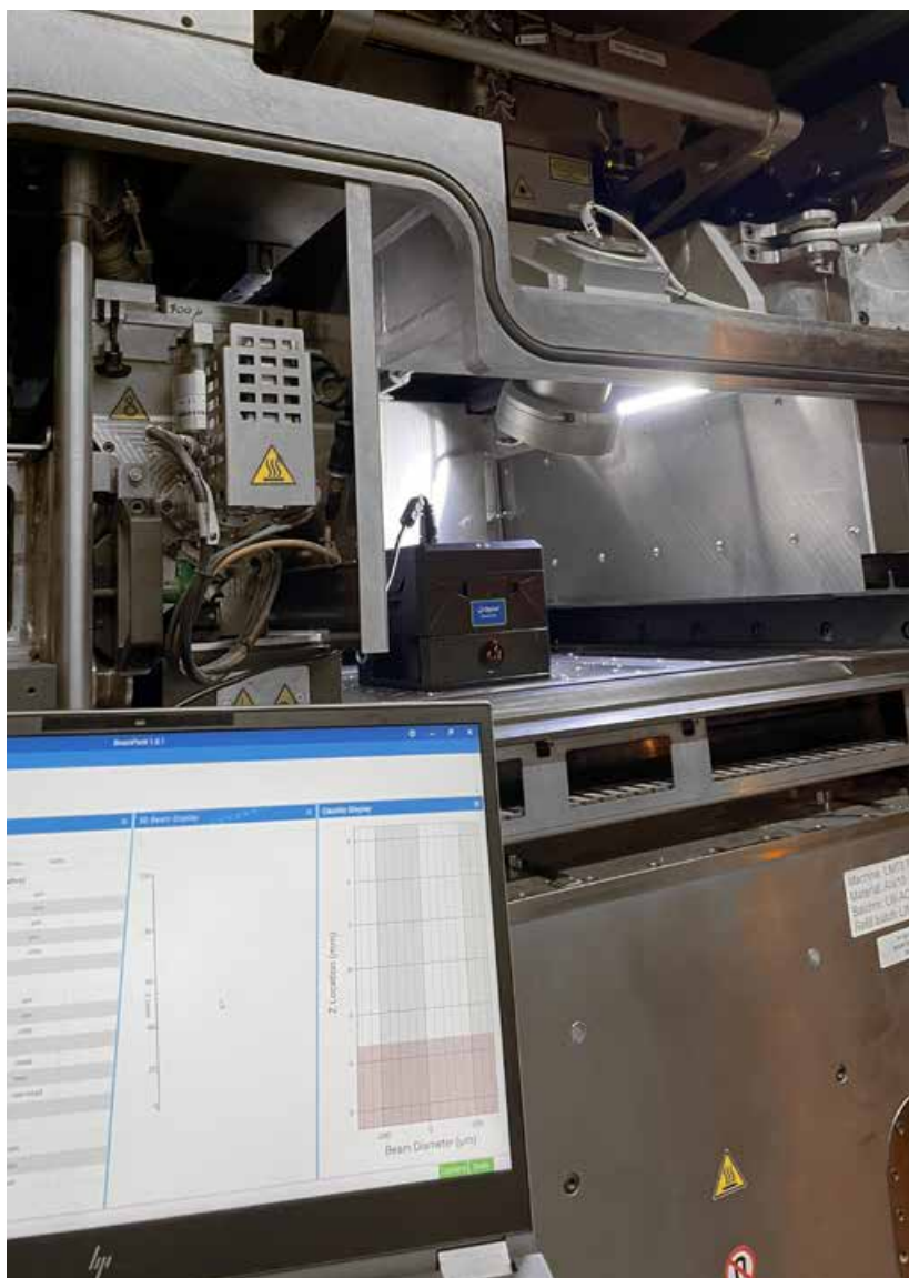
Fig. 2 Laser calibration underway at 3D Systems using MKS' Ophir technology (Courtesy 3D Systems)
