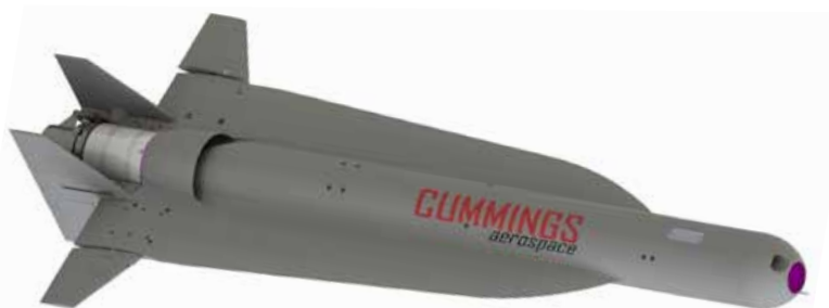
Hellhound is a turbo-jet-powered, additively manufactured kamikaze drone that can fly faster than 350 miles per hour. The drone is designed to equip the US Army's Infantry Brigade Combat Teams with the same combat power as Armoured Brigades (Courtesy Cummings Aerospace)
