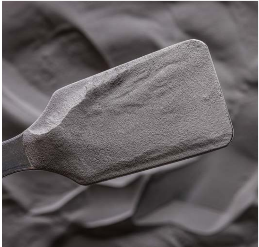
Fig. 8 Spherical Ti-6Al-4V powder developed by IperionX for use in AM and other processes (Courtesy IperionX)
