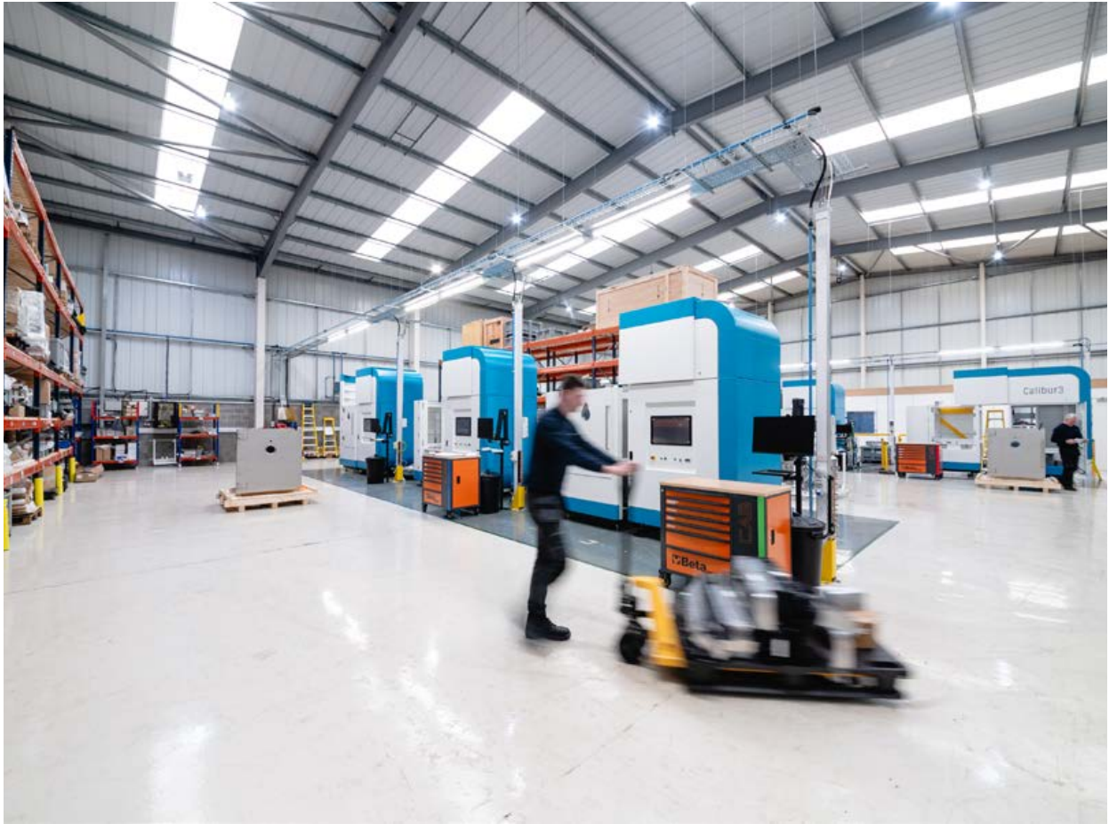
Fig. 12 Wayland Additive's production hall with the next ten Calibur3 machines in various stages of assembly (Courtesy Wayland Additive)
