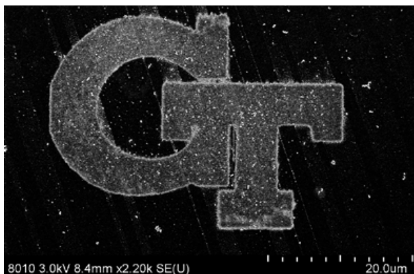
Scanning electron microscope image of additively manufactured silver Georgia Tech logo made with the SLP technique (Courtesy Jungho Choi/Georgia Tech)
