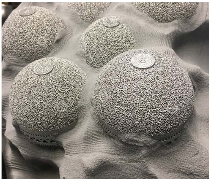
Fig. 2 Additively manufactured (PBF-EB) hip implants from implantcast GmbH shown in a powder 'cake' after the PBF-EB build process. The non-molten powder is blasted off in a Powder Recovery Station and fed back into the process through a special process (Courtesy implantcast GmbH)
