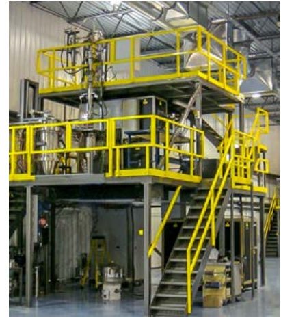
The company's Teknosphero-200 is designed for the large-scale production of spherical powders (Courtesy Tekna)
