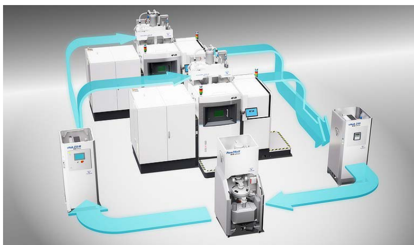
EOS closed loop Additive Manufacturing system diagram featuring Volkman powder transfer (Courtesy Volkman)
