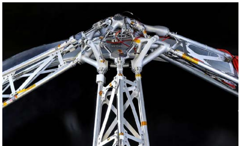
Fig. 1 Additively manufactured Scalmalloy thrust frame components (top centre of image), manufactured by APWORKS as part of an ArianeGroup GmbH technology demonstrator for the purpose of cryo-temperature and static loading tests, with funding from the German Aerospace Center (DLR) (Courtesy ArianeGroup/DLR/APWORKS)
