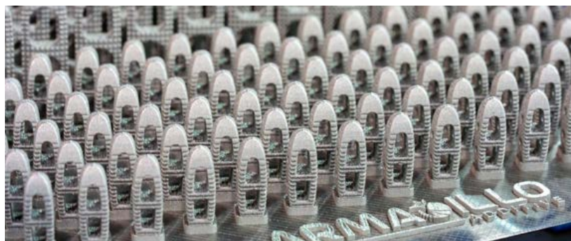
AM spinal implants made on the FormUp 350 (Courtesy Armadillo Additive)
