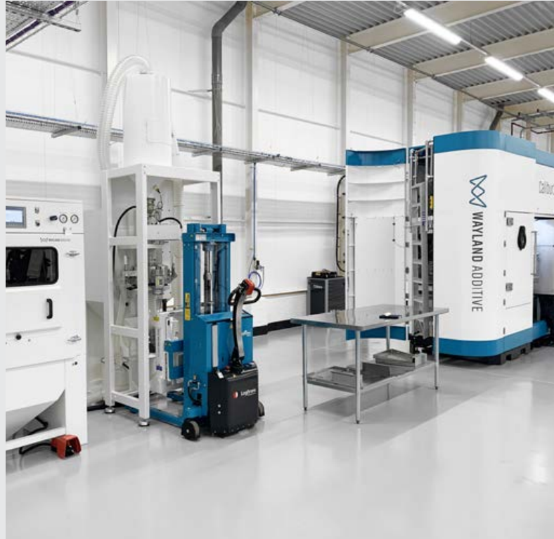
Fig. 10 Wayland Additive's Calibur3 metal AM machine installed at the RAF's Hilda B Hewlett Centre for Innovation (Courtesy Wayland Additive)
