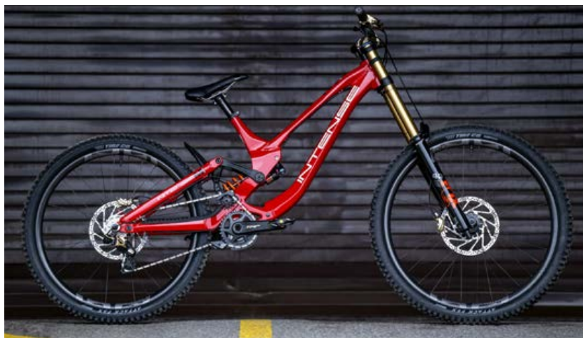
Intense Cycles is updating its classic M1 downhill race bike with an additively manufactured backbone (Courtesy Intense Cycles)
