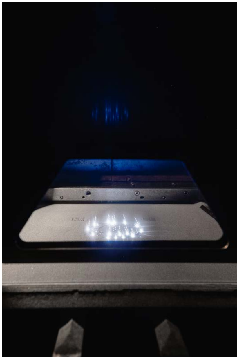
Fig. 4 A Calibur3 machine in operation. With NeuBeam, users can have thirty-two to sixty-four simultaneously active melt pools (Courtesy Wayland Additive)
