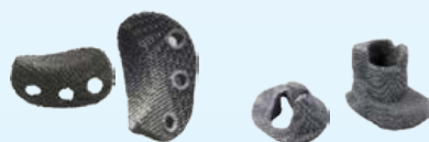
Customized porous Ta orthopedic implants.
