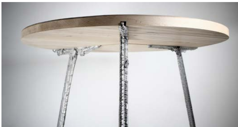
MIT Researchers have used Liquid Metal Printing to quickly additively manufacture parts such as chair frames and table legs (Courtesy MIT)
