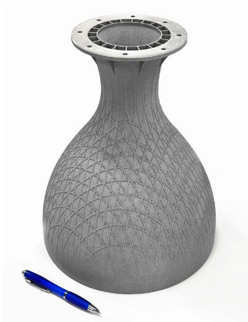
Fig. 6 A 330 mm x 280 mm double skinned rocket nozzle mock-up, produced in Ti-6Al-4V with no supports and no requirement for post-build stress relief, on a Calibur3 machine (Courtesy Wayland Additive)
