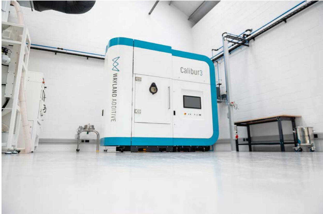
Fig. 5 A Calibur3 PBF-EB machine in the Production Suite at Wayland Additive is used on behalf of partners to run new projects (Courtesy Wayland Additive)
