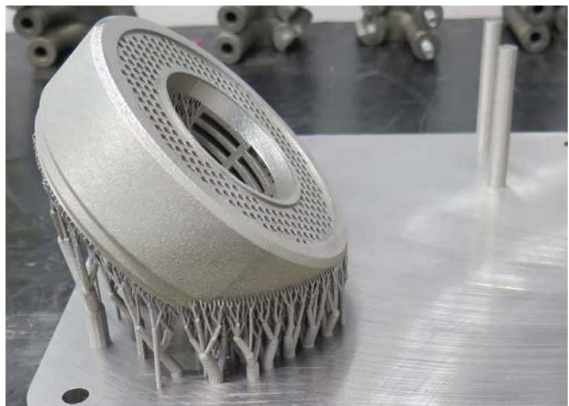
Fig. 1 The Variable Resistance Trim (VRT) component used in this study, shown on a successful build plate with power supports and test specimens (Courtesy Oqton/Baker Hughes)
