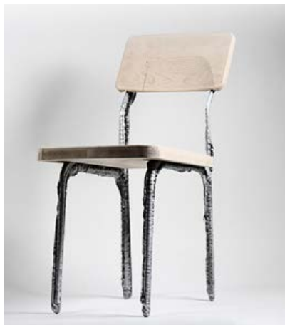
Researchers additively manufactured aluminium frames which were strong enough to withstand post-processing machining (Courtesy MIT)
