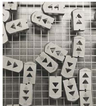
Zeda uses metal Additive Manufacturing to produce a range of medical implants (Courtesy Zeda Inc)
