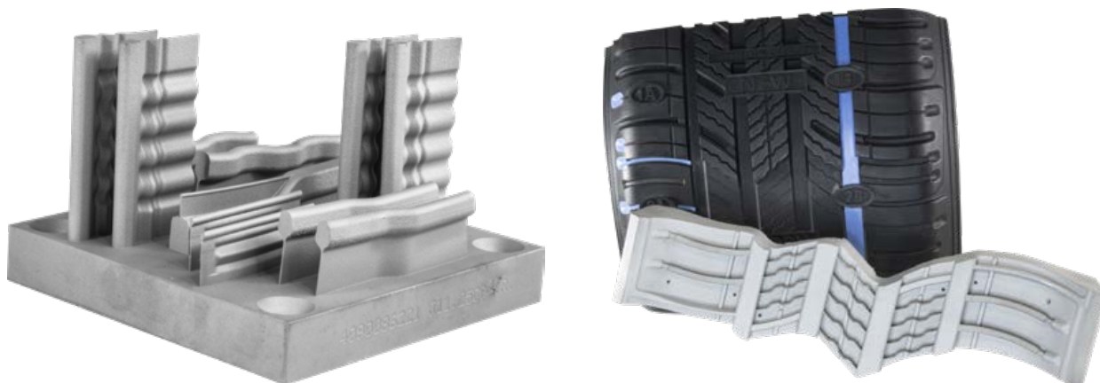
The build plate with tyre sipe mould inserts (left), and the tyre showing the tread pattern produced (Courtesy AddUp)
