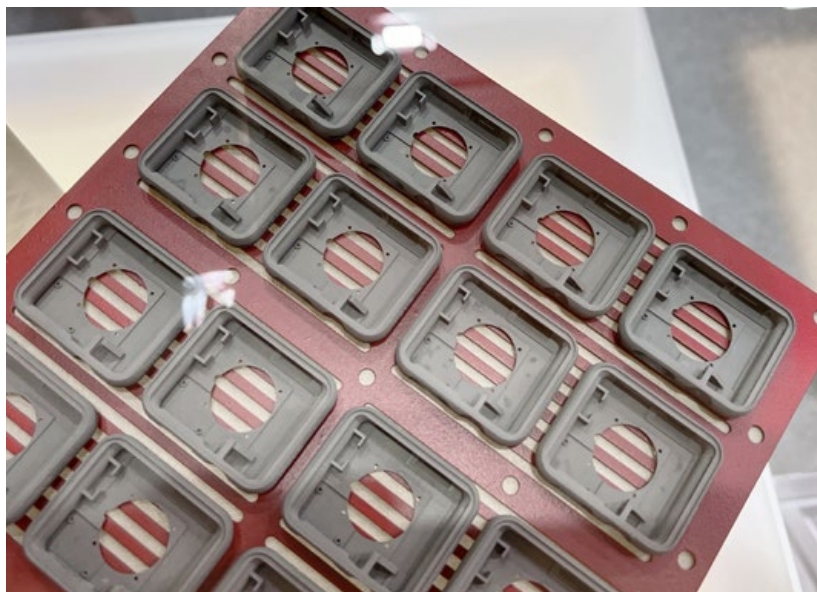
Fig. 13 Demonstration smartwatch cases produced on the Incus Hammer Pro40 machine. These parts are in the 'green', or un-sintered state. The MIM-like surface finish and resolution make this process highly attractive to producers of precision components who wish to minimise post-processing operations
