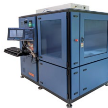
The Holo H200 has a build volume of 244 x 195 x 200 mm (Courtesy Holo)
