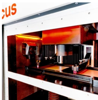
The Hammer Pro40 is designed for the production of large batches of intricate, specialty parts (Courtesy Incus GmbH)
