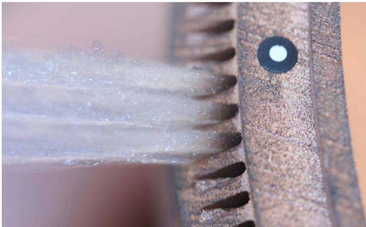
Fig. 8 Water flow test to confirm powder removal from internal cooling channels [5] (Courtesy NASA)
