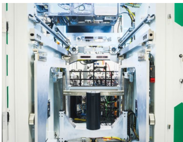
The fully swappable build cartridges in Seurat's Alpha system reduce machine downtime to minutes (Courtesy Seurat)
