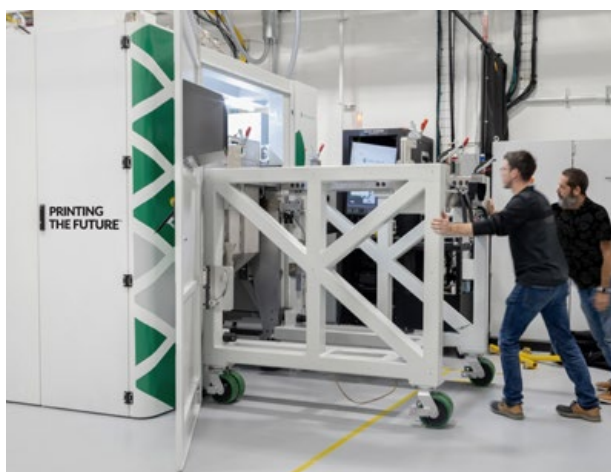
The fully swappable build cartridges in Seurat's Alpha system reduce machine downtime to minutes (Courtesy Seurat)
