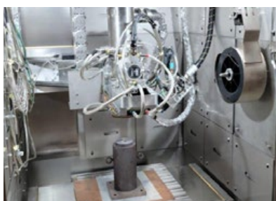
The EBAM-53 fits in a standard shipping container and is targeted at users who require research on a smaller scale, before a move up to the larger machines in Sciaky's range (Courtesy Sciaky)
