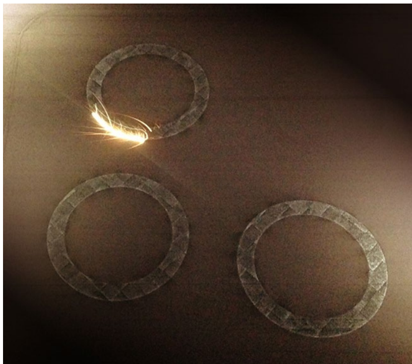
Fig. 5 GRCop-42 chambers being manufactured simultaneously by PBF-LB (Courtesy NASA)
