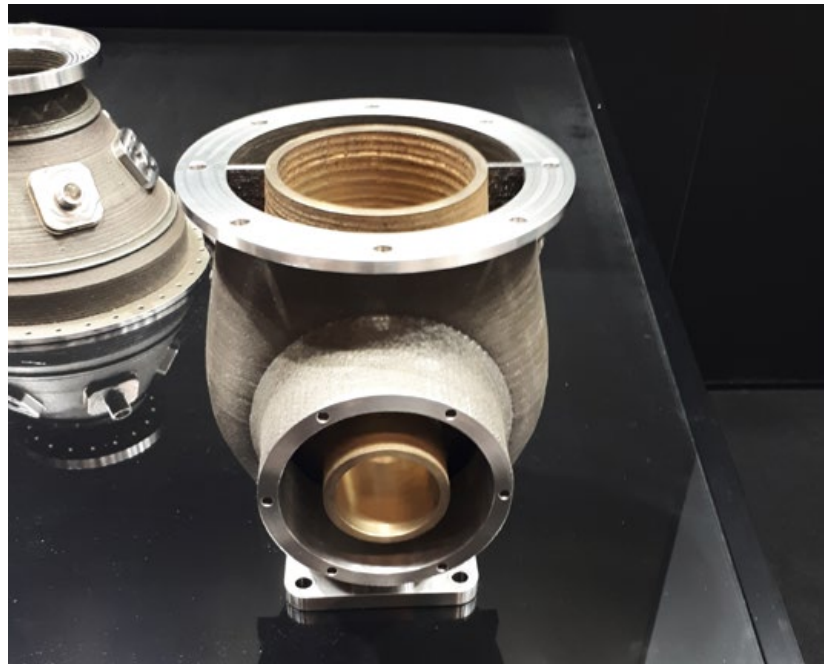
Fig. 11 A co-deposited bi-metallic valve housing displayed by DMG Mori and manufactured on the company's LASERTEC 65 DED Hybrid machine (Courtesy Martin McMahon)
