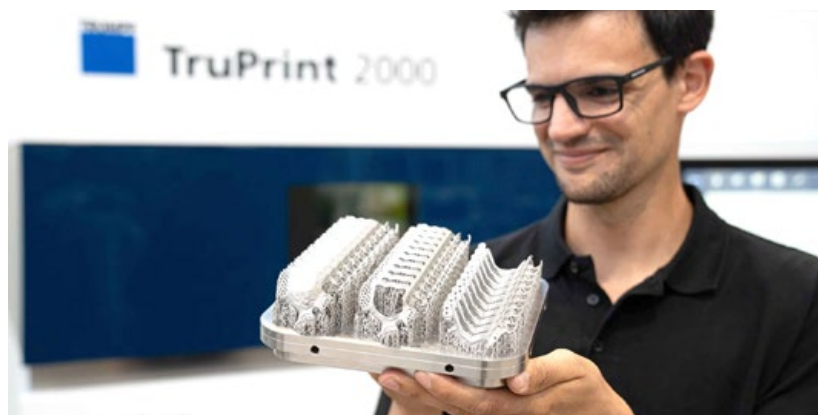
The square build plate and higher laser power of the updated TruPrint 2000 increases productivity (Courtesy Trumpf)
