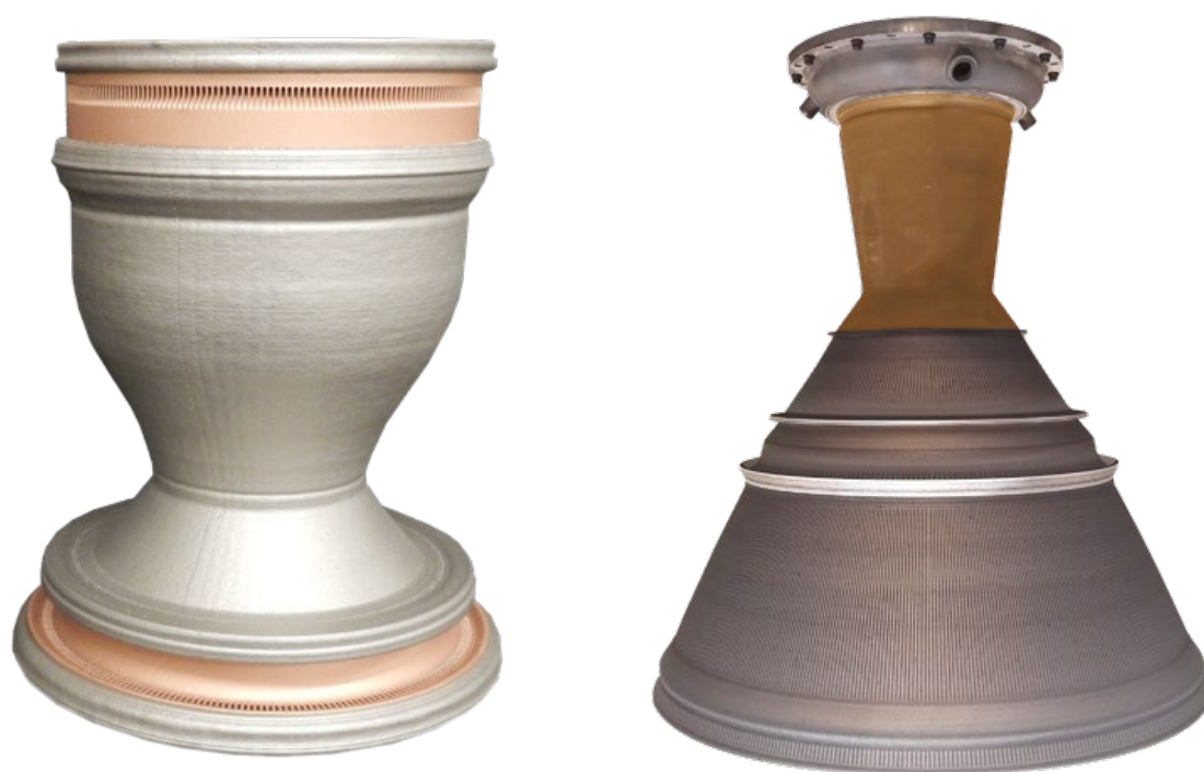
Fig. 11 Bimetallic thrust chambers using PBF-LB GRCop-42 for high conductivity and other superalloys for higher strength-to-weight ratio (Courtesy NASA)
