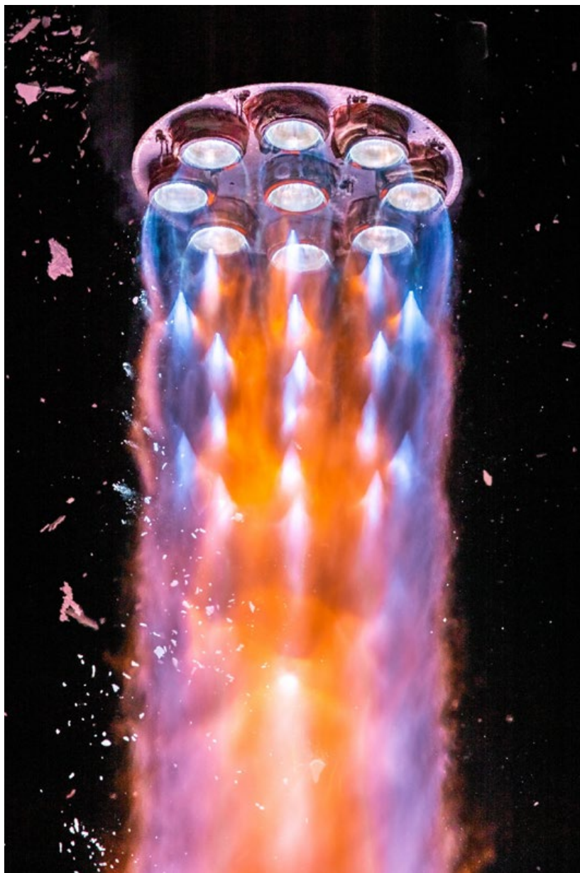
Fig. 2 PBF-LB GRCop-42 is used for Relativity Space's the Aeon 1 engines (Courtesy Relativity Space/photo John Kraus)
