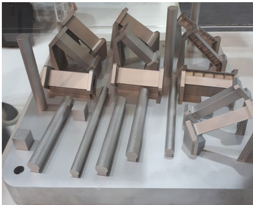
Fig. 15 An example of how Elementum 3D uses Dyndrite software to achieve low angle build parameters (Courtesy Martin McMahon)
