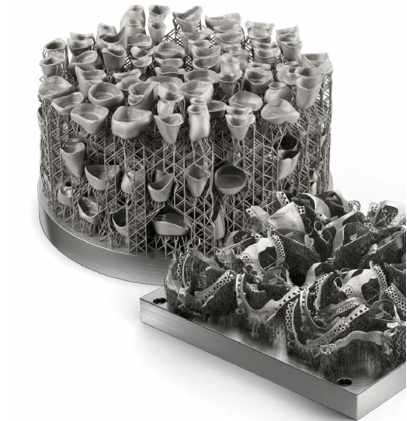
Fig. 3 Packing as many parts as possible into the metal AM machine helps increase volume and reduce costs. AI can provide optimised 2D and 3D nesting to boost machine output, including interlocking nesting (Courtesy Oqton)
