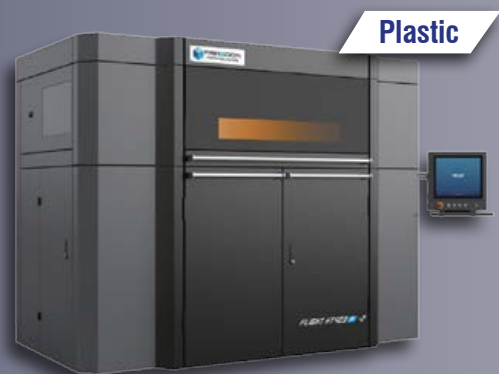
Flight® HT403P-2 2×300W Lasers 400×400×540mm Envelope
