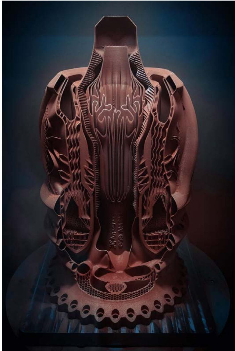
Fig. 11 Aerospike rocket engine with the most complex internal structures – designed using artificial intelligence by Hyperganic, built by AMCM on the AMCM M 4K with integrated Volkmann closed loop powder handling technology (Courtesy of AMCM)
