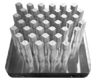
IN-718 fatigue specimens built on AddUp's FormUp 350 Laser Beam Powder Bed Fusion machine (Courtesy AddUp)
