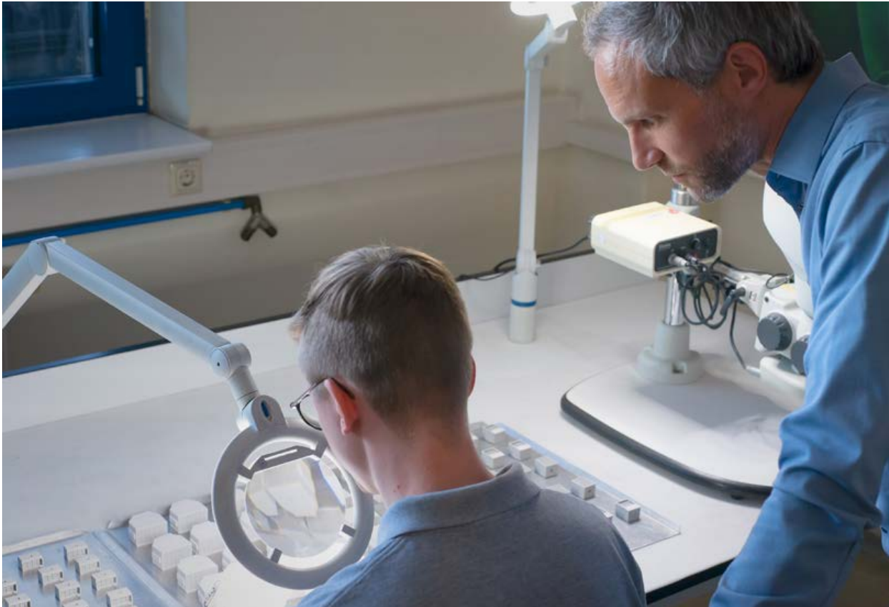
Fig. 7 Quality inspection of binder jetted parts (Courtesy GKN PM)
