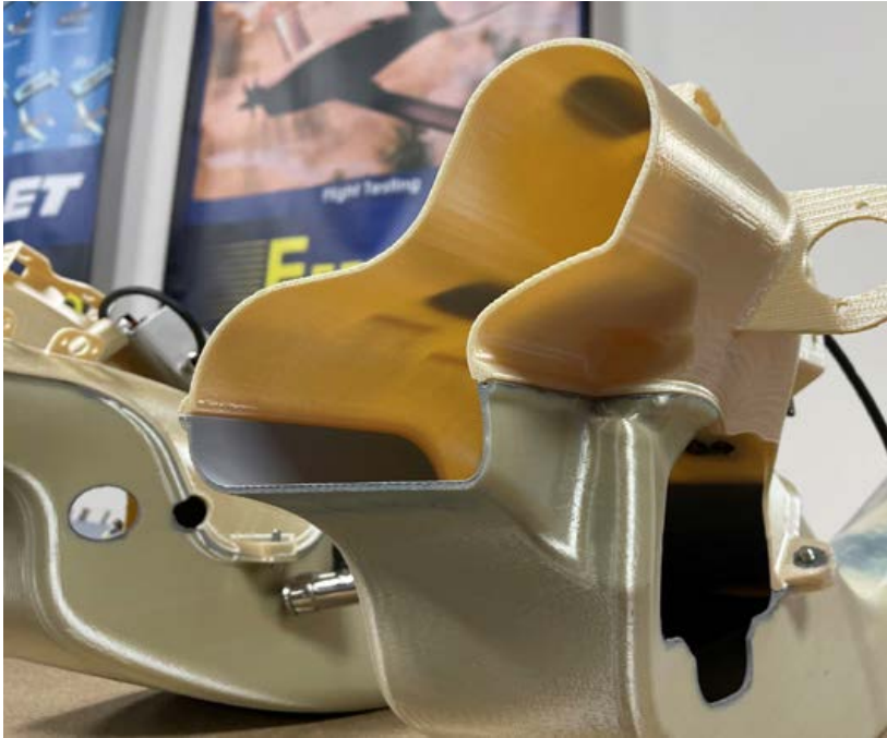
Fig. 2 An AM inlet air duct for a small UAS platform (Courtesy GA-ASI)
