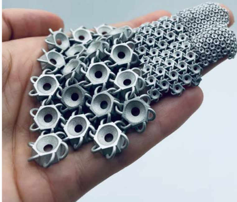
Fig. 3 Additively manufactured steel chain in three sizes, produced by the Vat Photopolymerisation (VPP) process (Courtesy Incus GmbH)
