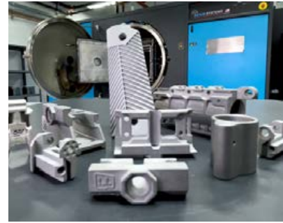
Tekna has collaborated with TriTech Titanium Parts in the successful Binder Jetting of titanium parts using a Desktop Metal P1 Additive Manufacturing machine (Courtesy Desktop Metal)
