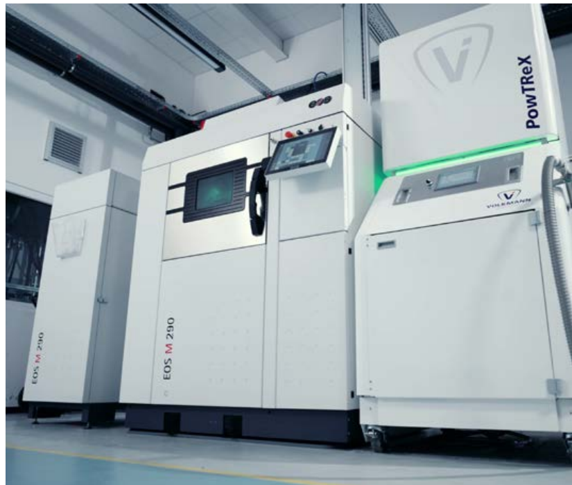
Fig. 3 PowTRex next to an EOS M 290 PBF-LB machine (Courtesy GKN Additive)
