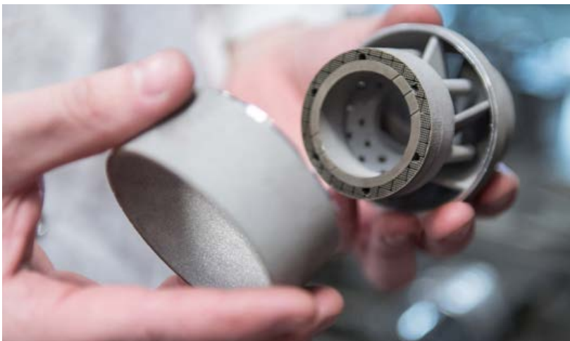
Siemens Energy already uses Additive Manufacturing to produce a number of parts, such as this gas turbine burner (Courtesy Siemens Energy)
