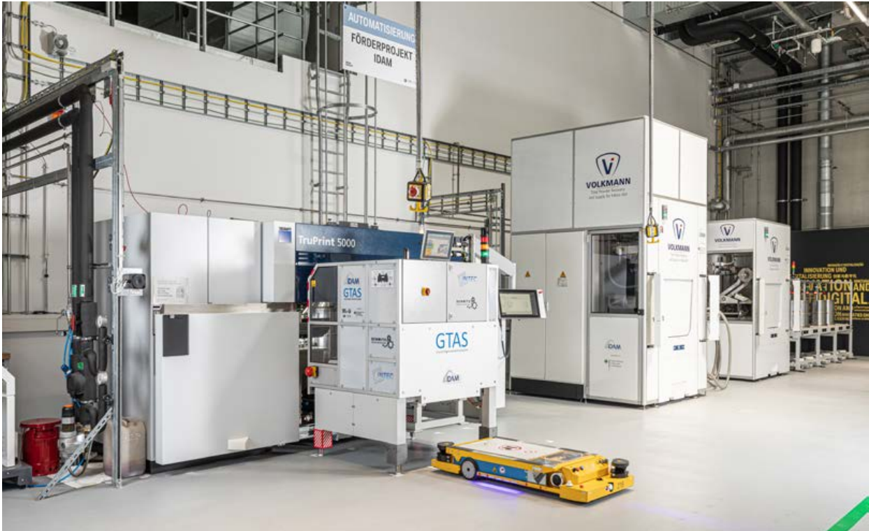
Fig. 5 The IDAM pilot plant at BMW Group. In the IDAM research project, fully automated AM production lines for automotive series production were developed by 12 companies and research institutes under the leadership of the BMW Group and GKN Additive from 2020 until 2022 [1] (Courtesy BMW Group)
