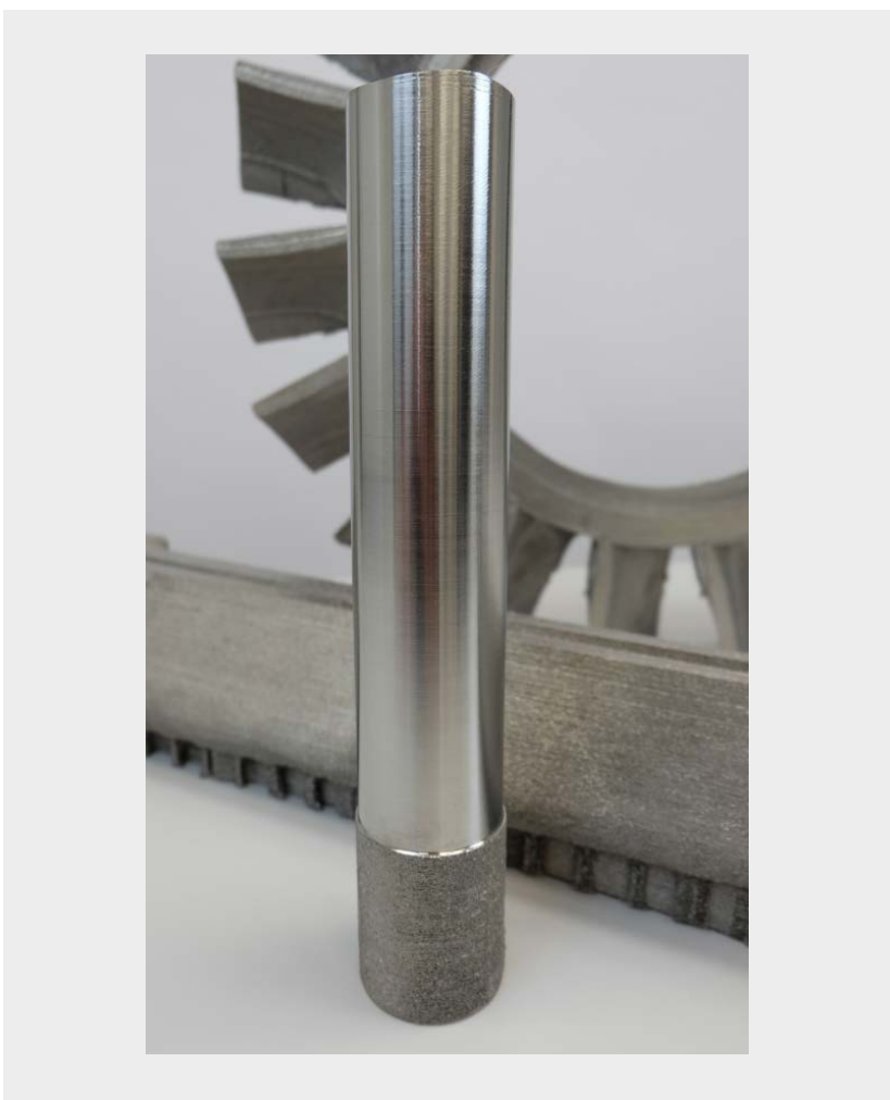
Fig. 8 Specimen (height 300 mm) built with highly-productive process parameters on ALD's EBuild 850. Bottom as-built, and top, machined (Courtesy ALD Vacuum Technologies)
