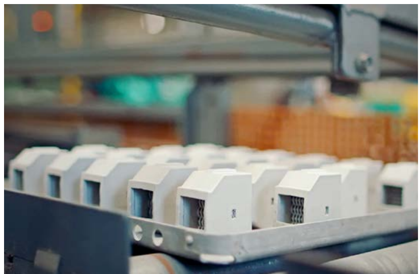
Fig. 1 GKN Additive has produced thousands of filters for Schneider Electric using HP's metal Binder Jetting technology, Metal Jet, with sintering taking place in high-capacity continuous furnaces (Courtesy GKN PM)
