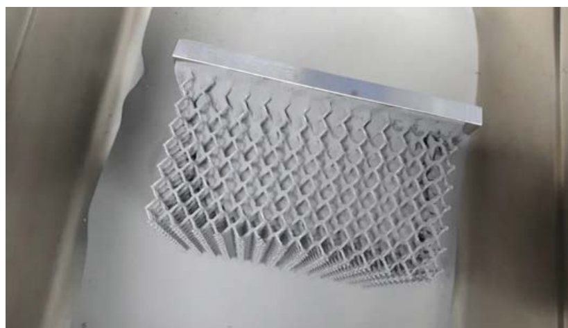
Fig. 6 Active charge neutralisation (top) and the sinter-free depowdering of a lattice structure (bottom) [7]
