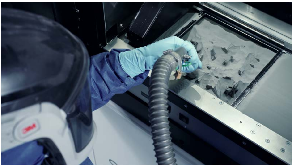
Fig. 2 Protective equipment during manual depowdering (Courtesy GKN Additive)
