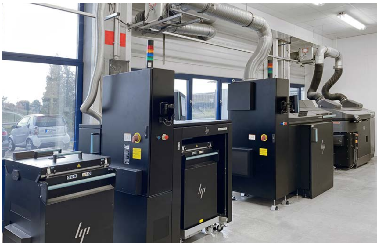
Fig. 2 HP's Metal Jet solution installed at GKN Additive. This image shows, from left to right: build unit, curing station, and printers (Courtesy GKN PM)
