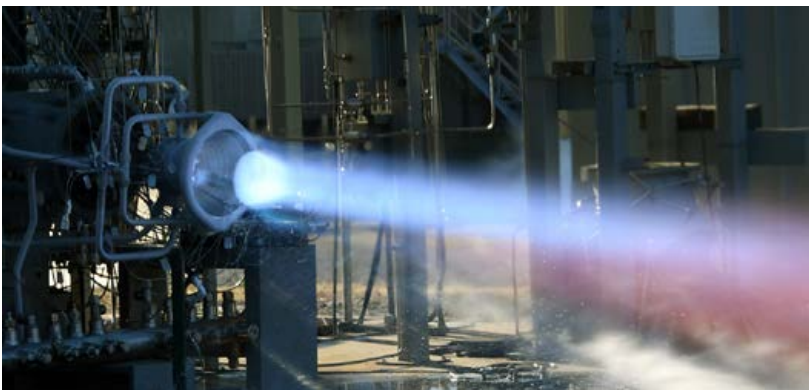
A NASA project called Long Life Additive Manufacturing Assembly is using Additive Manufacturing for building rocket engine component (Courtesy NASA)
