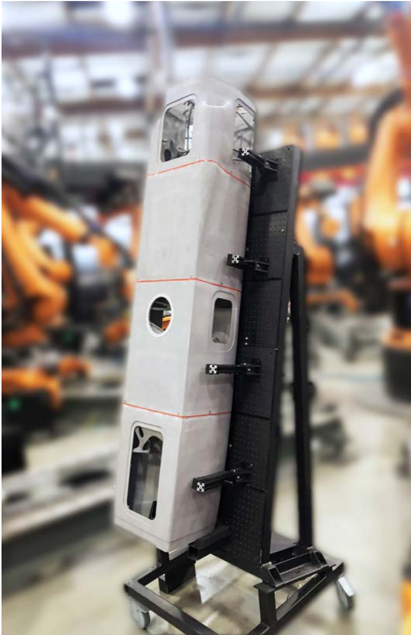
Fig. 7 Robotically assembled small UAS using DAPS technology, without use of custom tooling (Courtesy Divergent)
