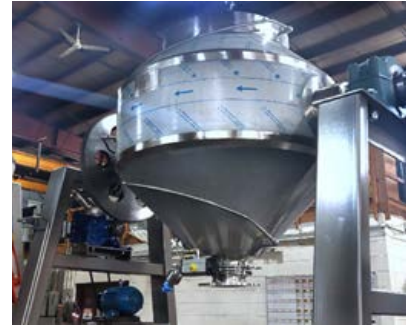
Gemco's mixing and drying equipment designed to process metal and ceramic powders (Courtesy Gemco)
