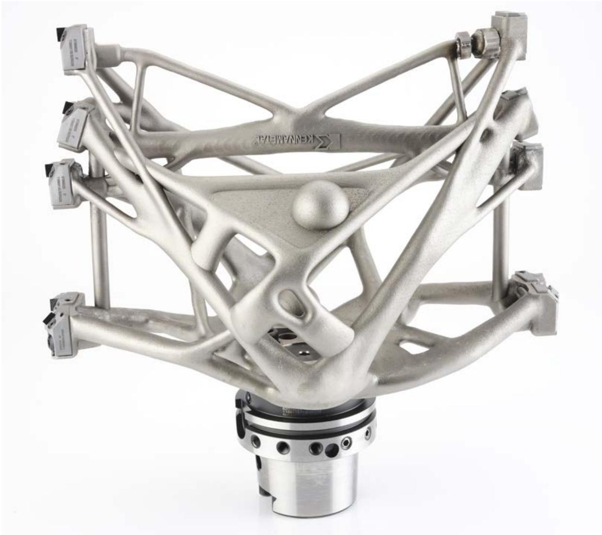
Fig. 15 Light-weighted PBF-LB steel cutter body with coolant channels for transmission housing boring operation (Courtesy Kennametal)
