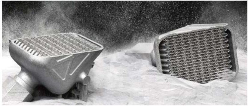
PWR Advanced Cooling Technology will use Constellium's Ahead CP1 aluminium powder to additively manufacture heat exchangers for F1 using Velo3D's Sapphire AM machines (Courtesy PWR Advanced Cooling Technology)
