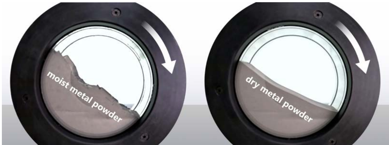
Fig. 7 Laboratory test of flowability of moist and dry stainless steel powder (Courtesy Volkmann GmbH)
