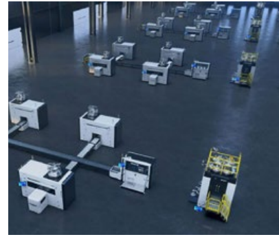
The Binder Jet Line offers scalability as a key advantage, and GE Additive envisages installations of forty to fifty to 100+ machines (Courtesy GE Additive)
