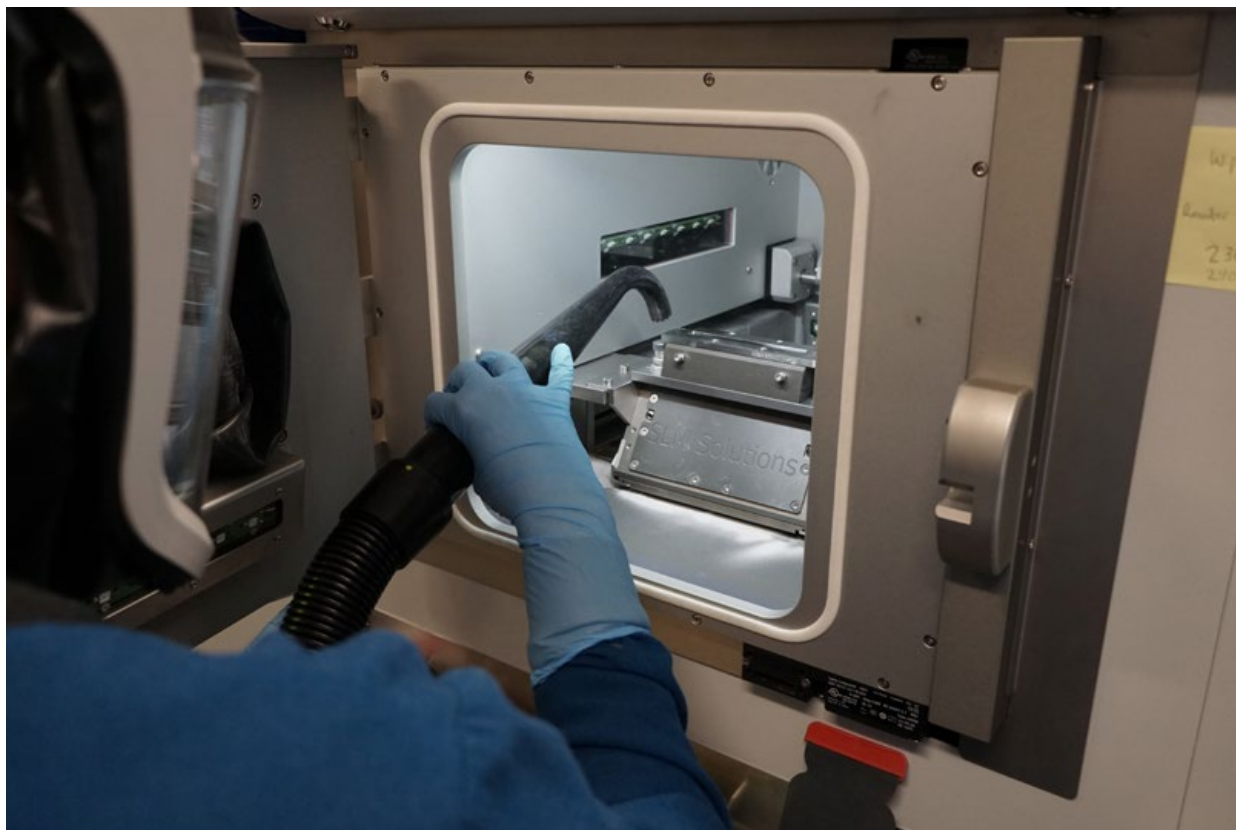
Fig. 4 NanoAL operator cleaning the SLM 125 build chamber after a successful build. The build volume measures 125 x 125 x 125 mm, effectively producing a part with a maximum dimension of 10.2 cm
