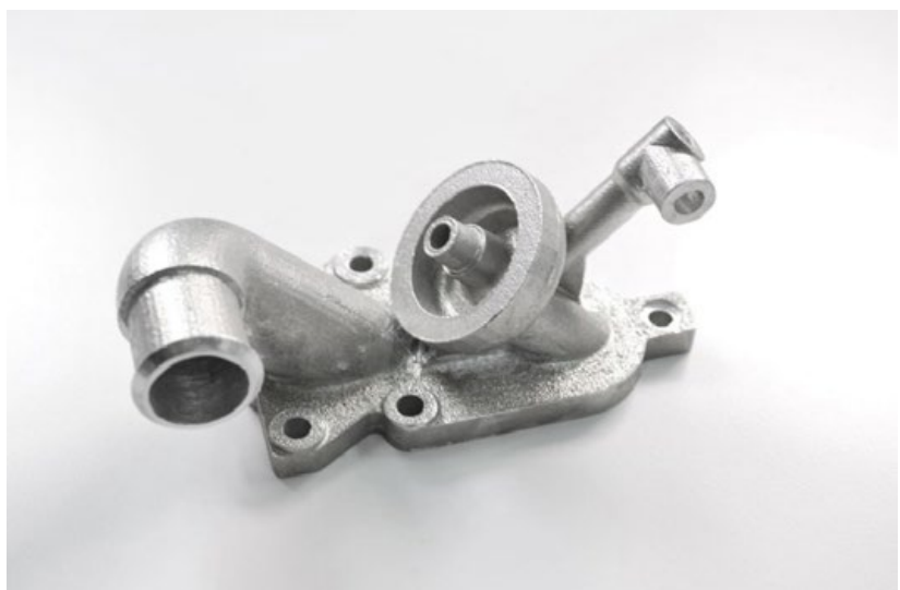
Fig. 1 A demonstration part built with a QuesTek developed high-temperature aluminium alloy for PBF-LB
