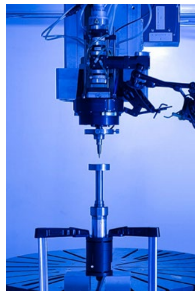
Experimental set-up for ultrasound-assisted laser-directed energy deposition (Courtesy Fraunhofer IWS Dresden)
