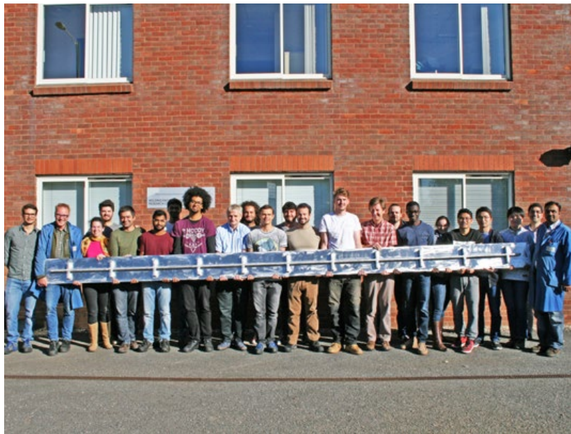
Fig. 8 A 6 m long aluminium spar demonstrator, built at Cranfield University in 2016 on a large prototype WAAM system featuring multiple robots and a 10 m long build envelope (still in use today), in the as-built condition. The part demonstrated distortion control over even larger scales than before, laying the foundations for subsequent multi-metre titanium parts. The picture was taken outside Cranfield University's Welding and Additive Centre
