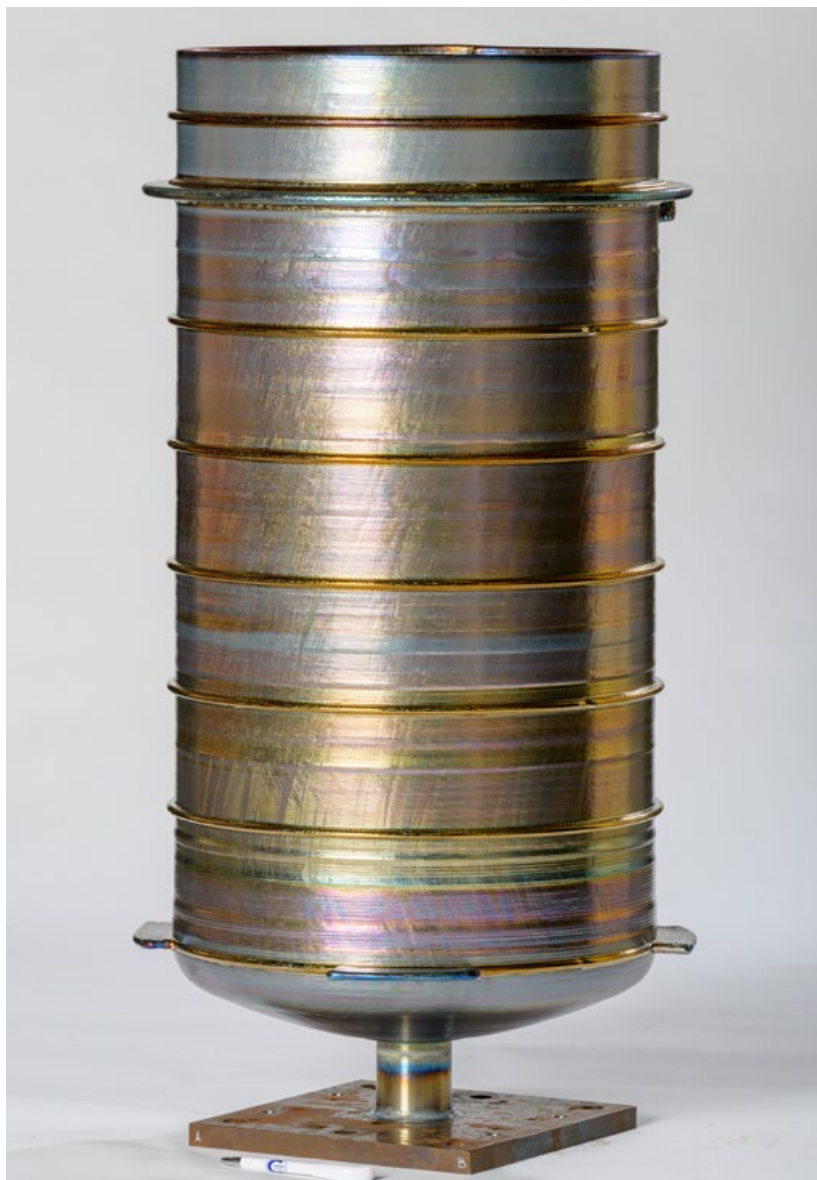
Fig. 11 A 1 m tall Ti-6Al-4V pressure vessel for space exploration, built in 2017 at Cranfield University for Thales Alenia Space, in the as-built condition. The part delivered 80% material savings, 40% cost savings and potentially 65% lead time savings compared to the previous manufacturing route. Before as well as after machining, the part was CT-scanned and ultrasonically inspected, satisfying all technical and quality requirements (Courtesy Cranfield University and Thales Alenia Space)
