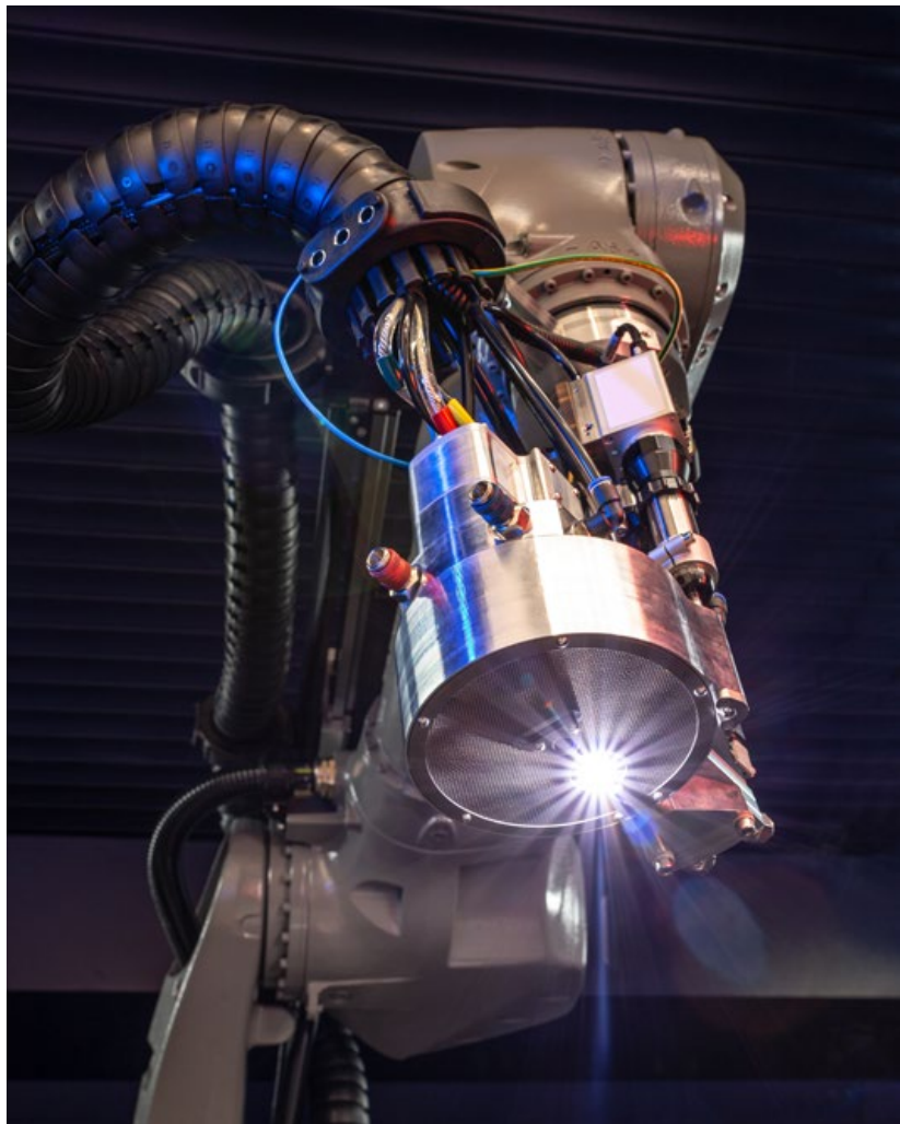
Fig. 5 The Plasma Transferred Arc variant of WAAM3D's End-Effector. It features double wire feeding for increased deposition rates, or multi-material deposition; a closed-loop-based wire positioning system for consistent transfer of metal drops; a leading pyrometer to ensure a consistent deposition-start temperature; a trailing pyrometer to monitor the temperature profile behind the melt pool; a melt pool monitoring camera with video feed sent to the control centre and recorded throughout the building of the part; and finally ShapeTech™, WAAM3D's proprietary sensor to measure layer height and 3D profile in real time; all connected to the WAAMCtrl® software. The variant shown also features a local shielding device for the deposition of reactive metals. WAAM3D has commercialised several End-Effector variants, provided either as part of RoboWAAM, or on their own
