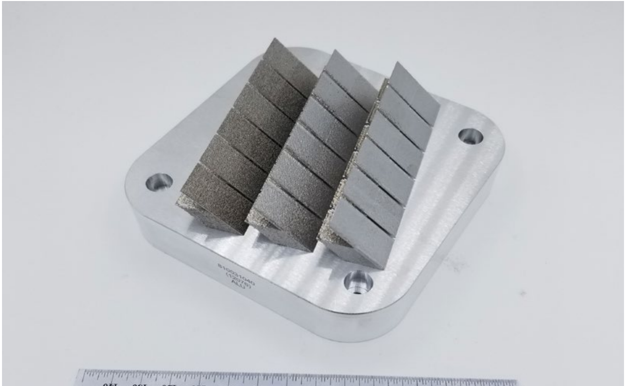
Fig. 10 A design of experiment combining wide cross sections with thin walls, overhanging, upskin, vertical and horizontal surfaces. Each surface is characterised for roughness and each feature is measured for geometric tolerance to feedback into the parameter optimisation cycle
