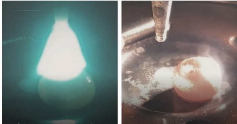
Fig. 5 Arc melting of a button sample at QuesTek's materials lab to characterise and test novel alloy designs
