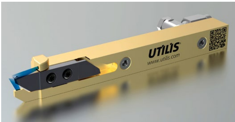
The tool holder includes extremely small cooling channels and is made using the ColdMetalFusion process - a sinter-based AM method that results in parts with properties similar to MIM (Courtesy Headmade Materials)
