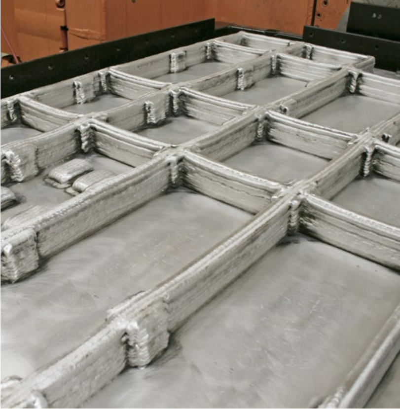
Fig. 6 Close-up of an as-built 2319 satellite breadboard, built at Cranfield University for Thales Alenia Space in 2016, in the as-built conditions. Distortion control for parts of this type was fixed by this time, however geometry control made this component incredibly difficult to make. For aluminium deposition there is little choice outside MIG-based processes, with which it is hard to control material feed and heat input independently. This is a key requirement when dealing with intersections, to achieve the target layer height whilst avoiding lack-of-fusion defects (Courtesy Cranfield University and Thales Alenia Space)
