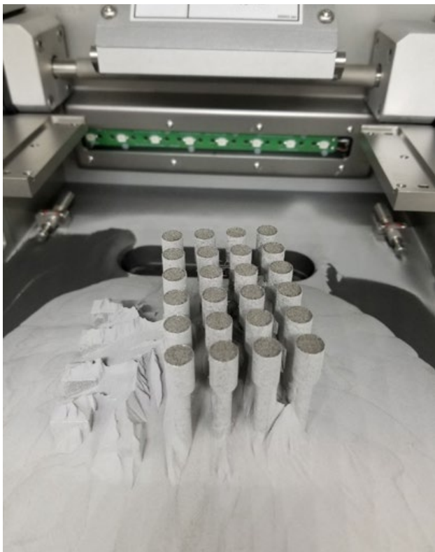
Fig. 9 Net-shape tensile bars built on the SLM 125 at NanoAL. Testing is performed in-house with a Shimadzu frame
