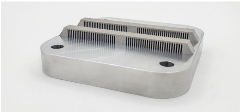
Fig. 11 A cantilever bar build used for residual stress testing and to develop optimal stress relieve treatments for new alloys. Deflection along the bar is measured before and after thermal stress relief tests to determine the effectiveness of the thermal treatment
