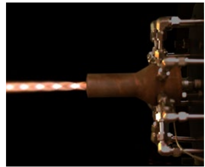
A filtered composite image of the first hot fire test taken using a high-speed camera; 500 frames per second (Courtesy SPEE3D)
