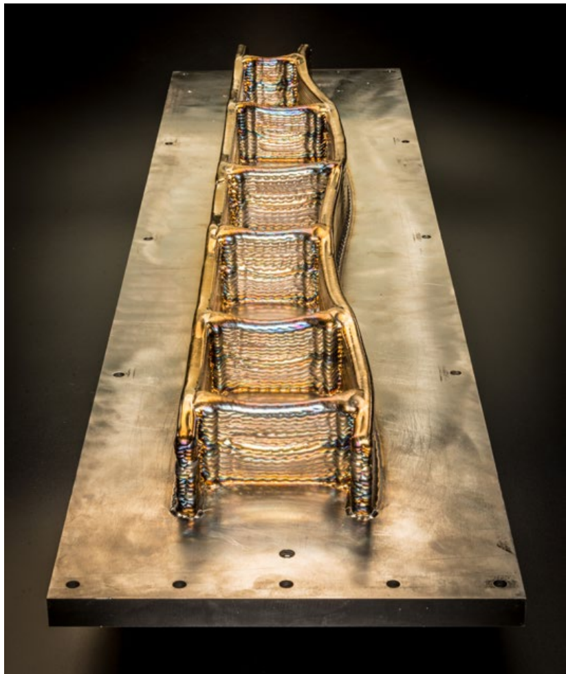
Fig. 3 A 1.2 m long Ti-6Al-4V wing spar demonstrator, built at Cranfield University for BAE Systems in 2012, in the as-built condition. It demonstrated successful control of distortion and the possibility to deposit large components back-to-back, however it also highlighted the requirement for better thermal compensation strategies to control the layer height in critical areas (Courtesy Cranfield University and BAE Systems)
