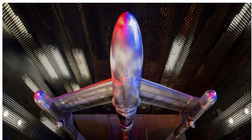
Fig. 1 A 2319 aluminium wind tunnel model featuring a nose cone produced by WAAM3D for the UK's Aircraft Research Association, demonstrating that prototypes can be developed quickly and to defined tolerances using DED-Arc. Material usage was reduced by 74%. Activity funded by a Clean Sky 2 research and innovation programme under GA Agreement 864803 (Courtesy WAAM3D and ARA Ltd)
