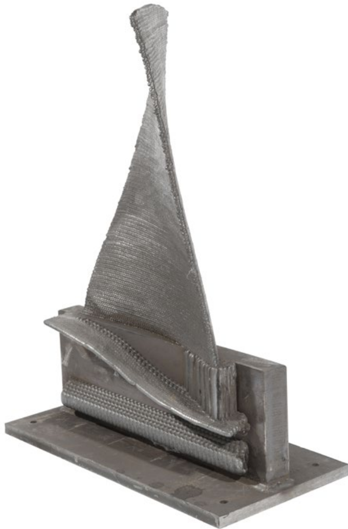
Fig. 10 A 1 m tall steel industrial gas turbine blade, built in 2013 at Cranfield University for GE Power and Water, in the as-built condition. The part was deposited using multi-orientation and multi-hierarchical approaches, in a variety of different alloys (Courtesy Cranfield University and GE Power and Water)
