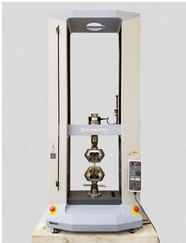
Fig. 9 Net-shape tensile bars built on the SLM 125 at NanoAL. Testing is performed in-house with a Shimadzu frame
