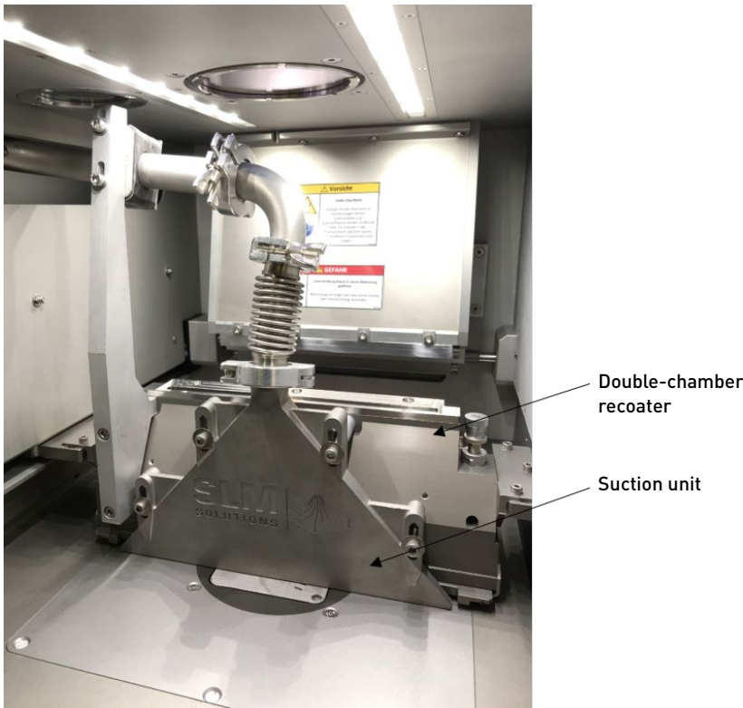
Fig. 5 View inside a multi-material-capable SLM® 280 2.0 machine at Fraunhofer IGCV laboratory Augsburg (Courtesy Fraunhofer IGCV)
