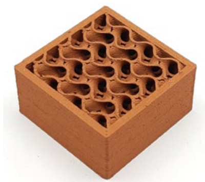
A copper test sample produced at VITO (Courtesy VITO)
