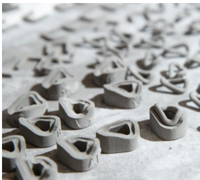
Components built with the HP Metal Jet machine (Courtesy HP)
