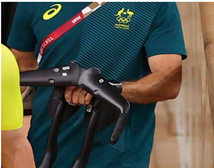
Fig. 8 The broken handlebars, showing the point of failure, being carried off the track in Tokyo (Photo credit Reuters/Kacper Pempel)
