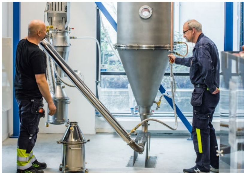
The atomisation unit for the production and development of metal powders (Courtesy Swerim/Kanthal/Anneli Nygård)
