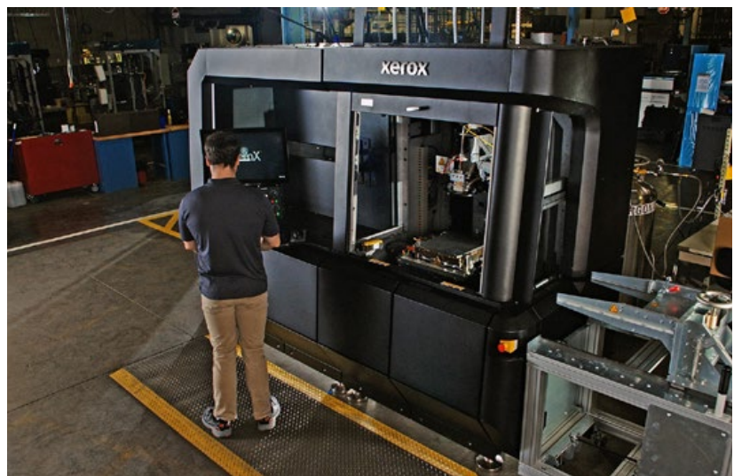
Fig. 1 The ElemX AM machine, capable of >99% dense aluminium parts using wire feedstock (Courtesy Xerox)
