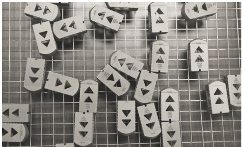
Fig. 1 FDA cleared GAIA lumbar cages manufactured by PrinterPrezz [Courtesy PrinterPrezz]
