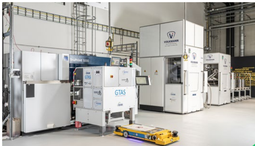
A fully automated Additive Manufacturing production line has been established for automotive part production at the BMW Group Additive Manufacturing Campus (Courtesy BMW Group)
