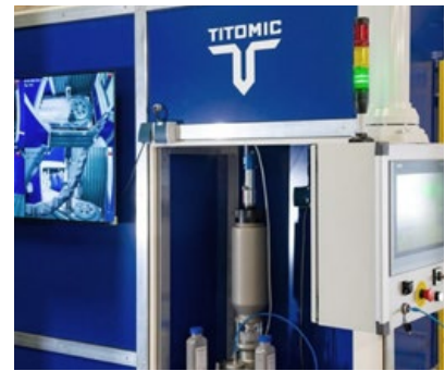
Titomic has developed a system for the coating and repair of glass moulds (Titomic)
