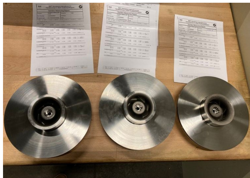
Fig. 1 Finished impellers manufactured by PBF-EB, one of several metal AM technologies evaluated in Phase II (Courtesy Eureka)
