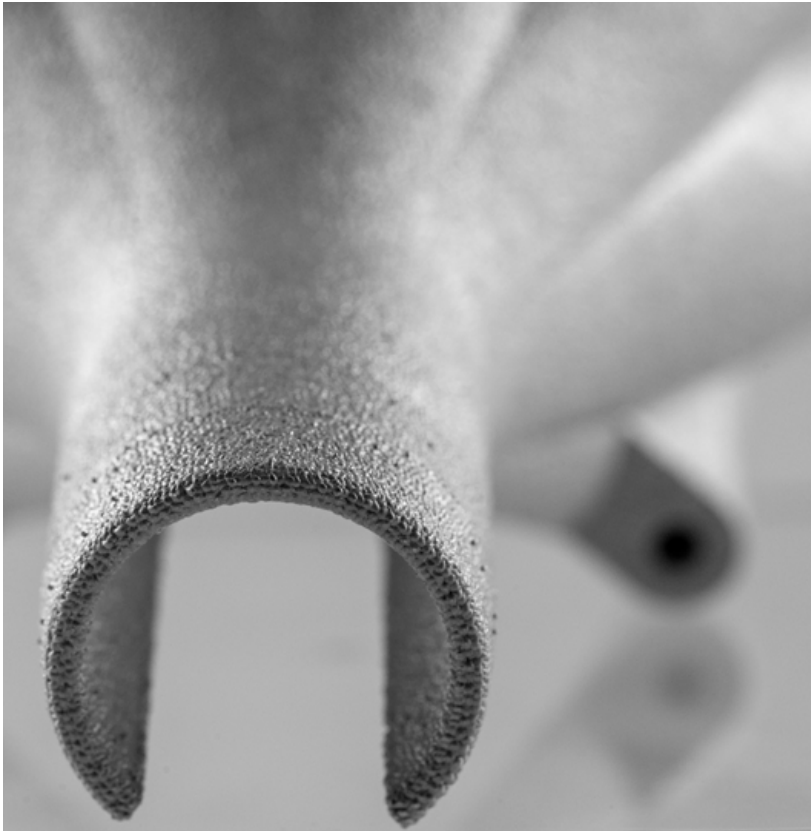
Fig. 10 Detail showing typical as-built surface finish. Droplets are ~240 \mu\text{m} and are jetted at up to 400 droplets per second (Courtesy Xerox)
