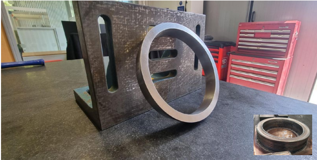
Fig. 2 The completed DED-LB wear ring, with the as-built ring shown inset (Courtesy NMIS and Eifeler - Voestalpine)
