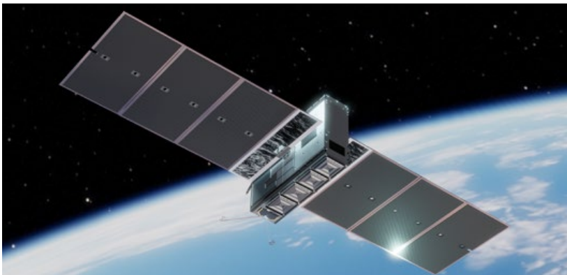
Fleet Space has launched its Centauri 5 satellite which features additively manufactured metal patch antennas (Courtesy Fleet Space Technologies)
