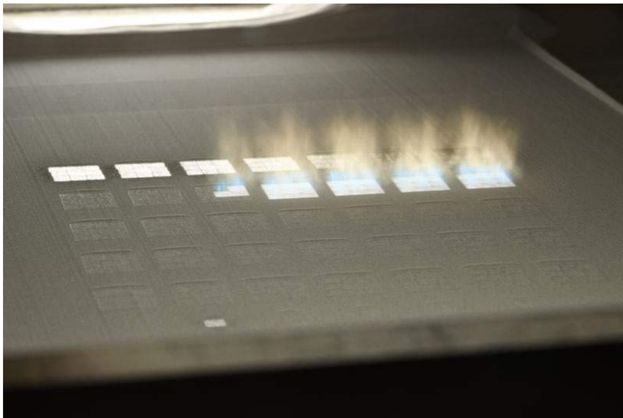
Fig. 4 Area Printing prints one tile next to the other. Over 2.3 million pixels are used to define the shape of each tile achieving a pixel size of 6–10 \mu\text{m} , which exceeds the current xy-resolution of PBF-LB systems by far
