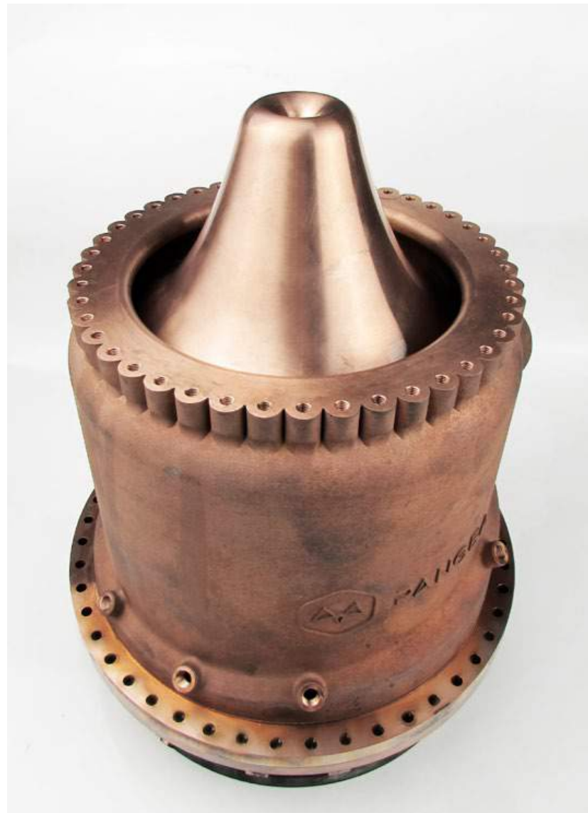
Fig. 4 The DemoP1 is the first additively manufactured aerospike engine in the world to be powered by liquid methane and liquid oxygen (Courtesy Pangea Aerospace)
