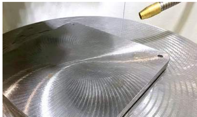
Rotary grinders efficiently remove a range of metal remnants such as aluminium, titanium, and Inconel from the build plates (Courtesy DCM Tech Inc)
