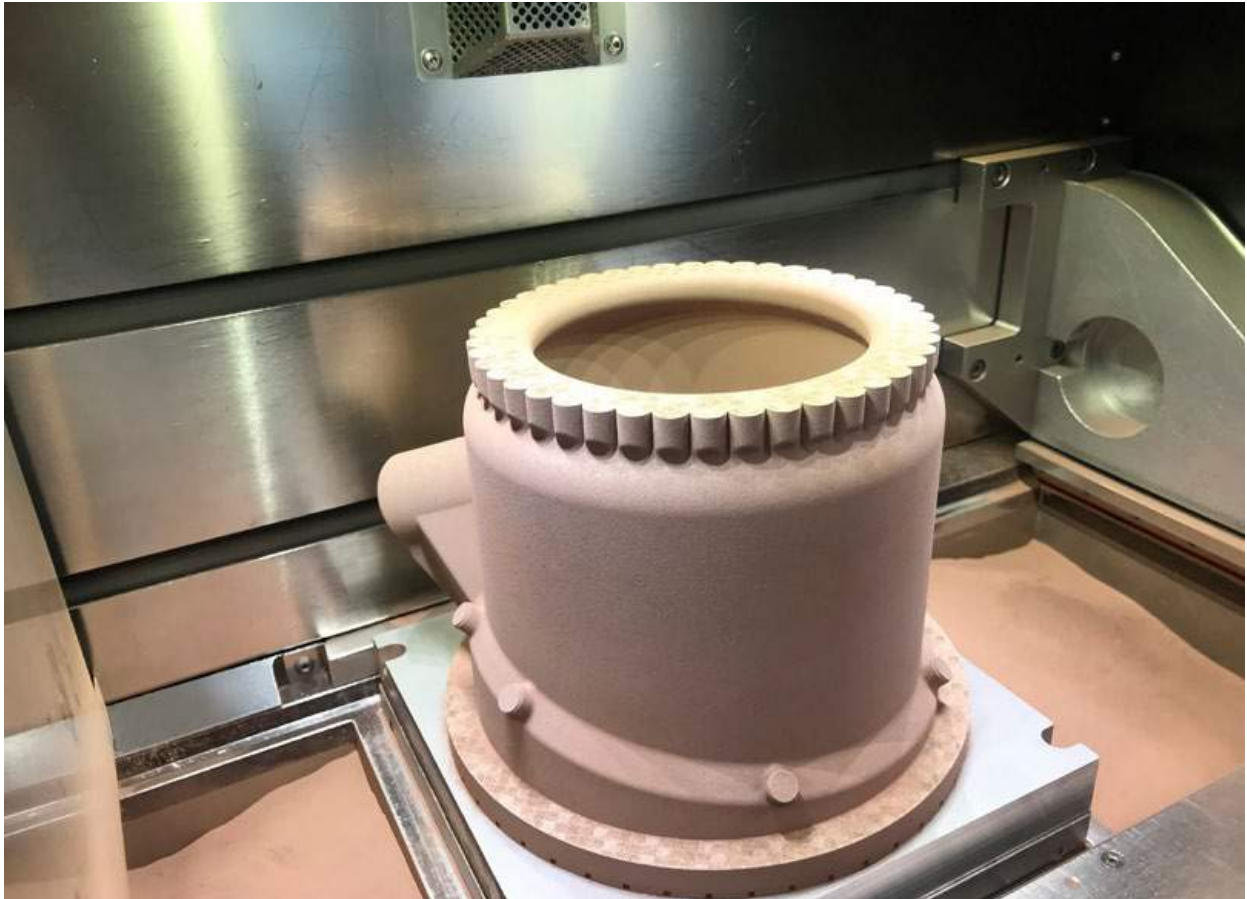
Fig. 6 DemoP1's jacket in the PBF-LB build chamber (Courtesy Aenium Engineering)
