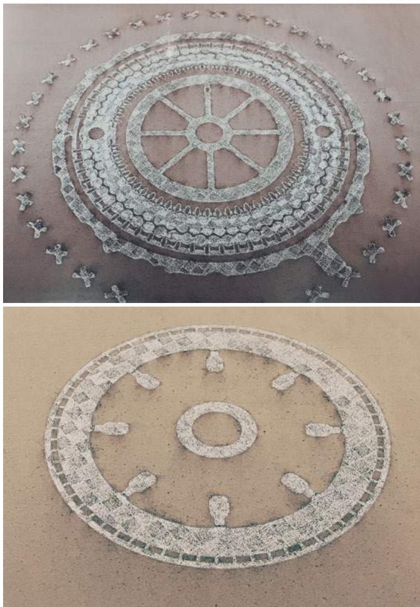
Fig. 9 Build chamber views showing sections of the cooling channels employed in the aerospike engine (Courtesy Aenium Engineering)
