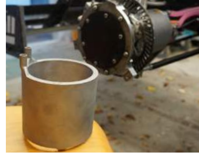
The additively manufactured aluminium cooling jacket was said to have aided the motor of E.Stall Esslingen's racecar to stay below 65°C (Courtesy Eplus3D)
