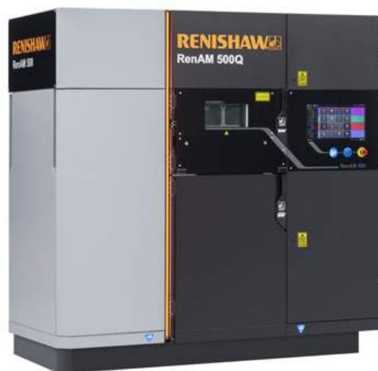
Fig. 1 Renishaw's flagship machine, the RenAM 500Q, with in-situ monitoring of the meltpool at the powder bed (Courtesy Renishaw)
