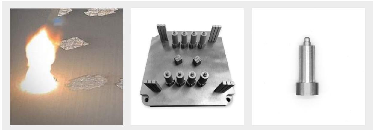
Fig. 9 Left; Area Printing in progress to form one of the steel core pins for an injection mould tool that will be used to manufacture brackets for aerospace and defence customer United Aircraft Technologies. Centre; Eight core pins (four in the front, four in the back) with tensile bars and test cubes also on the build plate. Right; the finished part, a single core pin, built in 316L stainless steel
