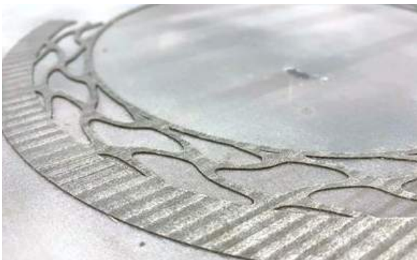
All residual metal left on the build plate between each build requires removal (Courtesy DCM Tech Inc)
