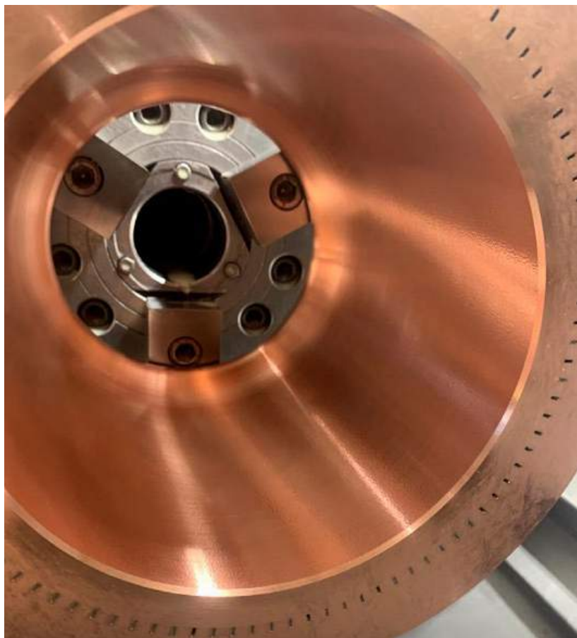
Fig. 5 The machined inner surface of the DemoP1's outer section, or jacket, with cooling channels visible (Courtesy Pangea Aerospace)
