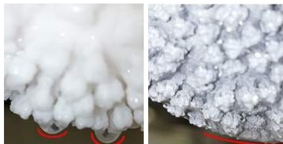
Comparison of water geometry on polymer (left) and metal (right) models (Courtesy MetShape)
