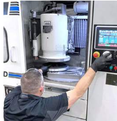
Advanced rotary surface grinders remove unwanted material on the build plate (Courtesy DCM Tech Inc)
