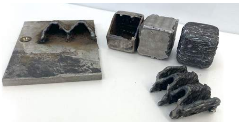
Students from the University of Bordeaux have developed an innovative WAAM process that can offer materials savings (Courtesy University of Bordeaux)
