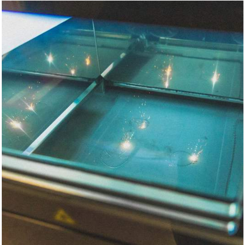
Fig. 3 A build underway in the RenAM 500Q (Courtesy Atherton Bikes/Dan Griffiths)
