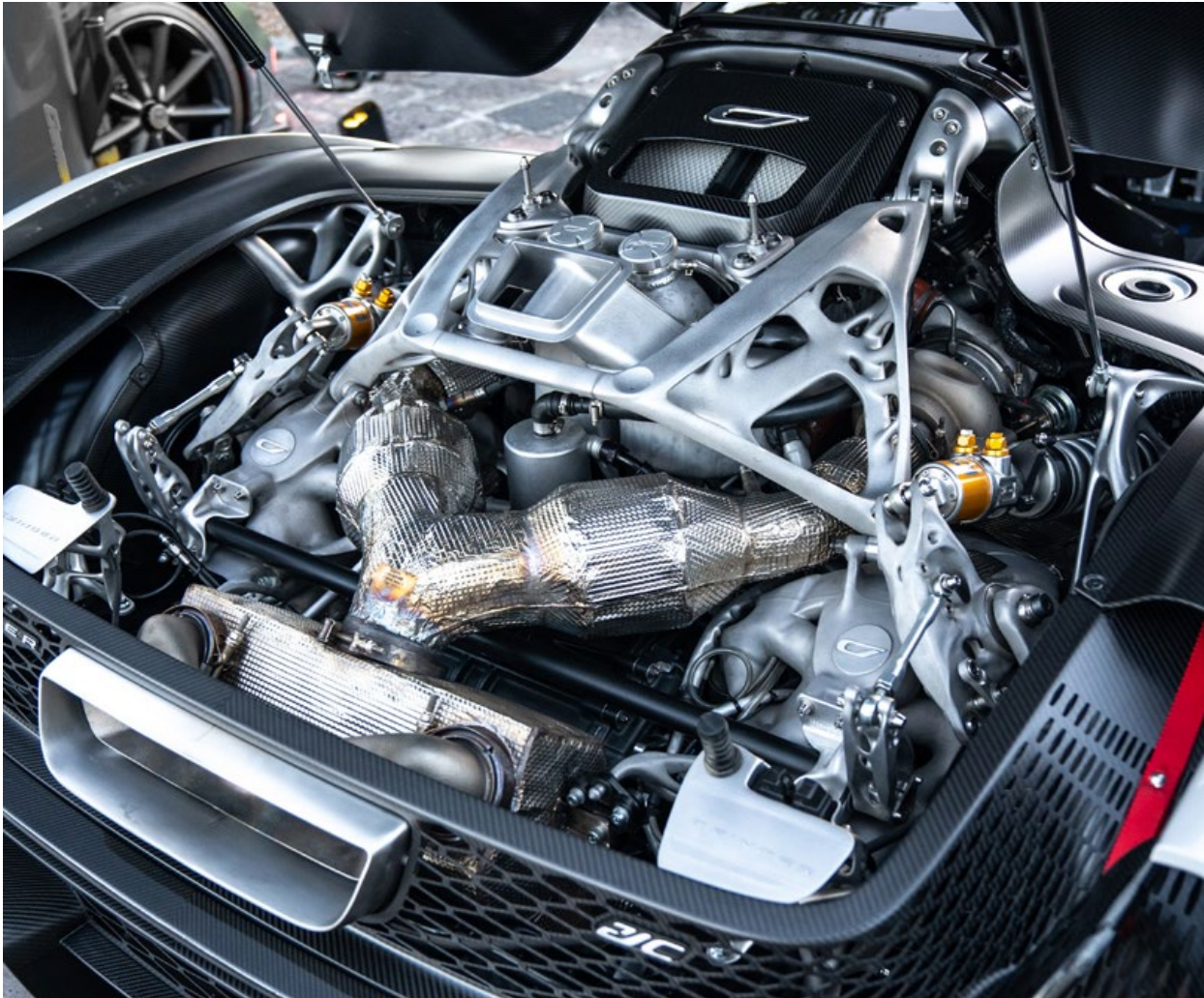
Fig. 2 View inside the engine bay of the Czinger 21C, clearly showing how the potential of metal Additive Manufacturing has been heavily leveraged throughout the car, from the vehicle's chassis to brake, suspension and exhaust components (Courtesy Czinger Vehicles)
