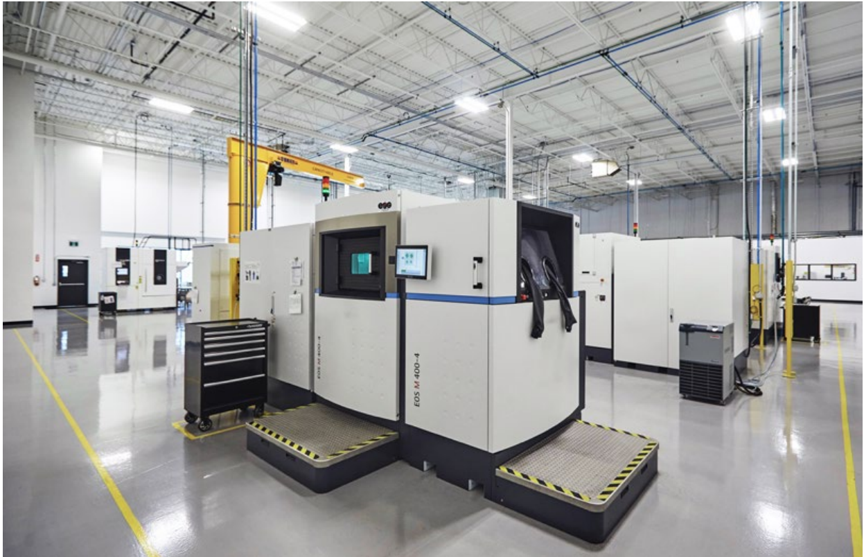
Fig. 3 Whilst larger format PBF-LB machines such as these EOS M 400 4 quad laser machines bring enhanced build speeds, post-processing remains a challenge when looking to scale production (Courtesy Burloak Technologies)
