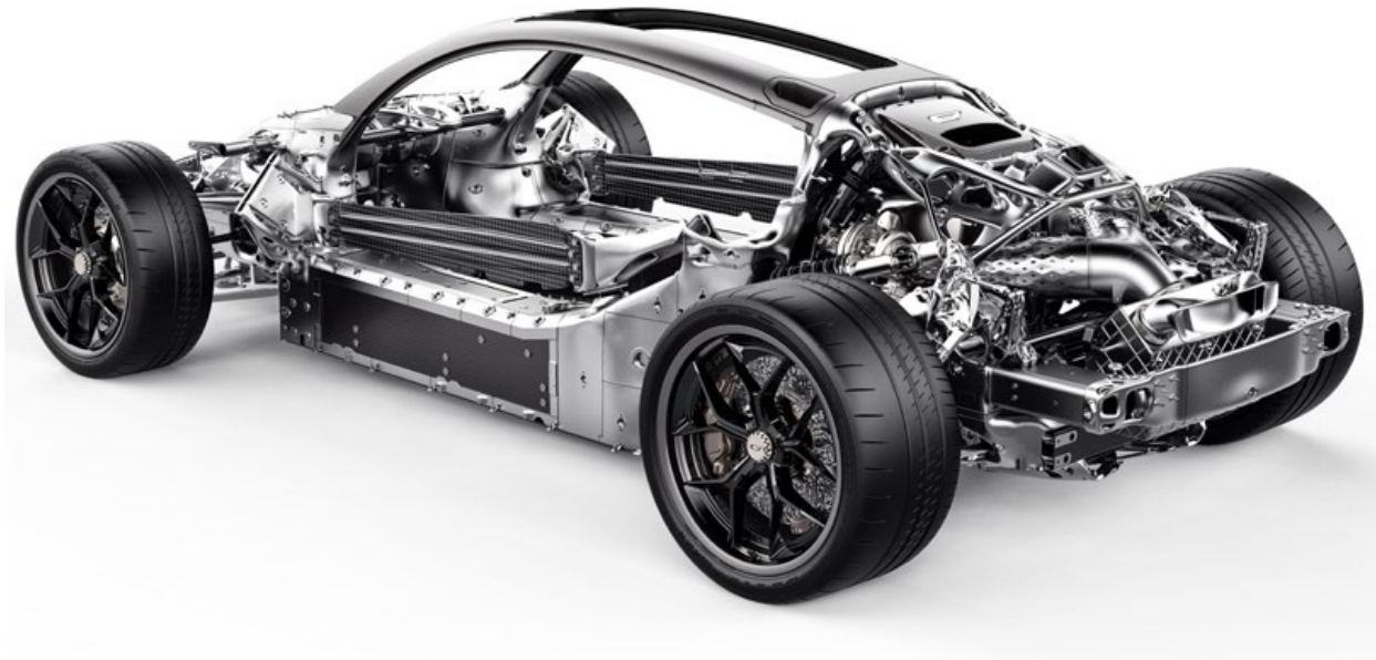
Fig. 3 This render of the Czinger 21C's rear structure shows how a lack of traditional processing and tooling constraints results in an integrated, more organic geometry (Courtesy Czinger Vehicles)
