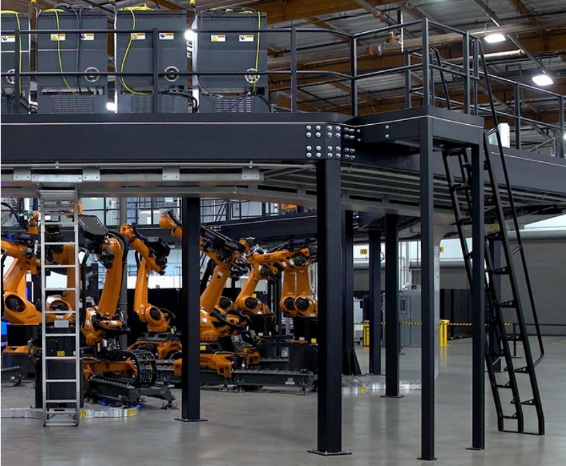
Fig. 11 The Divergent Adaptive Production System (DAPS) is a complete software/hardware solution designed to replace traditional vehicle manufacturing (Courtesy Divergent 3D)
