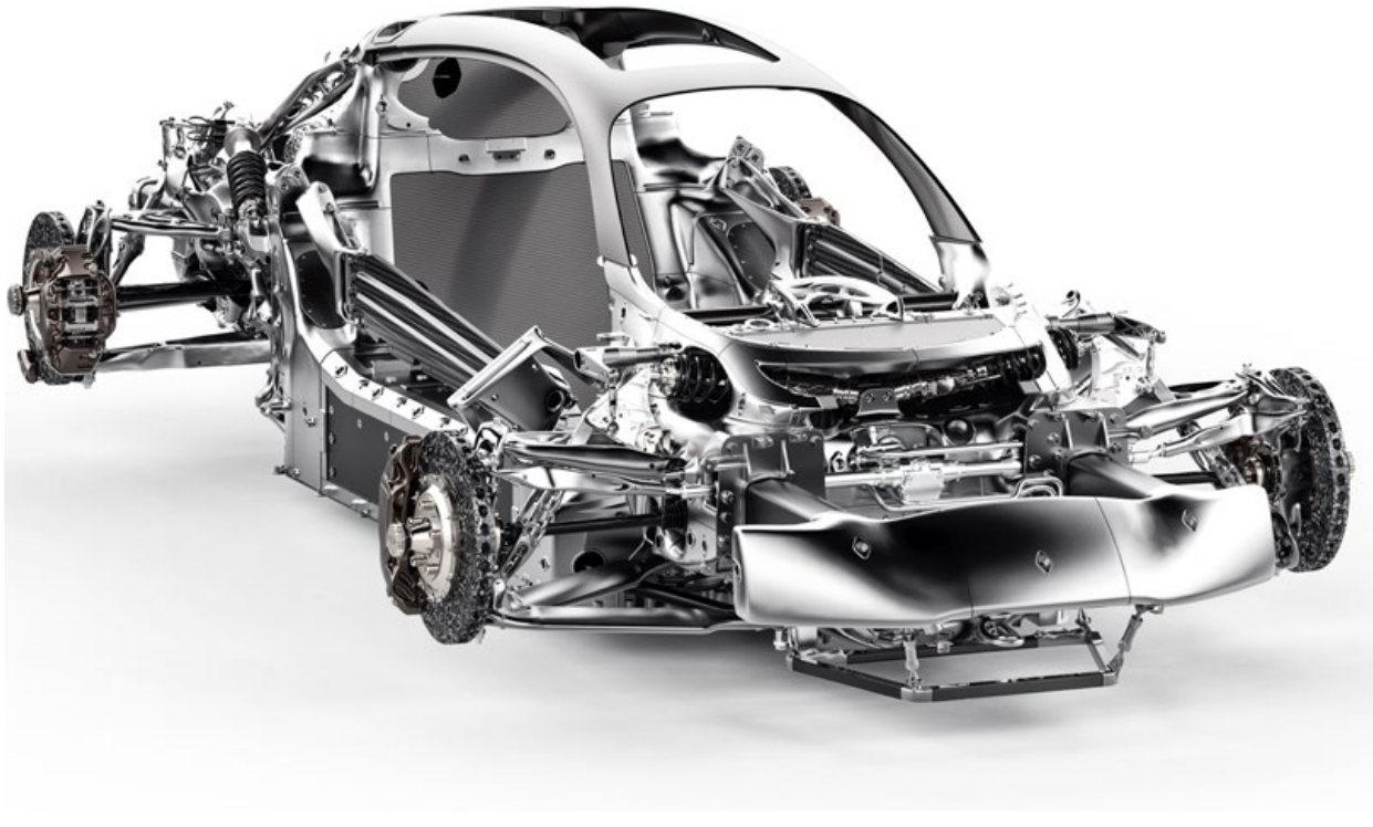
Fig. 10 Render showing the front safety structures, suspension and braking systems, all of which leverage AI to optimise component designs for performance whilst taking advantage of the opportunities presented by AM (Courtesy Czinger Vehicles)
