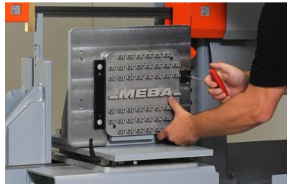
The MEBA3D 335 is equipped with a special clamping device for holding the build plates (Courtesy Meba)
