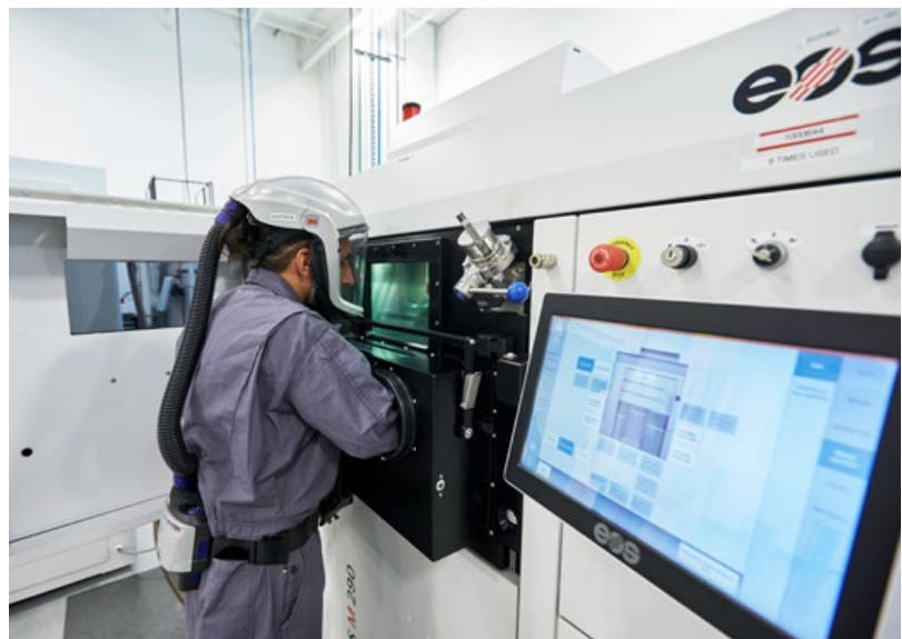
Fig. 1 An EOS M 290 Laser Beam Powder Bed Fusion AM machine post-build (Courtesy Burloak Technologies)
