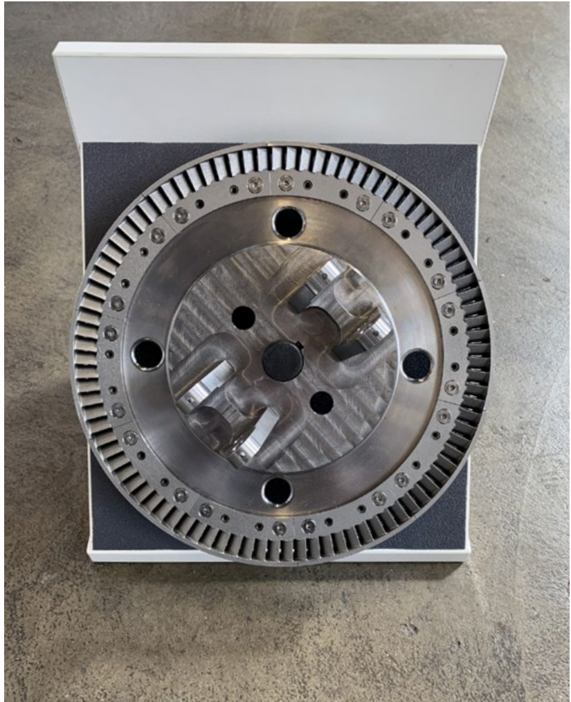
Fig. 2 A turbine paddle wheel for the dynamo machine of a steam locomotive, produced by DED AM (Courtesy Deutsche Bahn)
