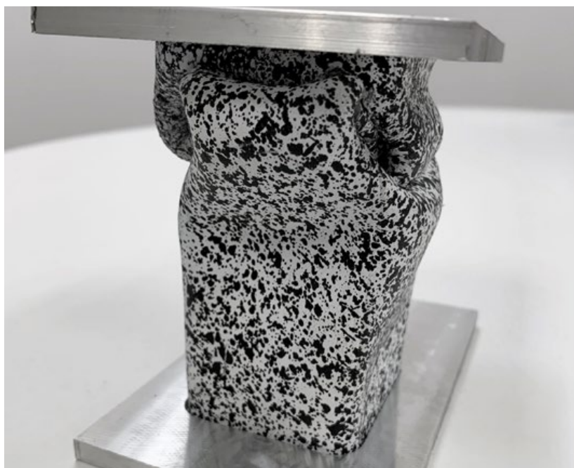
Fig. 9 Trapezoidal crush rails used for performance testing of the custom Divergent Crash Alloy (Courtesy Divergent 3D)
