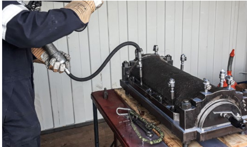
The clamp undergoing radiographic testing (Courtesy Merlin Moritz, MX3D)
