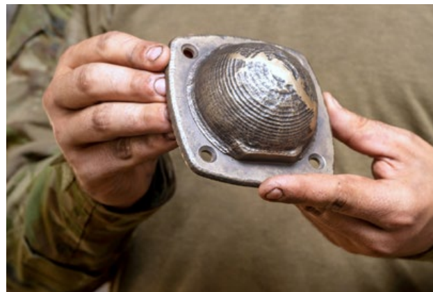
The additively manufactured wheel bearing part took just twenty-nine minutes to build (Courtesy SPEE3D)
