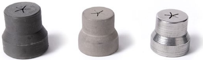
Parts additively manufactured using the Metal Pack on one of BCN3D's Epsilon AM machines, showing as built part (left), sintered part (centre) and post-processed part (right) [Courtesy BCN3D]
