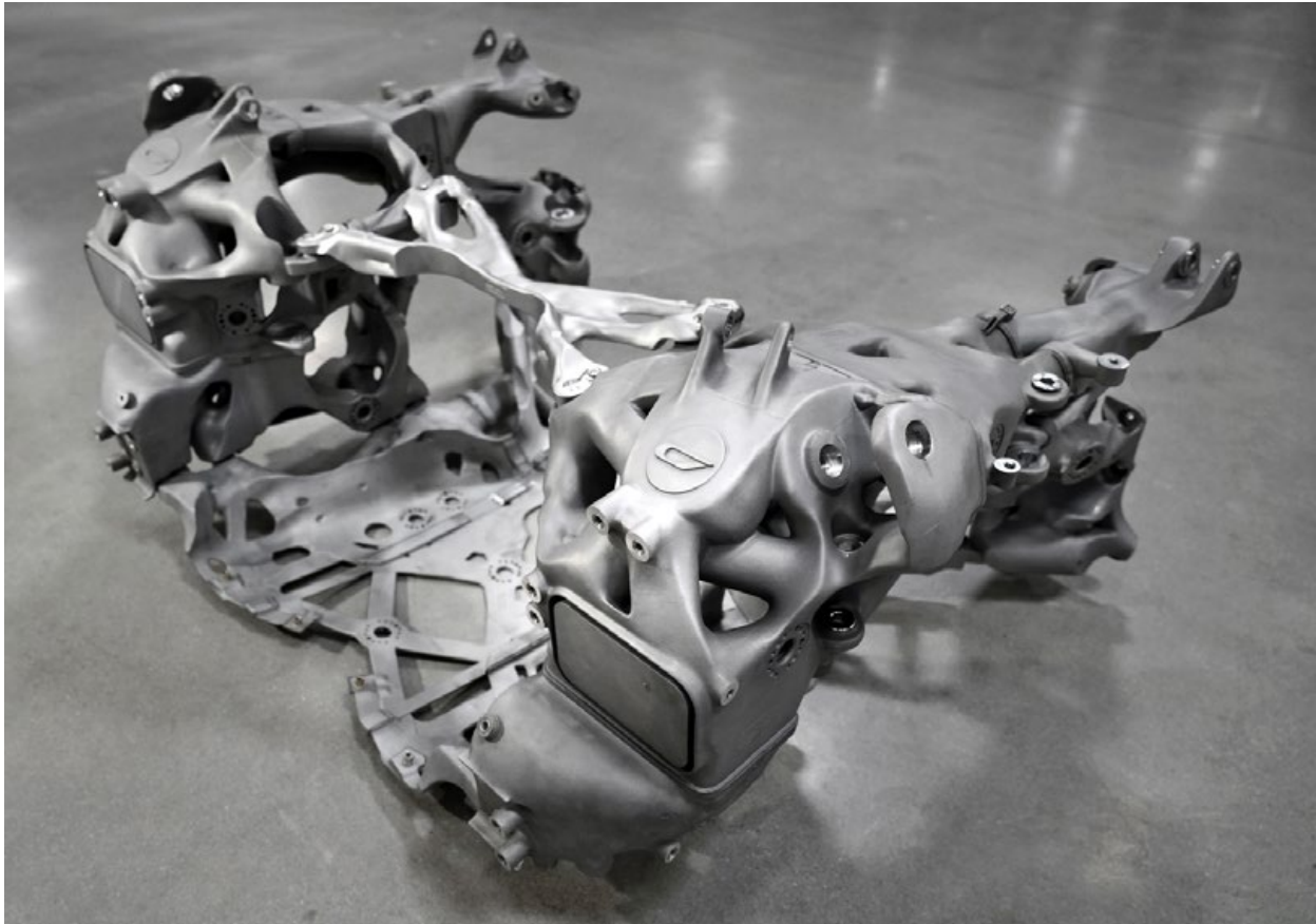
Fig. 12 The assembled rear structure, showing the extent to which metal Additive Manufacturing has been used on the 21C (Courtesy Czinger Vehicles)
