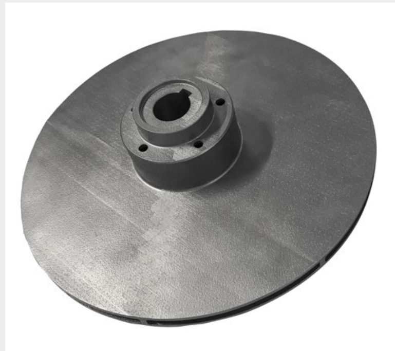
An additively manufactured 316L stainless steel impeller for a pump used in mining equipment, produced using Laser Beam Powder Bed Fusion (PBF-LB) (Courtesy Ivaldi)
