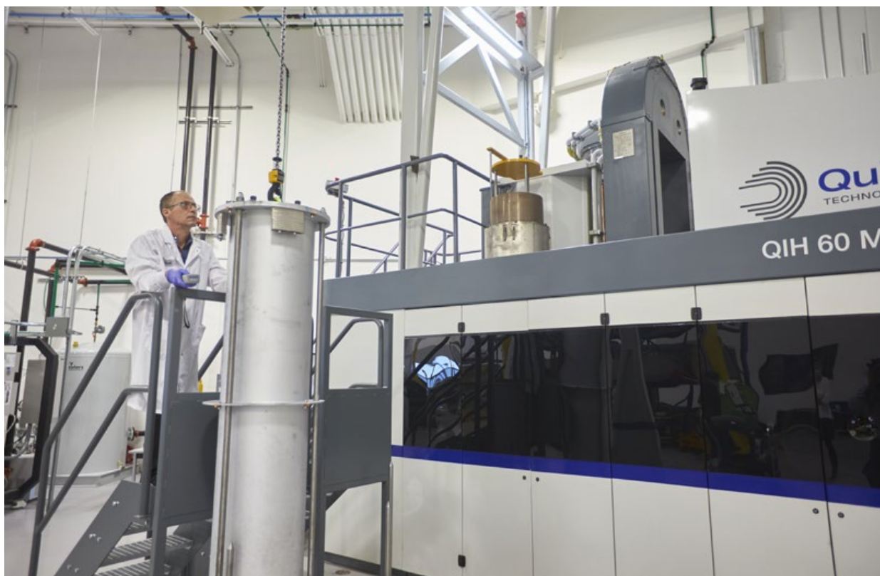
Fig. 7 Hot Isostatic Pressing technology is used as a final processing step for some metal AM applications to eliminate residual porosity or optimise microstructures (Courtesy Burloak Technologies)
