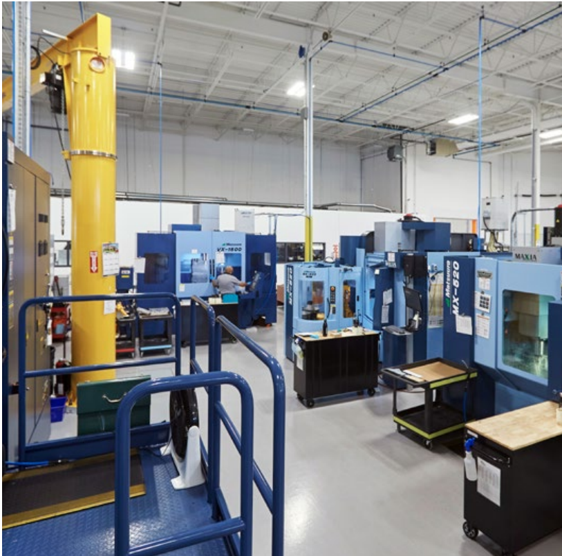
Fig. 5 A bay of CNC machines for the post-processing of AM parts (Courtesy Burloak Technologies)
