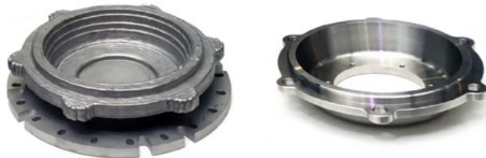
Fig. 3 An additively manufactured wheel-set bearing cover for a Class 294 locomotive, produced on a Gefertec arc605 DED system (Courtesy Deutsche Bahn)
