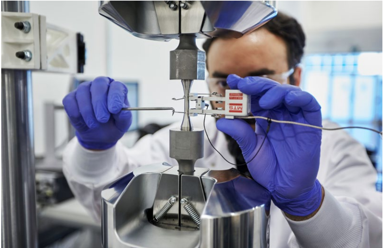
Fig. 4 Tensile testing of built samples. Conducting high volumes of testing simply isn't feasible at a larger scale, so quality plans need to be put in place to streamline the process (Courtesy Burloak Technologies)
