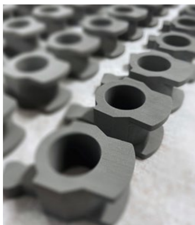
Control Finger for automotive gear boxes, binder jetted with DM 4140 and shown here in a green state (Courtesy Digital Metal)
