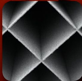
Finest tungsten wall structure 100 \mu m thickness
