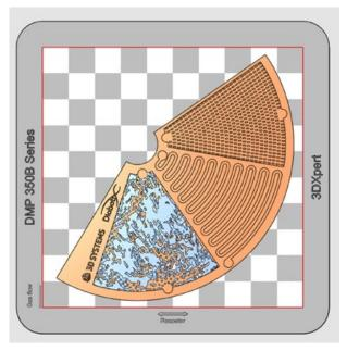
Fig. 14 Cooling strategy demonstrator prepared with 3DXpert (Courtesy 3D Systems)
