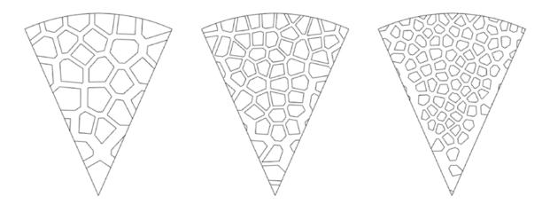
Fig. 5 Parametric line work model of a best first guess Voronoi structure and its limitations in parametric variations (Courtesy 3D Systems)
