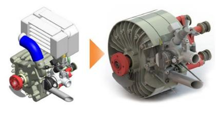
Original rotary engine (left) post-project engine (right) (Courtesy DRAMA/AIE)
