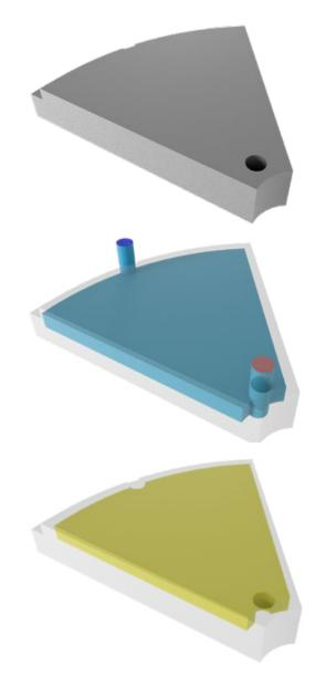
Fig. 8 Top: solid part; middle: fluid region; bottom: design region (Courtesy Diabatix)
