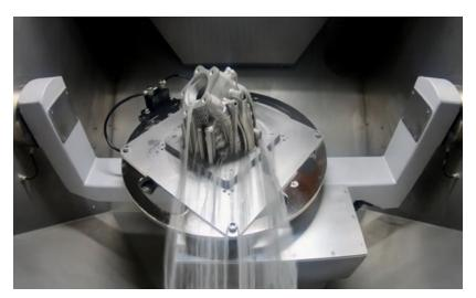
Solukon's depowdering systems incorporate its Smart Powder Recuperation technology (Courtesy Solukon Maschinenbau GmbH)
