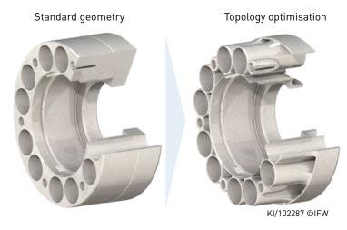
The spring disk component in original condition (left) and after topology optimisation (right) (Courtesy IFW)
