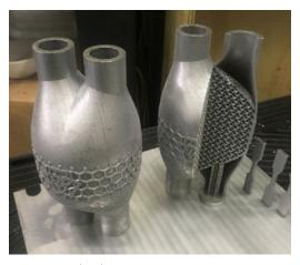
Fig. 6 Section view of completed heat exchanger, including hot and cold fluid zones (left), and the printed part showing minimal support material requirements (right).
