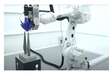
The Meltio system can be integrated into a robotic arm as a cost-effective solution for large metal part manufacturing (Courtesy Meltio)
