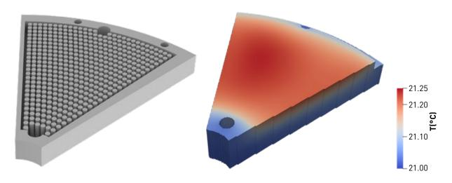
Fig. 10 Left; pin-fin design reference, right; heat map for pin-fin strategy (Courtesy Diabatix)
