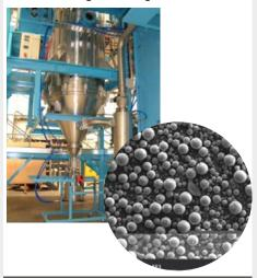
HERMIGA - Vacuum Inert Gas Atomiser (VIGA) supplied by PSI Ltd www.psiltd.co.uk
