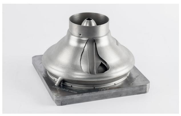
Fig. 4 An aerospace part produced by EOS using state-of-the-art NextGenAM processes (Courtesy EOS)
