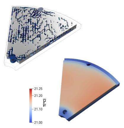
Fig. 12 Top: generative result reference; middle: close up of generative result; bottom; heat map for generative strategy (Courtesy Diabatix)
