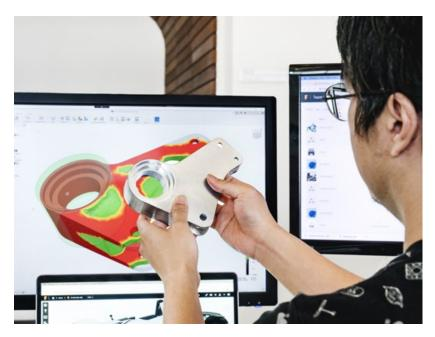
Fig. 5 A mechanical engineer checking his part against FEA data in Autodesk Fusion 360 (Courtesy Autodesk)
