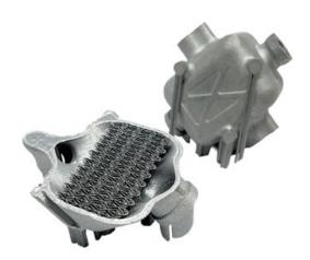
Two views of additively manufactured Aluminium F357 heat exchangers. Note the ultra-thin features in the core (cross-section image at left). The AM process for using Aluminium F357 in Velo3D's Sapphire AM machine was developed jointly with PWR, a global supplier of advanced cooling solutions to Formula 1, NASCAR, other motor racing series, and the automotive, military and aerospace industries (Courtesy Velo3D)
