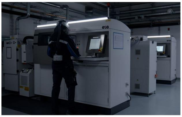
Fig. 3 An operator uses an EOS metal Additive Manufacturing machine in a Materialise production facility (Courtesy Materialise)
