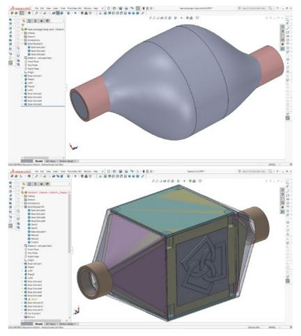
Fig. 2 Basic CAD bodies of one side of a heat exchanger (top), and basic bodies for a radiator showing ten separate bodies that form the radiator subcomponents (bottom)
