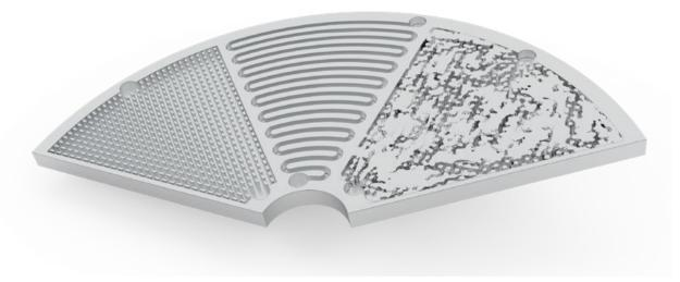
Fig. 9 Three possible cooling strategies presented as  $45^{\circ}$  sections of a design in order to compare performance (Courtesy 3D Systems)
