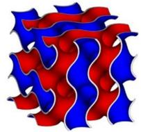
Fig. 1 Single gyroid cell (left) and network of connected gyroid cells (right). The red (hot) zone is kept separate from the blue (cold) zone
