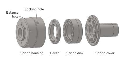
The four clamping system components to be optimised (Courtesy IFW)
