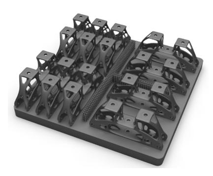
Fig. 7 A tray of parts with segmentation walls to separate parts that require different post processes (Courtesy Siemens)
