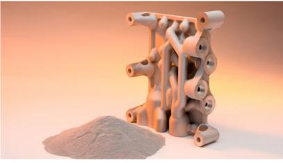
AMT has secured aerospace recognition with the publication of AMS7033 standard for its A20X aluminium powder (Courtesy AMT)
