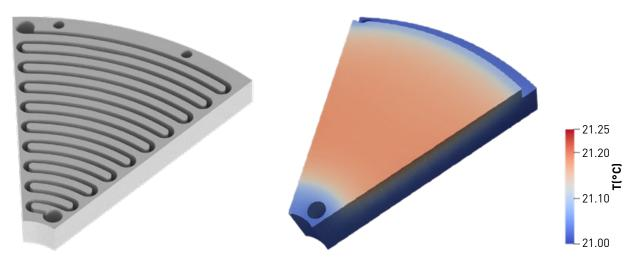
Fig. 11 Left; serpentine design reference, right; heat map for serpentine strategy (Courtesy Diabatix)
