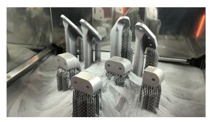
The first build of test cases for HAP, showing forward and aft service handles (Courtesy HAP)
