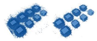
Spatter formation using argon gas only (left image) versus spatter formation using novel argon-helium gas mixture (right image) (Courtesy Linde)
