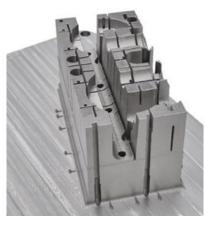
Erofio Group's mould core, which represents the first part manufactured in the company's trialling of the Concept Laser M Line (Courtesy Erofio Group)
