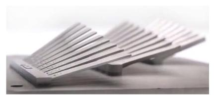
Free Float is said to enable the Additive Manufacturing of overhangs at 10° in long range geometry and 5° in short range (Courtesy SLM Solutions)
