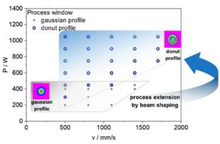
nLIGHT AFX-1000 with switchable donut profiles offers potential for widening and smoothing the melt pool and expanding the process window (Courtesy nLIGHT/Optoprim/TUM)
