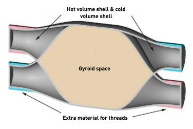
Fig. 3 Creation of various heat exchanger bodies
