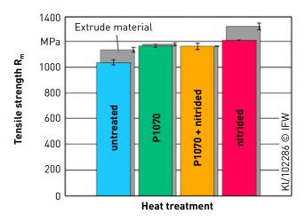
Tensile strengths of 1.4542 in different treatment states (Courtesy IFW)
