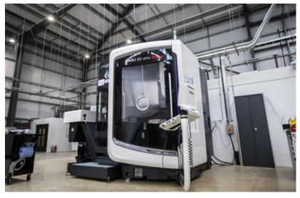
Fig. 5 A DMG Mori 5-axis CNC machine at the DMC (Courtesy DMC)
