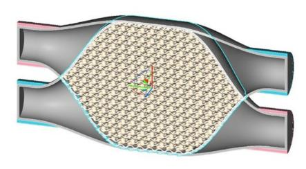
Fig. 4 Creation of gyroid with a cell size and wall thickness to meet specified heat transfer characteristics (left) with a cross section of the TPMS (right).
