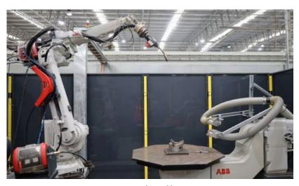
AML3D's Wire Additive Manufacturing (WAM®) process, seen here in an ARCEMY Production Cell (Courtesy AML3D Limited)
