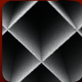
Finest tungsten wall structure 100 \mu m thickness
