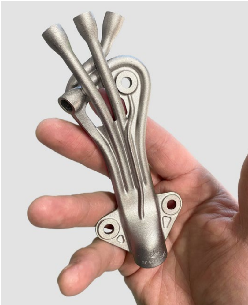
Fig. 2 An additively manufactured hydraulic manifold produced on 3D Systems' DMP 350 platform (Courtesy 3D Systems)
