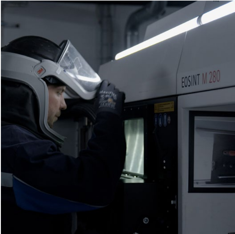
Fig. 4 An operator observes the build process on an EOSINT M 280 machine at Materialise's production facility (Courtesy Materialise)
