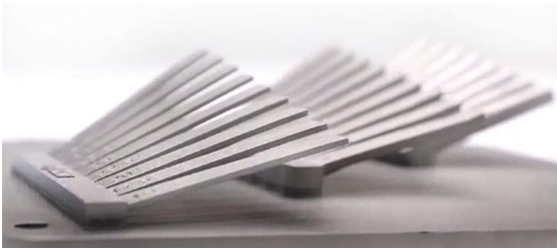
Free Float is said to enable the Additive Manufacturing of overhangs at 10° in long range geometry and 5° in short range (Courtesy SLM Solutions)
