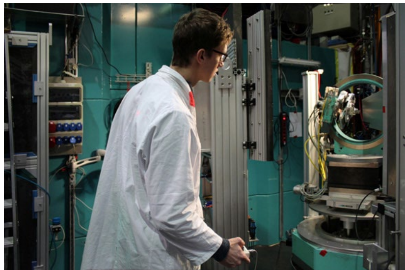
Using the remote control Dr Tobias Fritsch brings the lattice structure into the correct measuring position in the residual stress diffractometer STRESS-SPEC at the research neutron source (Courtesy Dr Michael Hofmann / TUM)
