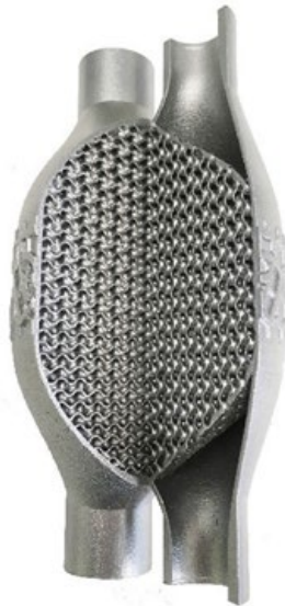
Fig. 7 Additively manufactured heat exchanger section (left) and assembly for testing (right)
