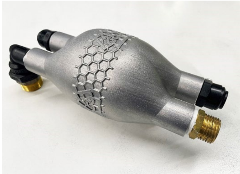
Fig. 7 Additively manufactured heat exchanger section (left) and assembly for testing (right)
