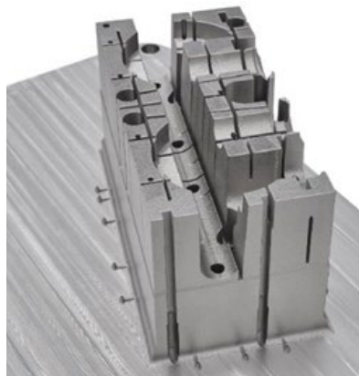
Erofió Group's mould core, which represents the first part manufactured in the company's trialling of the Concept Laser M Line (Courtesy Erofió Group)
