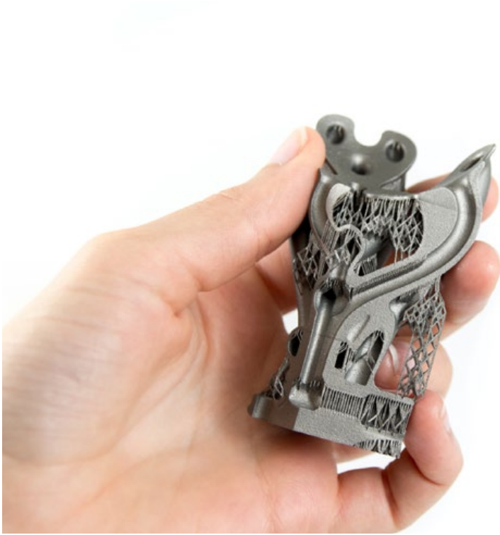
Fig. 6 In 2017, Materialise e-Stage became the first software in the world to automate support generation for titanium, stainless steel and aluminium AM parts (Courtesy Materialise)
