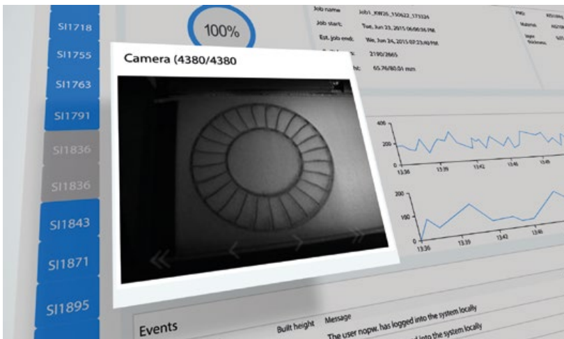
Fig. 3 EOSTATE software is used to monitor how machines are performing to enable predictive maintenance (Courtesy EOS)
