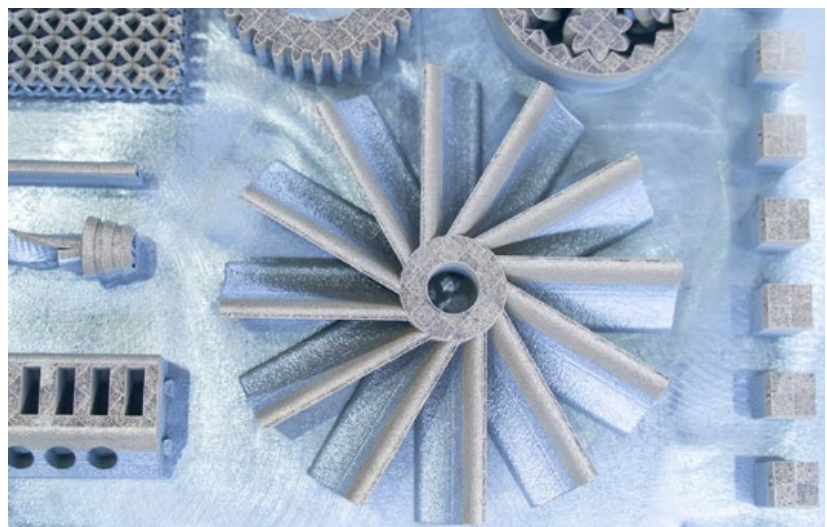
Fig. 1 Sigma Labs aims to accelerate the growth of the AM industry by collecting data on the PBF-LB AM process. Pictured are test parts produced using metal PBF-LB (Courtesy Sigma Labs)
