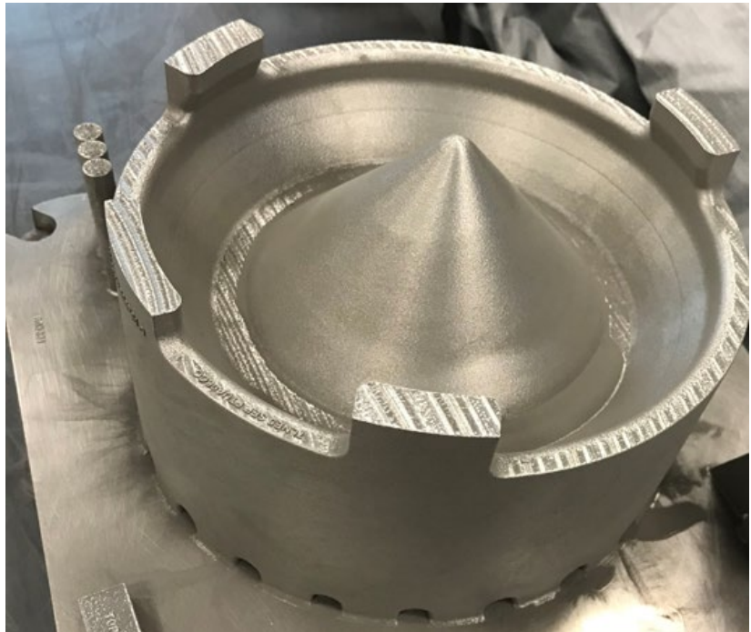
Additively manufactured, cobalt-chrome sump cover for F110 engine. Produced on a GE Additive Concept Laser M2 machine at the GE Additive Technology Center in Cincinnati, as part of collaboration with the US Air Force's Rapid Sustainment Office (Courtesy GE Additive)
