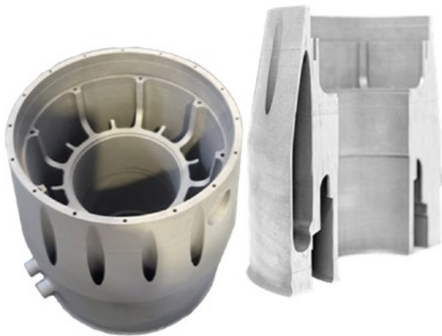
KW Micro Power designs and manufactures compact turbogenerators for high power density energy generation. The company redesigned its aerospace-grade auxiliary power unit (APU) model for metal AM, using aluminium F357, and built the component on a Velo3D machine, reducing weight by 44% (Courtesy Velo3D)
