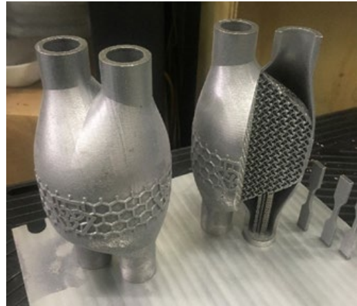
Fig. 6 Section view of completed heat exchanger, including hot and cold fluid zones (left), and the printed part showing minimal support material requirements (right).
