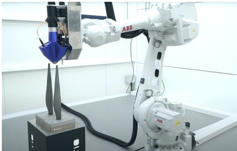
The Meltio system can be integrated into a robotic arm as a cost-effective solution for large metal part manufacturing (Courtesy Meltio)
