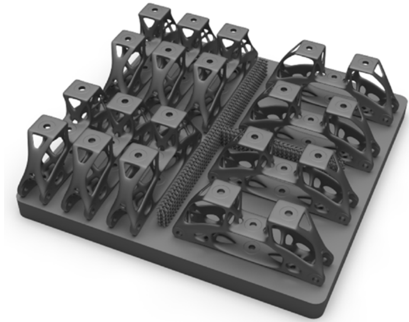
Fig. 7 A tray of parts with segmentation walls to separate parts that require different post processes (Courtesy Siemens)
