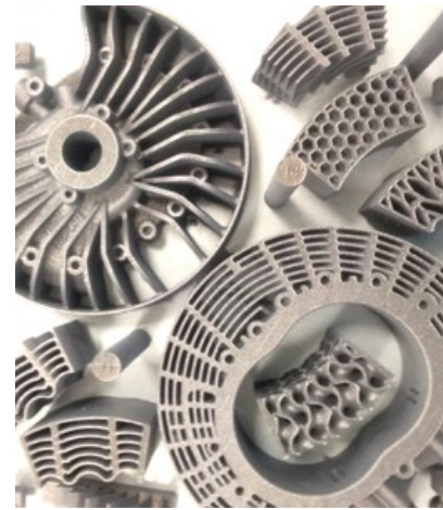
Various fin geometries tested against AIE's operational requirements (Courtesy DRAMA/AIE)
