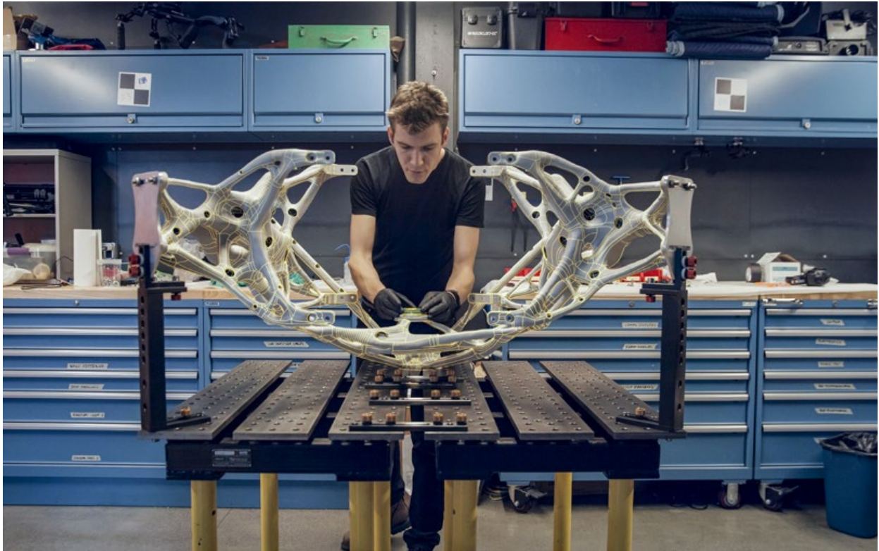
Fig. 7 A portion of the Lunar Lander concept made in collaboration with JPL, using generative design and Autodesk Fusion 360 (Courtesy Autodesk)
