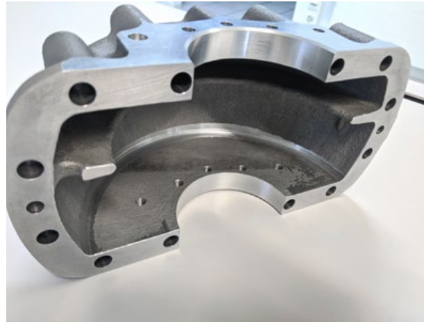
After the build, the gearbox casing was machined to required tolerances (Courtesy Sauber Engineering)
