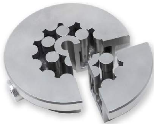
Fig. 7 Additive Manufacturing can be used for complex geometries with extremely small and intricate internal channels that would be difficult, if not impossible, to obtain with traditional technologies. This AM aerospace component has been cut open to show such internal channels (Courtesy BEAMIT)
