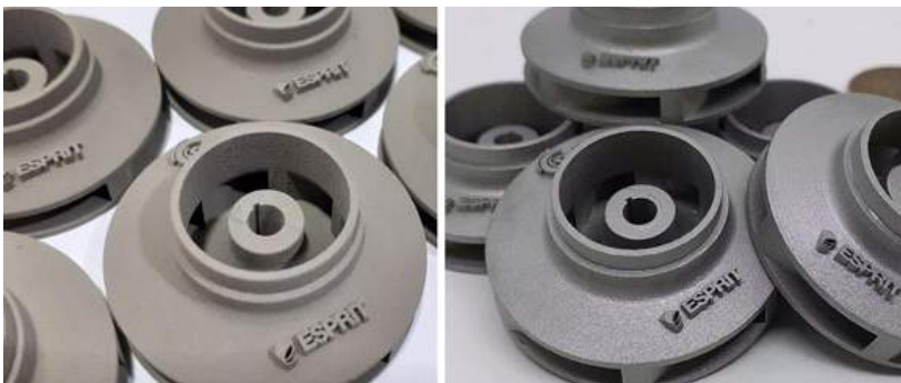
As built (left) and sintered (right) 40 mm impeller designed by Cetim, prepared with ESPRIT CAM and additively manufactured on Digital Metal equipment (Courtesy Cetim/ESPRIT CAM)
