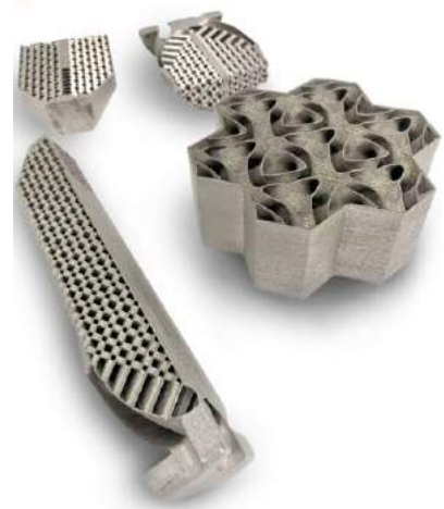
Test samples of different additively manufactured heat exchangers built in the Additive Manufacturing Lab at GE Research in Niskayuna, New York, USA (Courtesy GE Research)
