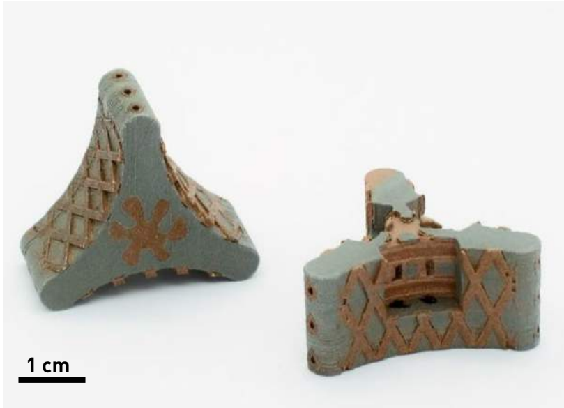
Fig. 8 Multi-material part, consisting of tool steel (1.2709) and a copper alloy (Courtesy of Fraunhofer IGCV)
