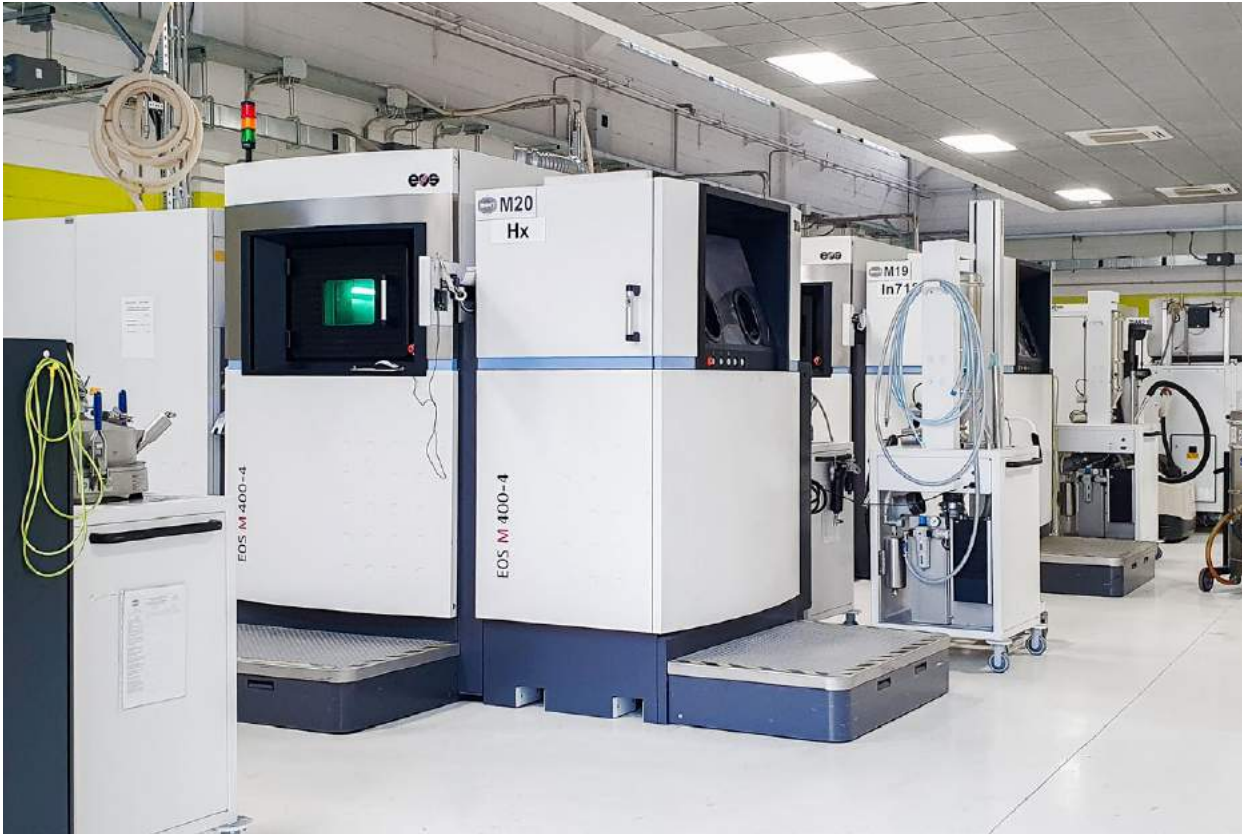
Fig. 8 EOS M 400-4 Laser Beam Powder Bed Fusion machines at BEAMIT (Courtesy BEAMIT)
