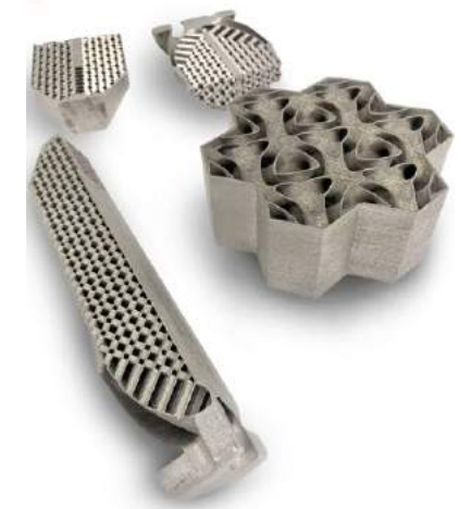
Test samples of different additively manufactured heat exchangers built in the Additive Manufacturing Lab at GE Research in Niskayuna, New York, USA (Courtesy GE Research)
