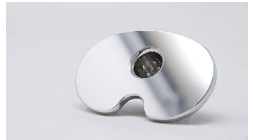
Fig. 6 Some of the first metal AM applications were in the area of medical implants. This tibial implant is produced in Ti6Al4V and CNC machined (Courtesy BEAMIT)
