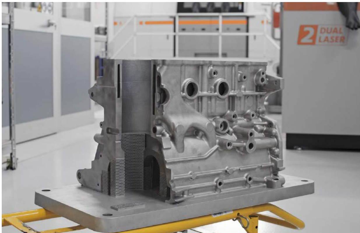
Fig. 12 Light alloys such as aluminium are ideally suited to single-piece AM engine blocks for motorsport (Courtesy BEAMIT)
