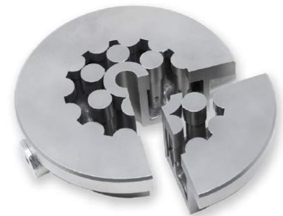
Fig. 7 Additive Manufacturing can be used for complex geometries with extremely small and intricate internal channels that would be difficult, if not impossible, to obtain with traditional technologies. This AM aerospace component has been cut open to show such internal channels (Courtesy BEAMIT)
