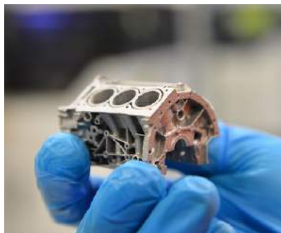
This aluminium 6061 engine block model demonstrates the high resolution and geometric control that can be produced in a new patent-pending binder jet AM process developed by ExOne and Ford Motor Company (Courtesy ExOne)
