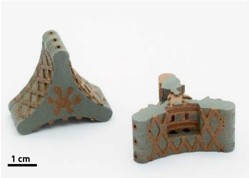
Fig. 8 Multi-material part, consisting of tool steel (1.2709) and a copper alloy [Courtesy of Fraunhofer IGC]
