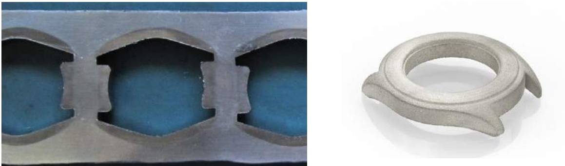
Fig. 2 Scrap from stamping (left) vs a near-net-shape AM watch case (right)
