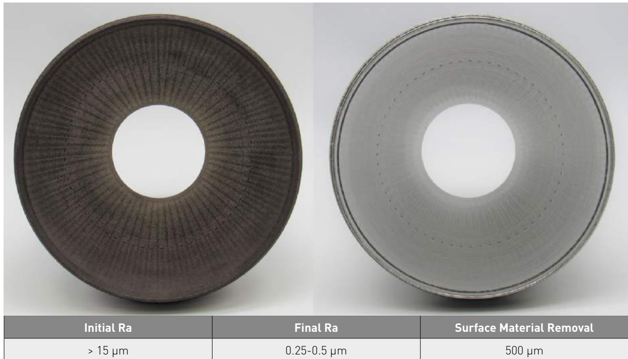
Fig. 14 1.2K BP-DED NASA HR-1 nozzles: (left) as-built/HIPed, (right) after in-development OFT (Manufactured by RPM Innovations, image courtesy NASA)
