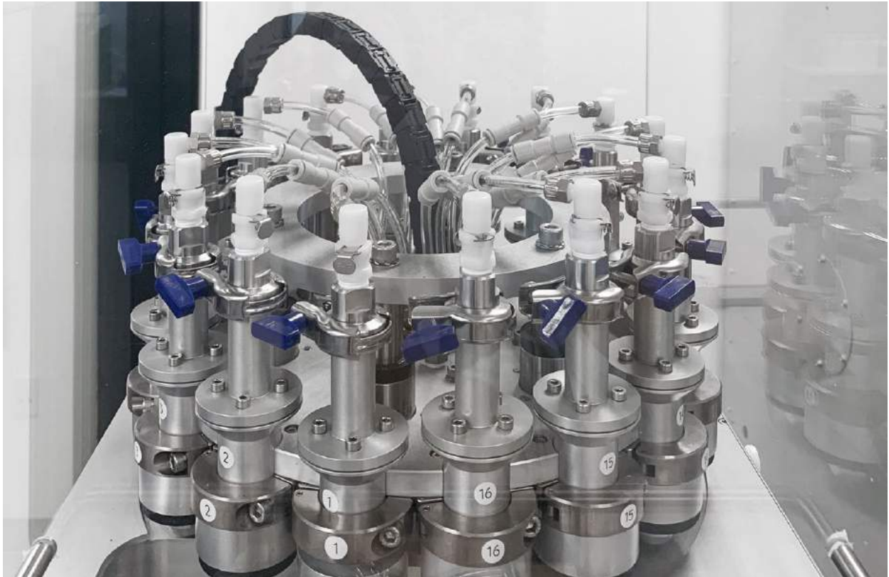
Fig. 5 FormAlloy's Alloy Development Feeder, designed for materials development and research (Courtesy FormAlloy)
