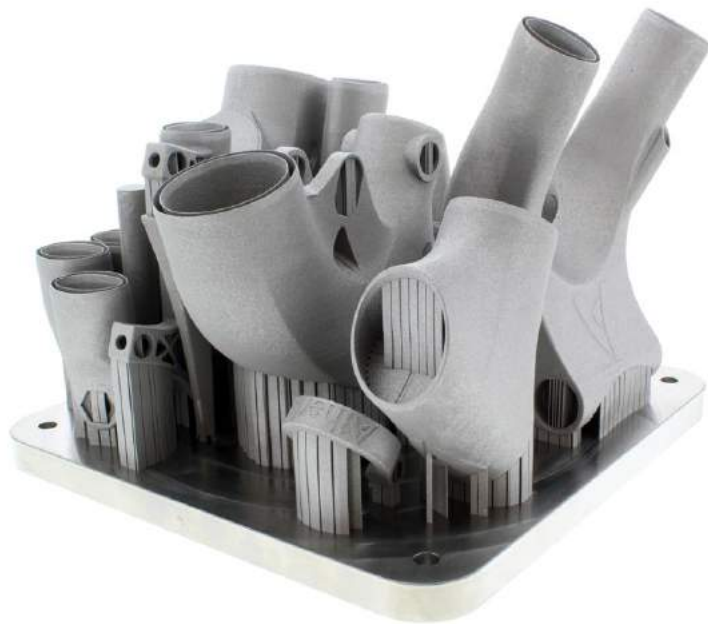
Fig. 6 The lug set on the build plate after removal from the RenAM 500Q build chamber. Note the structures that serve to both support the parts during the build and manage thermal stresses (Courtesy Renishaw PLC)
