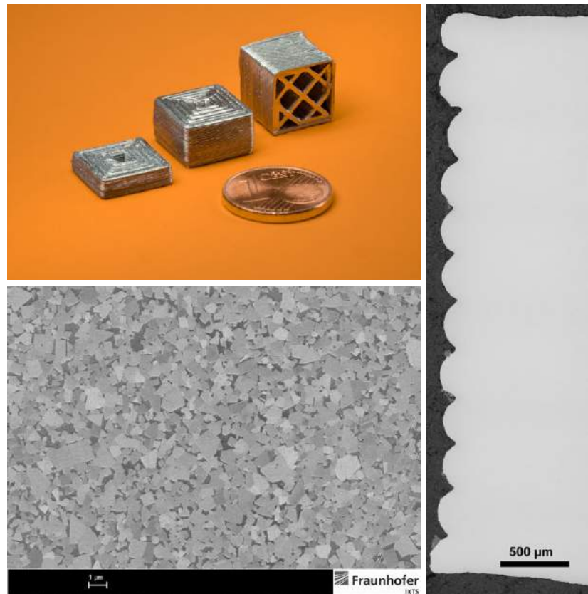
Fig. 7 MEX produced hardmetals (top left), SEM image of a dense WC-8 wt.% Ni hardmetal (bottom left) and optical image of a surface cross section (right)
