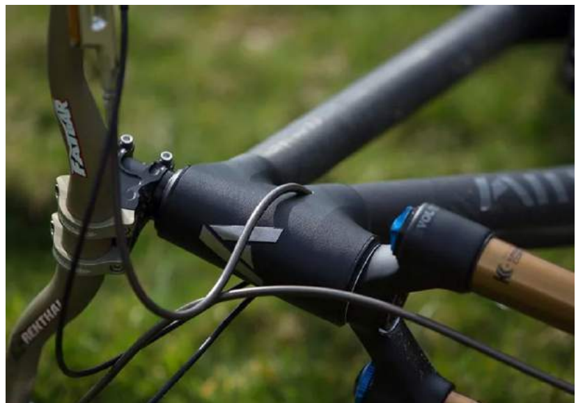
Fig. 1 Detail of the metal and carbon fibre frame construction used by Atherton Bikes, initially for competition and now for commercial sale (Courtesy Sven Martin)
