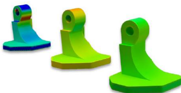
Three phases of automated optimisation show compensation for distortion using the metal Binder Jetting module in Simufact Additive. The results show the deviation between the simulated part and its initial CAD geometry – blue/red = bad; green = good (Courtesy Simufact)
