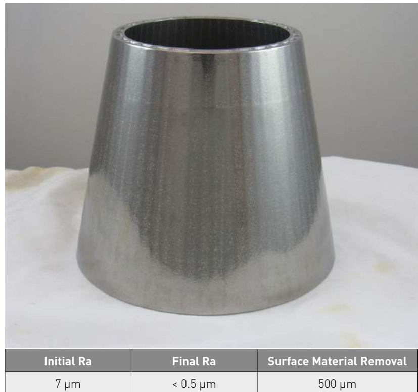
Fig. 10 OFT demonstrator part, PBF-LB IN625
