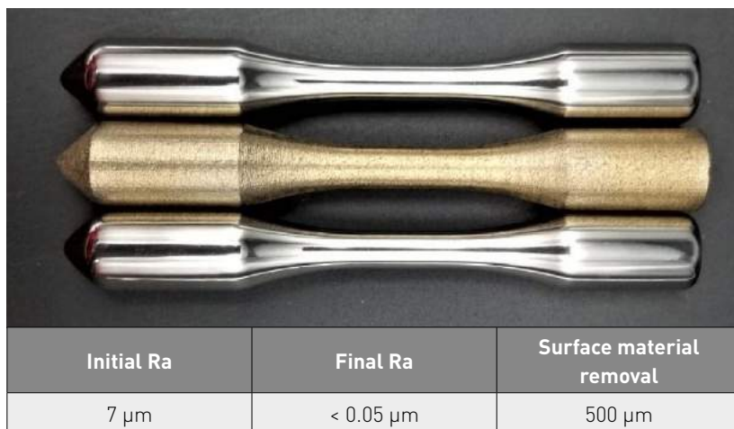
Fig. 12 PBF-LB IN718, as-built/HIPed (middle) and after OFT (top and bottom)
