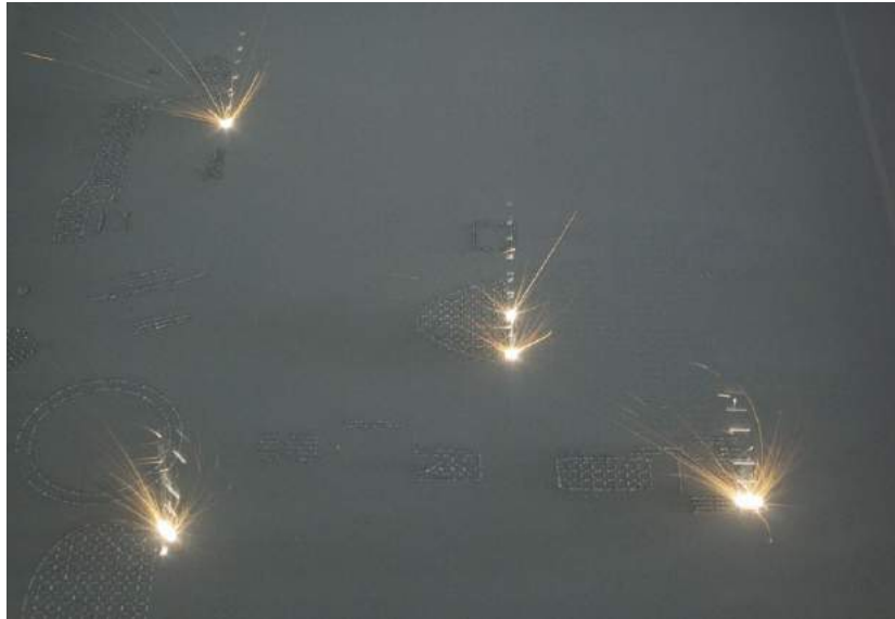
Fig. 5 A set of lugs being built on a RenAM 500Q four-laser PBF-LB system. (Courtesy Renishaw PLC)
