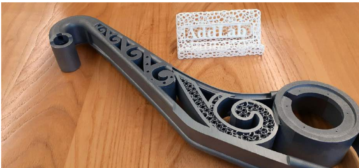
Fig. 3 Air New Zealand monitor bracket, with weight reduction of 40% (Courtesy AddLab)
