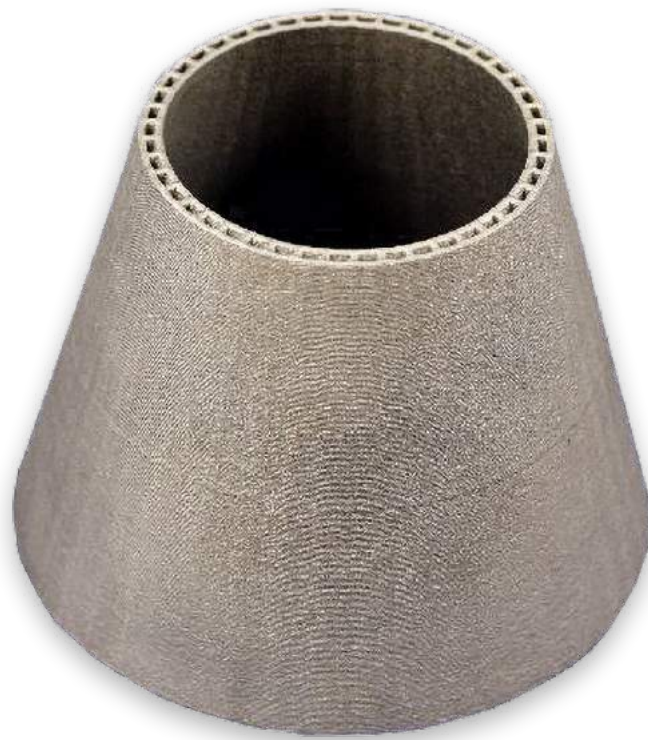
Fig. 6 Demonstrator component, BP-DED IN625 (Courtesy NASA MSFC)
