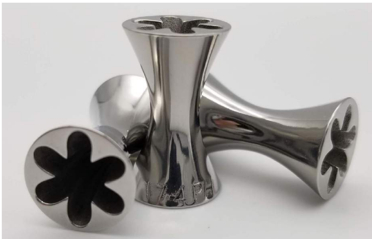
Fig. 5 Chemical-mechanical polished 17-4 PBF-LB component examples, additively manufactured by 3 rd Dimension Industrial Printing
