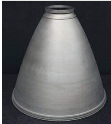
Blown powder Directed Energy Deposition can produce large structures such as these engine nozzles (Courtesy NASA)
