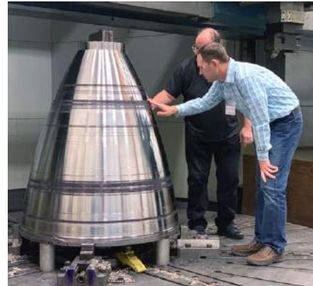
Blown powder Directed Energy Deposition can produce large structures such as these engine nozzles (Courtesy NASA)
