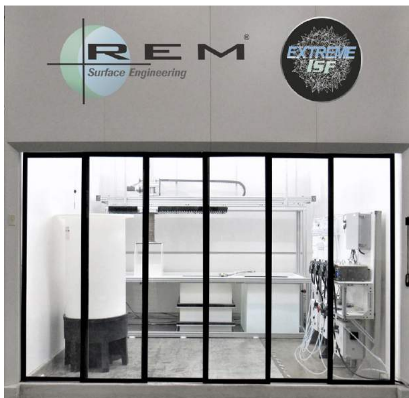
Fig. 13 Automated chemical polishing processing cell
