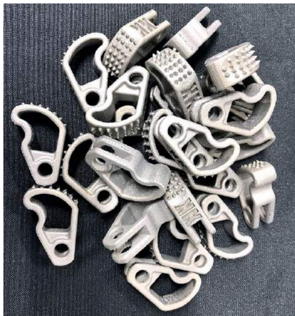
Fig. 7 Kiwi Klimbers toothed cams for climbing equipment (Courtesy of RAM3D)
