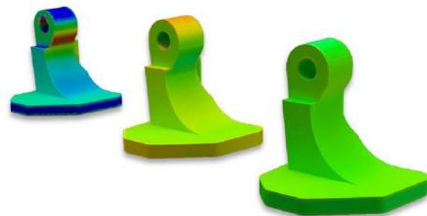
Three phases of automated optimisation show compensation for distortion using the metal Binder Jetting module in Simufact Additive. The results show the deviation between the simulated part and its initial CAD geometry – blue/red = bad; green = good (Courtesy Simufact)
