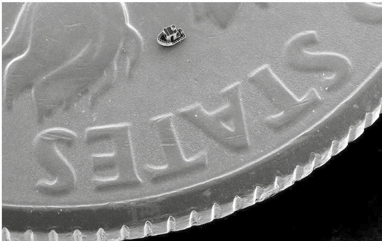
Fig. 12 A Benchy calibration part manufactured using the LRM process on top of an American quarter coin [Courtesy Micromaker]
