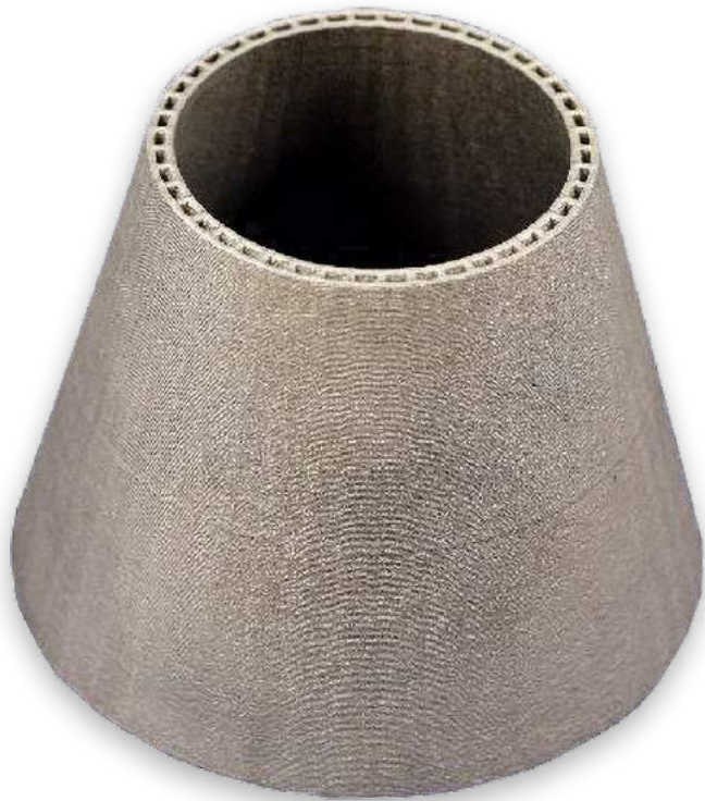
Fig. 6 Demonstrator component, BP-DED IN625 (Courtesy NASA MSFC)
