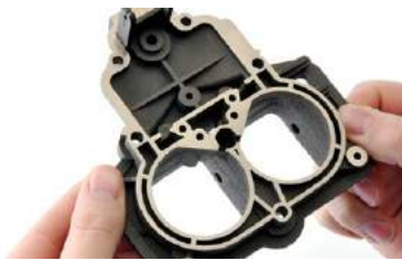
The carburettor for a vintage Ferrari, reproduced using Binder Jetting (Courtesy The ExOne Company)
