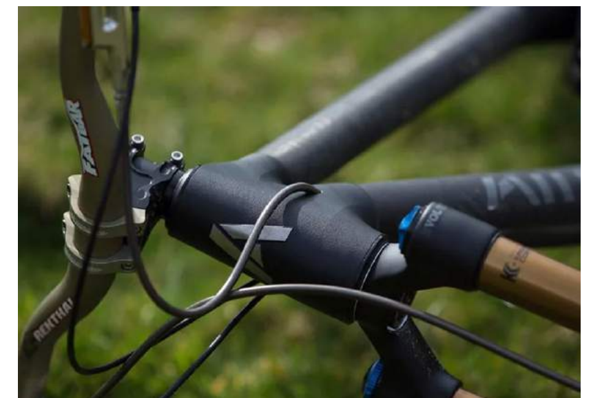
Fig. 1 Detail of the metal and carbon fibre frame construction used by Atherton Bikes, initially for competition and now for commercial sale [Courtesy Sven Martin]
