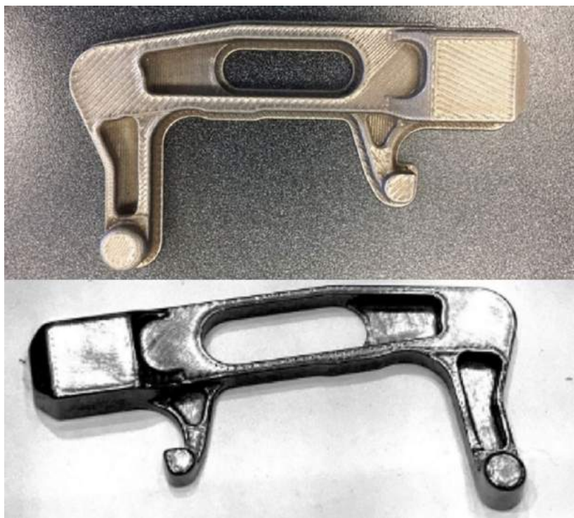
Fig. 7 A door handle produced by FormAlloy for a commercial aerospace application. Top: the as-built part, Bottom: the chemically finished part (Courtesy FormAlloy)
