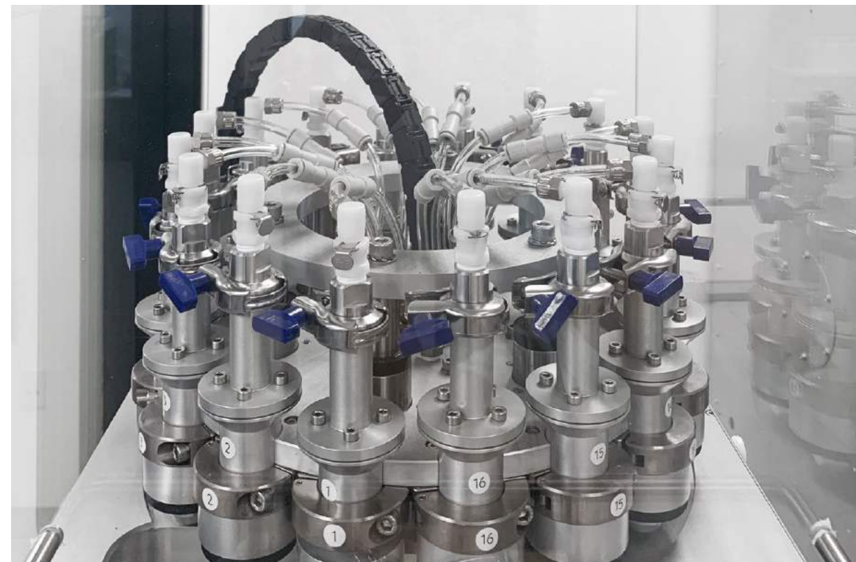
Fig. 5 FormAlloy's Alloy Development Feeder, designed for materials development and research (Courtesy FormAlloy)
