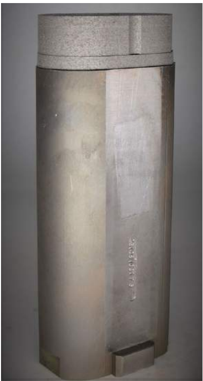
Fig. 13 Hybrid AM mould insert as it comes off the DMP Flex 350 machine. Finely tuned laminar argon flow guarantees a high removal rate of fumes which are the main driver of inconsistent density. Thanks to the unique calibration process, the alignment between the AM section and the preform is very accurate
