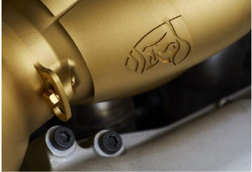
Fig. 5 FZed exhaust collector additively manufactured in titanium and PVD-coated in titanium nitride [Courtesy Rodin Cars]
