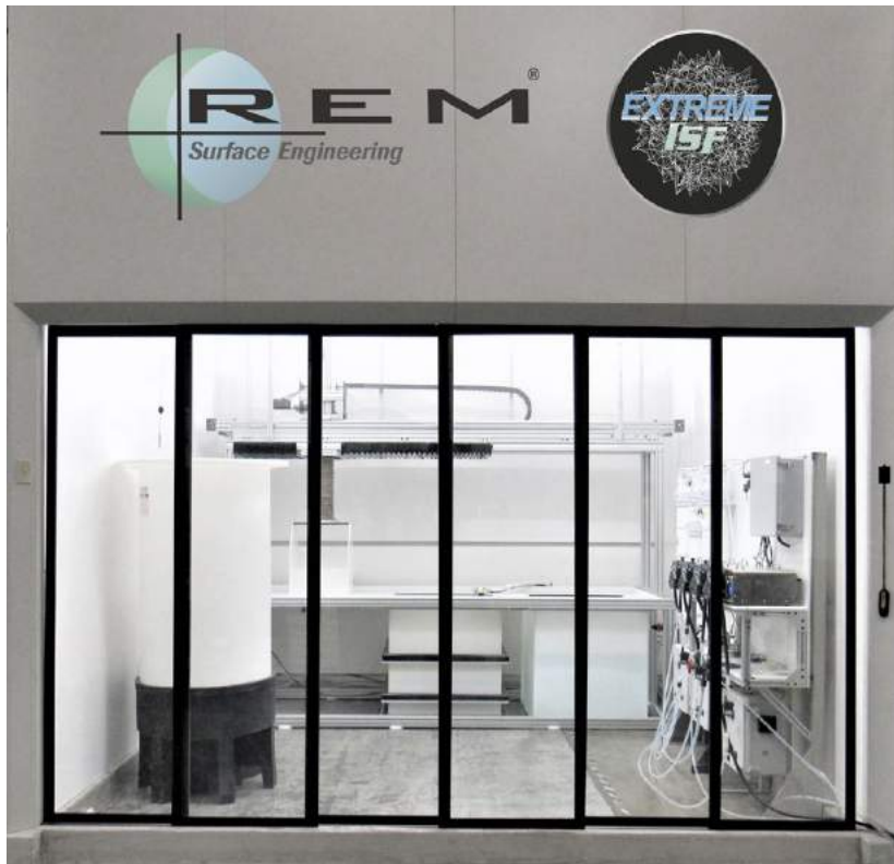
Fig. 13 Automated chemical polishing processing cell
