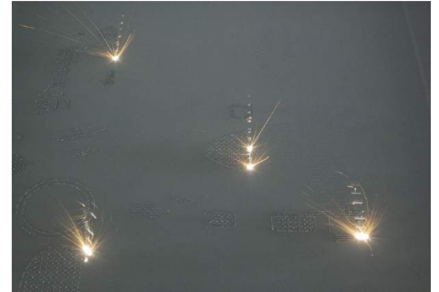
Fig. 5 A set of lugs being built on a RenAM 500Q four-laser PBF-LB system. (Courtesy Renishaw PLC)
