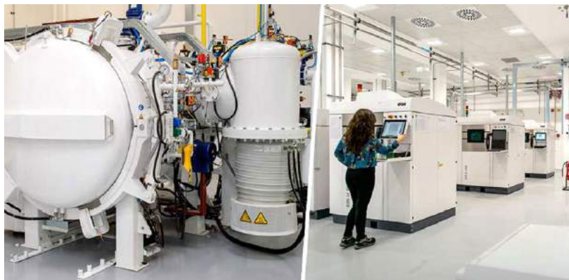
A vacuum furnace (left) and EOS metal Additive Manufacturing machines (right) at Lincotek Additive's Additive Production Center (Courtesy Lincotek Additive)
