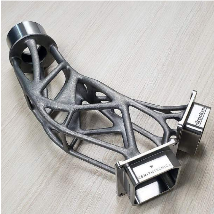
Fig. 2 Satellite bracket produced by EBM [Courtesy Zenith Technica]
