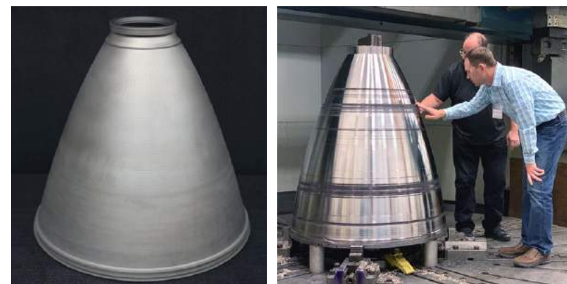
Blown powder Directed Energy Deposition can produce large structures such as these engine nozzles (Courtesy NASA)
