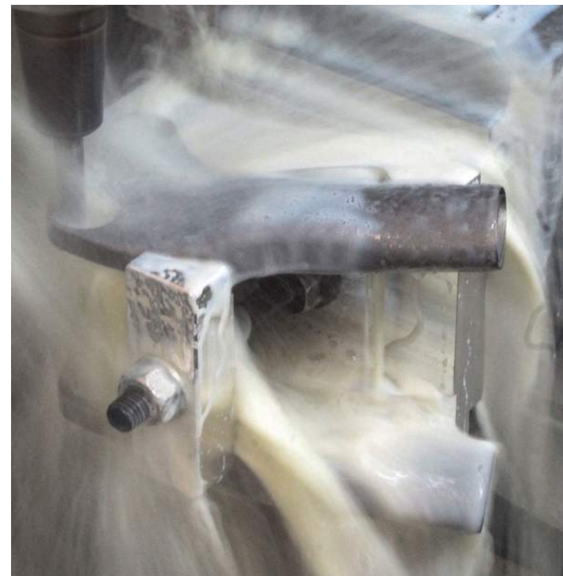
Fig. 8 After heat treatment to relieve stresses from the build process, parts have to be removed from the build plate and machined to remove support structures. Critical surfaces are also machined to meet tolerances or provide a necessary functional surface (Courtesy Renishaw PLC)
