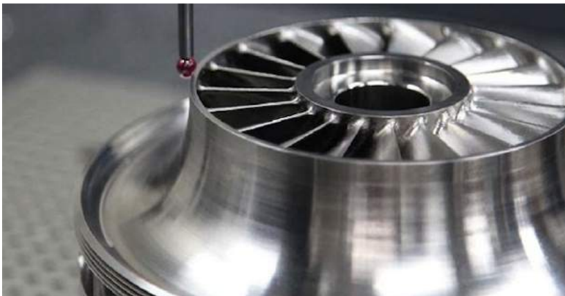
The additively manufactured shrouded radial expander wheel for a solar power array (Courtesy Velo3D)
