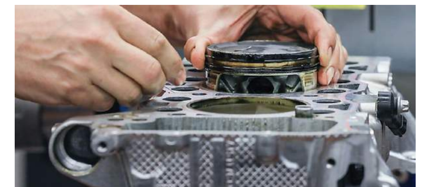
An aluminium AM piston is installed for testing on the engine test bench for Porsche's 911 GT2 RS sports car (Courtesy Porsche)
