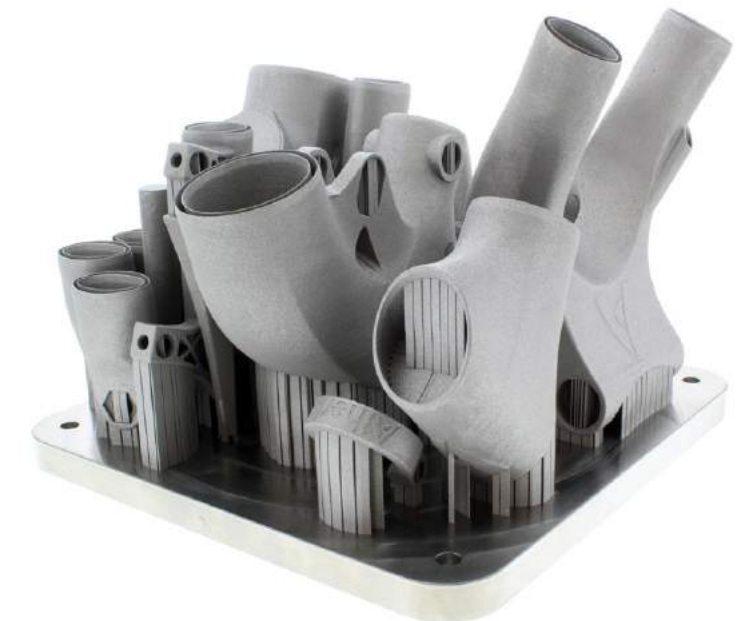
Fig. 6 The lug set on the build plate after removal from the RenAM 500Q build chamber. Note the structures that serve to both support the parts during the build and manage thermal stresses (Courtesy Renishaw PLC)
