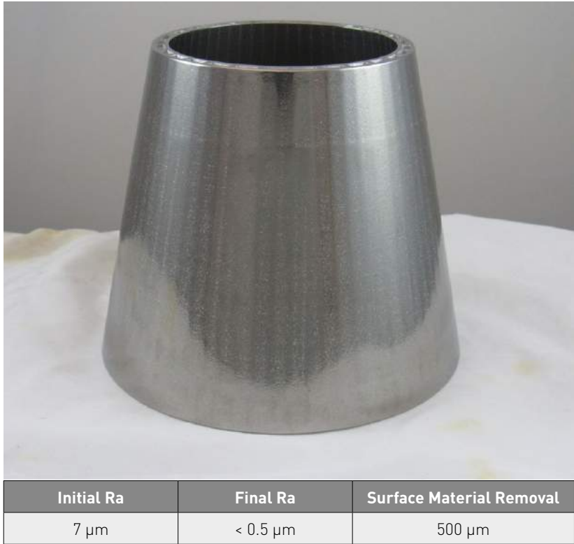
Fig. 10 OFT demonstrator part, PBF-LB IN625
