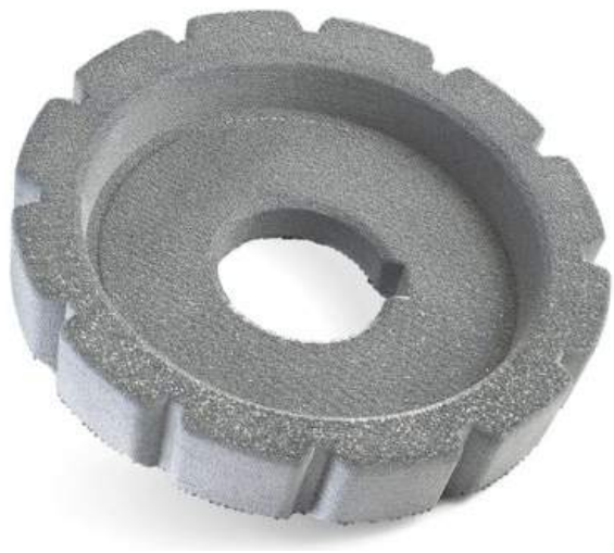
Fig. 7 A shape cutter (Ø 120 mm) in the as-built state, manufactured using PBF-EB by VBN Components AB from Vibenite® 290, an Fe/Co/W base material that combines high wear resistance and heat resistance. The component has a hardness of approximately 72 HRC (Courtesy VBN Components AB)
