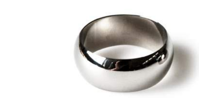
Fig. 15 An AM band produced using a gold and niobium powder blend. Weight is 12 g versus 16 g for regular palladium white gold. Premium white WGC colour, fineness 750%, manufactured by Progol3D® [Courtesy Progold S.p.A.]
