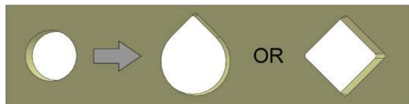
Fig. 6 For horizontal holes, use a teardrop or diamond shape whenever possible
