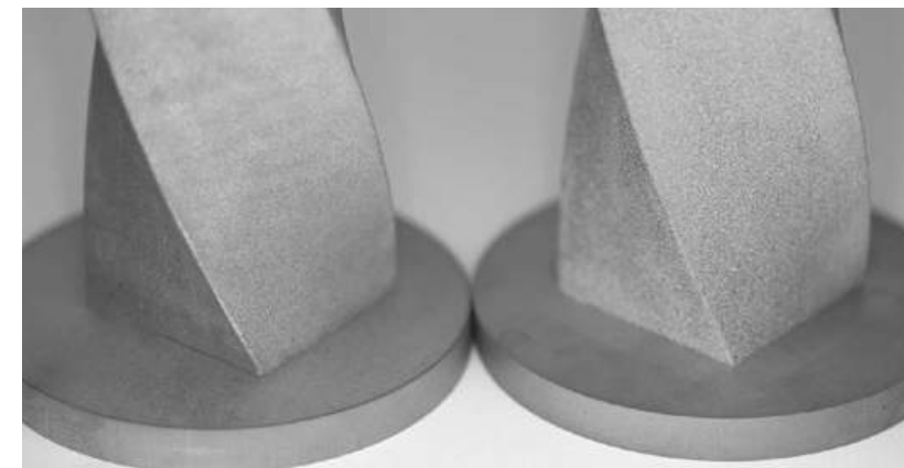
Fig. 6 Two geometries in 316L stainless steel, one built with 15–53 \mu\text{m} powder and 30 \mu\text{m} layers (left) and one built with 53–150 \mu\text{m} powder and 100 \mu\text{m} layers. Each build plate is 100 mm in diameter and the powder was supplied by Carpenter Additive. Both builds ran smoothly without smoke events or other issues. As can be expected, the fine powder and thinner layers give a notably better surface finish (Courtesy Freemelt AB)
