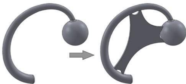
Fig. 4 Make parts strong enough to handle in their green state
