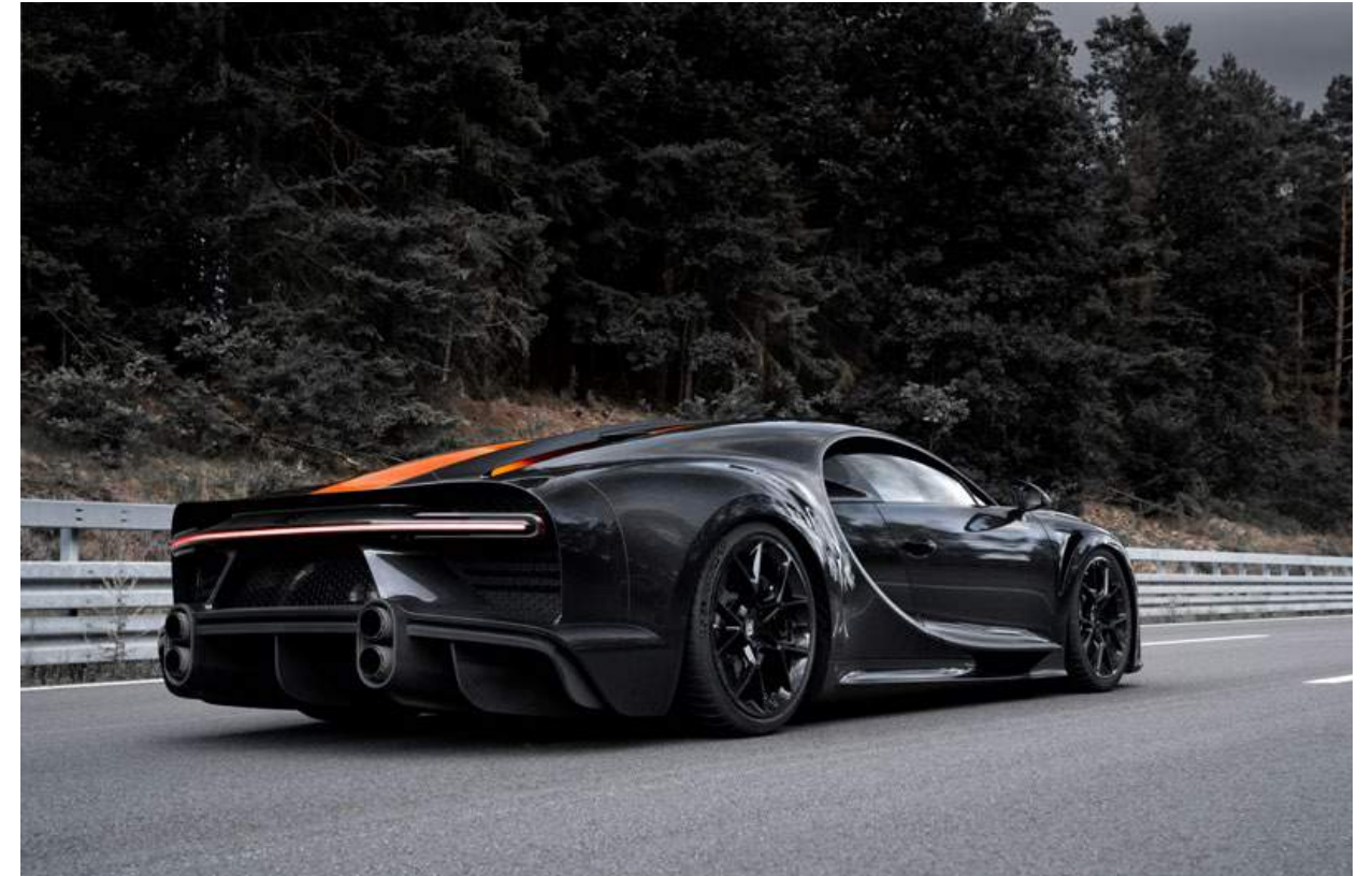
Fig. 8 This Bugatti Chiron Super Sport 300+ broke the 300 mph barrier with AM exhaust finishers produced by APWORKS (Courtesy Bugatti Automobiles S.A.S.)
