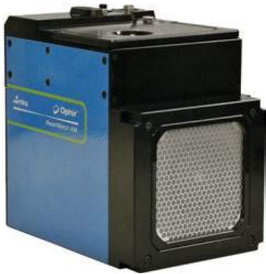
Fig. 6 The Ophir BeamWatch AM measures beam position and angle of incidence, focal spot size, position and quality parameters such as M² and beam caustic in real-time in AM machines
