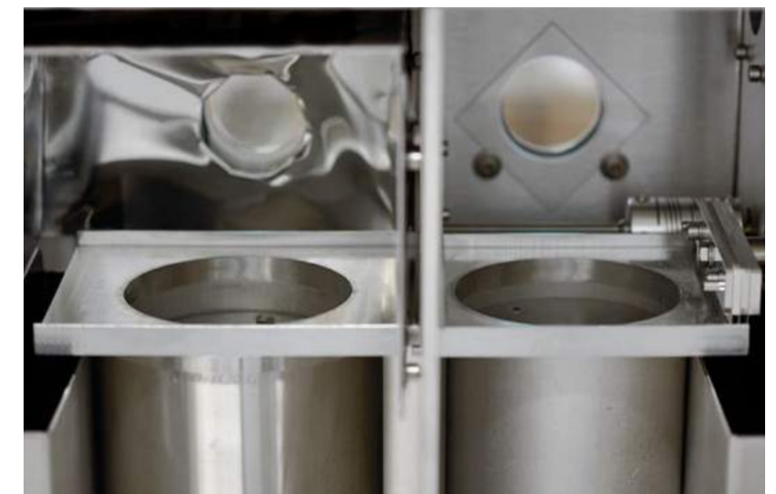
Fig. 1 View into the Freemelt ONE Electron Beam Powder Bed Fusion system's build chamber (Courtesy Freemelt AB)
