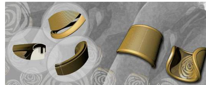
Fig. 9 Various items including a miniature 18 Kt gold galleon as built in a Precious M 080 PBF-LB system from EOS GmbH and Cooksongold (Courtesy Frank Cooper, Birmingham School of Jewellery, UK / Cooksongold)
