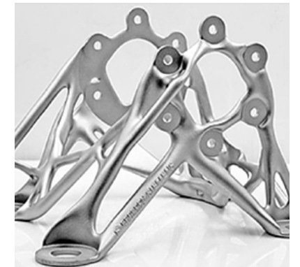
An aluminium gearbox mount from a Siemens sponsored Formula Racing car was the first collaboration. The part is designed by Siemens NX software and fabricated on a Farsoon FS301M (Courtesy Farsoon)
