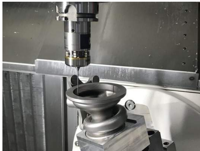
3T-am's part setup time was reduced from five hours to ten minutes (Courtesy MSP)
