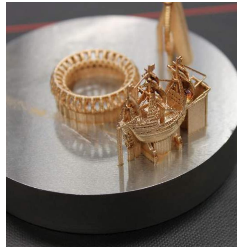
Fig. 9 Various items including a miniature 18 Kt gold galleon as built in a Precious M 080 PBF-LB system from EOS GmbH and Cooksongold (Courtesy Frank Cooper, Birmingham School of Jewellery, UK / Cooksongold)
