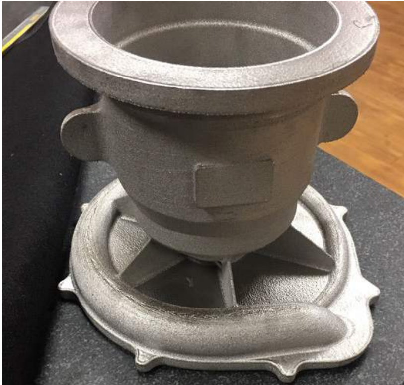
Fig. 6 Metal additively manufactured space housing produced by Collins Aerospace (Courtesy Collins Aerospace)
