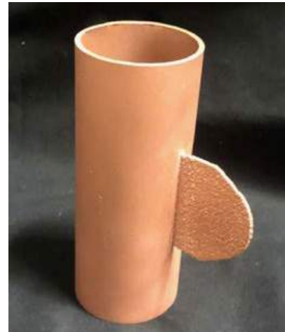
A pure copper fin feature added to a copper tube using Directed Energy Deposition (Courtesy Optomec)
