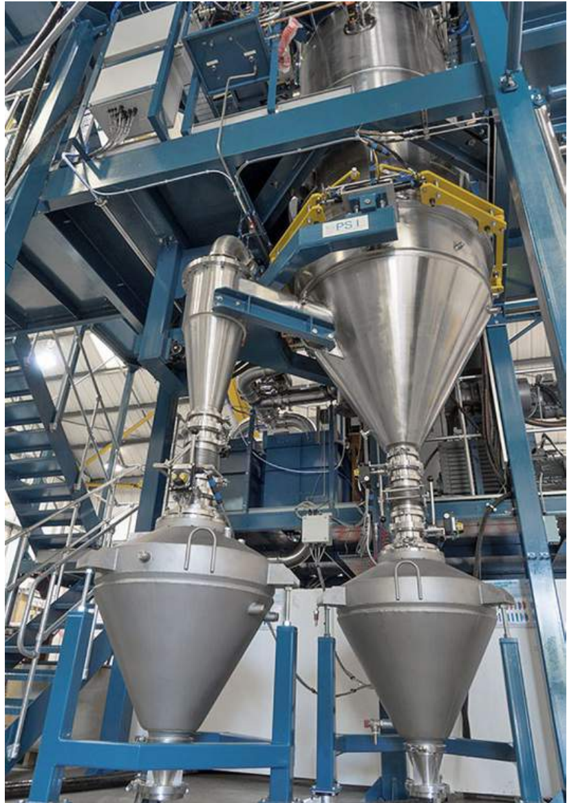
Fig. 3 A view of a Hermiga gas atomiser at the UK's PSI Ltd. Gas atomisation is currently the dominant technology for the production of metal powders for AM and a number of companies are able to supply production-ready atomisation systems that range from laboratory to industrial scale (Courtesy PSI Ltd)
