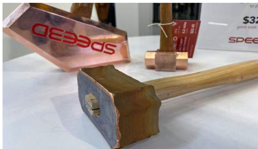
SPEE3D built this 1kg hammer head in just over ten minutes, live at Formnext
