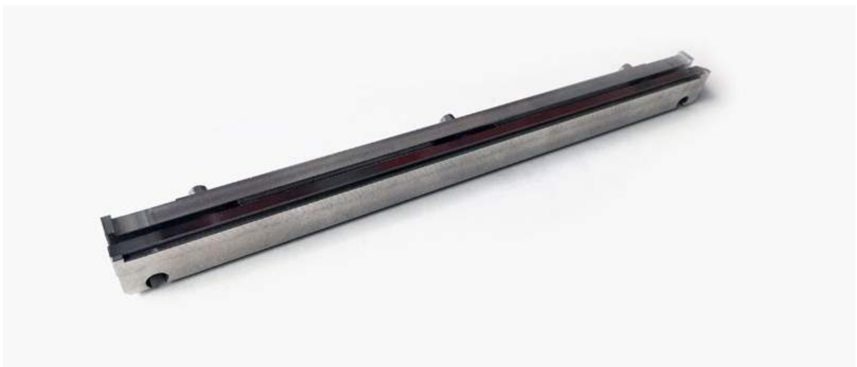
Fig. 3 Hard recoater with stainless steel blade
