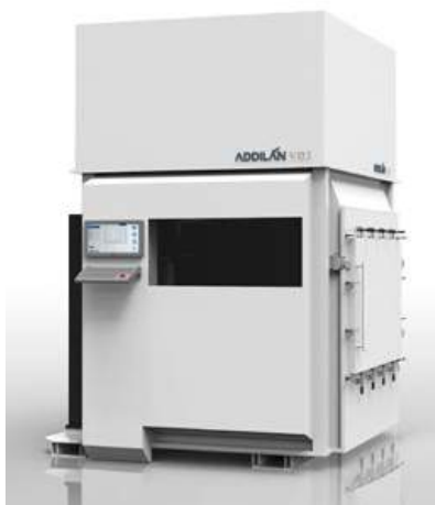
Addilan's WAAM machine is said to offer deposition rates up to 6 kg per hour (Courtesy Addilan)
