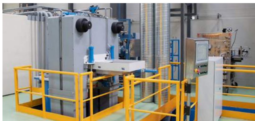
The new HIP has a maximum operating pressure of 2,050 bars and an oven that reaches 1,400°C (Courtesy Hiperbaric)
