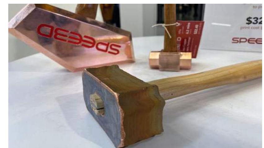
SPEE3D built this 1kg hammer head in just over ten minutes, live at Formnext
