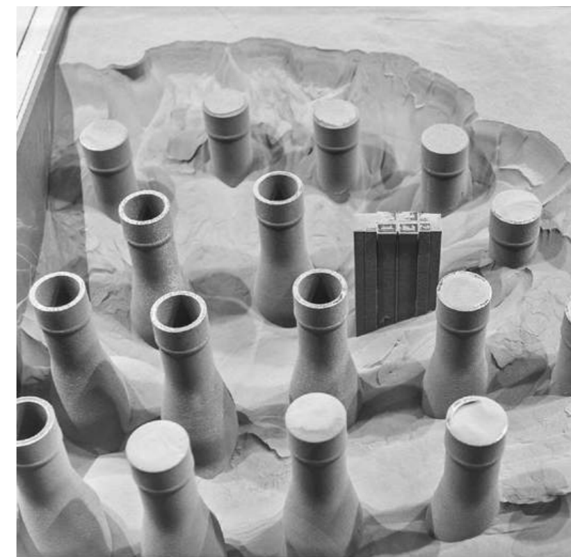
Fig. 5 Door latch shafts for the A350 XWB passenger aircraft produced using Laser Powder Bed Fusion at Airbus Helicopters Donauwörth (Courtesy Airbus)
