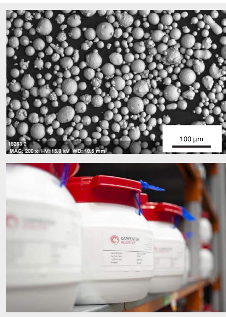
Fig. 4 Top image, SEM of Carpenter 316L AM powder. Lower image, containers of standardised materials in the PowderRange™ portfolio, specifically optimised for different types of AM processes and covering 80% of today's application and machine types
