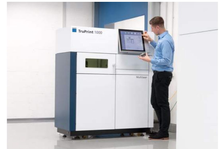
Fig. 1 Trumpf's TruPrint 1000 L-PBF machine
