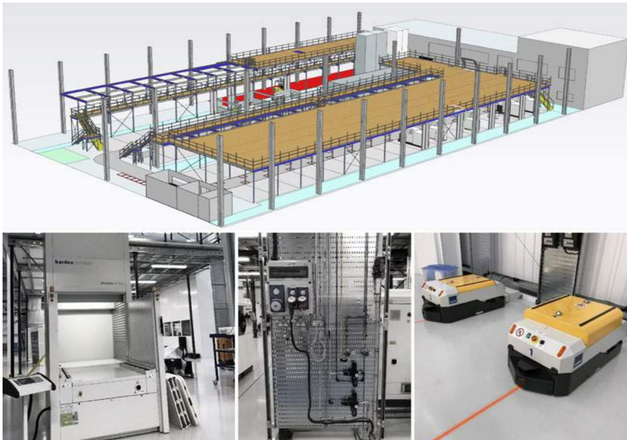
Fig. 8 Creating an effective factory layout for series L-PBF production at Materials Solutions
