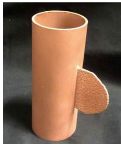
A pure copper fin feature added to a copper tube using Directed Energy Deposition (Courtesy Optomec)
