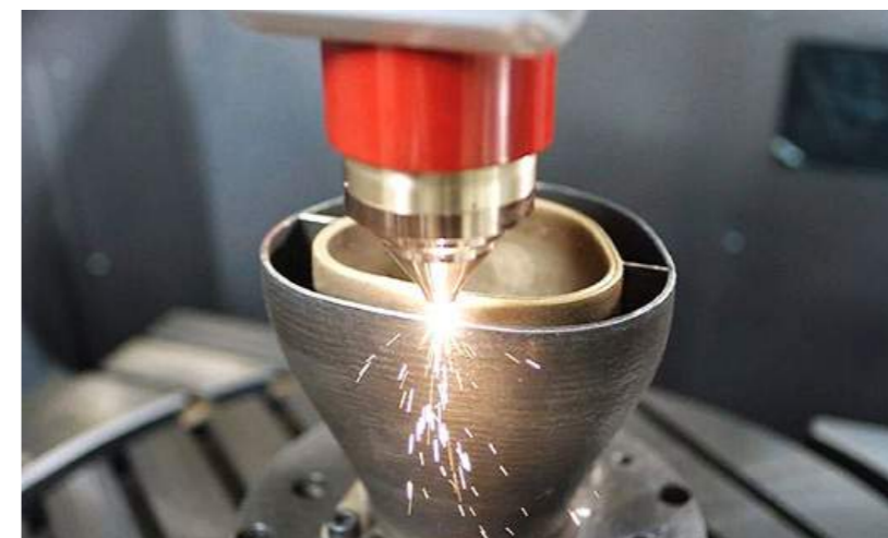
Multi-material applications and graded materials can be produced with the company's hybrid machines (Courtesy DMG MORI)
