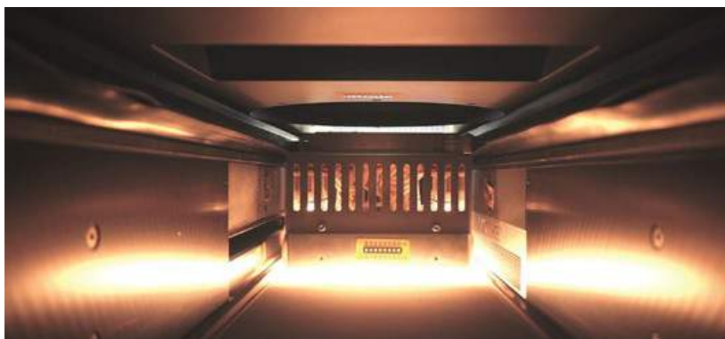
Preheating the machining plane with the NIR is said to significantly reduce stresses in the L-PBF additively manufactured component (Courtesy Fraunhofer ILT)
