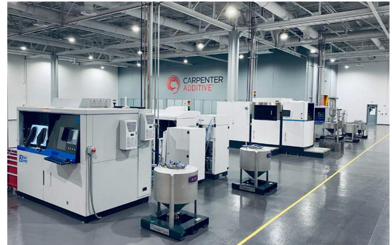
Fig. 9 Carpenter Additive's newly built Emerging Technology Center in Athens, Alabama, includes both Electron Beam Melting machines and L-PBF systems
