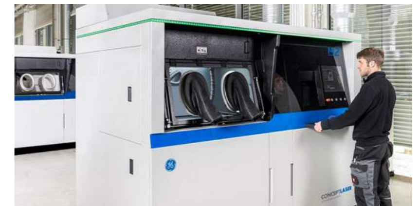
The new M2 Series 5 includes a dual laser system (Courtesy GE Additive)
