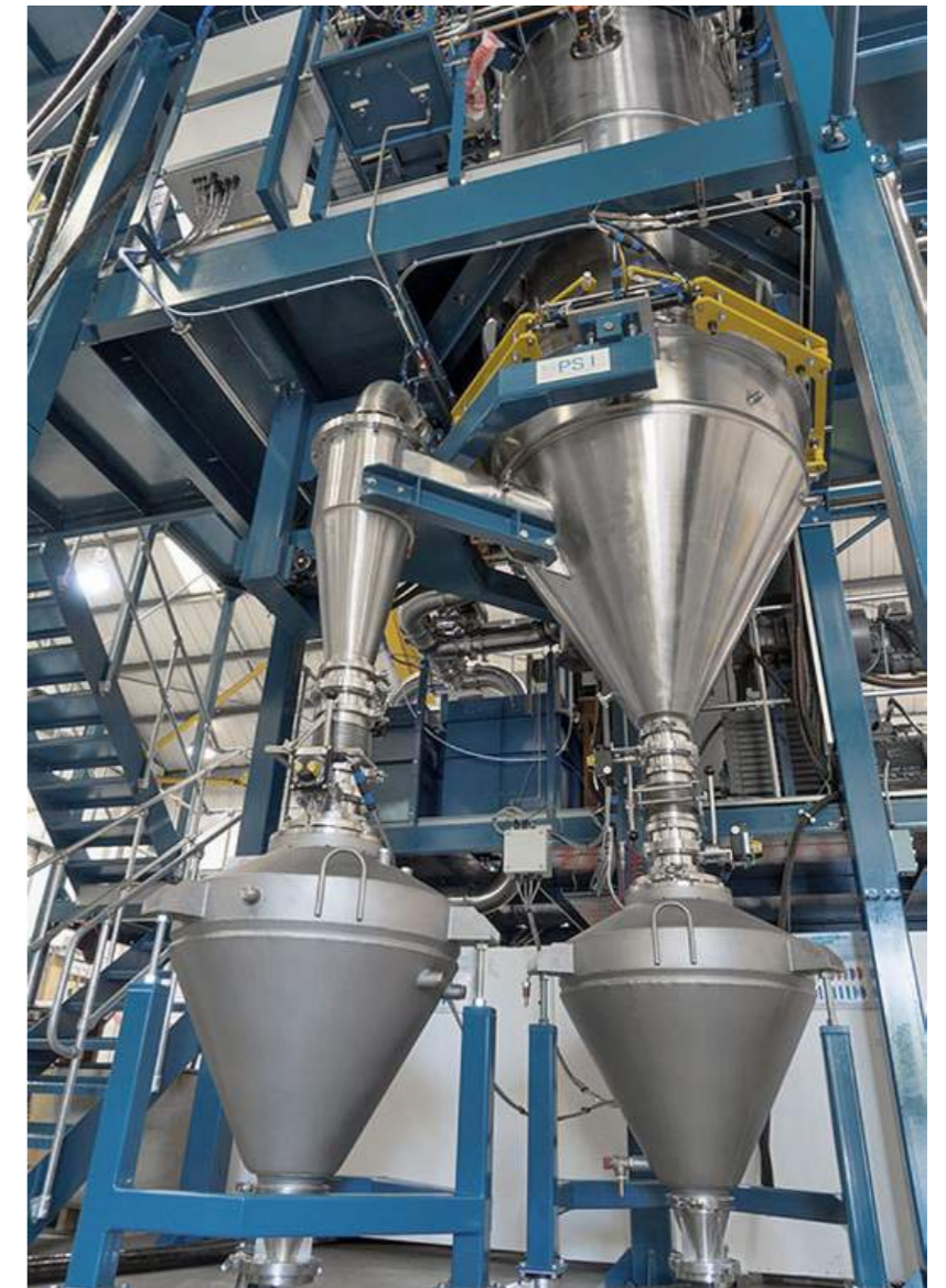
Fig. 3 A view of a Hermiga gas atomiser at the UK's PSI Ltd. Gas atomisation is currently the dominant technology for the production of metal powders for AM and a number of companies are able to supply production-ready atomisation systems that range from laboratory to industrial scale (Courtesy PSI Ltd)
