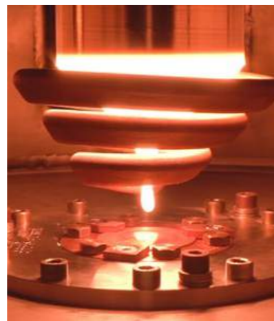
Titanium atomisation at Sandvik's new facility [Courtesy Sandvik]
