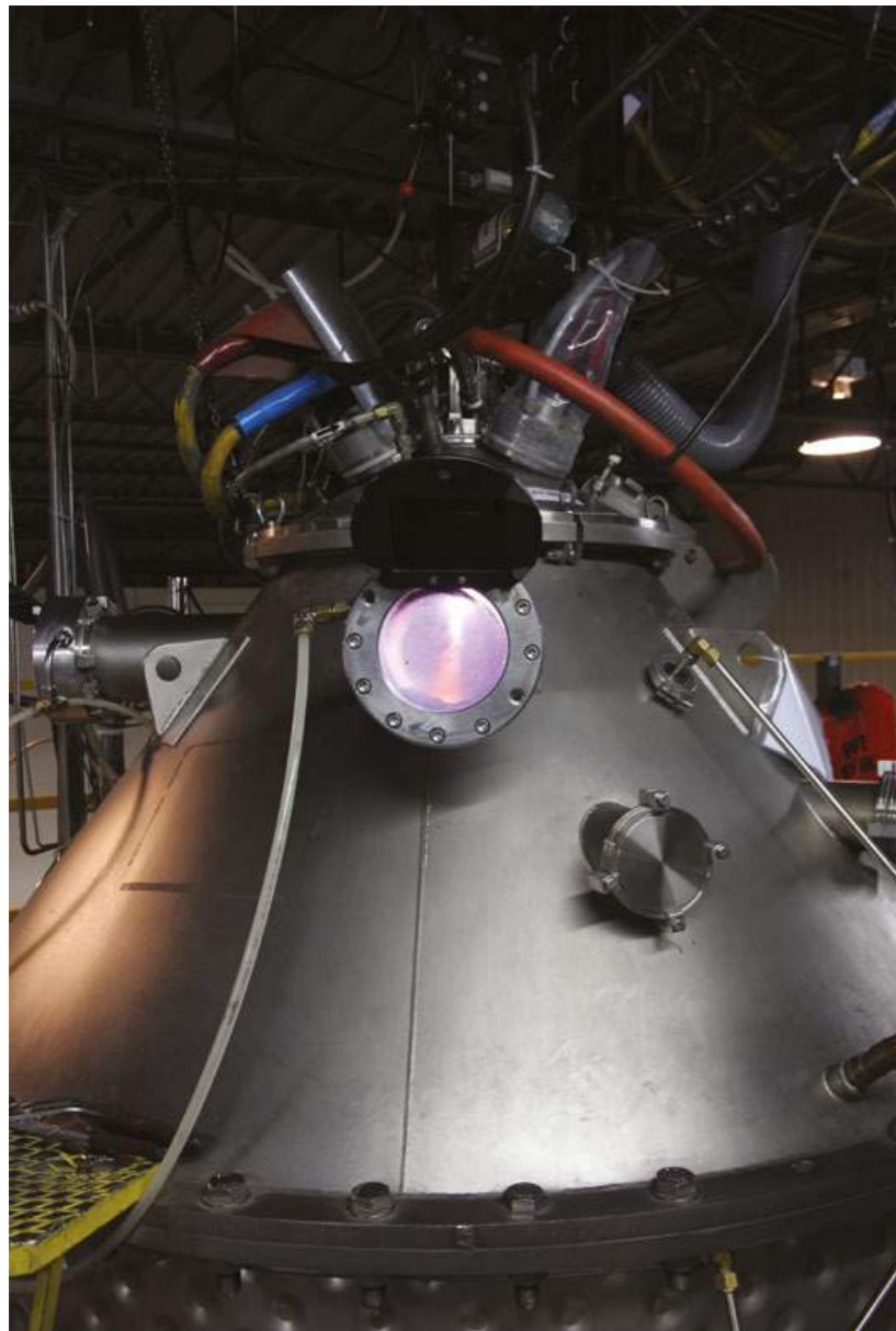
Fig. 4 Plasma atomisation underway on an industrial scale at Canada's AP&C. GE acquired AP&C as part of its Arcam acquisition (Courtesy AP&C)
