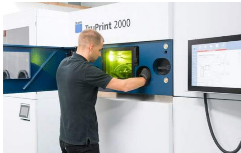
The TruPrint 2000 enables the operator to remove excess metal powder without having to take it from the machine (Courtesy Trumpf)
