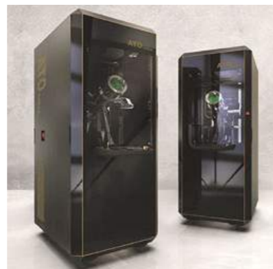
The AtoNoble powder atomiser for precious metal powders (Courtesy 3D Lab sp. z.o.o.)
