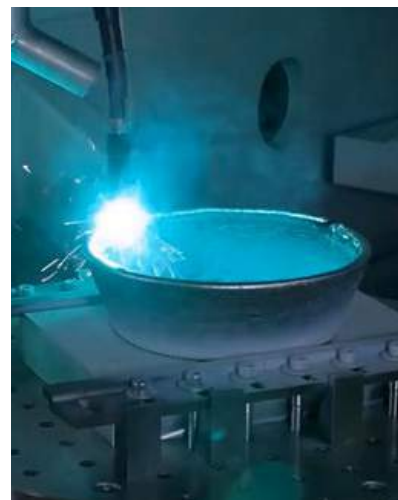
Gefertec's 3DMP process is a wire-based Additive Manufacturing system (Courtesy Gefertec)
