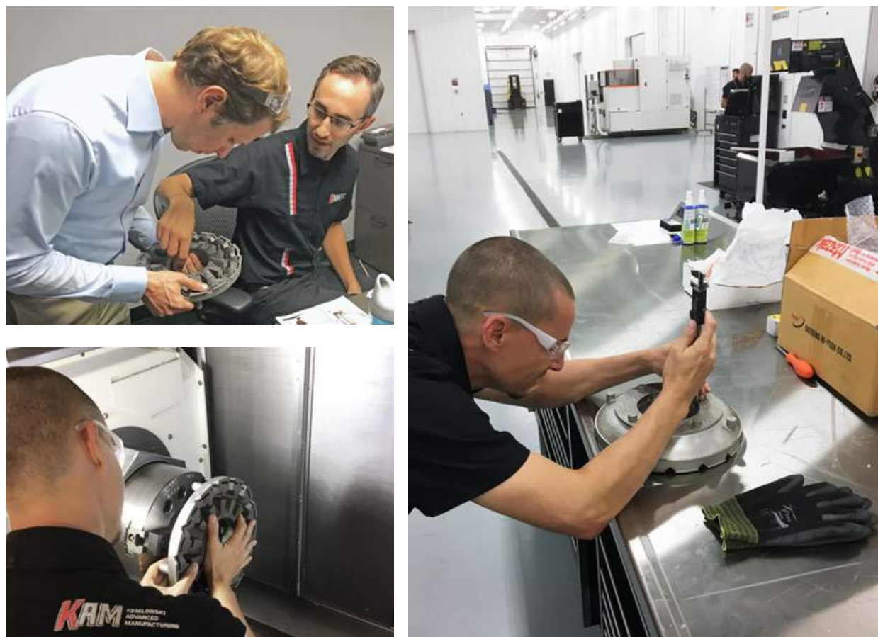
Fig. 8 Top left, Brad Keselowski, Founder & CEO of KAM, and Michael Mullen, KAM Engineering Manager, discuss the differences between two builds of the KW MicroPower diffuser before machining. Bottom left, qualifying the diffuser's datum surface on MAZAK i300 Integrex Mill/Turn machining centre. Right: CNC machinist Colby Burgin checks the diffuser dimensions for best fit of machining to built part, ensuring proper alignment of the part envelope with the machine work coordinate system
