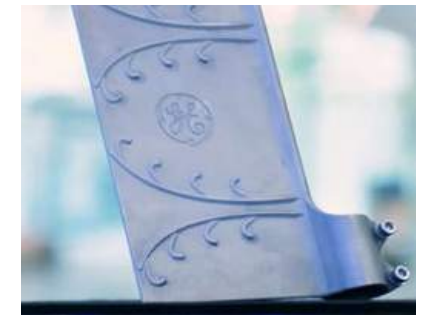
The racking blade incorporates internal channels to distribute water evenly (Courtesy GE Additive)
