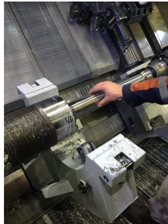
Fig. 6 Circulating head for Vallourec. Designed by Vallourec, shown as welded, during machining process using Böhler X90-IG
