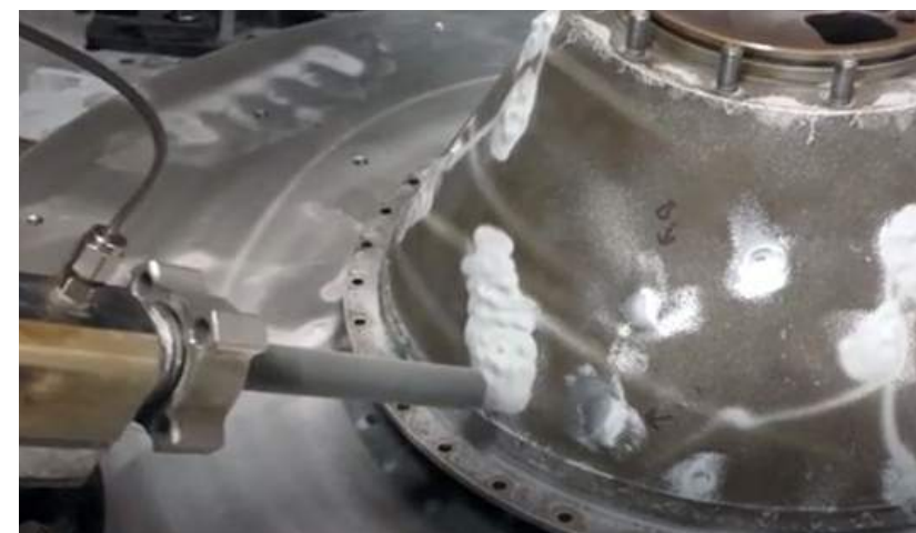
Cold spray Additive Manufacturing can be used to perform surface repairs on damaged metal structures (Courtesy Worcester Polytechnic Institute)
