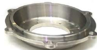
An additively manufactured wheel-set bearing cover for a Class 294 locomotive, produced on a Gefertec arc605 system at Rolf Lenk (Courtesy Deutsche Bahn)
