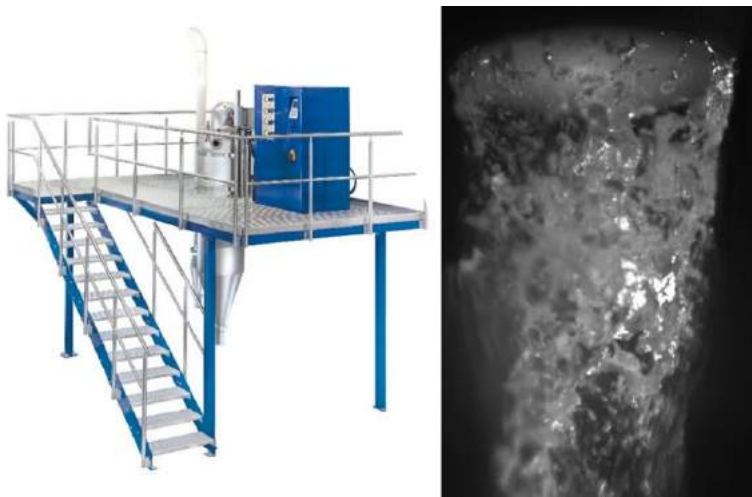
Fig. 3 Blue Power AU3000, with high-speed image of the CCA gas atomisation process [1]
