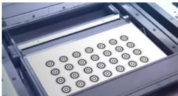
HP's Metal Jet system can produce high volumes of parts, with a Binder Jetting build size of 430 x 320 x 200 mm (Courtesy HP)
