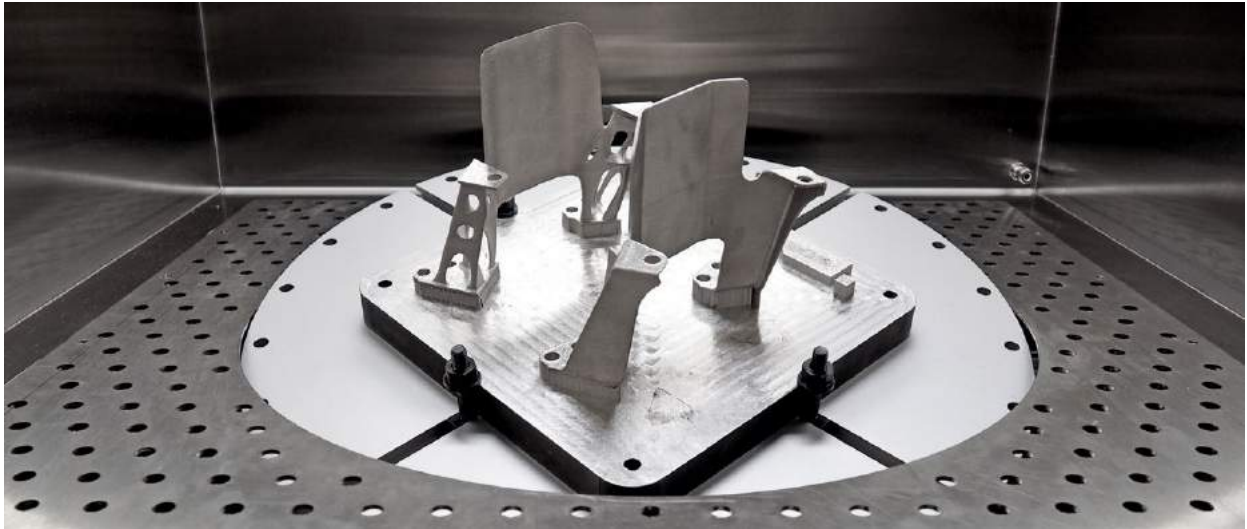
Fig. 2 Internal view of PowderShield system (Courtesy of Inert Corporation)
