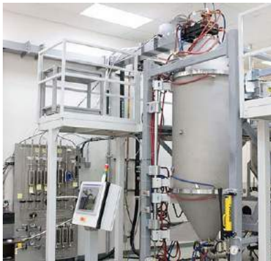
Amastan uses advanced microwave based plasma systems capable of manufacturing a broad array of materials for the advanced materials markets [Courtesy Amastan]
