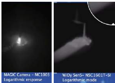
Screen images highlighting the improved definition seen using short-wave infrared imaging (Courtesy NIT)
