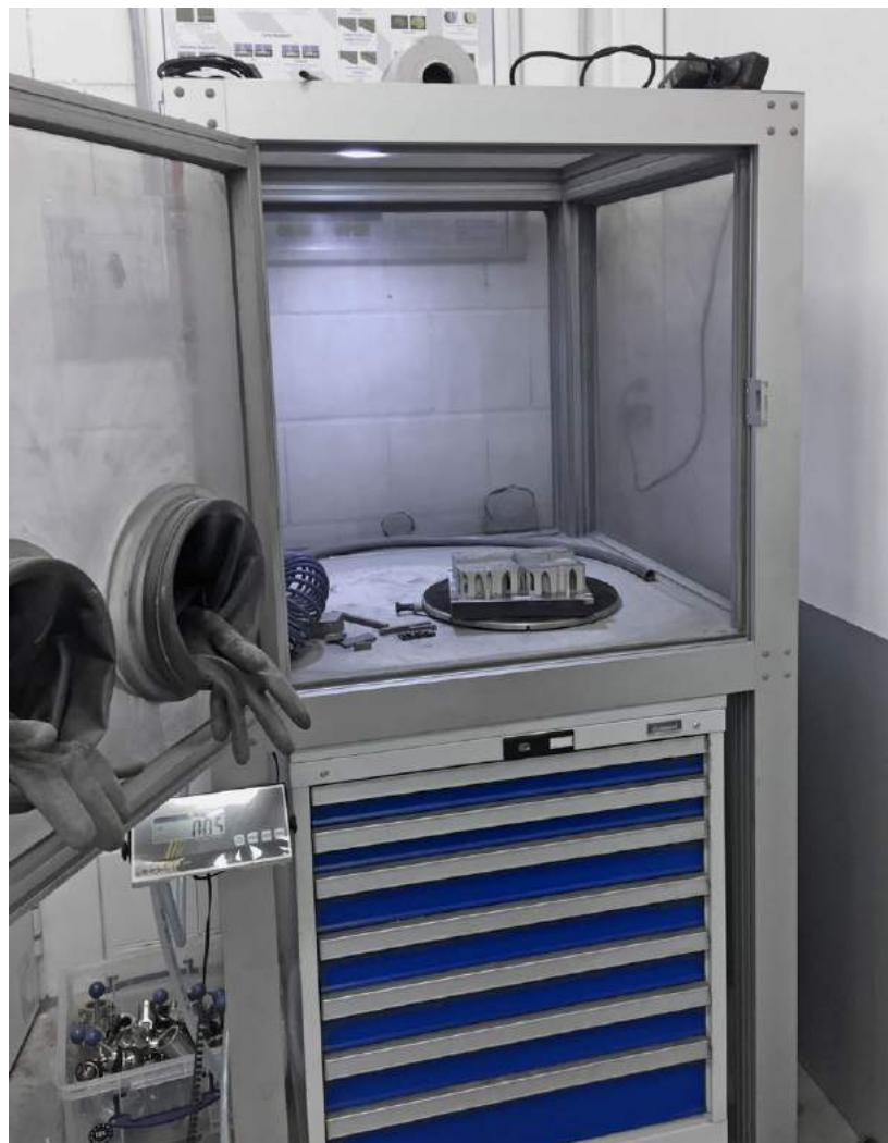
Fig. 5 Manual depowdering cabin at Voestalpine prior to replacement with automated depowdering system (Courtesy of Voestalpine)
