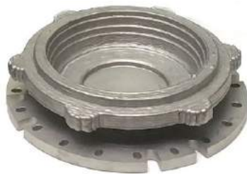
An additively manufactured wheel-set bearing cover for a Class 294 locomotive, produced on a Gefertec arc605 system at Rolf Lenk (Courtesy Deutsche Bahn)
