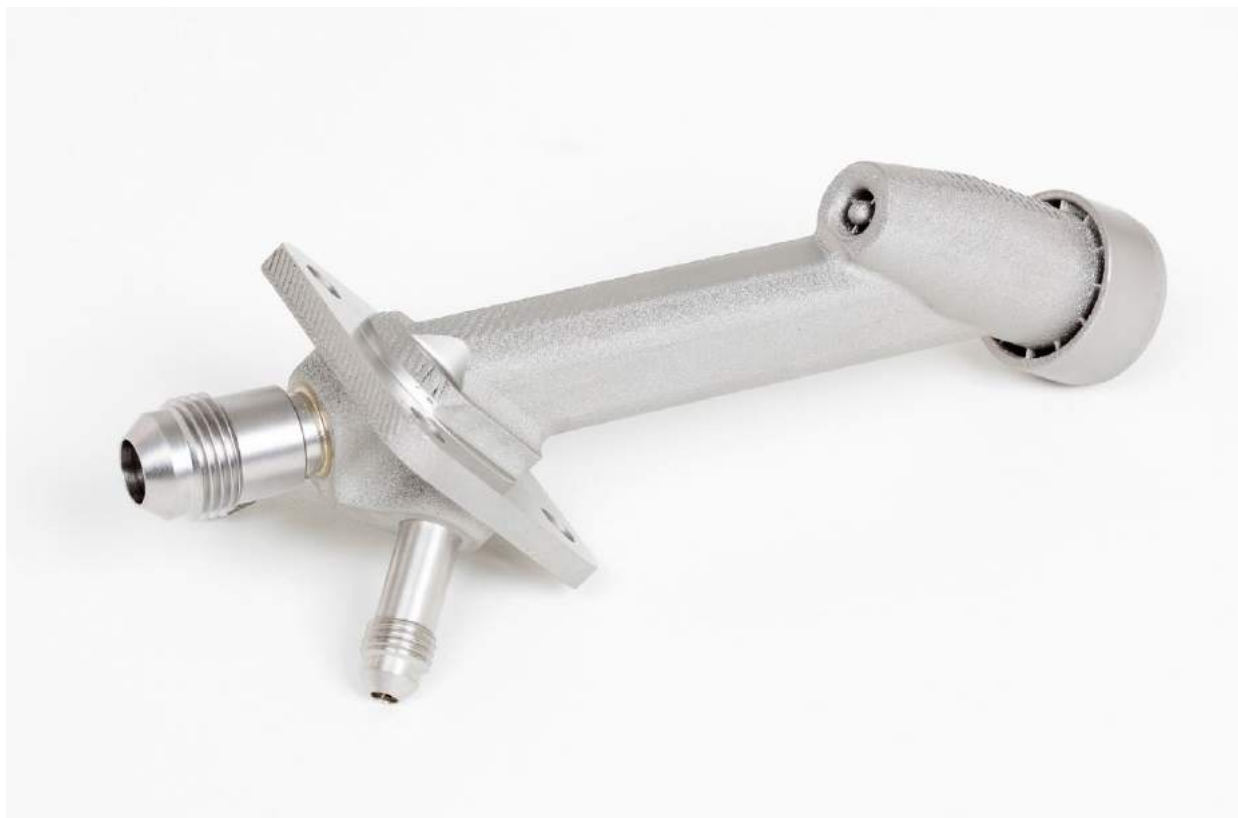
Fig. 3 This fully additively manufactured fuel nozzle for land-based industrial gas turbines for power generation applications was developed by Collins Aerospace. It is produced with just four components – compared with the seventeen components necessary for a legacy standard fuel injector shown in Fig. 4
