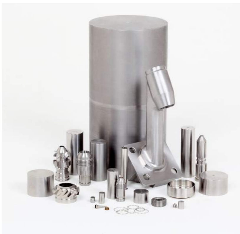
Fig. 4 The conventionally manufactured fuel nozzle showing the volume of raw material required for its production
