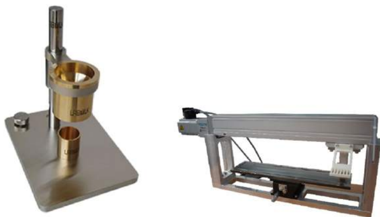
Fig. 5 Hall-Flowmeter and system for the simulation of the powder coating process for flowability control [2]
