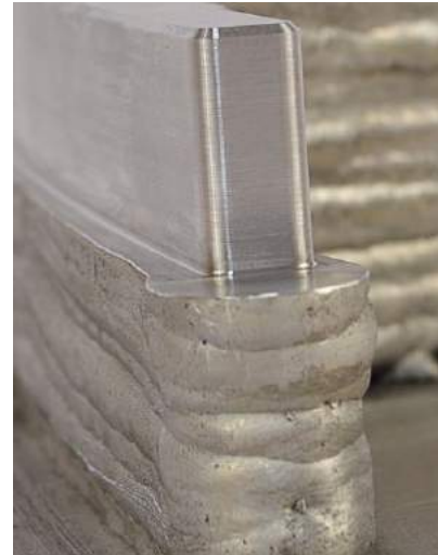
SBI uses a Wire-Arc AM process (Courtesy SBI International)
