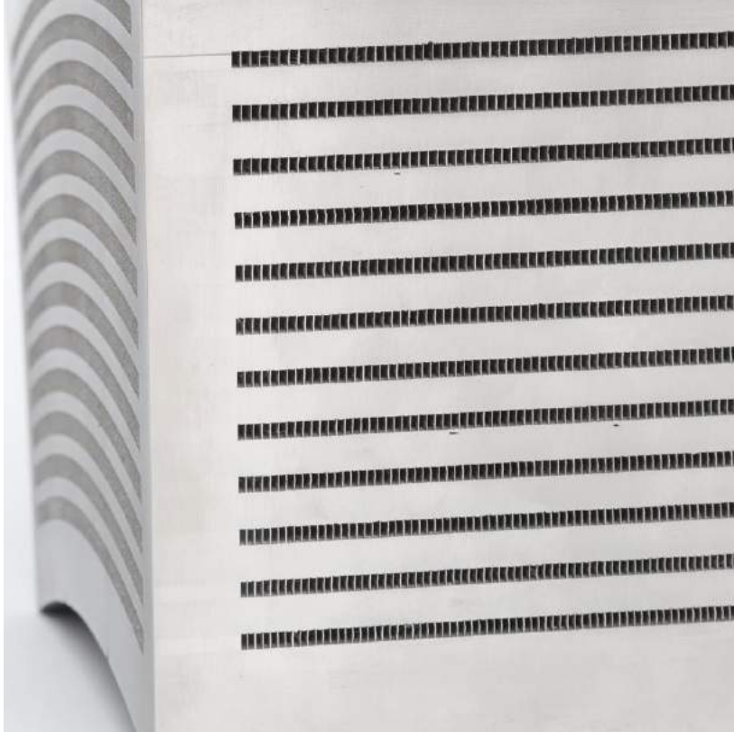
Fig. 11 Detail of the Inconel 625 alloy heat exchanger showing detail of the thin fins
