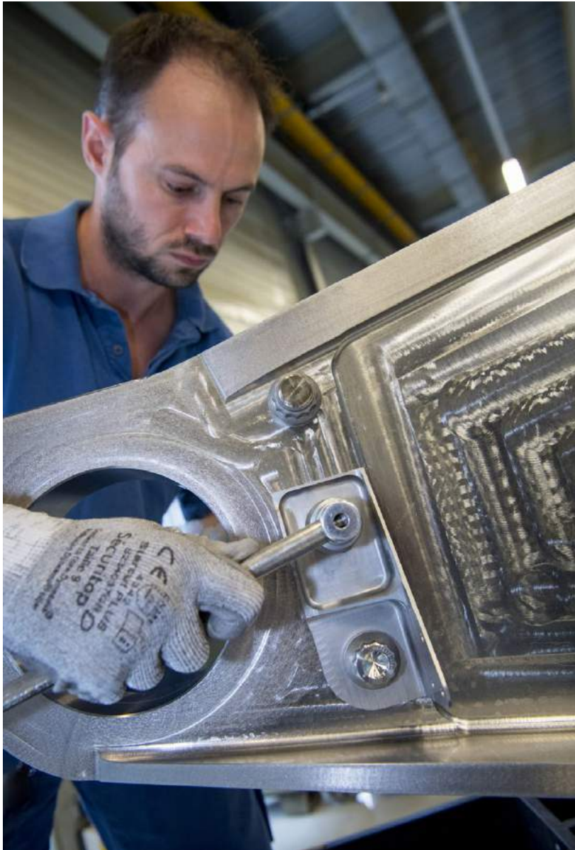
Fig. 2 Titanium alloy bracket produced using metal PBF being fitted to a section of the Airbus A350 jetliner [Courtesy Airbus]
