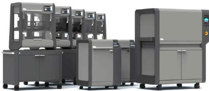
Desktop Metal's Studio System can be scaled to meet low-volume production of metal AM parts (Courtesy Desktop Metal)
