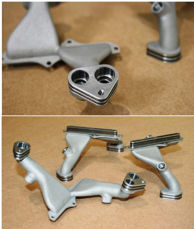
Fig. 7 Double water inlet/outlet produced for a Formula 1 car (Courtesy CA Models)
