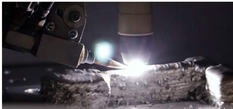
Production of an aluminium part using SBI International's M3DP WAAM machine (Courtesy SBI International)
