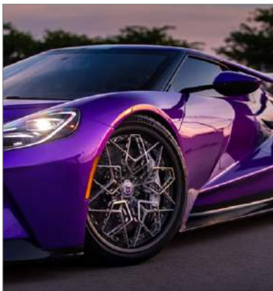
The second generation HRE3D+ wheel on a 2019 Ford GT (left), the build-plate (centre) and the finished wheel (right) [Courtesy HRE Performance Wheels]
