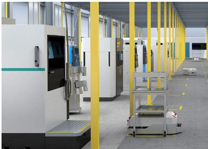
Fig. 7 A digital render of Materials Solutions' facility in Worcester, UK that includes three Solukon depowdering systems (Courtesy Material Solutions/Siemens)
