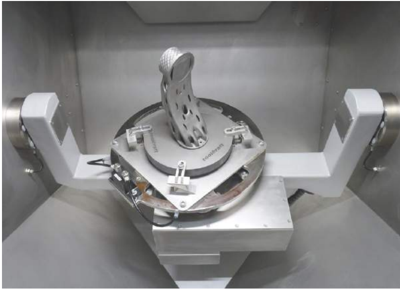
Fig. 6 Automated part cleaning at Toolcraft (left) and Solukon SFM-AT800-S system in operation at Toolcraft (right) (Courtesy of MBFZ toolcraft)
