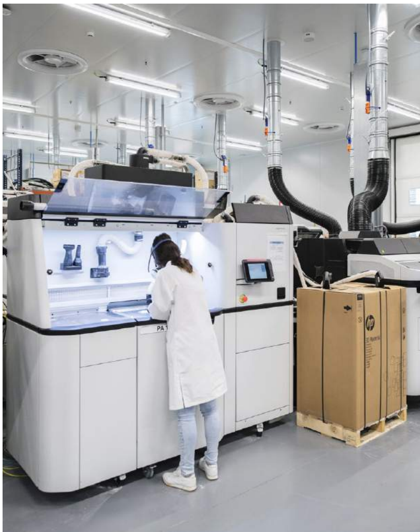
Fig. 4 A polymer AM system at HP Barcelona. The company uses the same printhead technology in every single printer it produces, enabling them to be produced quickly and at a low cost (Courtesy HP)
