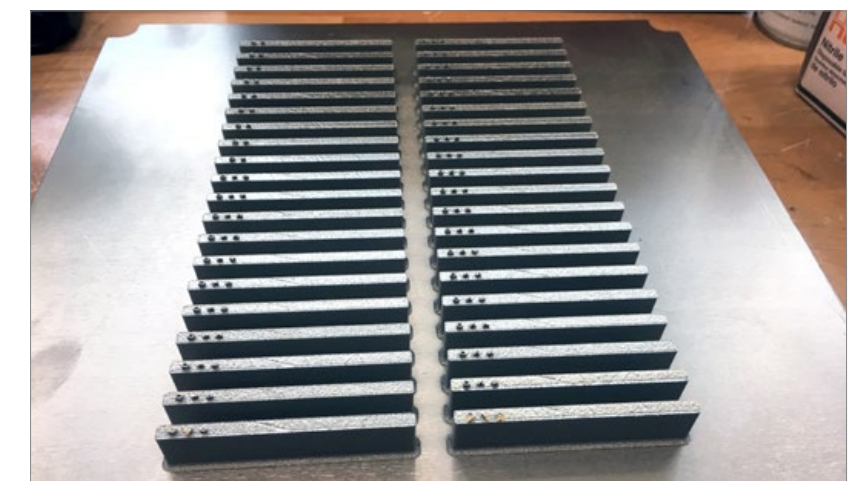
Fig. 1 Ti-6Al-4V (Ti64) specimens built on a Laser Powder Bed Fusion machine. The specimens were later tested and used as training data for Senvol's machine learning software
