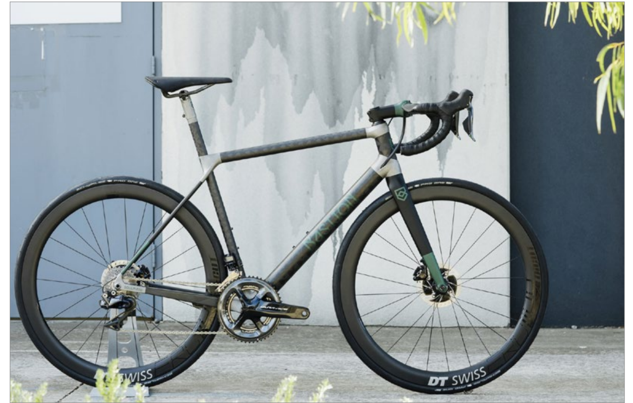
Fig. 8 A high-performance bicycle from Bastion Cycles, made from carbon fibre tubing and AM titanium lugs. The resulting product is a very high strength, lightweight bicycle that is perfectly tailored to each individual customer
