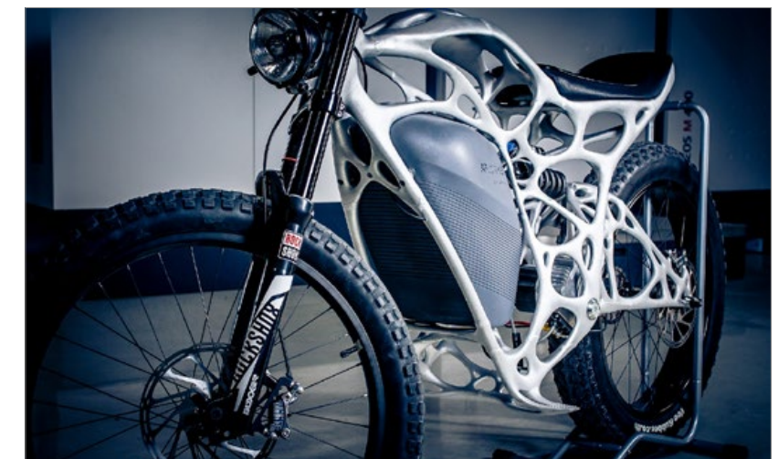
Fig. 1 This Light Rider electric motorcycle from APWORKS features an additively manufactured Scalmalloy frame
