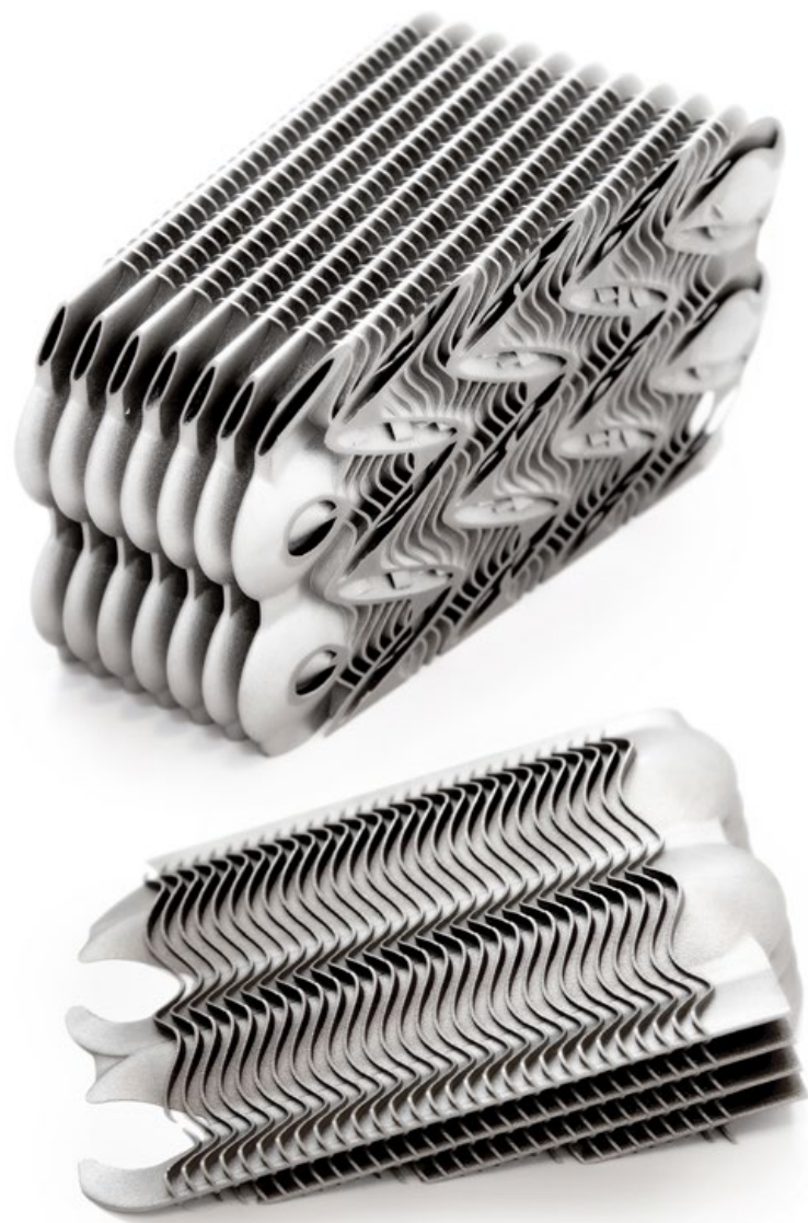
Fig. 5 This heat exchanger concept effectively demonstrates the complexity that can be achieved in metal AM part production
