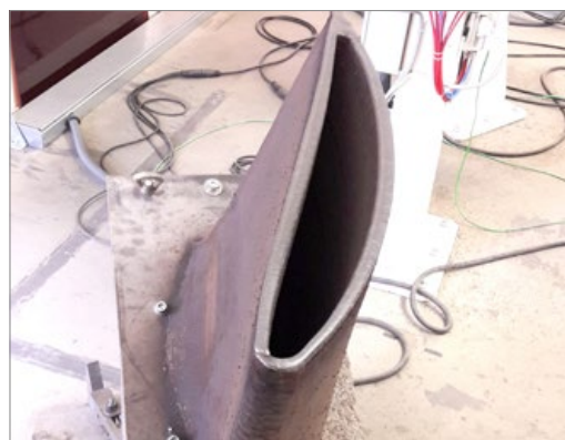
The hollow blade produced using WAAM (Courtesy Naval Group/Centrale Nantes)
