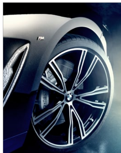
BMW used metal AM to produce the brake callipers for the one-off M850i Night Sky (Courtesy BMW M Automobiles)
