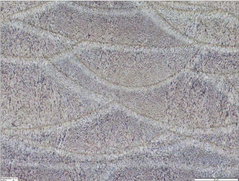
Fig. 12 Optical micrograph of as-built EOS F357 sample, showing melt pool lines crossing fine alternating aluminium-silicon cell structure. The growth direction of the lighter grey Al dendrites is revealed by elongated cells/grains in the vertical orientation. Scale bar is 20 µm. Etched with Groesbeck’s etch [4]
