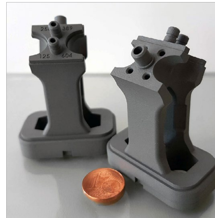
Fig. 3 Metallic green parts manufactured by LMM (Courtesy Lithoz)
