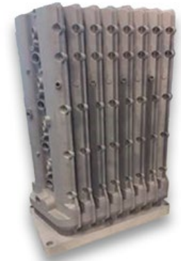
Prototype cylinder head covers [Courtesy SLM Solutions Group AG]
