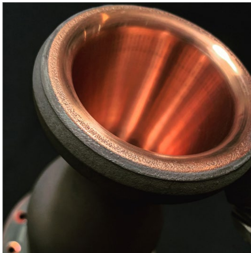
Fig. 7 View of the inside of the E1 rocket chamber after polishing. It should be noted that this component has a large number of complex internal features
