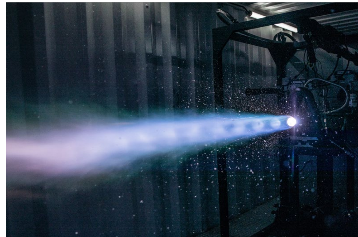
Fig. 9 The AM copper alloy rocket engine under test. This liquid oxygen (Lox) regeneratively cooled engine is, states Launcher, now proven as part of its quest to build its next, larger engine, the E-2
