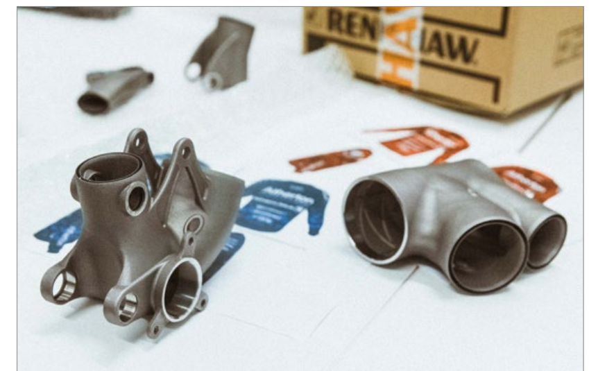
Titanium lugs, produced on a Renishaw 500Q, will join the carbon fibre tubing of the bike frame (Courtesy Renishaw)
