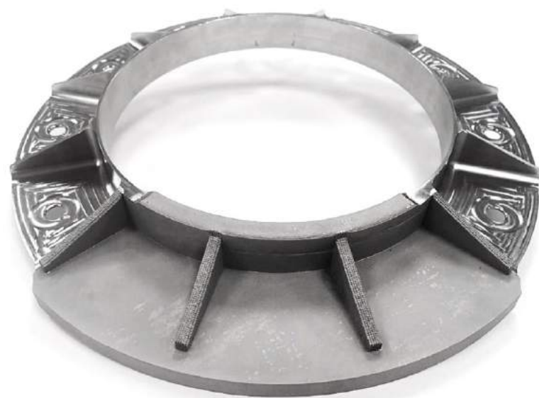
Aerospace flange in Ti6Al4V. Built using DED, heat treated and partially machined (Courtesy BeAM)
