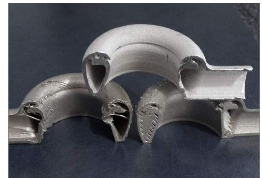
Fig. 1 Sections of circular nozzles, upper part by Binder Jetting without support structures; lower parts by LB-PBF with varying amounts of internal support structures
