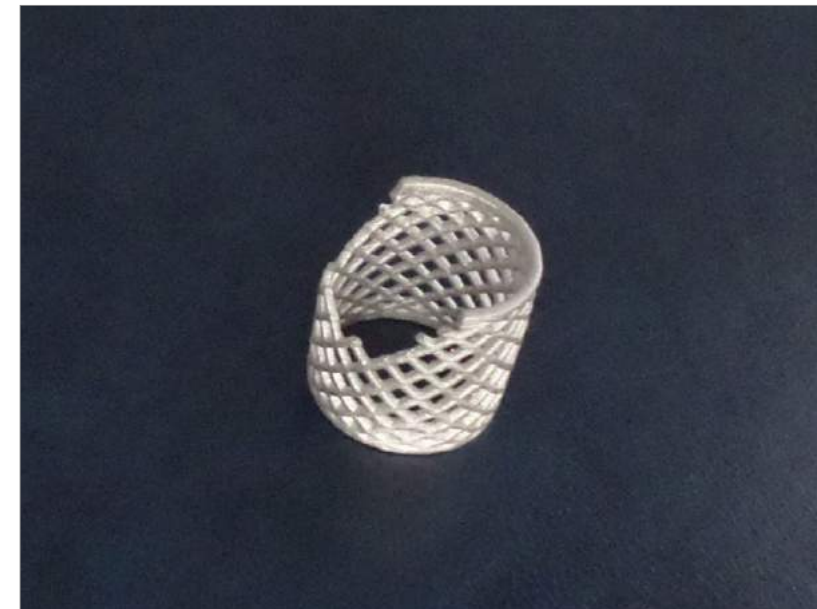
Fig. 6 Sintered part, broken during depowdering due to low green part strength
