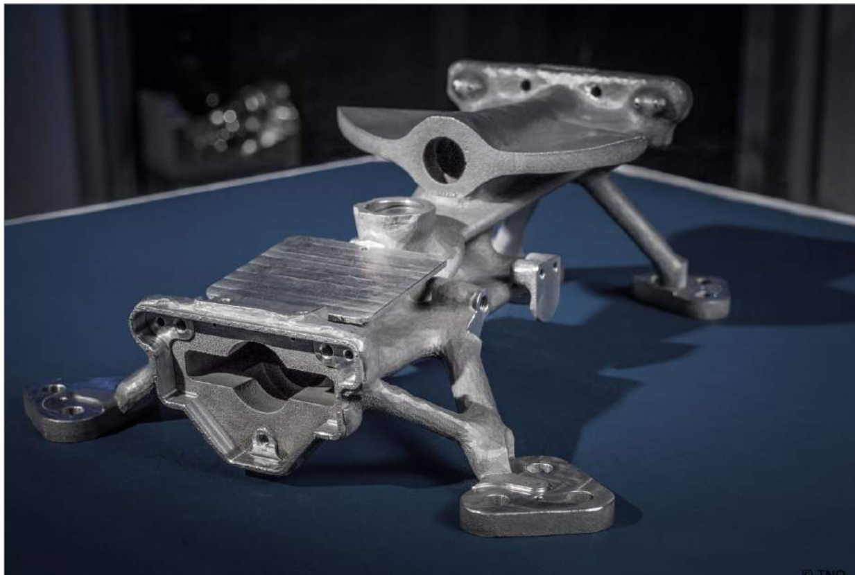
Fig. 4 Tim Domagala, Materialise, Belgium, presented a case study on the AM of parts for a two-mirror telescope used on satellites (Image ©TNO)
