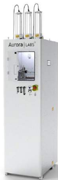
The Aurora Labs S-Titanium Pro has three modes – Selective Laser Melting, Selective Laser Sintering and Directed Energy Deposition
