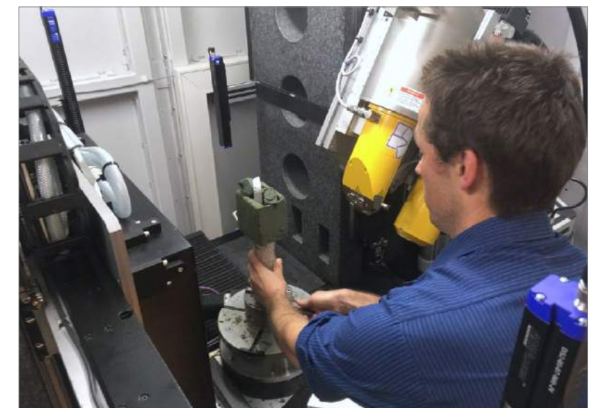
Fig. 1 A sample is mounted onto the turntable in the X-Ray CT scanner at Stellenbosch University's CT facility
