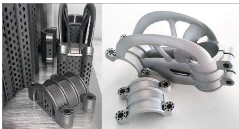
Fig. 7 Parts still attached to build platform with support material (left), and parts after post-processing and shot-peening (right)
