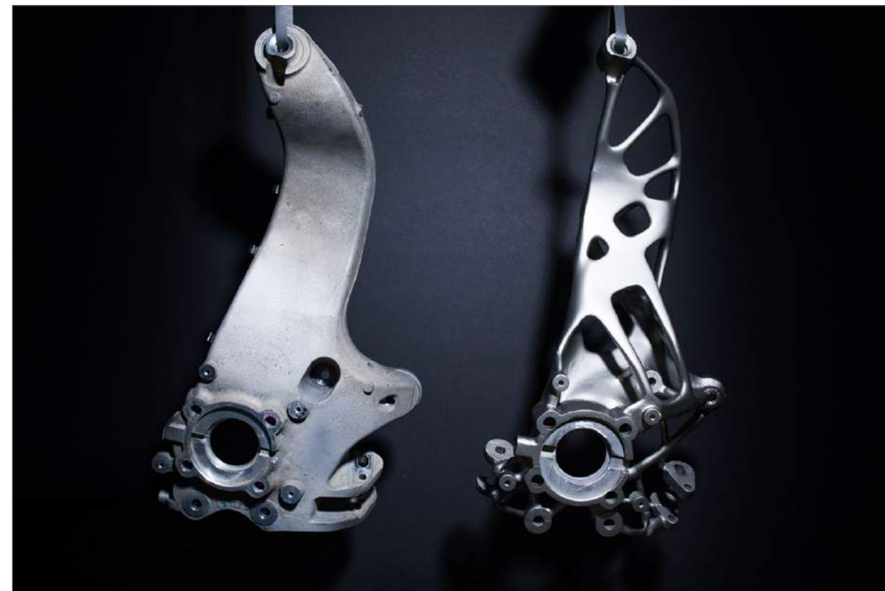
Fig. 11 A conventional Mini Cooper suspension trailing arm (left) and optimised one weighing 48% less, designed in ParaMatters (Courtesy ParaMatters, Techniplas and XponentialWorks)
