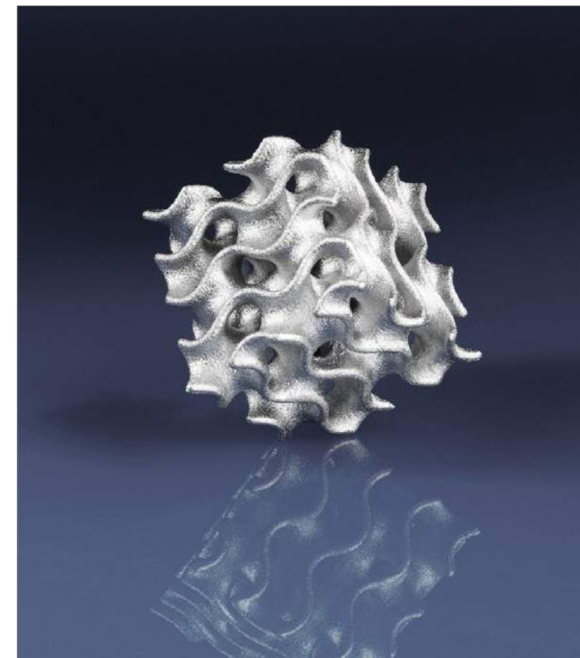
Fig. 8 Gyroid structure made of 316L via Binder Jetting
