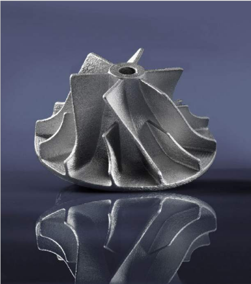
Fig. 4 Turbine wheel made of 316L via binder jetting
