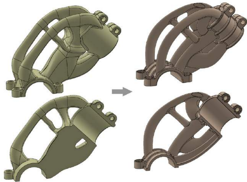
Fig. 6 Original topology-optimized bracket (left) and new bracket (right) with relatively even wall thicknesses in all locations. The new design weighs 53% less than the original bracket
