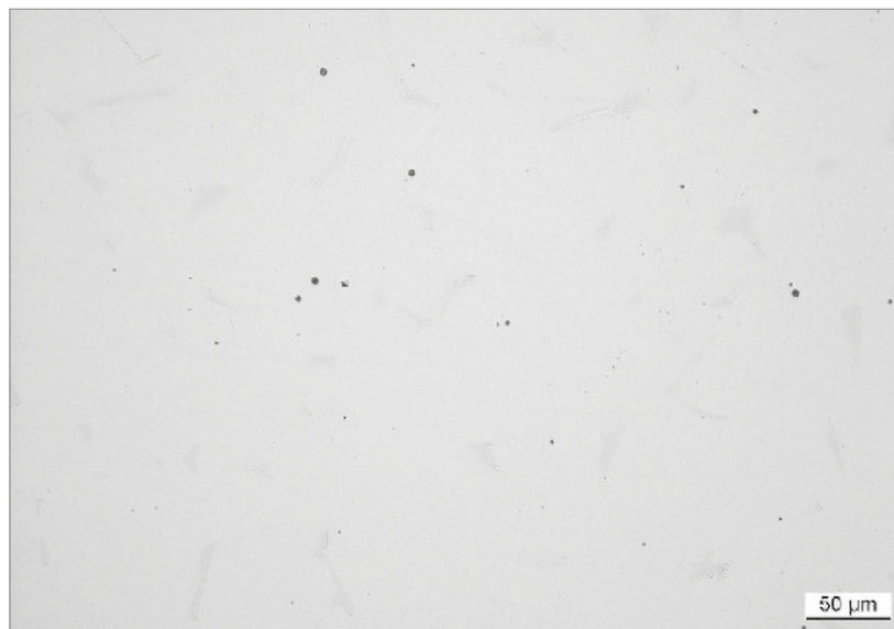
Fig. 7 Light microscopy image of a polished section of binder jetted and sintered 316L
