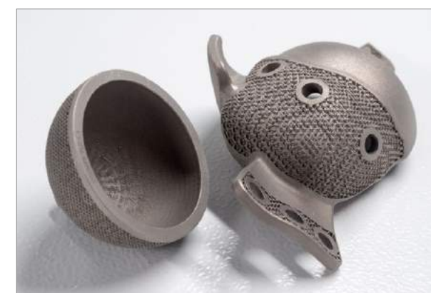
By heating the substrate plate, high-carbon steels or titanium alloys can be additively manufactured without cracking or severe warping
