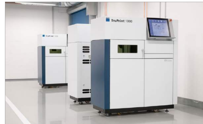
Conmet currently produces sixty implants a month with the TruPrint 1000 AM system, and compared to conventional machining methods the process saves 40% in production costs
