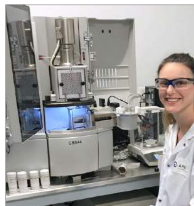
The final analysis to determine the content of carbon and sulphur within a metallic matrix, F357
