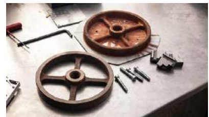
Components produced using SPEE3D's supersonic 3D deposition process (Courtesy SPEE3D)
