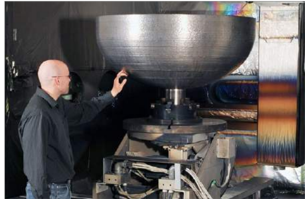
A Lockheed Martin engineer inspects one of the additively manufactured dome prototypes at the company's space facility in Denver. The final dome has a diameter of 116 cm (Courtesy Lockheed Martin)
