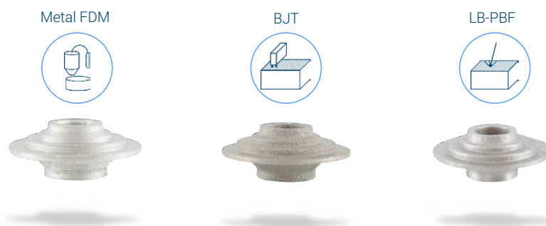
Fig. 1 The three major metal AM technologies for small-to medium size parts (Courtesy Ampower)
