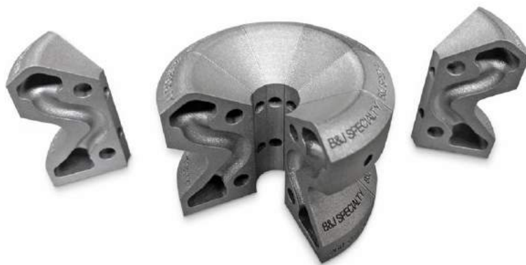
Fig. 1 Segments of a conformal cooling system manufactured by B&J Specialty on a 3D Systems ProX® DMP 300 Laser Powder Bed Fusion system
