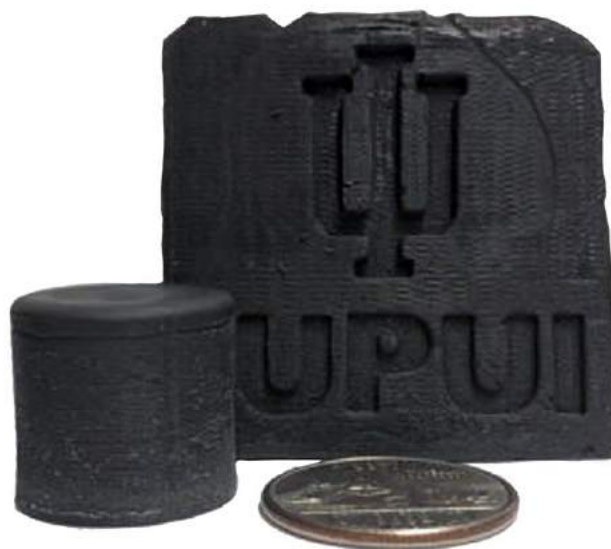
Fig. 9 Additively manufactured 17-4PH stainless steel samples [3]. The logo of IUPUI is shown on the plate sample
