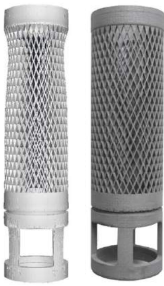
Fig. 6 Distortion compensated design from Ansys simulation results in the originally designed geometry when built
