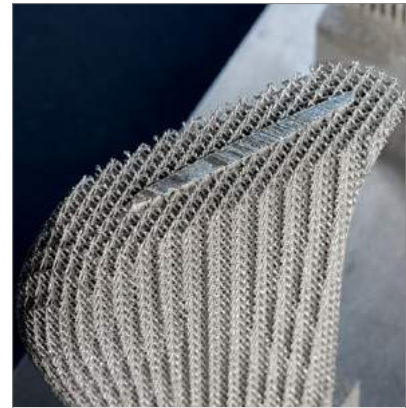
Fraunhofer IPT and ILT have developed a support structure design which is said to eliminate vibration during post-processing (Courtesy Fraunhofer IPT)
