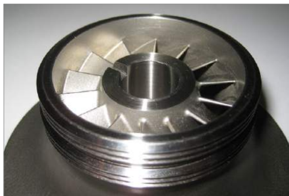
Following surface finishing using PostProcess's Hybrid DECI Duo solution, the impeller consistently passed aerodynamic tests (Courtesy PostProcess Technologies)
