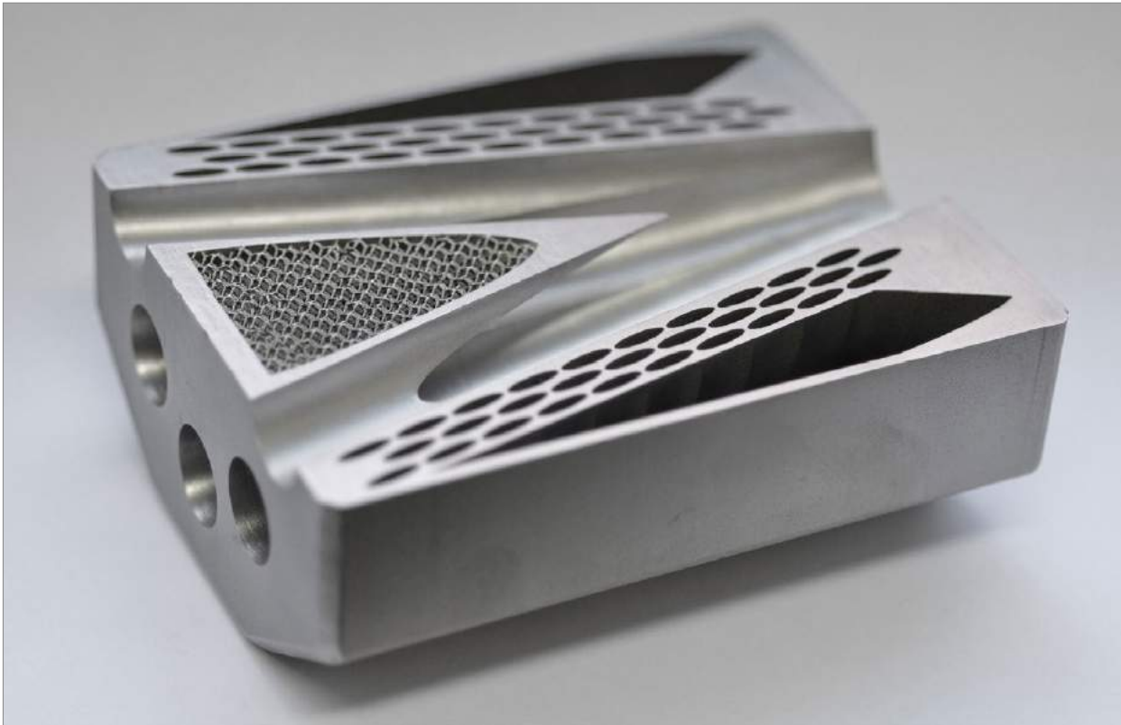
Fig. 4 A flow mixing part with conformal cooling channels. This example highlights why issues such as closed-loop water systems can be such an important factor (Couresty 3D Systems)
