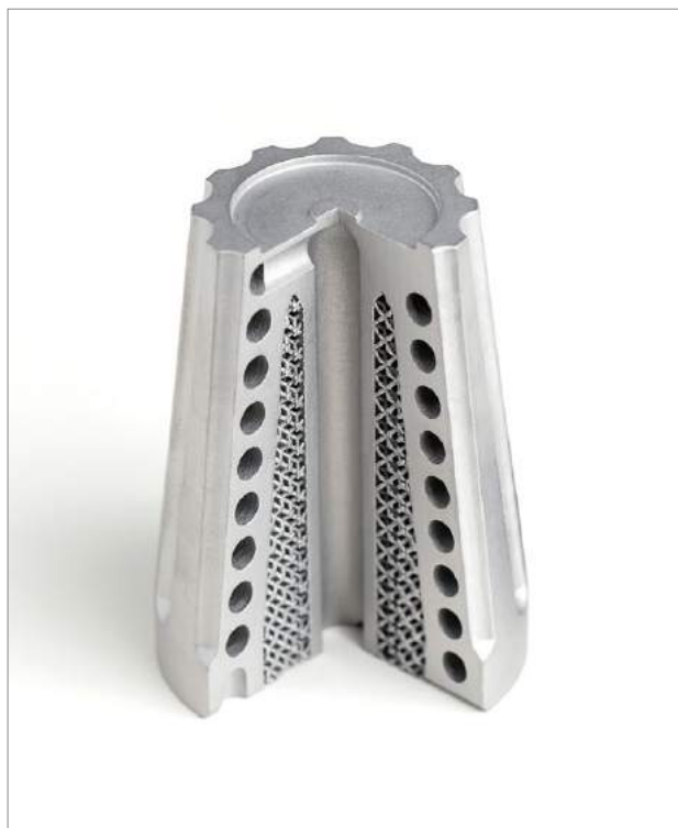
Fig. 4 A stainless steel mould insert produced on the BLT-A300 (Courtesy Bright Laser Technologies)
