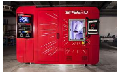
The SP3D machine fires metal powders onto a defined spot on a material carrier at 'three times the speed of sound' to produce components without melting or heat (Courtesy SPEE3D)
