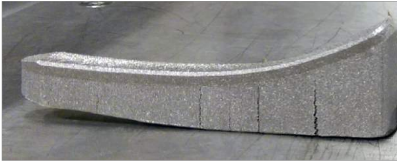
Fig. 2 Severe distortion in a collar bone implant after removal from the base plate. The distortion was severe enough that the implant could not be used on the patient (Courtesy the University of Pittsburgh)
