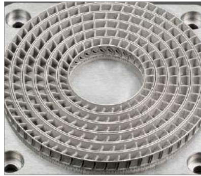
Multiple concentrically nested stator rings produced on the DMP Flex 100 system (Courtesy 3D Systems)
