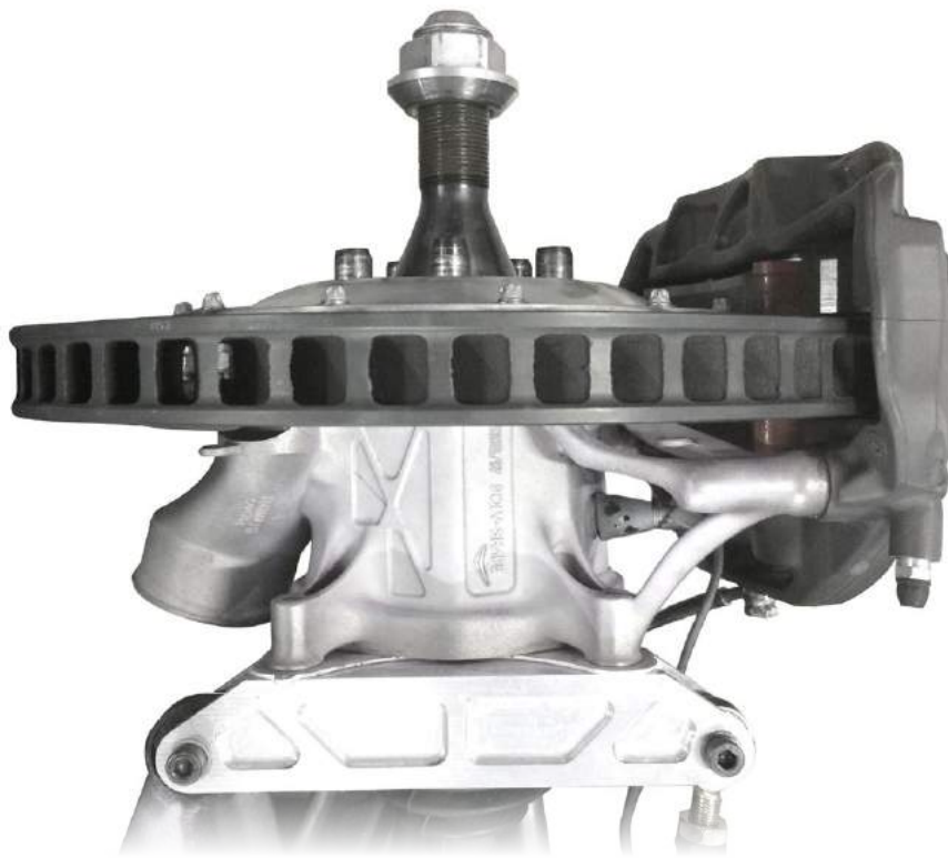
Fig. 3 The redesigned upright for the Norma MXX RD Limited was produced in Ti-Al-6V on an EOS M290 machine (Courtesy Poly-Shape)
