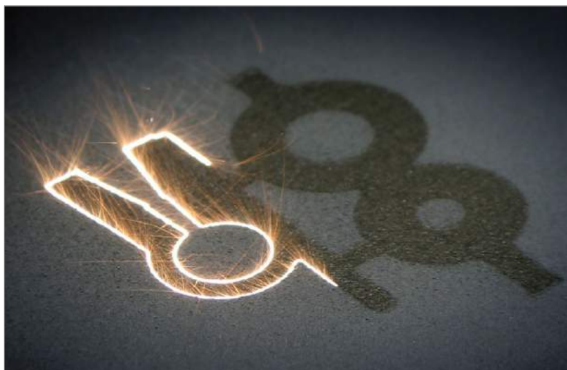
Fig. 1 The laser melting process in a Renishaw AM400 build chamber
