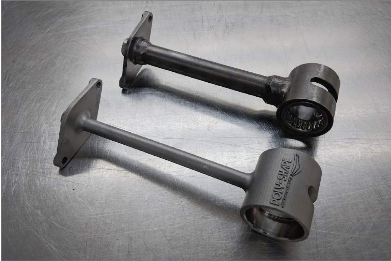
Fig. 8 The original Dallara anti-roll bar stem (top) and Poly-Shape's additively manufactured stem (bottom) (Courtesy Poly-Shape)
