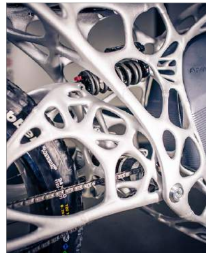
APWorks developed the Light Rider electric motorcycle, with its frame additively manufactured from Scalmalloy® aluminium alloy
