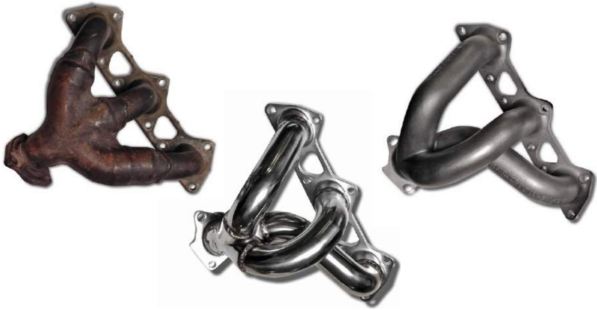
Fig. 10 The original exhaust collector, 3.13 kg (left), the SCART aftermarket collector, 2.45 kg (middle) and the final part produced by Poly-Shape, 2.3 kg (right)
