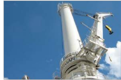
A 400 mt offshore mast crane aboard a subsea vessel (Courtesy Huisman Equipment)
