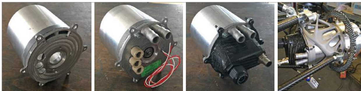
Fig. 4 Step-by-step assembly of the wheel-hub-drive (Courtesy Tufast Racing Team)
