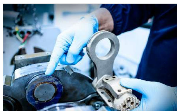
Fig. 1 Three components were chosen for initial benchmark testing: a saddle carrier, swing arm and connecting rod [Courtesy Desktop Metal]
