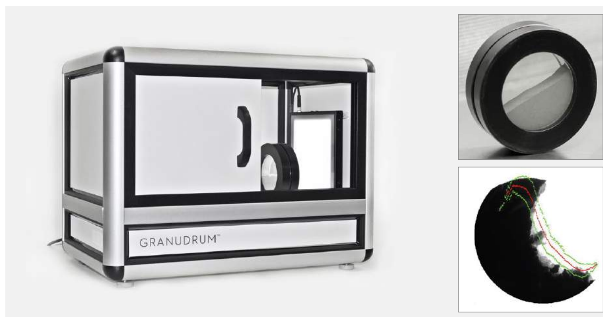
Fig. 8 The Granudrum works on the rotating drum measurement principle, associated with a customised image treatment algorithm (Courtesy Granutools)
