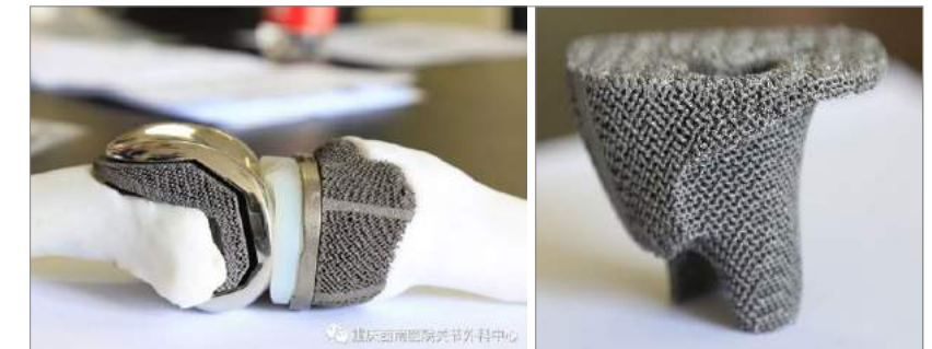
The custom, lattice-structured tantalum knee support component was produced for a knee surgery on an 83 year old patient (Courtesy Xi'an Sailong)
