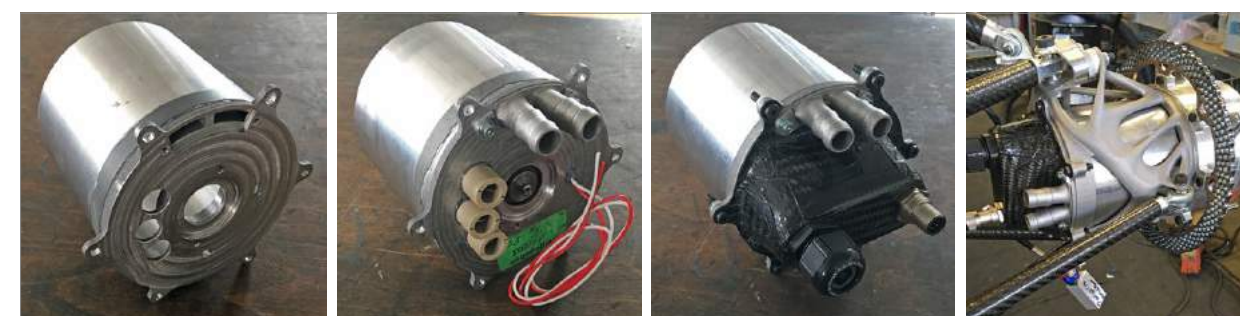
Fig. 4 Step-by-step assembly of the wheel-hub-drive (Courtesy TUfast Racing Team)
