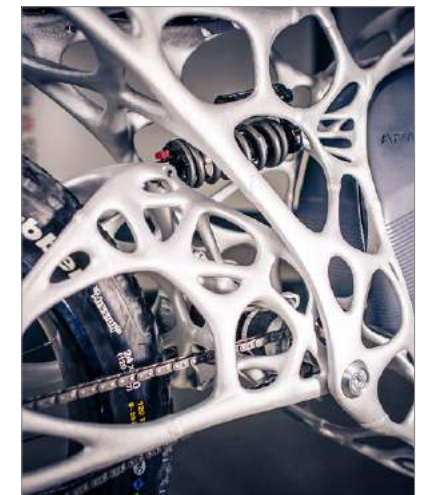
APWorks developed the Light Rider electric motorcycle, with its frame additively manufactured from Scalmalloy® aluminium alloy
