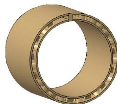
Fig. 3 The cooling structure has integrated cooling channels (Courtesy TUfast Racing Team)
