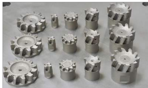
Multiple cutter parts are produced on a single build plate (Image Courtesy Komet Group)
