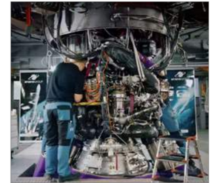
The Vulcain 2.1 engine incorporates a metal AM gas generator and is designed to power the main stage of the Ariane 6 launcher (Courtesy ArianeGroup)
