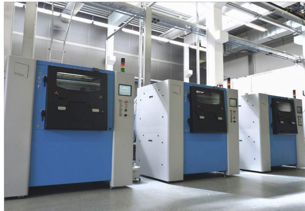
Fig. 3 Solukon SFM-AT800 depowdering systems at FKM Sintertechnik GmbH, Biedenkopf, Germany (Courtesy Solukon Maschinenbau GmbH)
