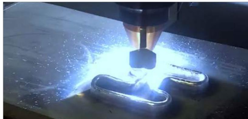
3D-Hybrid's Wire-Arc tool offers build speeds of more than 35 in 3 /min and can be used with a number of materials including aluminium alloys, stainless steel alloys and nickel-based super alloys (Courtesy 3D-Hybrid)
