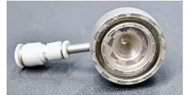
The final metal additively manufactured oil header (Courtesy GE Additive)
