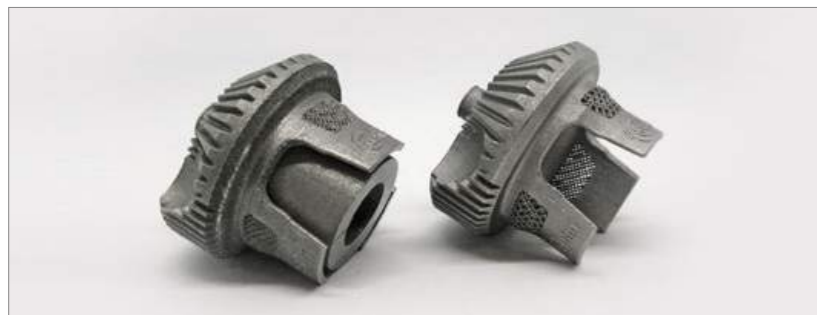
Fig. 5 The accuracy of a Digital Metal part (right) compared to an SLM part (left) (Courtesy CETIM)
