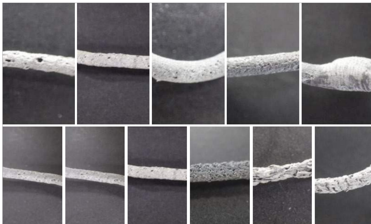
Fig. 16 Parameter testing with filament extruder setup for filament F1 and a nozzle of 0.8 mm. Top image: T = 250^\circ\text{C} , Extrusion Speeds from left to right: 7 mm/s [0.88 mm 3 /s], 14 mm/s [1.76 mm 3 /s], 42 mm/s [5.3 mm 3 /s], 70 mm/s [8.8 mm 3 /s], 98 mm/s [12.37 mm 3 /s]. Bottom image: 14 mm/s extrusion speed, temperatures extruded at 14 mm/s from left to right: 225°C, 235°C, 250°C, 270°C, 280°C, 290°C [3]
