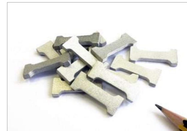
Fig. 5 Sintered tensile test specimen made from 316L stainless steel [1]
