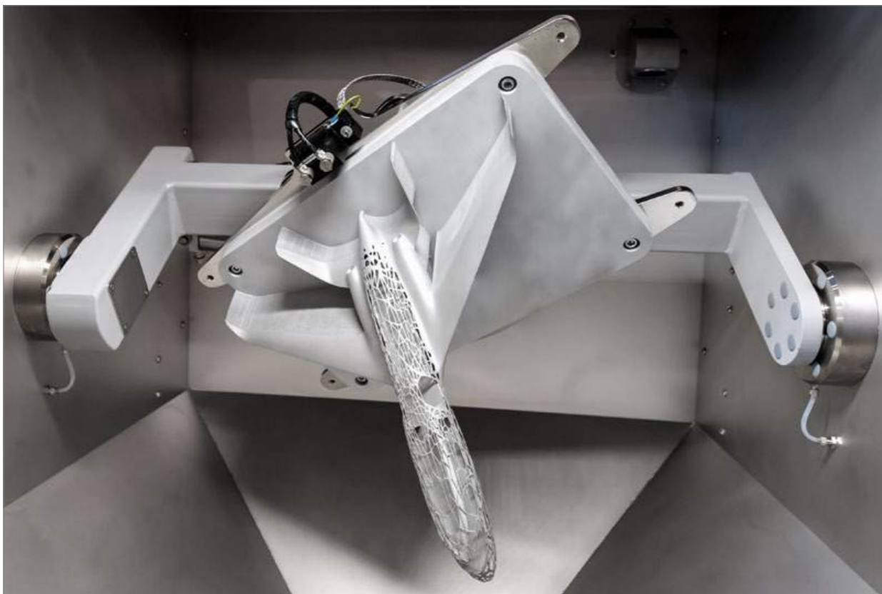
Fig. 4 Internal view of the Solukon SFM-AT800 system. Part designed by Airbus Operations GmbH and produced by Robert Hofmann GmbH (Courtesy Solukon Maschinenbau GmbH)
