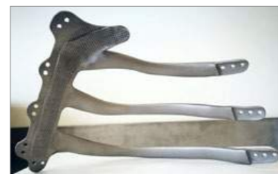
Using metal AM, the surgical team was able to produce a titanium implant to the patient's exact fit and specifications (Courtesy NHS Wales)
