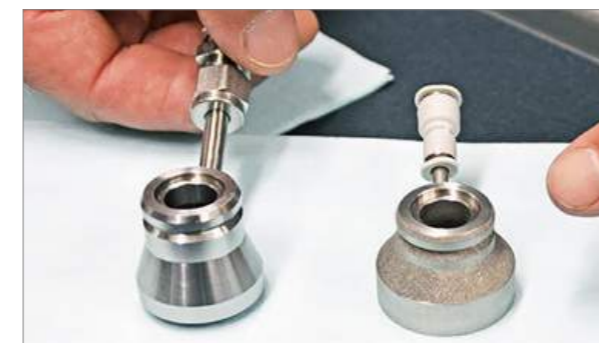
By re-engineering an oil header for AM, Concept Laser reduced the component from two parts to one (Courtesy GE Additive)
