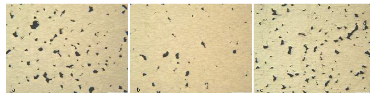
Fig. 12 Photomicrographs of Segment 11 (a) Part 2, 5.3% Porosity, (b) Part 5, 1.58% Porosity, and (c) Part 8, 4.77% Porosity.
