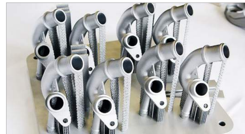
VW is already using on demand AM to make rarely needed water connectors for the Audi W12 engine (Courtesy VW Group)
