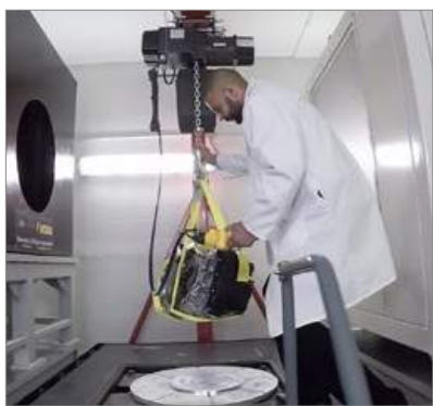
The system pairs a 3 MeV cone-beam X-ray source with a large format 2k x 2k flat panel digital detector
