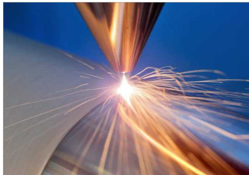
Laser material deposition is used in a variety of areas, including tool repair and the application of anti-corrosion coatings (Courtesy Fraunhofer ILT)
