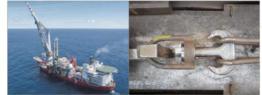
A typical offshore crane aboard a subsea vessel (left), additively manufactured crane hook under load test (right) (Courtesy Huisman Equipment)
