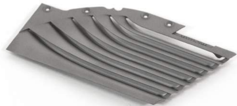
Fig. 7 Rear wing endplate louvre manufactured at 60% for the F1 wind tunnel model, material AlSi10Mg
