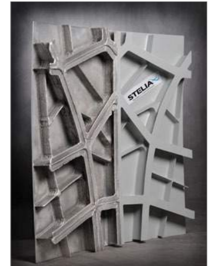
STELIA Aerospace's 1 m 2 aluminium WAAM demonstrator part (Courtesy STELIA Aerospace)
