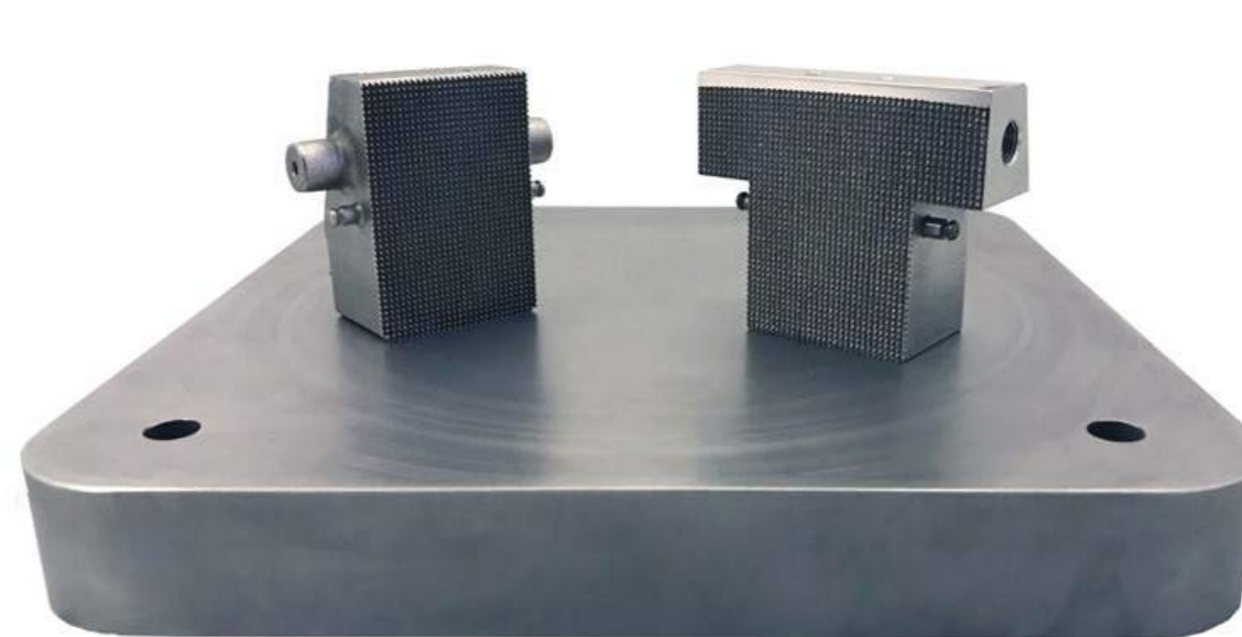
Fig. 3 Initial AM design (left) with 3.0 mm diameter triple loop interior channel; final AM design (right) with 5.0 mm diameter single loop interior channel
