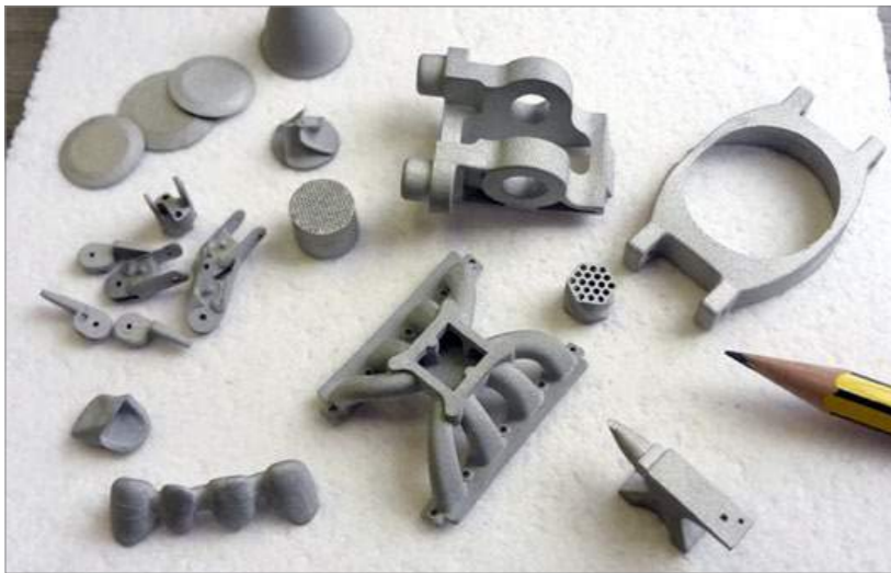
Fig. 7 Sintered parts made from 316L, according to the building platform shown in Fig. 3 [1]
