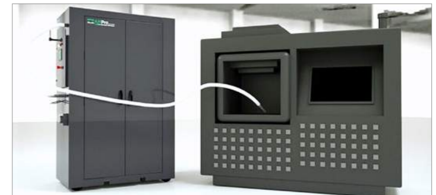
The Russell AMPro Sieve Station has a flexible design which makes it suitable for numerous powder handling tasks (Courtesy Russell Finex)
