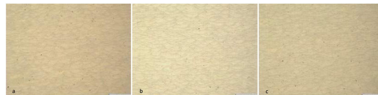
Fig. 10 Photomicrographs of segment 1 (a) part 2, 0.09% porosity, (b) part 5, 0.02% porosity, and (c) part 8, 0.07% porosity
