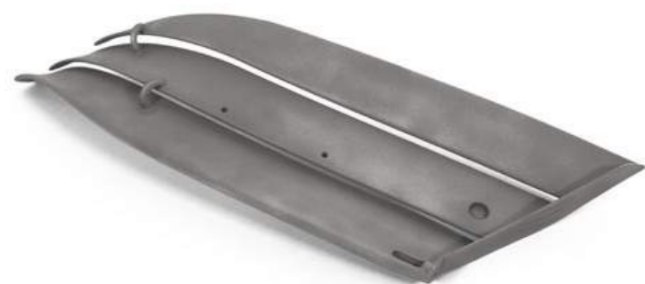
Fig. 8 A front wing flap manufactured at 60% for a wind tunnel model, material AlSi10Mg
