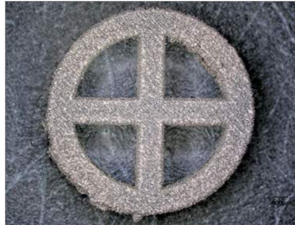
Synthetic nanodiamonds applied as a surface coating on a titanium scaffold may increase the biocompatibility of titanium AM implants (Courtesy RMIT University)
