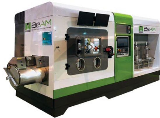
The Modulo 400 has a significantly reduced machine footprint compared to traditional DED systems
