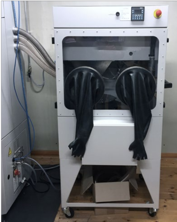
Fig. 2 A sieving station (Courtesy Olaf Diegel)
