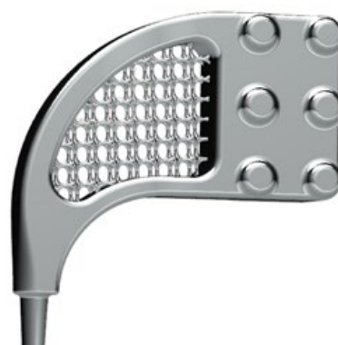
An example lattice structure created using the NX Lattice Structures Design module (Courtesy Siemens)
