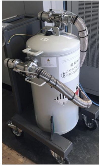
Fig. 8 A fume filter and collector (Courtesy Olaf Diegel)
