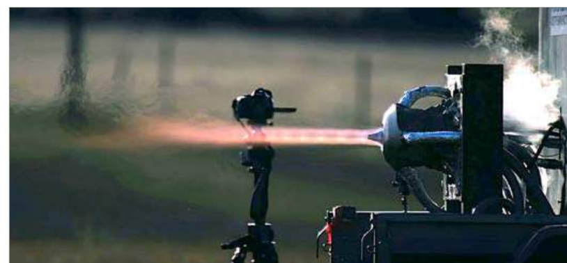
ProjectX engine during a test fire. The shock-cell structure in the rocket plume is visible [Courtesy NextAero]
