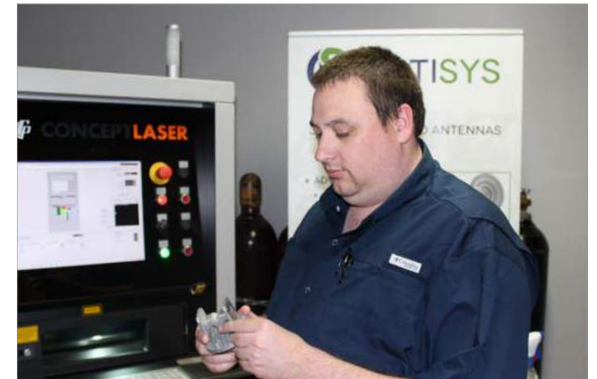
Fig. 6 Optisys CEO Clinton Cathey examines a microwave waveguide 'single-piece assembly' manufactured in the company's Concept Laser machine
