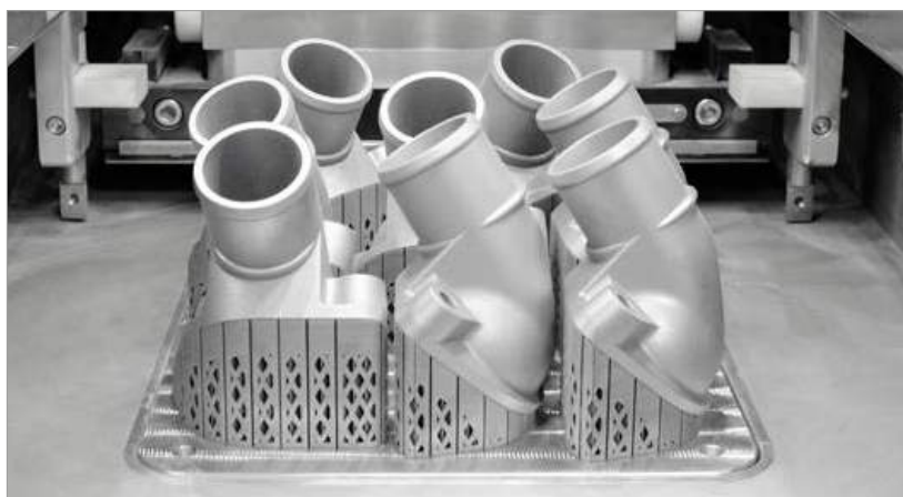
Mercedes-Benz Trucks' first metal AM spare part (Courtesy Daimler AG)
