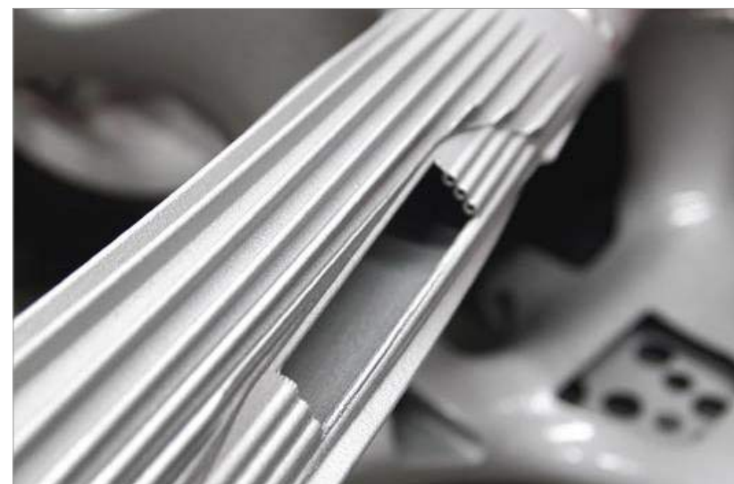
Fig. 3 Detail showing the complexity of the AM structure
