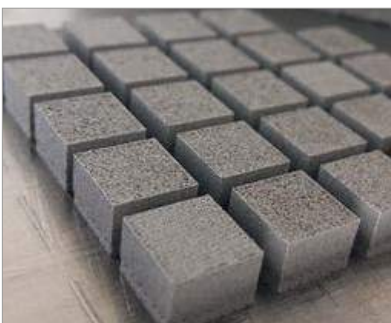
Fig. 1 Tungsten components manufactured by SLM (Courtesy Plansee)
