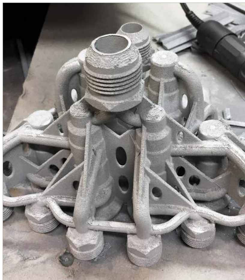
Fig. 3 The hydraulic manifold designed for metal AM with support structures removed
