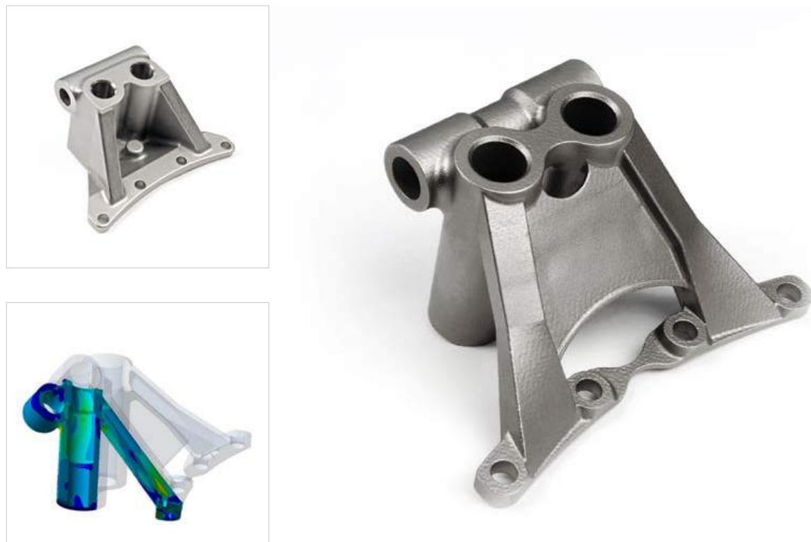
Fig. 9 A proof-of-concept Inconel 718 engine mount bracket. The original part (top left), topology optimised design (bottom left) and manufactured part using Laser Powder Bed Fusion (right). The process achieved a 56% weight reduction while maintaining desired strength
