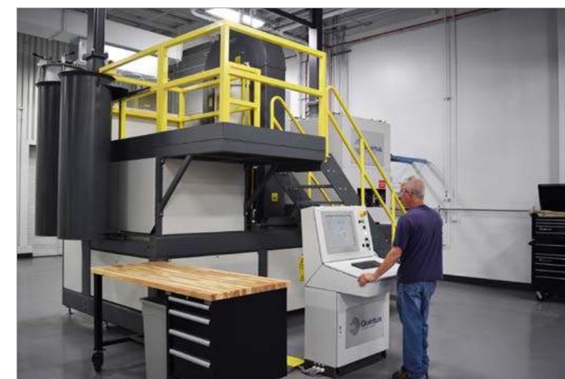
Fig. 16 A new Quintus HIP system for the final densification of AM parts
