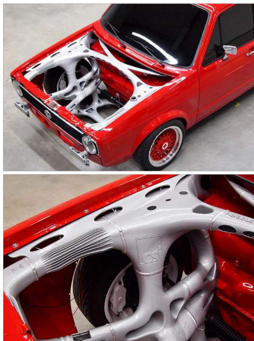
Fig. 1 The front-end structure of this VW Caddy has been completely redesigned using Additive Manufacturing
