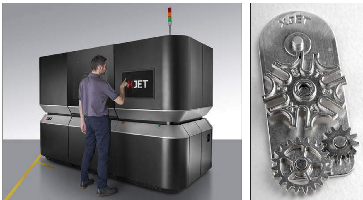
Fig. 5 An XJET machine and demonstration parts made from 316L stainless steel (Courtesy XJET)
