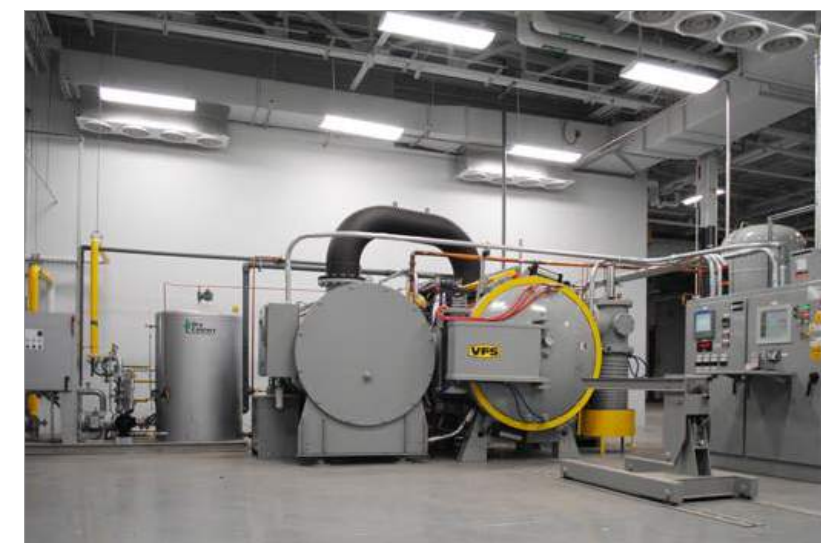
Fig. 17 A vacuum heat treatment furnace for the thermal processing of metal AM aerospace components
