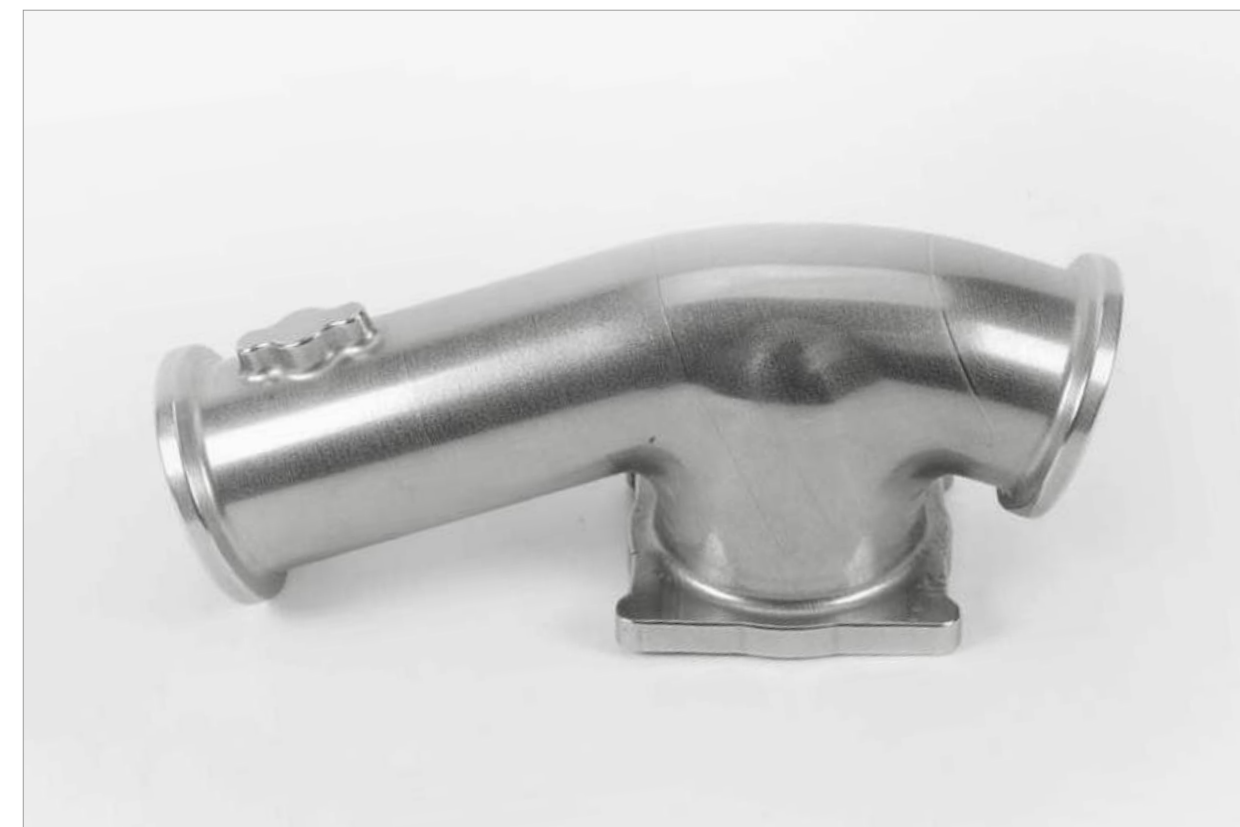
Fig. 7 Tubular parts are prime candidates for replacement with metal AM. This Inconel 718 part has completed certification at all three levels
