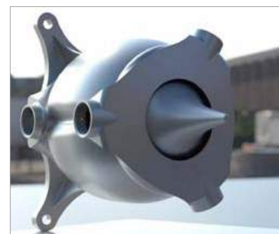
The ProjectX engine is built from high-strength nickel based superalloy Hasteloy X on an EOS M280 system [Courtesy NextAero]
