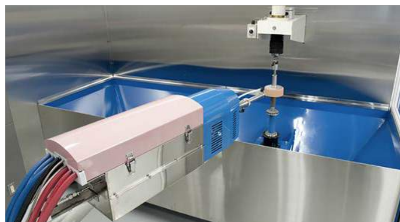
The TKF process applies titanium and titanium alloy powders onto a scaffold surface to rapidly produce titanium or titanium/composite products and parts (Courtesy Titomic)
