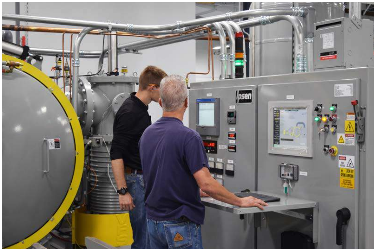
Fig. 12 Honeywell's new vacuum heat treatment system from Ipsen Industries
