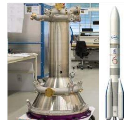
Vinci thrust chambers for the new Ariane 6 (Courtesy DLR)
