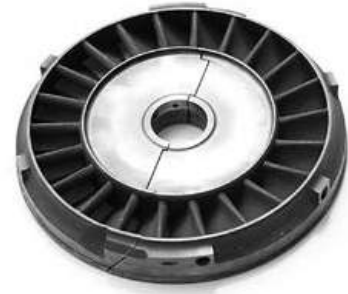
The turbine nozzle for the eAPU60 (Courtesy Safran Power Units – Astrid Desclos)
