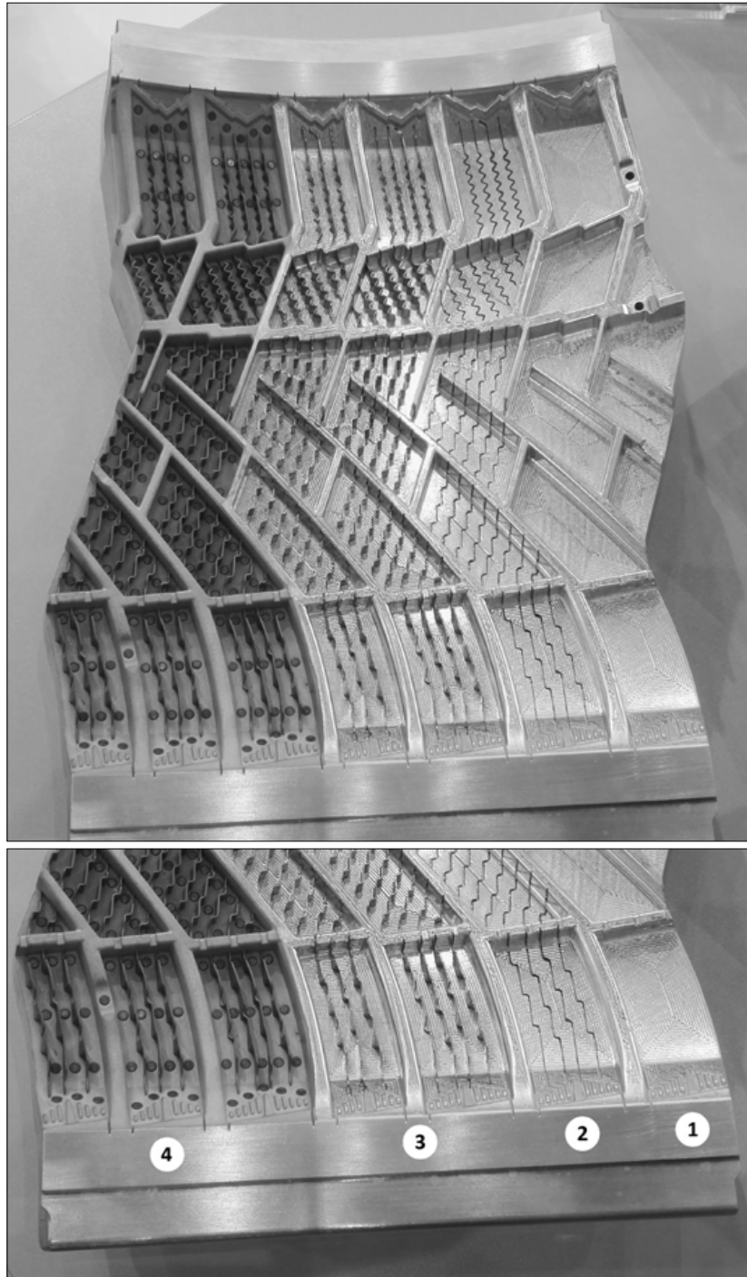
Fig. 3 A conventional tyre mould segment from Dahmen GmbH. The lower images demonstrates the mounting of steel sipes (from right to left): (1) milled raw profile, (2) slots to accommodate the sipes, (3) sipes inserted manually, (4) sipes fixed by laser beam welding
