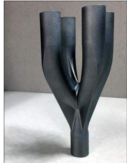
An example of an additively manufactured fluid delivery system produced by Canada Makes (Courtesy Canada Makes)
