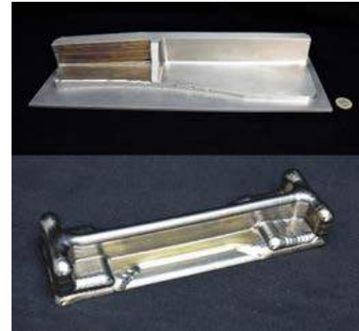
Example of AM and partially finish-machined titanium part (Courtesy Prodways)
