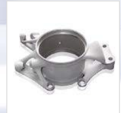
Knuckle made of EOS Aluminium AlSi10Mg: weight reduction of 660 g, increased rigidity. (Source: EOS / Rennteam Uni Stuttgart)
