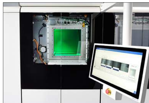
The build chamber on a MetalFAB1 machine (Courtesy Additive Industries)
