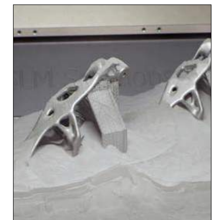
Part production at voestalpine's Additive Manufacturing Centre, Düsseldorf, Germany (Courtesy voestalpine)
