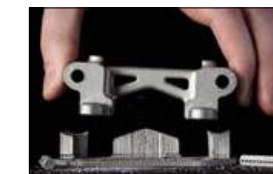
Cover image Desktop Metal's unique support structures use ceramic powder as the interface with the part surfaces (Courtesy Desktop Metal)
