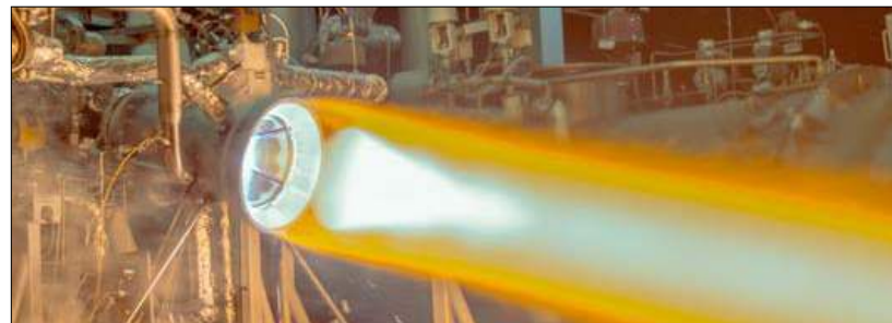
Aerojet Rocketdyne's full-scale, Additively Manufactured thrust chamber assembly in testing in West Palm Beach, Florida (Courtesy Aerojet Rocketdyne)
