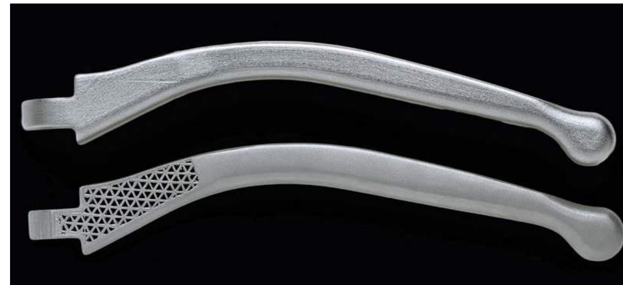
Fig. 4 Stainless steel brake levers manufactured using Markforged's Metal X system
