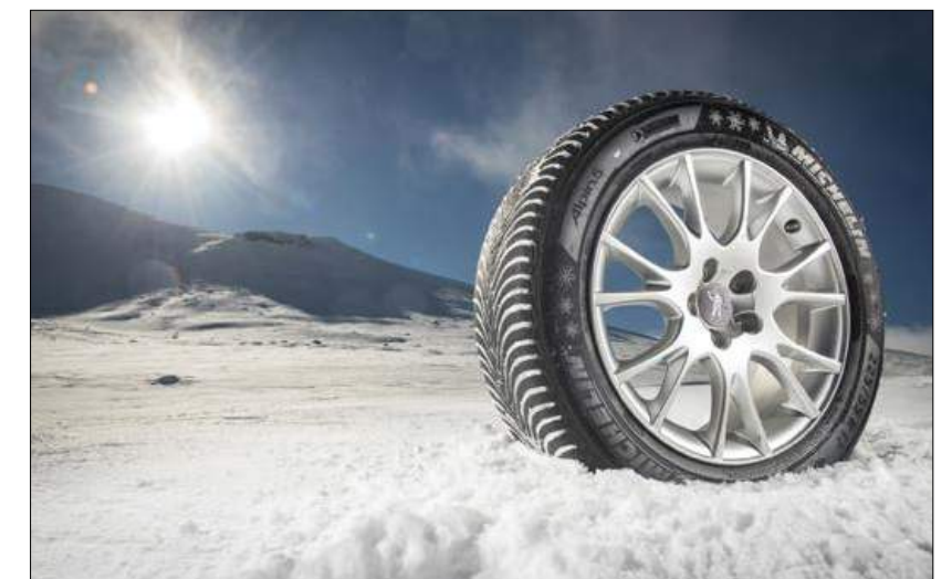
Fig. 1 The Michelin Alpin 5 winter passenger car tyre is siped to full tread depth, to better preserve the tyre's winter performance during the whole life of the tyre (Courtesy Michelin)
