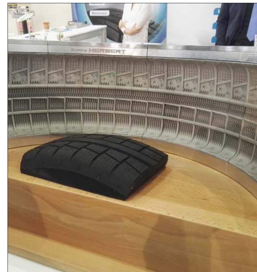
Fig. 5 Tyre mould with additively manufactured segments (Herbert)
