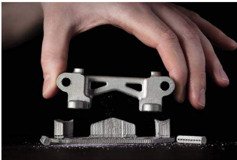
Fig. 2 Ceramic powder serves as the interface between the part surfaces and the support structures. Tapping the parts on a bench top and/or using a small ball-peen hammer is usually enough to remove the supports
