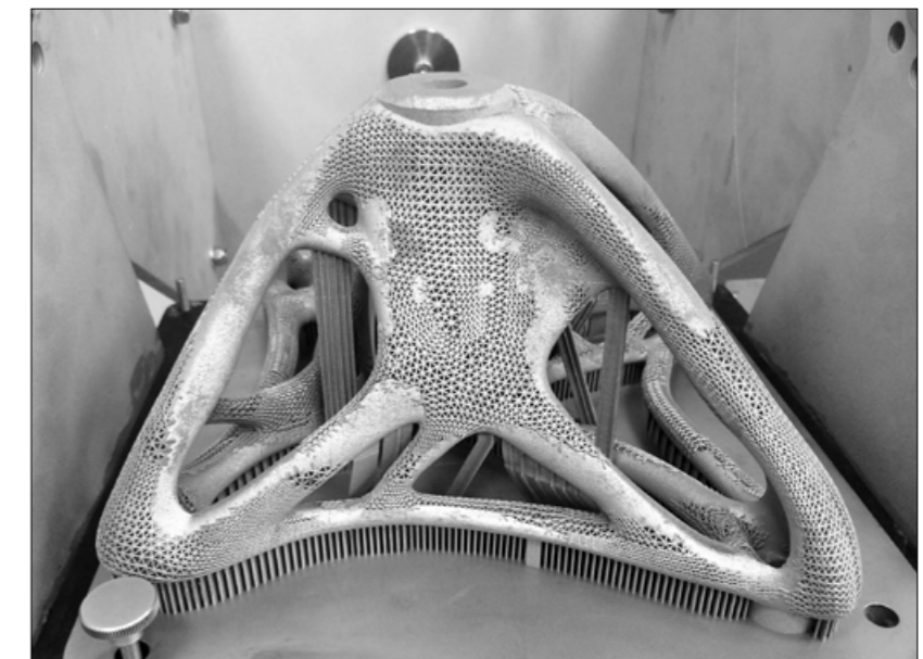
Fig. 13 Metal support structures generated with Materialise Magics (Courtesy Altair, Materialise and Renishaw)
