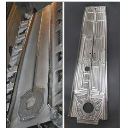
This photo highlights two different stages of an Airbus rear upper spar that was 3D printed in titanium with Sciaky's EBAM process. The image on the left shows the part in an early preform stage. The image on the right shows the finished part
