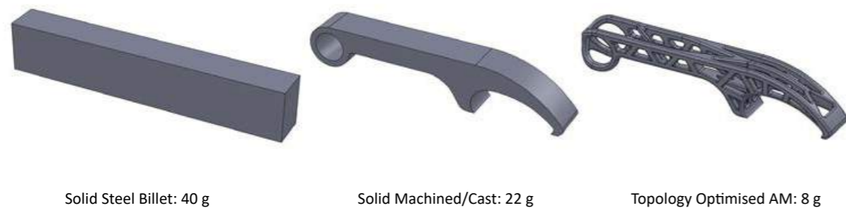
Fig. 3 Weight comparison between CNC machined and additively manufactured bottle openers
