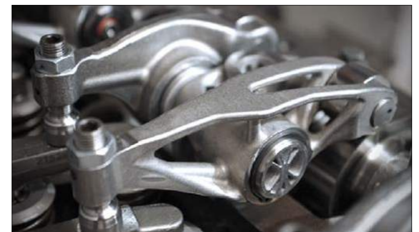
The re-designed metal AM version of the rocker arm is shown during a bench test inside a Euro 6 engine
