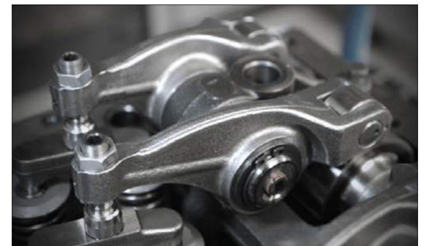
The original rocker arm in a Renault Trucks Euro 6 DTI 5 engine
