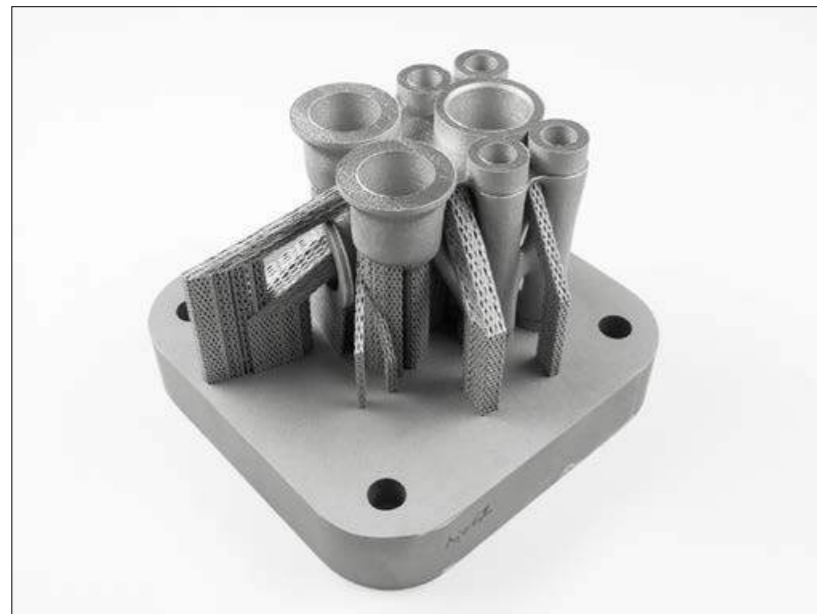
Fig. 6 This hydraulic valve by VTT and Nurmi Cylinders was anchored with angled support structures
