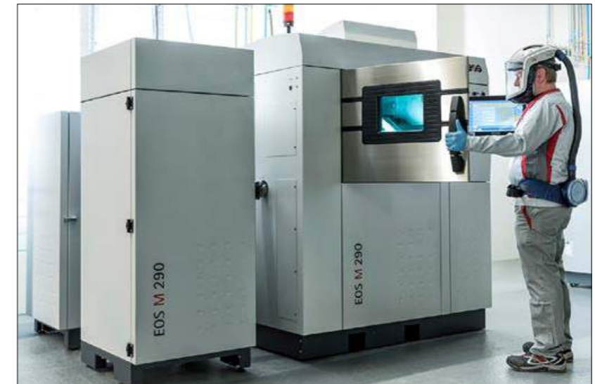
Fig. 6 Metal AM production at Audi using an EOS M 290 (Courtesy Audi AG)
