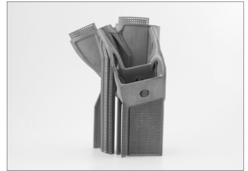
Fig. 7 This automotive part is supported by block support structures. Block support, as opposed to volumetric support, is not completely solid
