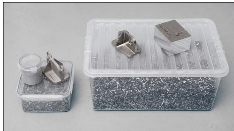
Fig. 11 This case study clearly demonstrates AM's material utilisation advantage compared to conventional processes
