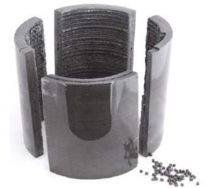
Composite pellets are melted, compounded, and extruded layer-by-layer into desired forms
