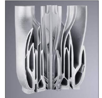
Complex interior structures can be built using laser metal fusion
