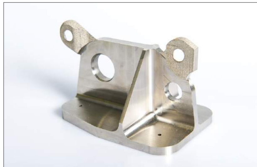
Fig. 7 A partly machined aerospace bracket produced using EBM
