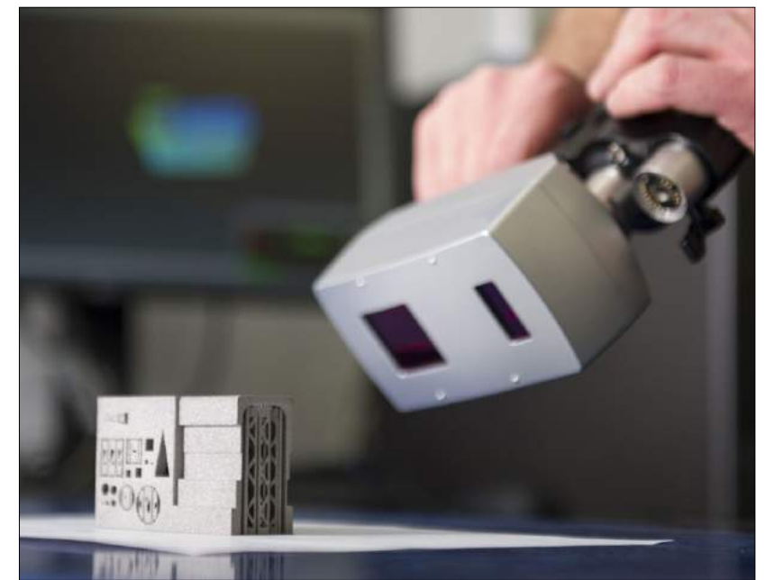
Fig. 5 A test build is analysed using a high performance laser scanner
