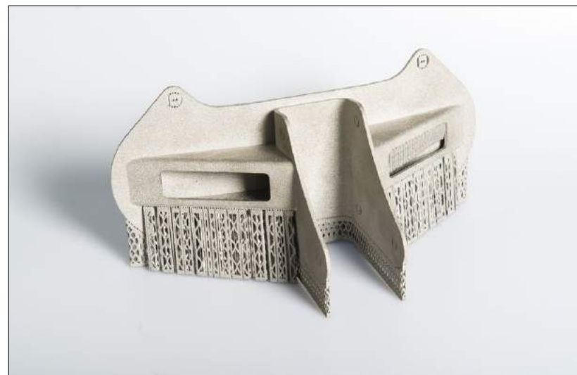
Fig. 8 An as-processed bracket prior to the removal of support structures
