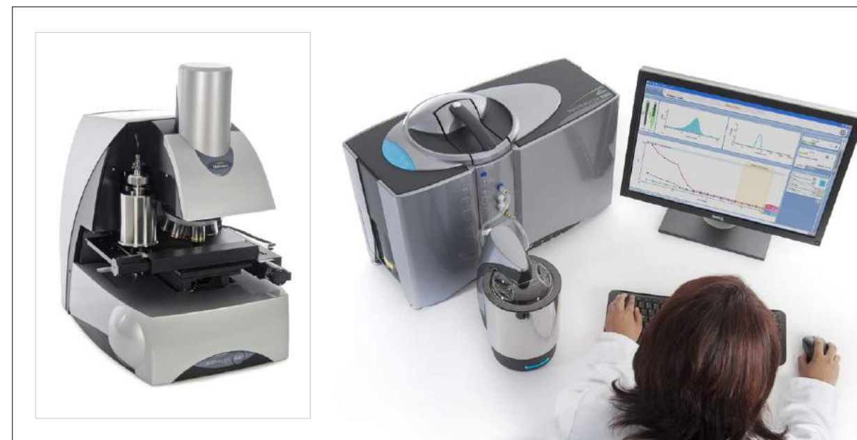
Fig. 6 High quality equipment is available for laboratory metal powder analysis of both size distribution and particle morphology but adapting these instruments for in-line monitoring would require significant development effort and current morphology measurement techniques are not suitable for 100% testing (Images courtesy of Malvern Instruments)
