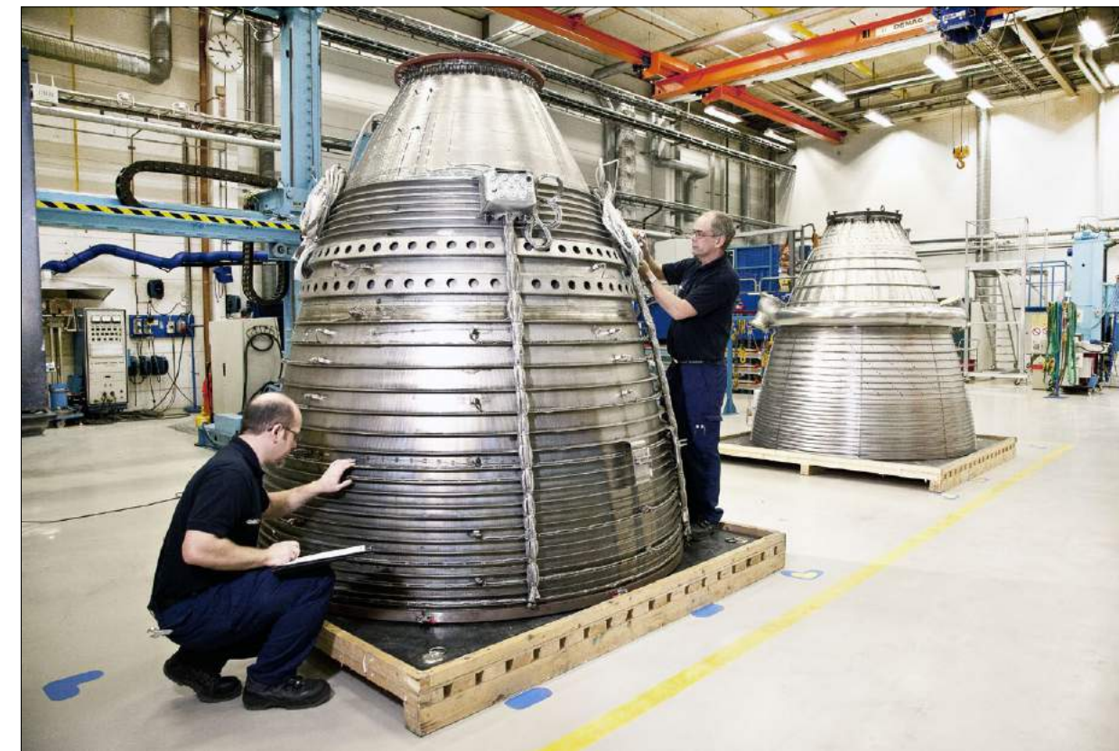
Fig. 10 In the foreground the Vulcain 2 demonstration nozzle stands with over 50 kg of Laser Wire AM deposition. It is not only used to reinforce the structure but also join to parts, which enabled significant cost savings. In the background is the Vulcain 2 nozzle for the Ariane 5 rocket
