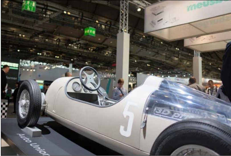
Fig. 21 A functioning scale model of a 1936 Auto Union Type C Grand Prix sports car demonstrated Audi Toolmaking's metal Additive Manufacturing capabilities
