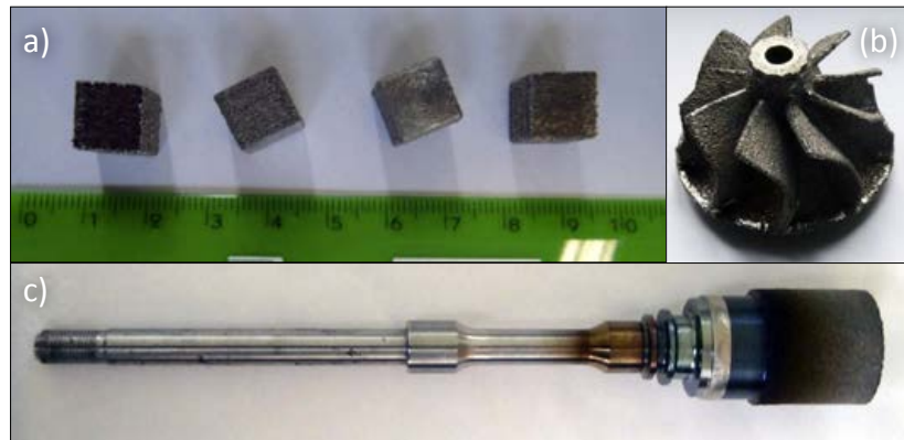
Fig. 9 (a) RNT650 EBM test samples, (b) EBW turbocharger wheel, (c) Joining trial [2]
