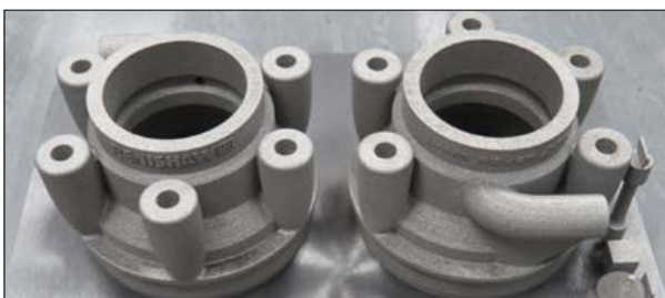
Manifold for Land Rover BAR produced on Renishaw Additive Manufacturing system (Credit Renishaw)
