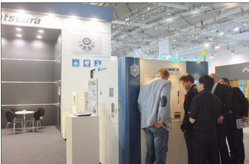
Fig. 18 Matsuura launched its Lumex Avance-25 hybrid metal laser sintering and milling machine to the European market at formnext
