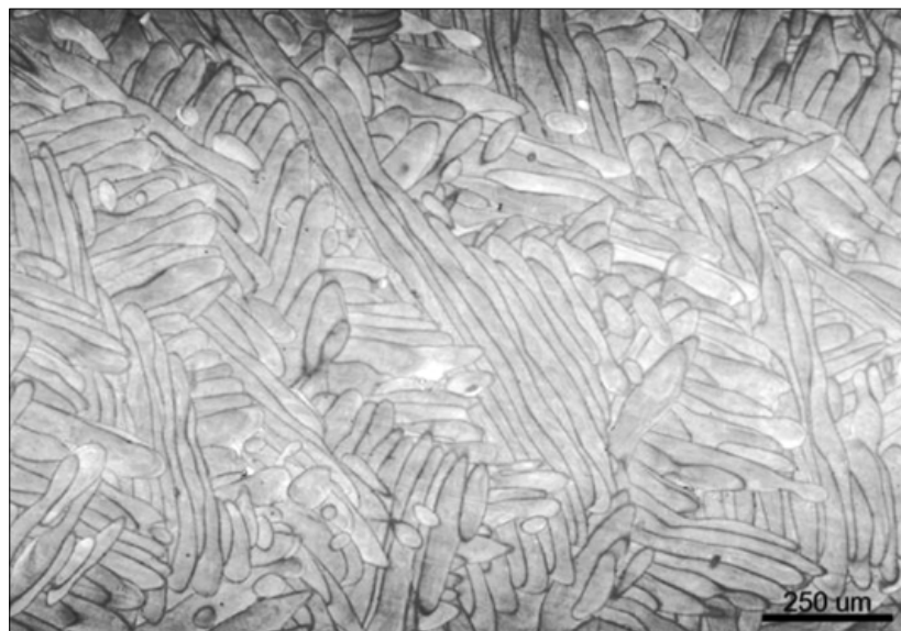
Fig. 1 As-manufactured microstructure, IN-939. Build direction is perpendicular (out of the plane) compared to the picture [1]
