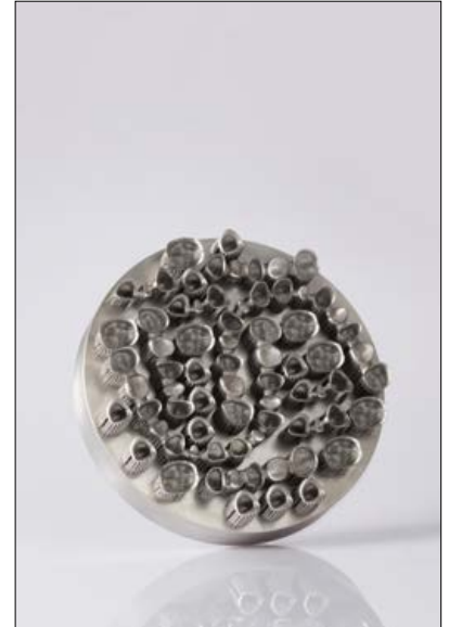
Fig. 12 The M 100 can manufacture around 70 cobalt chrome dental crowns and bridges in three hours (Courtesy EOS)
