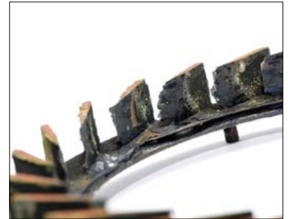
Erosion can result in lengthy repair times
