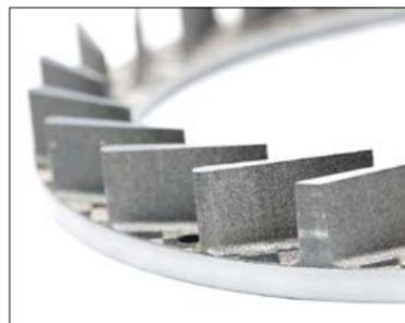
A proprietary AM process is used for the repair of turbocharger nozzle rings
