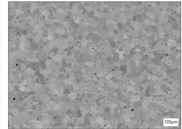
Fig. 16 Pore-and microstructure of bulk after shell-printing and sintering [4]
