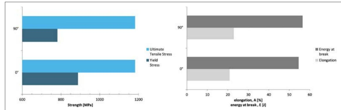
Fig. 2 Left: UTS and Yield stress for 0° and 90°, Right: Elongation and energy at fracture. As-manufactured condition [1]
