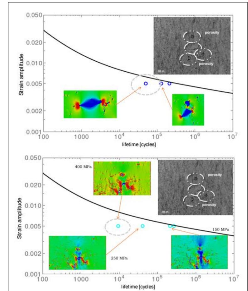
Fig. 22 Effect of residual stress (upper without, lower with residual stress) [4]
