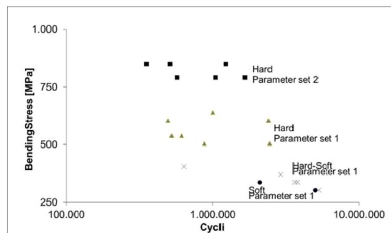
Fig. 21 Tooth bending fatigue test results [6]
