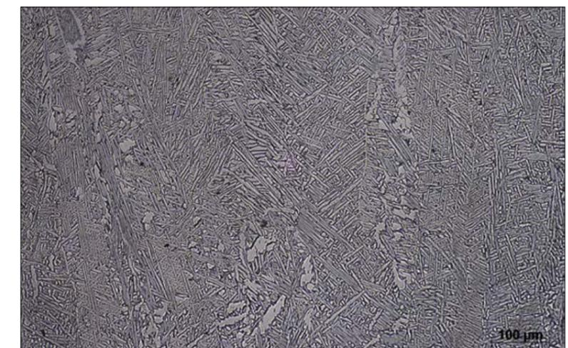
Fig. 1 Typical microstructure of EBM produced Ti-6Al-4V component with 35 mm diameter (image from centre point) [1]
