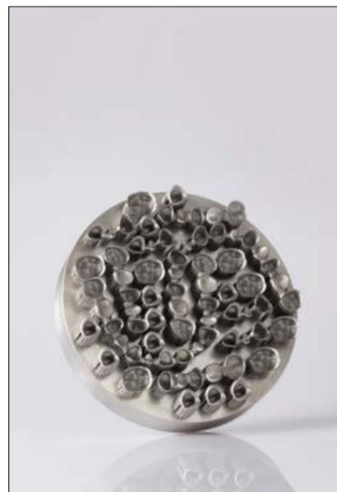
Fig. 12 The M 100 can manufacture around 70 cobalt chrome dental crowns and bridges in three hours (Courtesy EOS)
