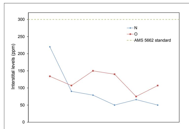
Fig. 7 Evolution of the N and O levels over the past year in Ni718 powder for laser melting powder bed application [2]
