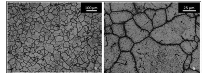
Fig. 12 Optical microscope images of Hastelloy X aged at 745°C for 3 h, after etching [3]
