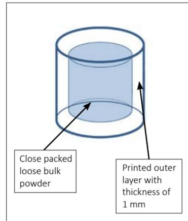
Fig. 14 Principle of shell printing [4]
