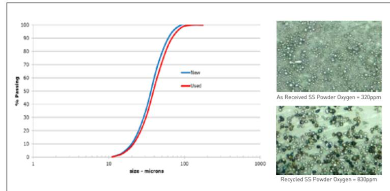
Fig. 15 PSD and visual changes from powder cycling [3]
