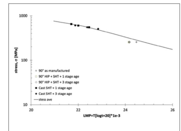
Fig. 6 Creep test results for AM IN-939 in 90° and cast IN-939 [1]
