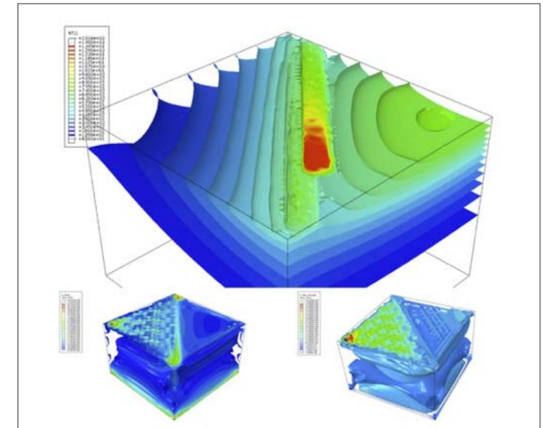
Fig. 19 Temperature isosurfaces during the simulation of the final layer and 1st principal and equivalent stresses [4]
