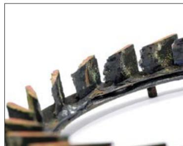
Erosion can result in lengthy repair times
