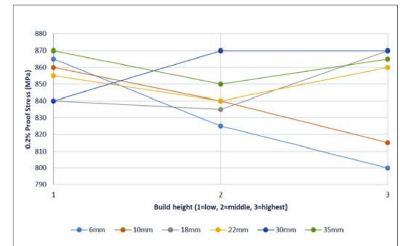
Fig. 5 Proof stress plotted versus the build height for Ti-6Al-4V component thickness [1]
