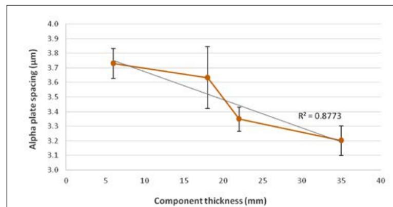
Fig. 8 Alpha plate spacing plotted versus component thickness [1]
