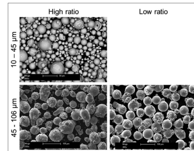
Fig. 9 SEM image of Pearl® Micro Ni718 powder for two particle size distributions (10 – 45 µm for powder bed application and 45 – 106 µm for deposition application) and two melt-to-gas mass flow rates ratios [2]
