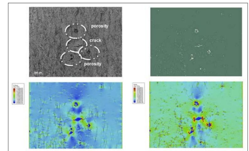
Fig. 20 Modelling procedure from upper left to lower right: microstructure, defect structure, equivalent stress and strain contours [4]
