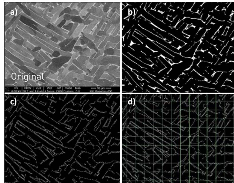
Fig. 7 Process of measuring the  $\alpha$ -plate spacing from an original SEM image (a), to threshold image distinguishing  $\alpha$  and  $\beta$  phases (b), edged image to outline phase boundaries (c) and use of linear intercept method to determine  $\alpha$ -plate spacing (d) [1]
