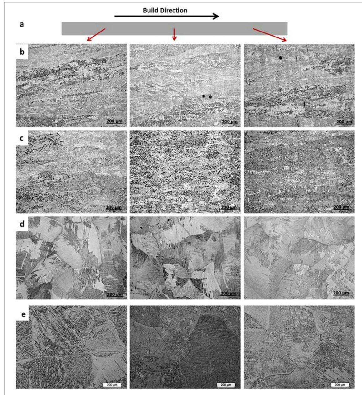
Fig. 7 (a) Build direction and micrograph position, (b) as-built samples, (c) PT1 standard HIP cycle with rapid cooling, (d) PT2 above  $\beta$ -transus HIP cycle with slow cooling (e) PT3 above  $\beta$ -transus HIP cycle with rapid quench
