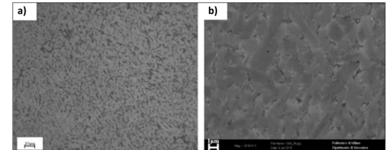
Fig. 24 Representative microstructure of 304 CS produced by SLM shown along the feeding direction (a) optical micrograph; (b) SEM micrograph [5]
