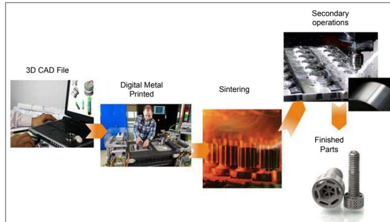
Fig. 13 Overview of the complete Digital Metal process [4]
