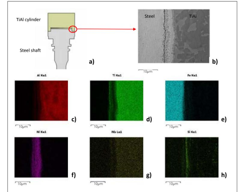
Fig. 13 (a) Joining trial scheme (section), (b) FE-SEM image at 5000x magnification of the EDS elemental mapping area, from (c) to (h) EDS elemental maps [2]
