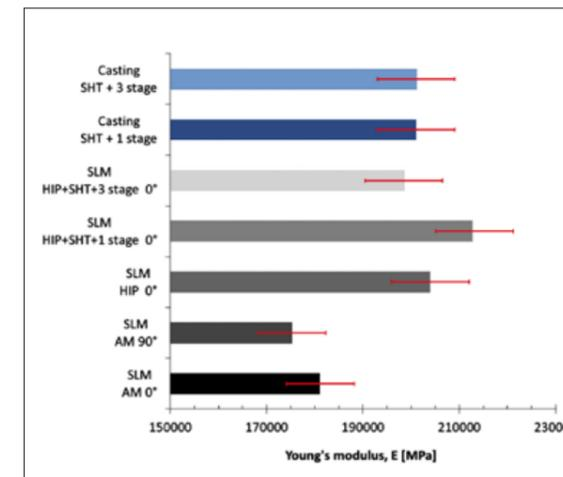
Fig. 4 Stiffness of as-manufactured and HIPed material. Data reported for AM material in the 0° direction. Typical (in-house generated) precision casting level indicated as reference [1]
