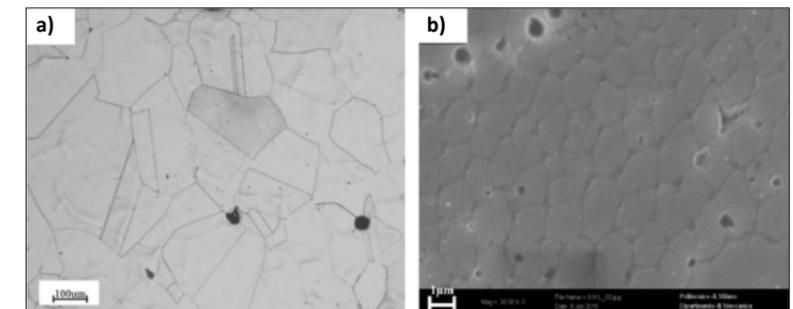
Fig. 25 Representative microstructures of austenitic 316L; (a) optical micrograph of cast 316L; (b) SEM micrograph of 316L steel along the feeding direction produced by SLM [5]
