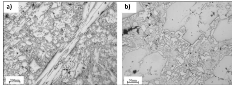
Fig. 23 Microstructure of 304 CS cast in alumina crucible [5]
