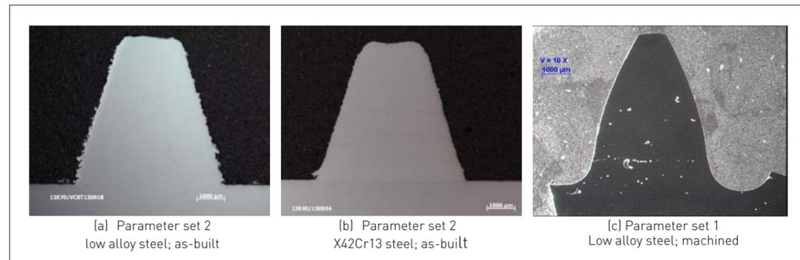
Fig. 20 Cross sections of teeth after Laser Metal Deposition [6]
