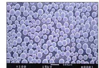
Highly flowable and pure spherical metallic powders from PyroGenesis
