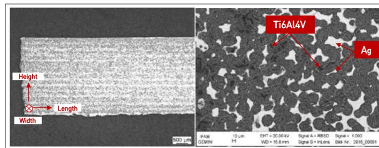
Fig. 17 Microstructure of infiltrated sample 75B [5]
