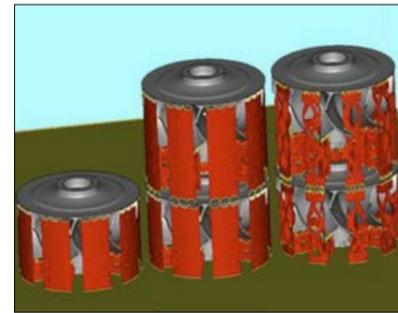
Fig. 11 Turbocharger prototypes: sample placement within build chamber with different support structures [2]
