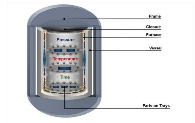
Fig. 1 A simplified schematic picture of the HIP equipment and process
