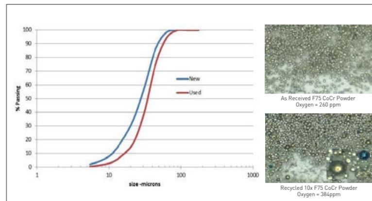
Fig. 16 PSD and visual changes from powder recycling [3]
