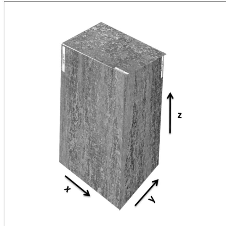
Fig. 5 Typical columnar grain structure of EBM Ti-6Al-4V [2]
