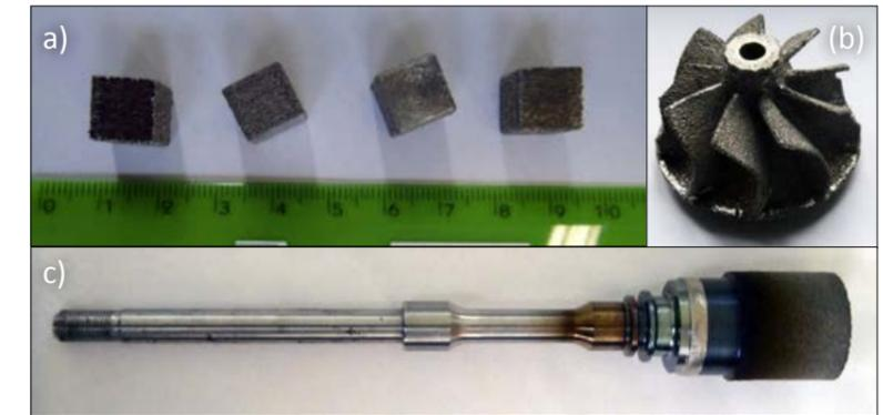
Fig. 9 (a) RNT650 EBM test samples, (b) EBM turbocharger wheel, (c) Joining trial [2]
