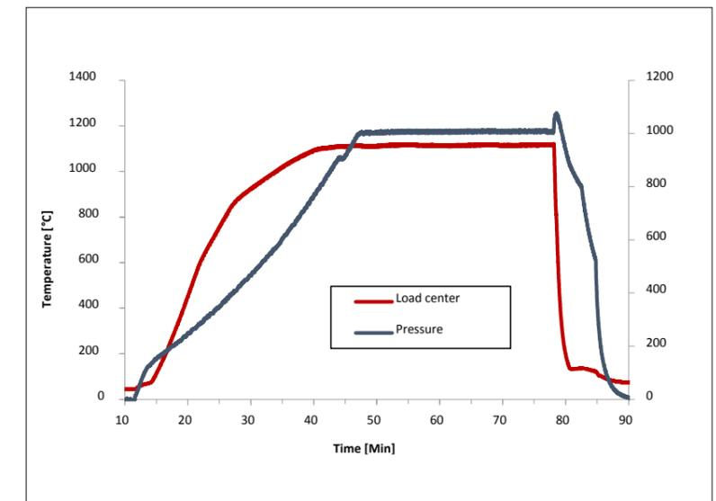
Fig. 6 PT3 HIP cycle logged data
