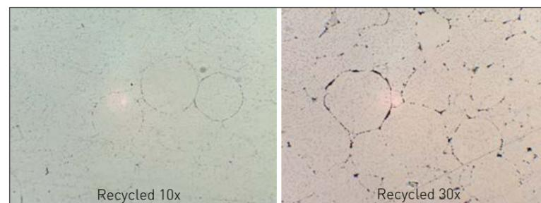
Fig. 17 Metallographic comparison of F75 at 10x and 30x recycled powder [3]
