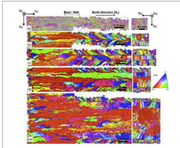
Fig. 2 EBSM maps of vertical cross sections from samples with different wall thicknesses (made with Ti-6Al-4V EBM), (a) shows an original  $\alpha$  phase map and (b) to (e) shows reconstructed  $\beta$  grain structures for 1 mm, 1.5 mm, 2 mm and 5 mm wall [1]
